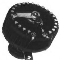
Our type R2 filament rheostat for power tubes—3.3 ohms, 4 amps. capacity
