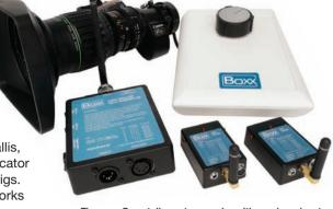
The new Boxx tally system works with any broadcast camera that uses a standard 12 pin Hirose lens cable.
