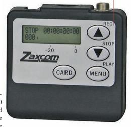
ZFR200 can output audio as either 24-bit/48-KHz timecode-stamped broadcast wave (.wav) files or timecode-stamped MP3 files. Each unit is powered with a single AA battery with up to 14 hours of run time.# # #
