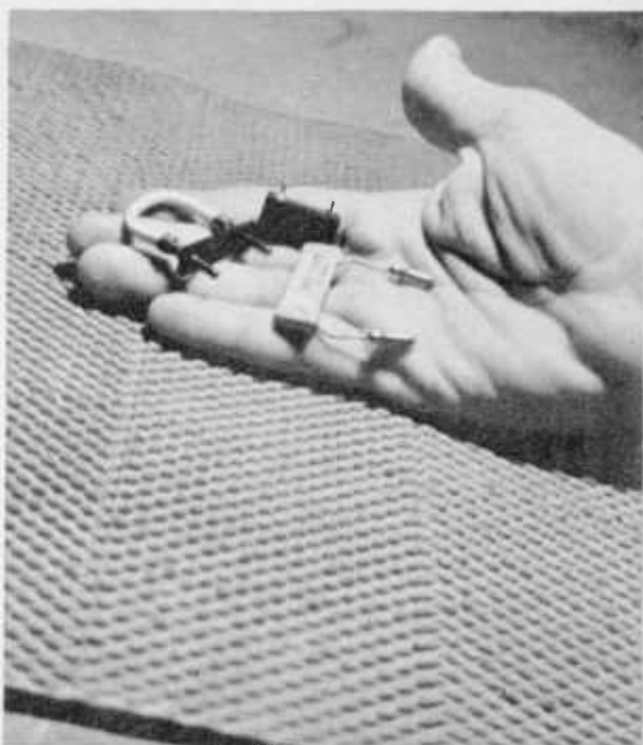
Fusistors come in many sizes, shapes and colors. They come in wire wound and also chemical state.
