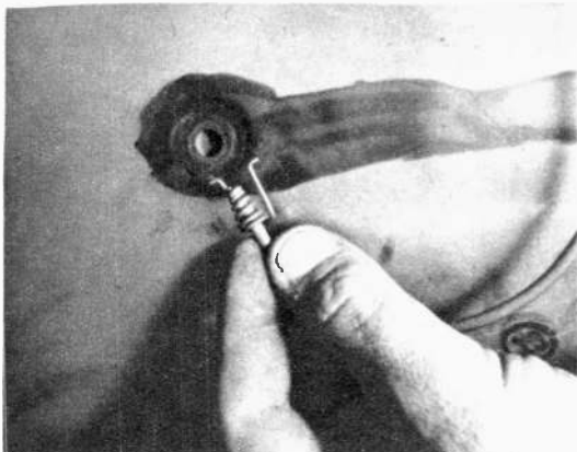
Be sure to continually discharge both anode lead and well every time you place your hands there.
