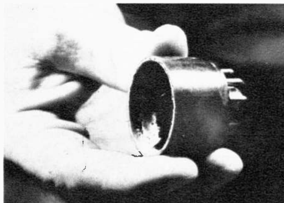
The CRT cap is only a plastic cover over glass. If the cap comes off you can thread it back on.
