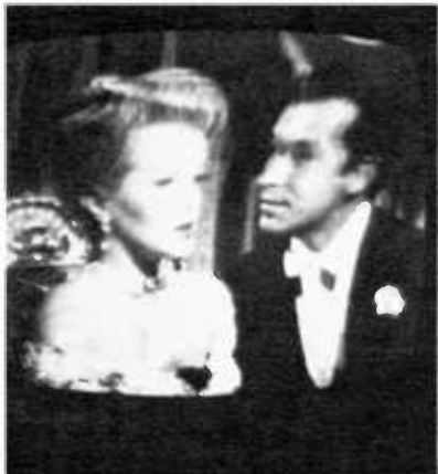
A pulsating picture that is vibrating horizontally is usually an IF tube that is oscillating.
