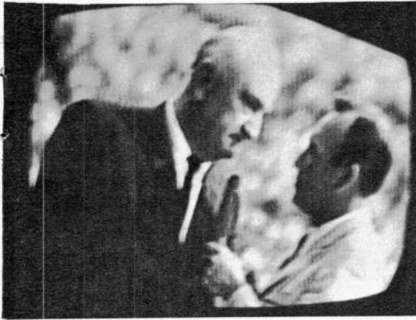
A tilted picture is easily straightened by loosening the yoke and then carefully rotating it into place.
