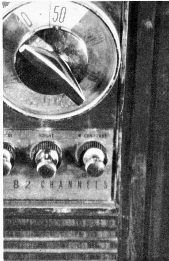
On this particular set the color tint is a duo control in combination with the brightness knob.
