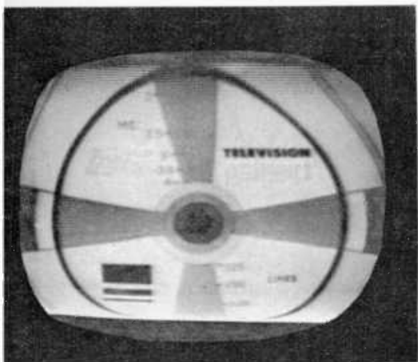
Pointed heads and stubby legs indicate vertical linearity and height control require adjustment.
