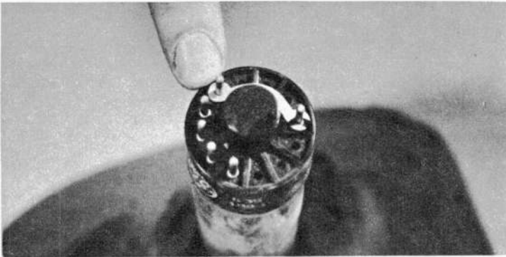
Sometimes a picture tube needs a strap between the heater and the focus anode mounted in electron gun.
