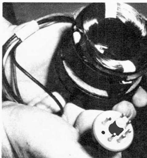
Yoke is mounted around neck of picture tube. It sweeps cathode ray, helps in making high voltage.
