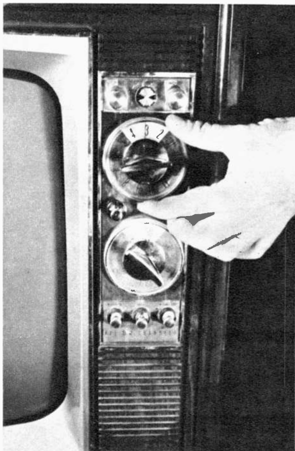
The fine tuner serves an important function for color. With a wrong setting you can lose color.
