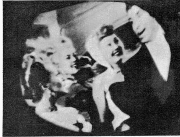
Black shadows in corner of tube are caused by yoke being mounted too far back from the bell.
