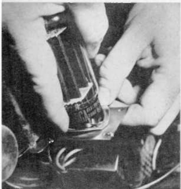
The typical low voltage rectifier tubes come in large glass envelopes. Press clip to release.
