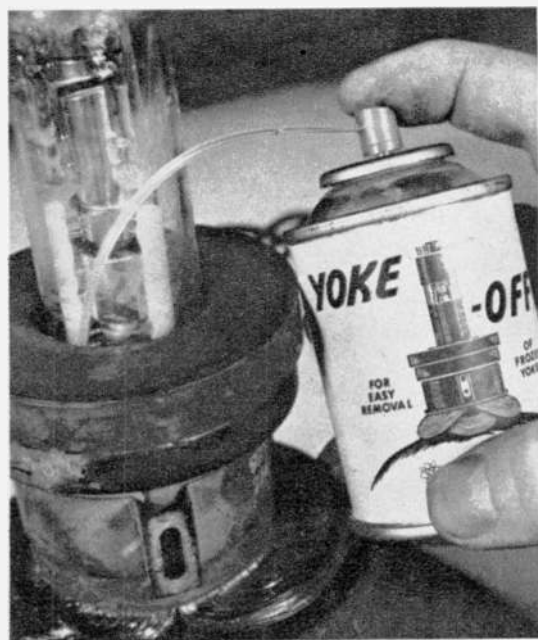
When a yoke freezes to the glass neck, it can be loosened easily with this special yoke loosener.
