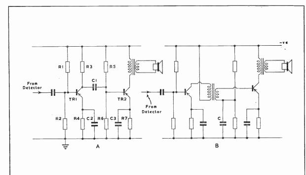
Fig. 17 Two common forms of single ended Output Audio Stages
