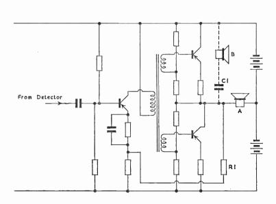
Fig. 15 Audio Section with single ended push-pull Output
