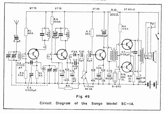
This transistor is operated in the common collector mode. Although this gives little actual gain, the transistor serves to match the relatively high impedance output of the diode to the low impedance of the fourth transistor. The output stage is Class B push-pull and drives a  $2\frac{1}{2}$ " speaker. The maximum output is 150mw.
