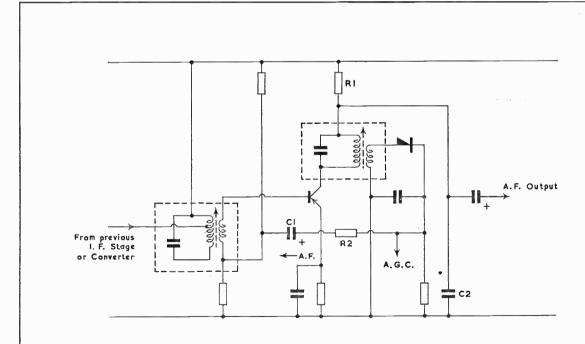
Fig. 12 Common Emitter Reflex 1, E-A.E. Amplifier
