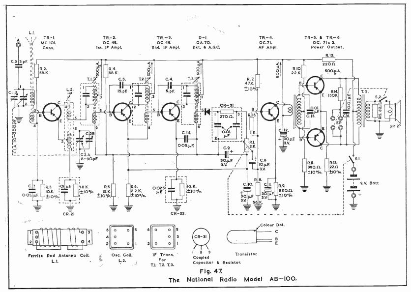
The audio amplifier uses three 0C71's, one as the driver and two in push-pull for the output stage. The output transistors can deliver 40mw. undistorted and 70mw. maximum into the primary of the output transformer. The loud-speaker used has a diameter of 2".
