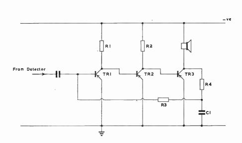
Fig. 18 Basic Three Stage Audio Section using Direct Coupling.
