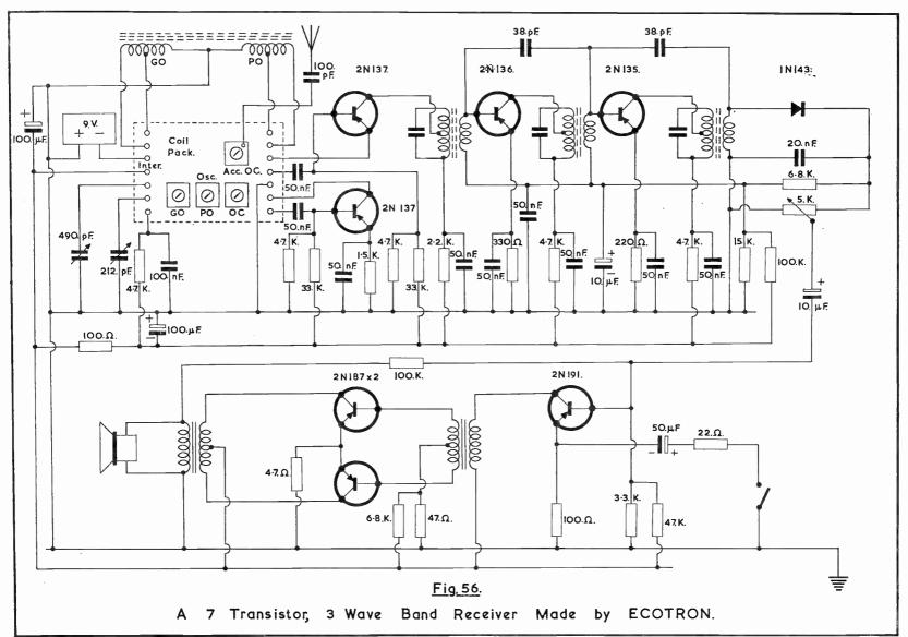
This reduces gain and so the diode acts as an auxiliary A.G.C. system augmenting the A.G.C. provided by the second detector. A.G.C. is applied only to the first I.F. stage, the second stage being operated at maximum gain all the time.
