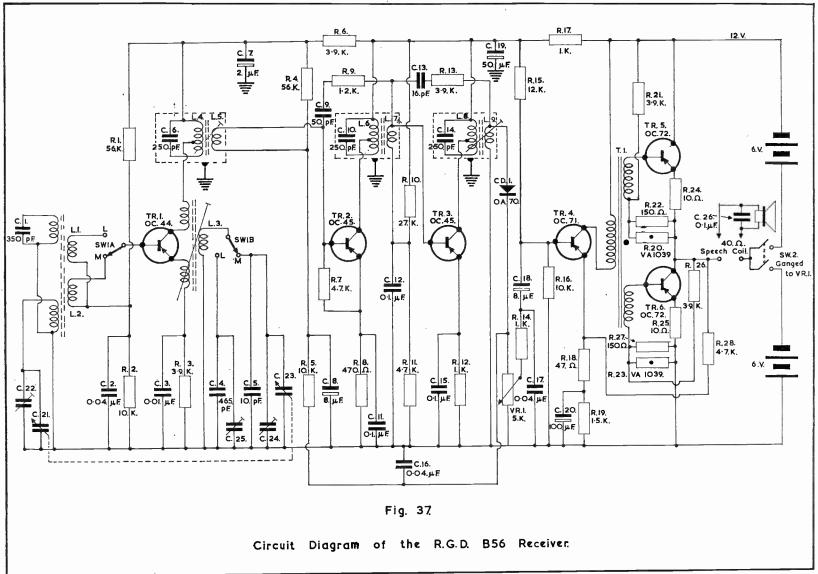
The conditions necessary for efficient and undistorted operation are that R21, R22, R20, and TR5 shall be perfectly matched to R25, R23, R27 and TR6.
