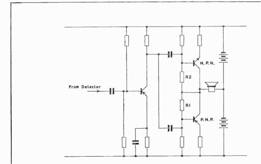
Fig. 16 Audio Section with Transformerless push-pull Output using P. N. P. and N. P. N. Transistors
