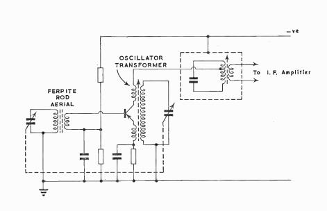
Fig. 6 An alternative type of Emitter Injected Autodyne Converter
