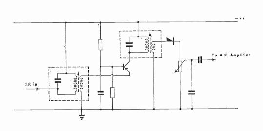
Fig.11 A typical form of Common Base I.F. Amplifier
