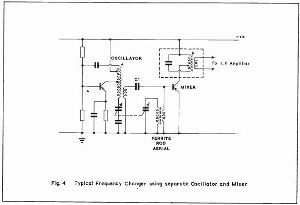
The conversion gain achieved with this circuit should be between 15 and 20 db with high gain—high frequency transistors.
