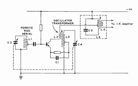
Fig. 5 A commonly used type of Autodyne Converter with Emitter Injection
