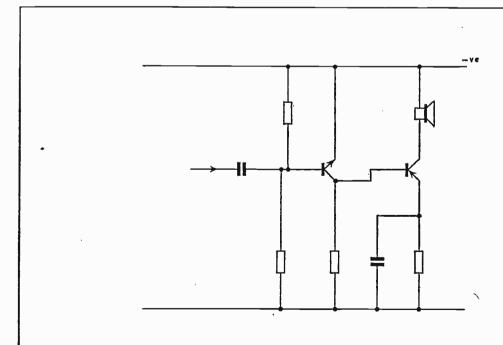
Fig. 20 Two Stage A.F. Section using P. N. P. & N. P. N. Transistors
