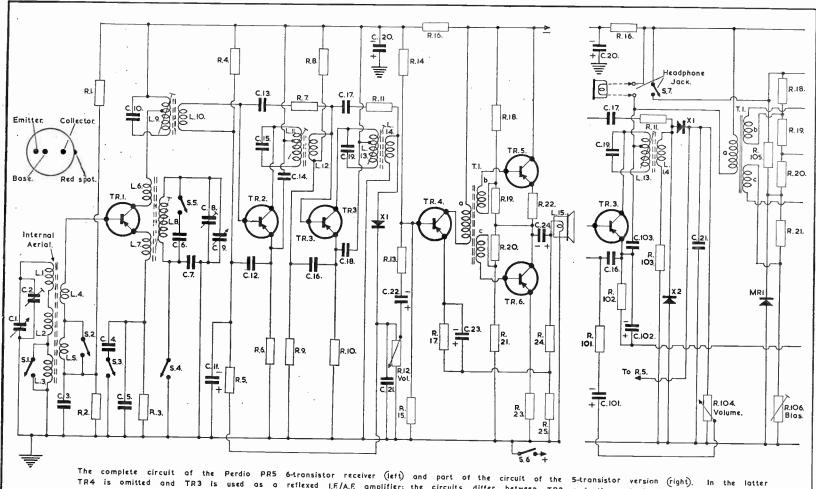
TR4 is omitted and TR3 is used as a reflexed L.F./A.F. amplifier; the circuits differ between TR3 and the output stages as shown.
