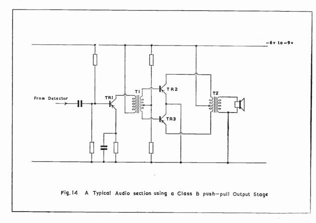
former winding. This means that the size of the transformer may be small compared with a Class A output transformer handling a similar amount of A.F. power. T2 may be, and often is, replaced by a centre tapped loudspeaker of suitable impedance. As there is no standing d.c. the cone will not be permanently displaced.
