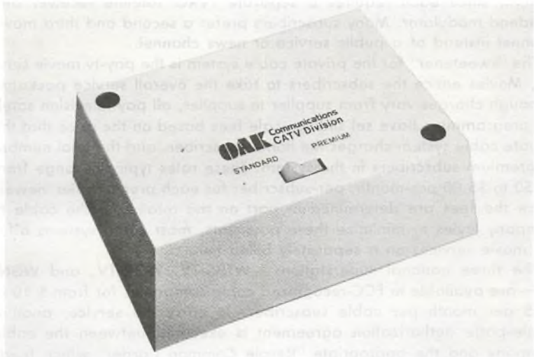
Fig. 5-11. A block converter used with an SMATV system to decode a group of channels for the local subscriber. (Courtesy Oak Communications)
