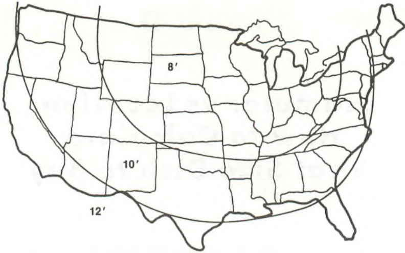
Fig. D-1. Footprint map of the US showing the minimum TVRO antenna size for good tv reception.
