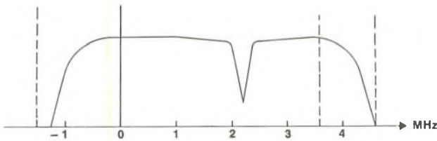
(B) Effect of trap to remove the jamming carrier(s).
