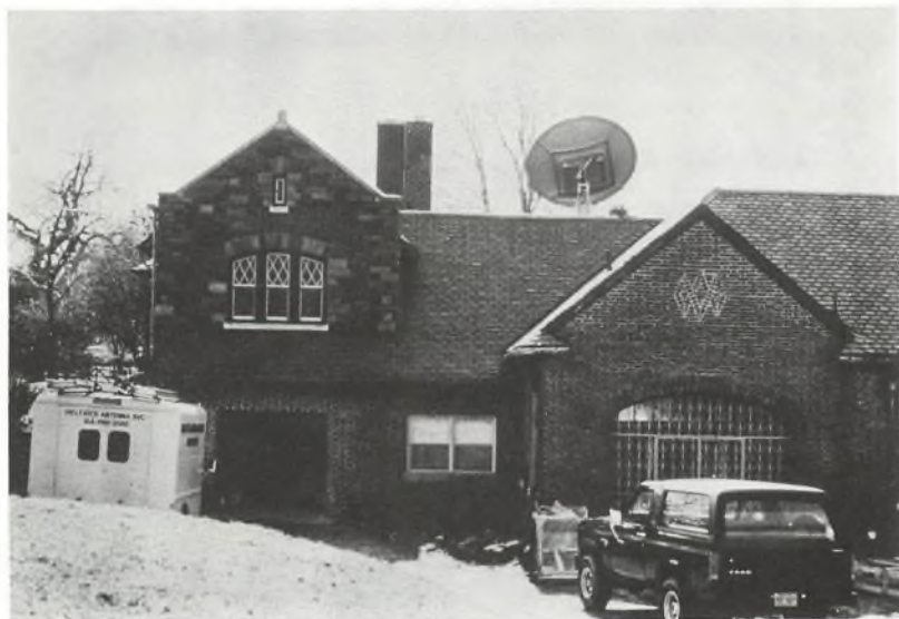
Fig. 6-11. A small TVRO antenna that can easily be mounted on the roof of a church or school building.
