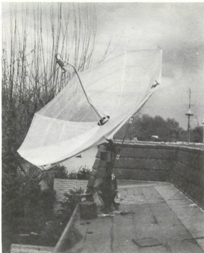
Fig. 8-7. The Paradigm 11-foot aluminum mesh dish comes knocked-down for easy assembly.
