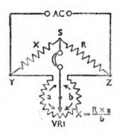
For example, if R is 10,000 ohms and gives a full-scale deflection when the test terminals are shorted, a resistance of 10,000 ohms applied across the test terminals will halve the current flowing so that the meter will read  $\cdot$ 5 mA, and this point on the scale represents 10,000 ohms. By a similar calculation, other points can be plotted for the scale.
