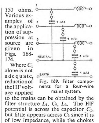
$L_1$ ,  $L_2$ , are of high impedance. Exact values of capacitance and inductance are best determined by trial, but will be within the ranges set out in Tables LVI and LVII.
