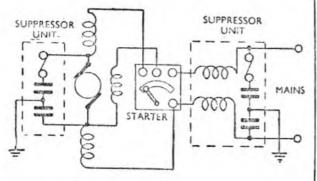
Fig. 168. Suppression applied to motor and starter.
