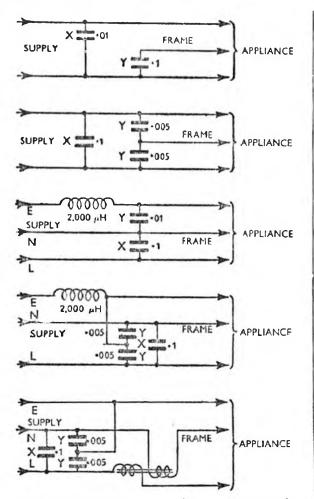
Fig. 170. Suppression filter circuits for mains leads to portable appliances.
