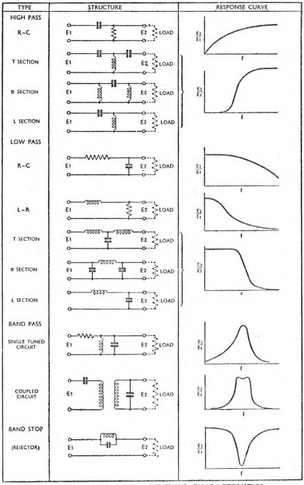
Fig. 59. FILTER CIRCUITS AND THEIR CHARACTERISTICS
