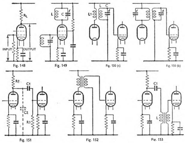
BASIC VALVE COUPLING CIRCUITS FOR HF AND LF
