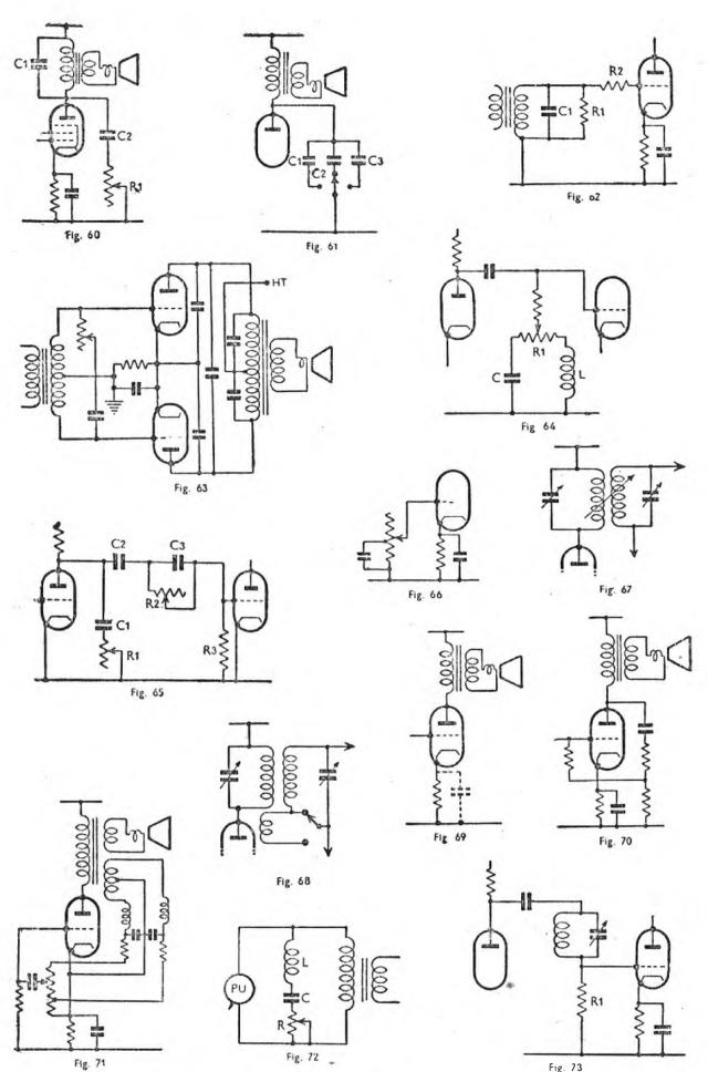
Fig. 71 Fig. 72 CIRCUITS THAT CONTROL AUDIO-FREQUENCY RESPONSE Figs. 60-73. This representative batch of tone-control circuits affords much scope for experiment, and includes methods to prevent shrillness.
