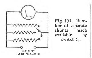
Physical Characteristics of Shunts. Shunts should be designed so that the temperature rise in the wire shall be as small as possible, otherwise their resistance values may increase with rising temperature. Shunts should, therefore, be made from wires which have a very low temperature coefficient and which are affected very little by ambient temperature changes.
