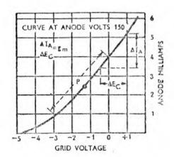
Fig. 109. Anode current/grid voltage curve of a triode valve.
