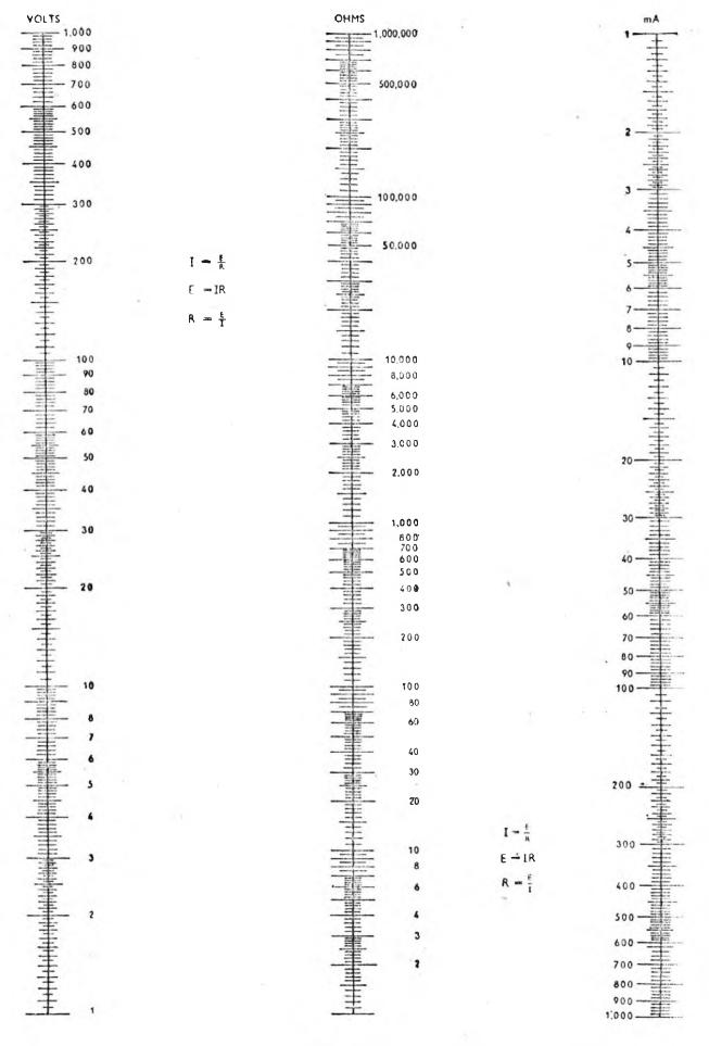
Fig. 16. ABAC 4: OHM'S LAW-VOLTS, OHMS, AMPERES
