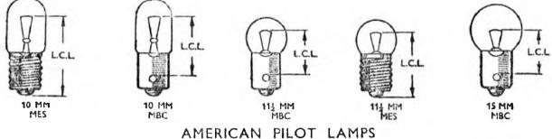
Fig. 163. Types and dimensions of the common pilot lamps in use in the U.S.A.
