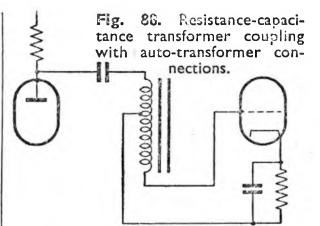
a level response well into the bass register, while low leakage inductance and self-capacitance permit efficient high-frequency response.
