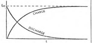
Fig. 54. How voltage across a capacitor varies during charge and discharge.
