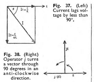
pointing downwards, while the magnitude (not the direction) of the resultant is  $\sqrt{a^2 + b^2}$ .
