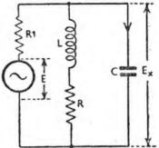
exists (as it must, since all sources have some internal resistance), the voltage across the parallel tuned circuit, which we might call  $E_x$  (Fig. 47), rises to a maximum at resonance
