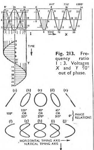
Fig. 214. Oscillograph traces indicate by shape and tilt the phase relations of waves having known frequency relationship.
