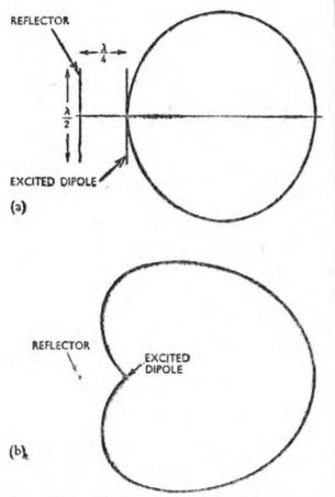
Fig. 237. (a) Vertical directivity curve of dipole with reflector. (b) Horizontal directivity curve of dipole with reflector.
