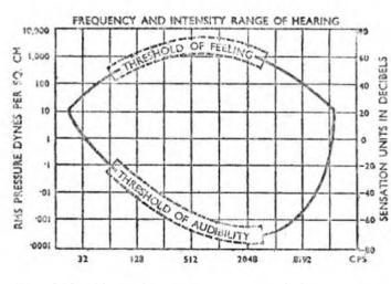
Fig. 183. How the average normal human ear responds to sound waves of different intensities and frequencies.
