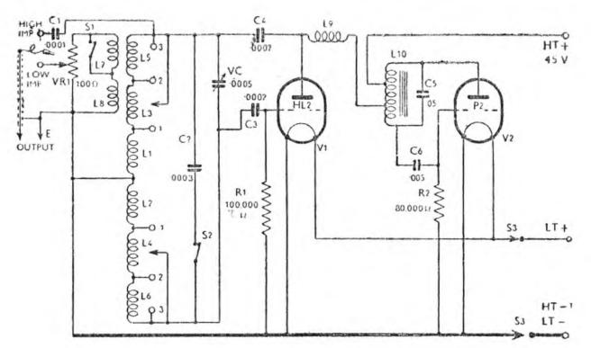
CIRCUIT FOR A BATTERY-DRIVEN SERVICE OSCILLATOR Fig. 202.  $V_1$  with its associated tuning circuit generates high-frequency oscillations which are modulated at audio-frequency by oscillations generated by  $V_2$  stage. Radio-frequency output can be calibrated against known frequencies.
