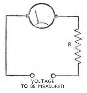
1 volt is applied to the test terminals.
