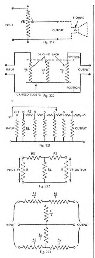
Fig. 219. Attenuator or volume control applied to a loudspeaker. Fig. 220. Three ganged potential dividers for attenuation with little effect on impedance matching. Fig. 221. Resistance network for attenuation with constant impedance. Fig. 222. Simple Tee attenuator. Fig. 223. Attenuator of two Tee units back to back.
