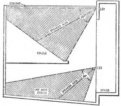
Fig. 188. Distribution angle of a speaker assists in preventing reflections. Note how the maximum sound from the upper speaker is kept parallel to the ceiling.
