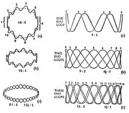
number of peaks on Fig. 216. (Left) Figure obtained with phase-splitting the top of the figure, circuit. Fig. 217. (Right) Frequency ratio determination and the number of loops by examination of peaks and end loops. These are 'flat' at one end. This is well patterns obtained when not using phase-splitting circuit.
