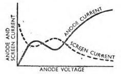
Fig. 106. Anode and screen current curves of a screen-grid valve have a characteristic kink.
