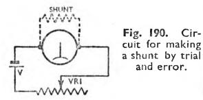
is less than that taken by the meter for full-scale deflection. For example, a 10-mA meter with a 3-volt dry cell would require a resistor of resistance at least 300 ohms, because, from Ohm's Law,  $R = \frac{E}{I} = \frac{3}{.01} =$ 300 ohms.
