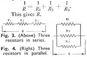
Resistance networks. The total resistance of some forms of resistance networks can be found by calculating the resistance of groups of resistors forming the network, until the network is resolved into the simplest form containing what are effectively a number of single resistors in series or one resistor. This method cannot be used in all cases (e.g. certain bridges), and the use of Kirchhoff's laws is then convenient.
