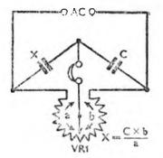
Fig. 199. Bridge circuit for finding reactance of X when C and ratio a/b are known.
