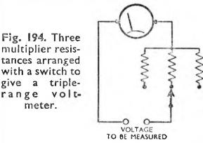
of the meter must be taken into account. For example, if the resistance of the meter is 50 ohms, then the multiplier should have a resistance of 950 ohms on the I-volt range, and 9,950 ohms on the 10-volt range.
