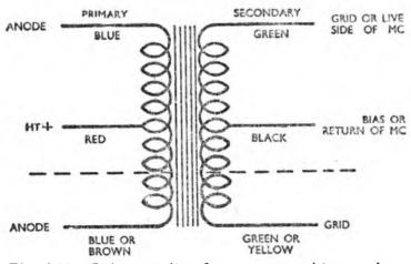
Fig. 165. Colour coding for output and intervalve transformers.
