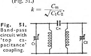
Types (1) are most commonly used for coupling between valve stages; for example, in the IF amplifiers of super-heterodyne receivers, while the remaining types are met with more usually in the aerial coupling circuits of the pre-selector stage.
