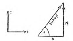
Fig. 41. (Left) Shows voltage and current in a capacitor, and Fig. 42 (Right) the appropriate impedance triangle.
