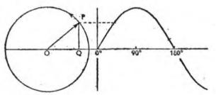
Fig. 26. Showing how a sine curve is developed by using basic principles.
