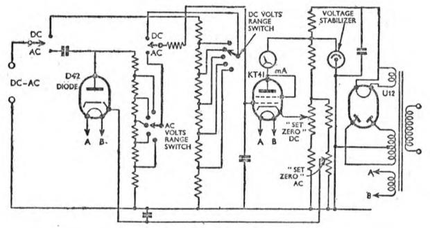
MAINS-DRIVEN VALVE VOLTMETER FOR AC AND DC READINGS Fig. 229. Showing a direct-voltage valve voltmeter with the addition of a diode and separate range resistance network for reading alternating voltages.
