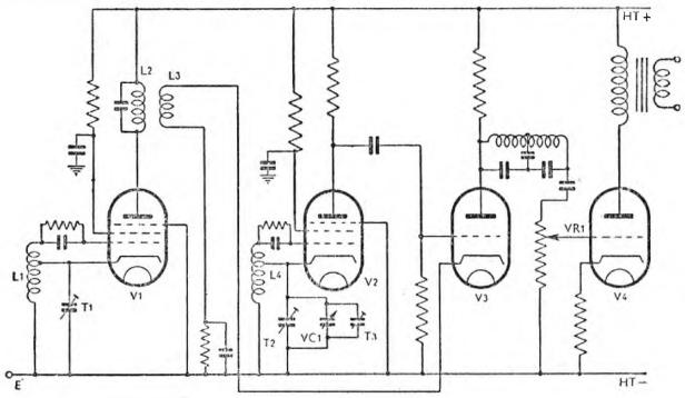
ANOTHER AUDIO-FREQUENCY OSCILLATOR CIRCUIT Fig. 205.  $V_1$  and  $V_2$  are two high-frequency oscillators. Their outputs are combined, forming in  $V_3$  an audio-frequency beat signal which is amplified by  $V_4$ .
