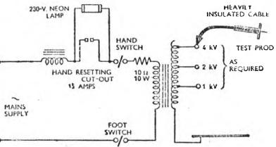
Fig. 87. Circuit for a high-voltage flash tester.
