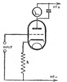
Fig. 225. Mains-driven version of Fig. 224. R not only biases the valve, but extends the input volts range.
