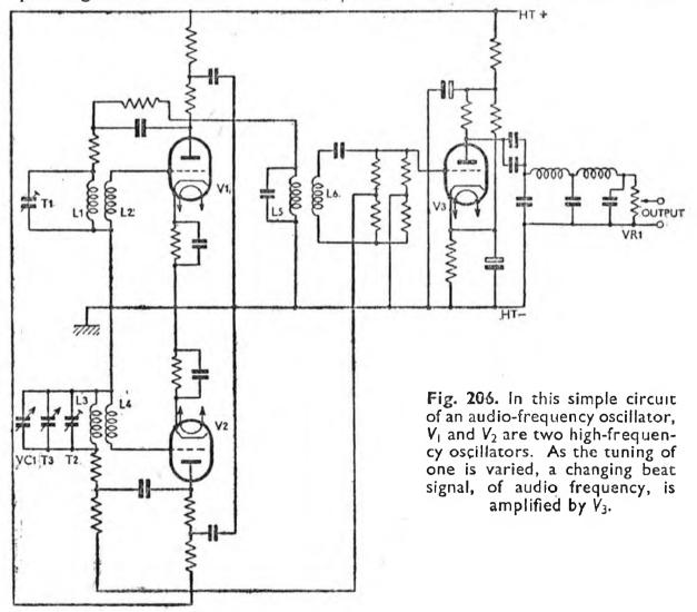
be used as the source of known frequency, and the remainder of the BFO scale calibrated.
