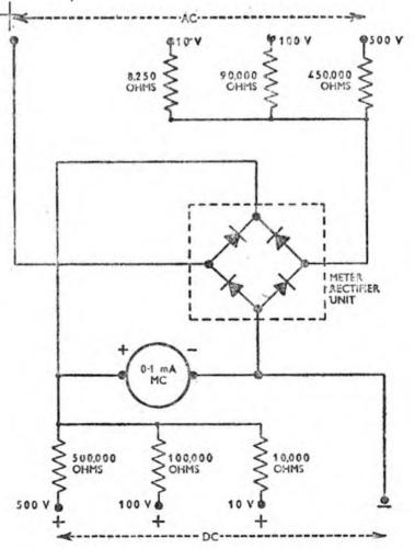
voltmeter and the current Fig. 196. Circuit for a triple-range AC-DC voltmeter. required to operate it (which Note the lower values of AC multipliers to compensate for voltage drop across rectifier unit.
