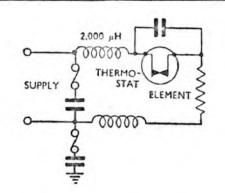
Fig. 171. Suppressor for a thermostat as fitted to a refrigerator or cooker. It consists of two 2,000-microhenry chokes in series with the appliance and a parallel capacitor of .005 mFd or more.
