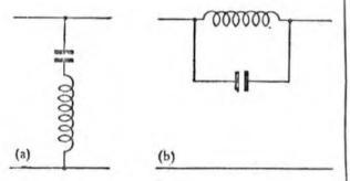
Fig. 58. Basic forms of tuned circuit. (a) Series and (b) parallel.
