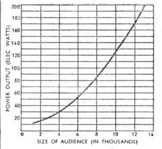
Fig. 184. Approximate power required for public-address installations which cater for an open-air audience.
