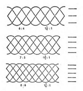
Fig. 218. Frequency ratio determination by peaks and lines of intersection.
