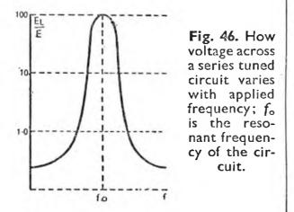
circuit, is  $\approx \pm \frac{2\Delta f}{f_0}$ , so that  $Z_{po} = \frac{\omega_0 L Q_0}{1 \pm j \frac{2\Delta f}{f_0} Q_0}$  $= \frac{\omega_0 L}{\frac{1}{Q_0} \pm j \frac{2\Delta f}{f_0}}$
