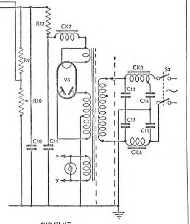
CIRCUIT RF oscillator, and  $V_2$ , with associated components, generates audio-frequency modulation.  $V_3$  is the full-wave mains rectifier. previously mentioned, and switches have been incorporated to enable the output from the instrument to be connected to the LF modulator valve, so as to obtain an audiofrequency output. This is arranged by feeding the switch  $S_4$  (contact 6) from the anode circuit of  $V_2$  via  $C_6$ .
