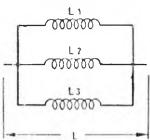
Inductors are treated as resistors; when in series their values are added, when in parallel the reciprocal of the total inductance is given by the sum of the re-
