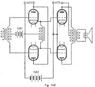
Fig. 157. Output valves connected in parallel. Fig. 158. Transformer-fed push-pull output stage. Fig. 159. Graphical representation of pushpull operation. Fig. 160. Push-pull stage cathode-coupled to a push-pull output stage. Fig. 161. RC coupling to push-pull output using paraphase stages. Fig. 162. Two methods of connecting a 'phase splitter' valve when using resistance-capacitance coupling to push-pull valves.
