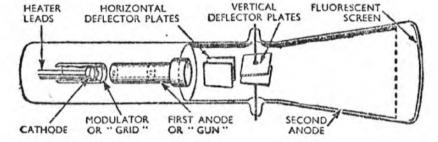
Fig. 207. Simplified sectional diagram of a cathode-ray tube emelectrostatic ploying deflection.
