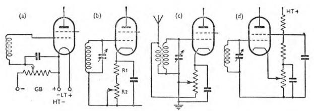
FOUR MANUAL VOLUME-CONTROL CIRCUITS FOR HF STAGES Fig. 95. (a) Variation of the battery grid bias; (b) variation of the cathode bias; (c) simultaneous regulation of aerial input and cathode bias; (d) an improved cathode bias control circuit.
