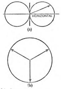
Fig. 236. Directivity curves of vertical dipole in free space. (a) Vertical directivity curve; length of the arrow indicates the intensity of radiation in that direction. (b) Horizontal directivity curve; the dipole radiates equally well in all horizontal directions.
