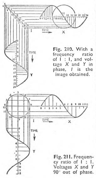
of the voltages is known, the frequency of the other voltage can be determined by knowledge of the resultant of combination.
