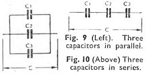
C of the combination is given by  $\frac{1}{C} = \frac{1}{C_b} + \frac{1}{C_4}$ . This gives C. If this process were done algebraically, the value of C would be,
