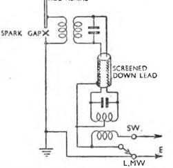
Fig. 178. Anti-static lead-in system used with Belling Lee 'Skyrod' aerial.
