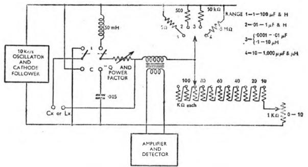
**Fig. 78.** Gives direct readings of impedance of a capacitor or an inductor.
