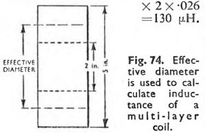
When dealing with a multi-layer coil, d is mean diameter, that is, the inside diameter of the coil plus half the difference of the inside and outside diameters. The inside diameter of the coil shown in Fig. 74 is 2 in., and the outside diameter 5 in., so that the effective value of d to be used in finding the inductance is :
