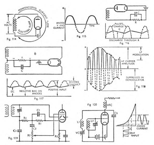
CIRCUITS FOR RECTIFICATION AND DEMODULATION Figs. 114, 115. Illustrating the principle of rectification. Fig. 116. Use of filter. Fig. 117. Full-wave rectifier. Fig. 118. Principle of demodulation. Fig. 119. Using diode for demodulation. Fig. 120. Anode-bend 'detection'.
