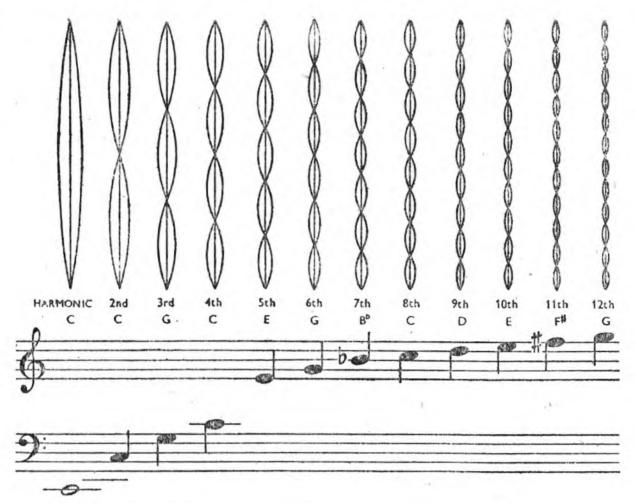
HARMONICS WITH CORRESPONDING VIBRATIONS Fig. 182. Fundamental vibration of a cord and its harmonics. If the length of the cord is such that the fundamental is C, the harmonics have the notation shown.
