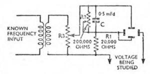
Fig. 215. Method of applying two wave forms with phase shift control.
