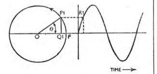
Fig. 18. Derivation of a sine curve.
