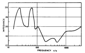
FIG. 5.18. Experimental impedance curve of Goodman's Axiom 12-inch unit, Type 150, Mk. II, in a reflex enclosure which has a  $1\frac{1}{2}$ -inch slate front.
