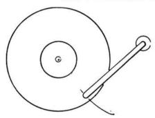
FIG. 7.18. Illustrating tracking error. The broken line shows the path traced by the recording stylus and the full line the path traced by the reproducing stylus.
