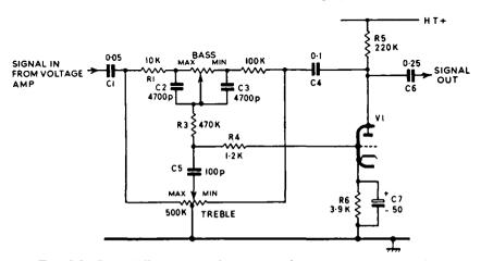
FIG. 2.8. Baxandall tone-control circuit, with typical component values.
