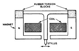
FIG. 7.2. Moving-armature pick-up unit.
