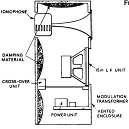
FIG. 5.5. Suggested cabinet and mounting for the ionophone.
