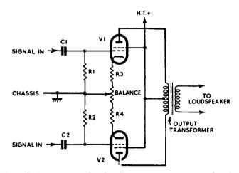
FIG. 3.8. Basic circuit of push-pull output stage using tetrode valves.
