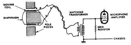
FIG. 8.2. The moving-coil (dynamic) microphone. Its low impedance requires the use of a matching transformer.
