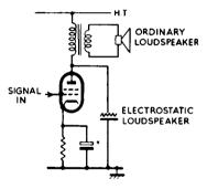
the low-impedance polarizing source from short-circuiting the signal. For the simple application of an electrostatic unit, the h.t. voltage at the anode of the output valve can be used as a polarizing voltage, as shown in Fig. 5.7. This voltage is varying at the signal frequency, and is fairly high
