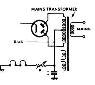
In very high-gain low-level stages the valve heaters are sometimes energized by direct current as a means of reducing the hum level. If the required d.c. is not obtained from a small l.t. rectifier in association with an l.t. winding on the mains transformer, the h.t. current is suitably adjusted and allowed to pass through the heater chain.
