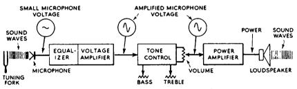
FIG. 1.6. Block diagram of the three main sections of a hi-fi amplifier.
