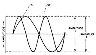
F1G. 6.2. Diagram of constant-amplitude recording for two frequencies.
