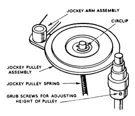
ment is shown in Fig. 7.14. The jockey wheel is made of hard rubber, and should therefore be kept absolutely free from oil or grease.
