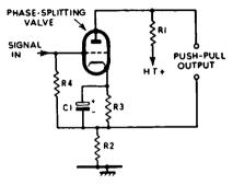
FIG. 3.11. In order to obtain sufficient drive signal for the push-pull power valves, additional amplifying valves may be necessary, as shown.
