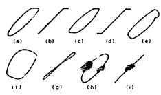
FIG. 4.12. Phase-shift patterns. The waveforms at (a) to (c) reveal clipping of the output signal due to overloading or incorrect operating conditions of the valves: (f) and (g) show the presence of harmonic distortion as the result of excessive non-linearity: waveforms (h) and (i) show the presence of a spurious signal.
