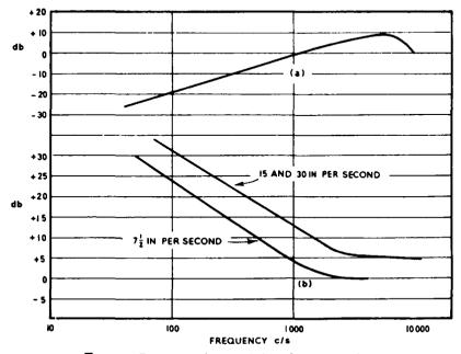
FIG. 9.9. Frequency characteristics of tape recording.
