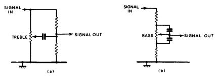
FIG. 2.9. Two simple resistor-capacitor passive tone-control circuits: (a) providing control of treble and (b) control of bass.
