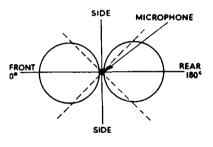
FIG. 8.6. The figure-of-eight response of pressure-gradient microphones.
