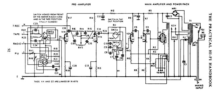
FIG. 4.14. Circuit diagram of the Pye Mozart combined pre-amplifier and power amplifier.
