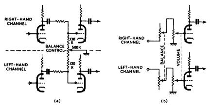
FIG. 10.11. Two balance-control systems: (a) circuit with variable loading; (b) with balance control associated with ganged volume control.
