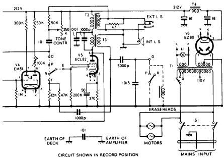
The "record/replay" switch is actuated by a relay whose winding —denoted R/P switch solenoid on the diagram—is energized by the instantaneous shorting together of the two wires labelled "brake" on the diagram. This action trips the relay switch so that it returns to the "replay" position. It is necessary to re-set the switch to the "record" position by pressing the appropriate button on the amplifier control panel.
