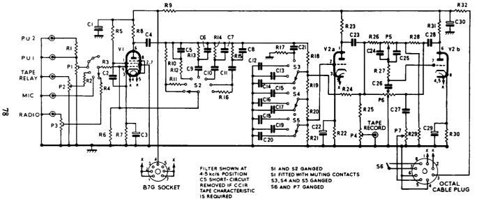
FIG. 4.2. Circuit diagram of the RD Junior control unit, Mk. II.
