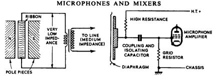
(Left) FIG. 8.3. The ribbon microphone. Its very low output impedance usually requires the use of a microphone transformer in the housing to produce a reasonable line impedance. (Right) FIG. 8.4. The condenser microphone requires a polarizing voltage, which is obtained from the h.t. line through a resistor.
