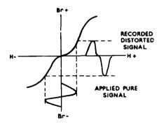
FIG. 9.3. The transfer characteristic of the remanence curve, showing how the kink in the curve distorts the recorded signal.
