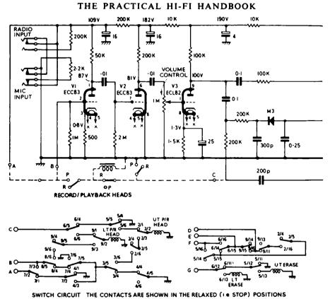
FIG. 9.11. Circuit diagram of the Sound Sales A20 tape recorder. Connexions shown as dotted lines in the circuit diagram are simplifications of switch connexions, the true connexions being given in the lower diagram.
