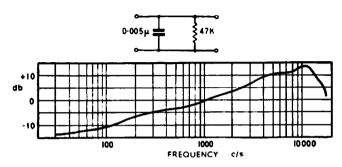
FIG. 7.11. The network recommended for the Acos Black Shadow pick-up to provide a velocity characteristic as shown by the curve. This enables the pick-up to be connected by way of the magnetic pick-up terminals of the control unit.
