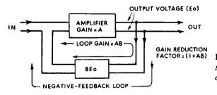
FIG. 2.4. Block diagram showing the application of negative feedback to an amplifier.
