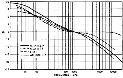
FIG. 2.6. Equalization curves in current use.
