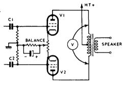
remaining circuit elements should be checked for balance. If a valve tester is not available, and it is found that the voltmeter pointer remains one side of zero over the full range of the "balance" control, the position of the output valves should be reversed. A low-emission valve is definitely responsible if this change causes the voltmeter pointer to remain on the other side of zero over the full range of the "balance" control.
