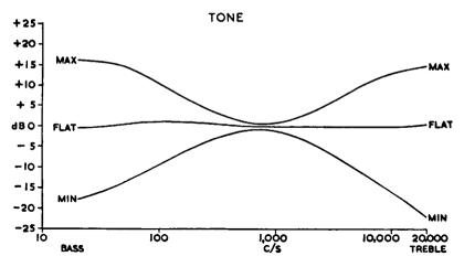
FIG. 1.5. Curves showing how the bass and treble response of an amplifier can be altered to suit the acoustics of the listening room.
