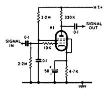
FIG. 2.1. Pentode voltage-amplifier stage.
