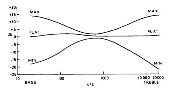
FIG. 2.18. Tone-control characteristics of the Pye HF25A pre-amplifier.
