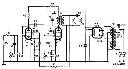
FIG. 3.3. Circuit diagram of the Cossor 562K amplifier kit. The component values are given below.
