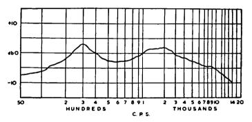
FIG. 5.1. Response curve of the WB 8-inch loudspeaker, Model HF816.
