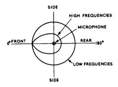
does not respond at all to sounds arriving at the sides but has a usable response over about 100 deg. both at the front and rear. The polar response can, however,
