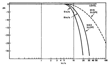
FIG. 2.10. Two-position filter characteristic with a slope control.
