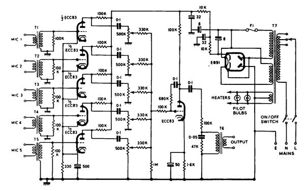
FIG. 8.8. Circuit diagram of the Pumphonic mixer unit, Model 5W/600.
