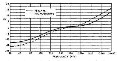
(Opposite page) FIG. 6.4. Recording characteristics approximating those used by leading record manufacturers. (Above) FIG. 6.5. Recording characteristic equal to B.S. 1928: 1955.
