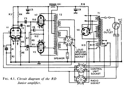
at a fairly high temperature, and if they are only just warm there is a strong likelihood of a burnt-out h.t. rectifier valve, V4; failing that, the h.t. feed resistor R14 should be subjected to a continuity test. It is surprising how much can be done in the way of simple servicing and diagnosis without instruments —merely by applying a little well-concentrated thought.
