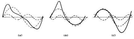
FIG. 4.6. Various modes of second-harmonic distortion.
