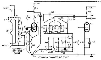
FIG. 4.16. Circuit of input stage, showing common connecting points.
