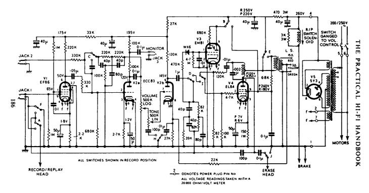
FIG. 9.10. Circuit diagram of the Truvox Type K tape-recorder amplifier.
