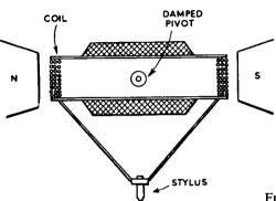
dynamo whose output voltage is governed by the speed (velocity) of the driving wheel. The latter type rely upon the property of Rochelle salt crystals of producing a potential difference when subjected to changes of pressure.
