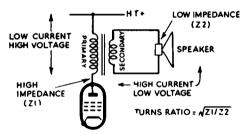
FIG. 3.1. Matching the speaker to the output stage is an important consideration in hi-fi practice.
