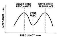
As the frequency decreases below the resonance of the enclosure, the output from the vent falls off, but the output from the speaker rises due to a lowering of its resonant frequency as the result of the air-pressure build-up between cone and vent. However, since the sounds from the two sources approach the anti-phase condition, the resultant sound output diminishes fairly quickly, and no useful increase in bass response is obtained by lowering the resonance of the loudspeaker.
