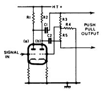
FIG. 3.13. Circuit diagram of a floating paraphase inverter stage.
