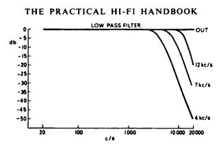
FIG. 2.19. Filter characteristics of the Pye HF25A pre-amplifier.
