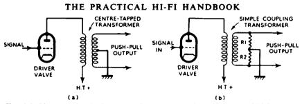
FIG. 3.9. Phase-splitting (a) by means of a centre-tapped transformer, and (b) by means of a simple transformer and resistive divider.
