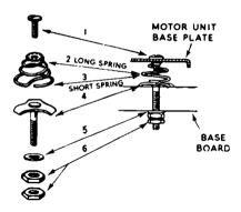
Fig. 7.15. The Goldring-Lenco method of player-unit suspension.
