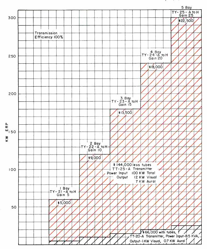
Figure 18 E.R.P. VS. 1 KW AND 12 KW TRANSMITTER-ANTENNA COMBINATIONS FOR UHF CHANNELS 14–83
