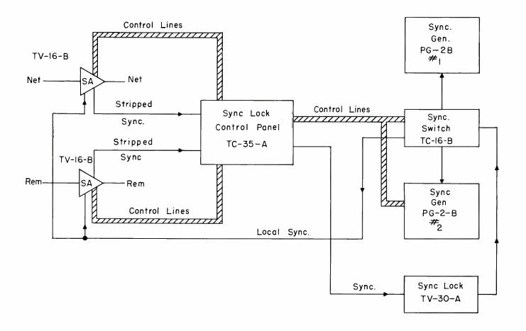
Figure 2 SYNC-LOCK CONTROL SYSTEM
