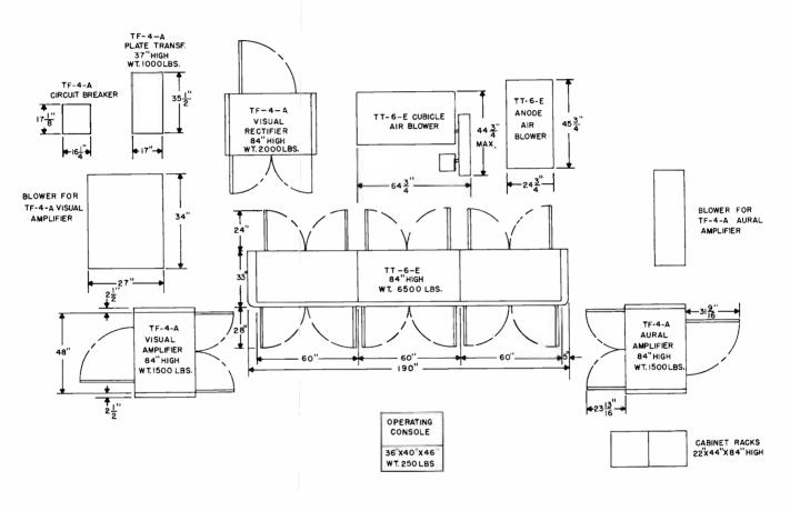
POWER REQUIREMENTS: EXCITER TT-6-E 208/230 VOLTS 3¢,50/60 CYCLES,20KW (BLACK PICTURE) AMPLIFIER TF-4-A 208/230 VOLTS 3¢,50/60 CYCLES,60KW (BLACK PICTURE) PRELIMINARY NOT FOR CONSTRUCTION
