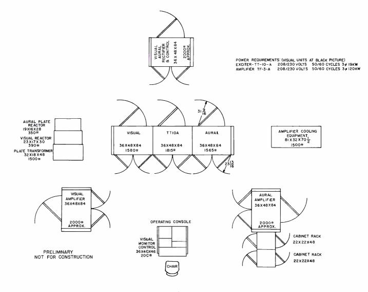
Figure 4 SUGGESTED LAYOUT OF THE TF-3-A LOW CHANNEL 35 KW AMPLIFIER (WITH TYPE TT-10-A 5 KW DRIVER)
