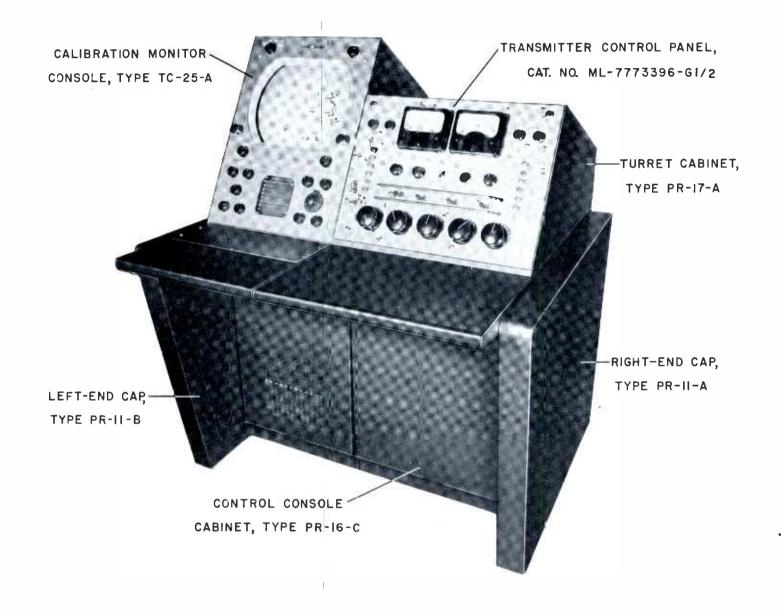
Figure 20 TRANSMITTER CONTROL CONSOLE
