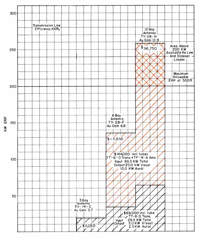
Figure 17 E.R.P. VS. TRANSMITTER-ANTENNA COMBINATIONS FOR VHF CHANNELS 7-13
