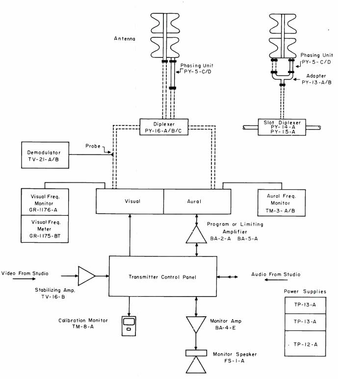
Figure 24 BASIC TRANSMITTING SYSTEM FOR VHF CHANNELS 2-13
