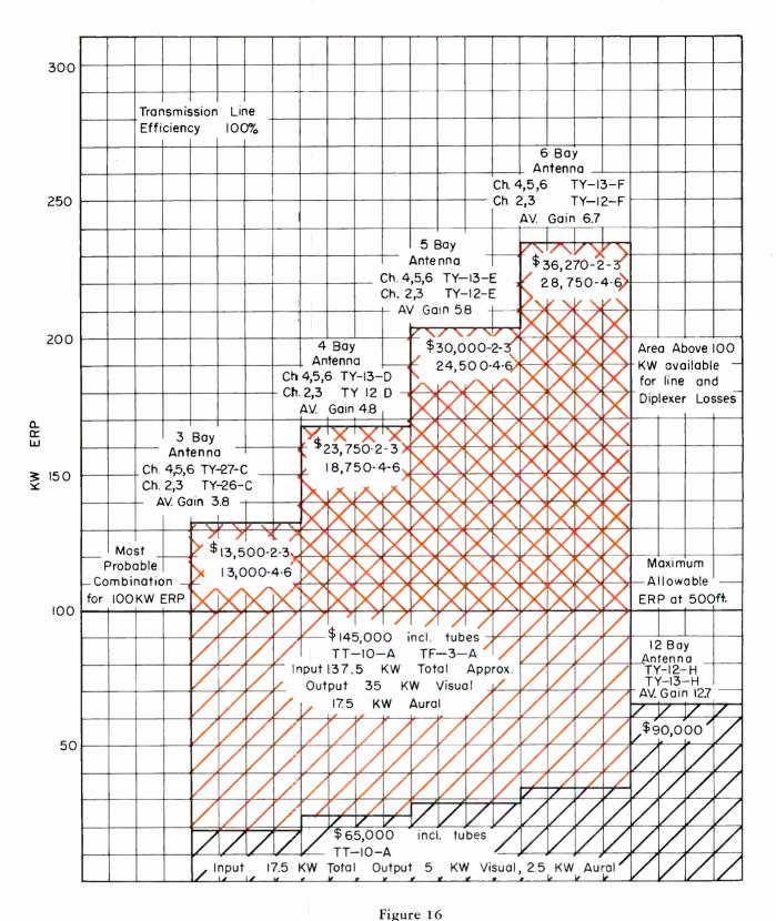
E.R.P. VS. TRANSMITTER-ANTENNA COMBINATIONS FOR VHF CHANNELS 2-6
