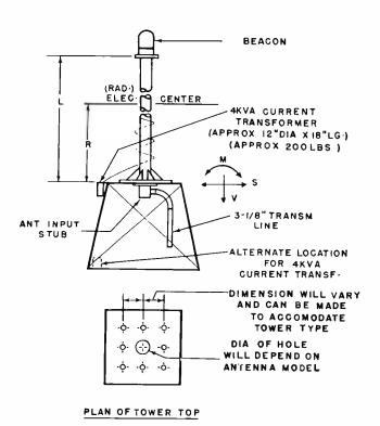
Tower fabricator shall consult G.E. Co. for bolt spacing and clearances required at antenna top.
