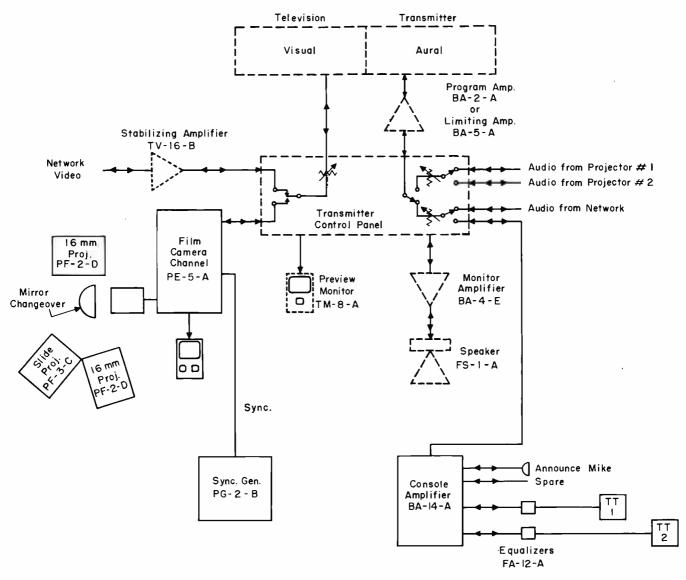
NOTE: The equipment shown in dotted lines is included in the basic transmitter system.
