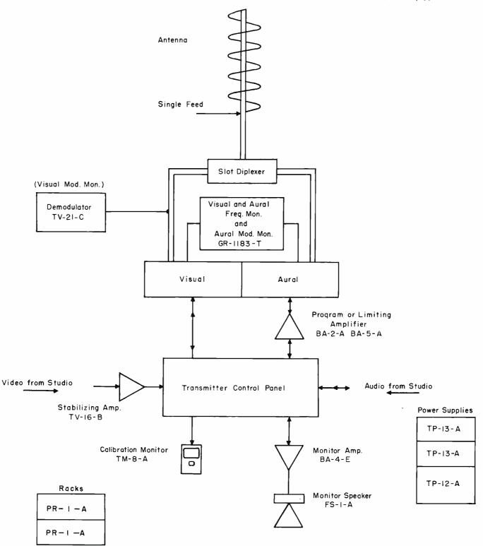
Figure 25 BASIC TRANSMITTING SYSTEM FOR UHF CHANNELS 14-83
