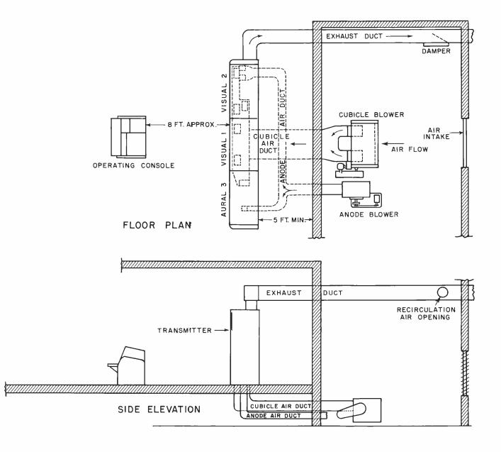
Figure 2 SUGGESTED AIR DUCT LAYOUT FOR THE TT-6-E HIGH CHANNEL TRANSMITTER
