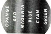
FIGURE 53 The rainbow display pattern produced by the B & K Television Analyst.
