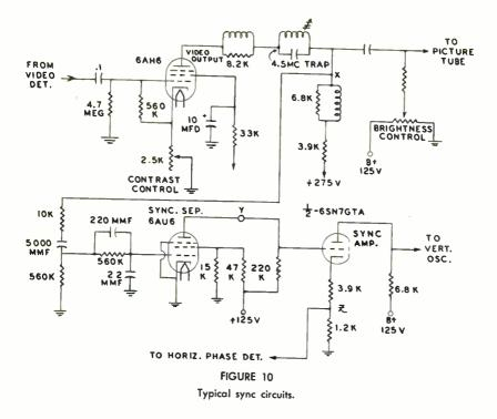
The next step is to check the signal at the output of the sync separator stage. The pattern that appears on the scope screen when the vertical input lead is connected to point Y is shown in Fig. 11. Note that the horizontal sync pulses are clearly visible, while much of the video signal has been removed. This is the proper function of the sync separator stage and we conclude it is operating normally.
