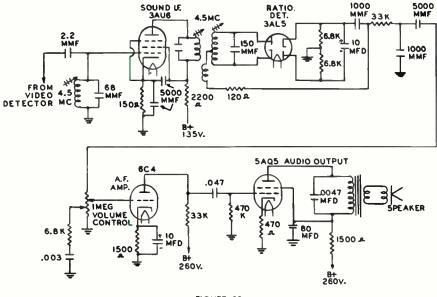
FIGURE 30 Audio system being analyzed.
