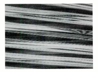
FIGURE 9 Loss of Horizontal Sync.
