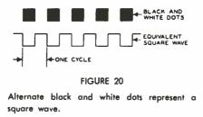
By closely placing the black dots one above the other, we obtain a black line, and similarly, for the white dots, we obtain a white line. Actually, white lines are represented by the spaces between the black lines. It is these alternate black and white lines that form the wedges observed on the test pattern.
