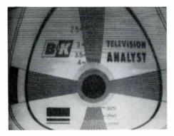
FIGURE 42 Another form of vertical distortion.
