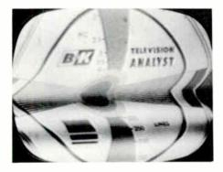
FIGURE 27 The effect on an image of a heater-to-cathode short in one of the signal tubes.
