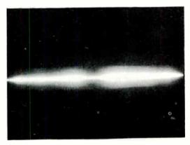
FIGURE 12 Loss of vertical sweep.
