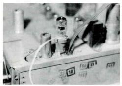
FIGURE 35 A tube adaptor, as shown will permit voltage measurements to be made directly from the topside of the chassis.
