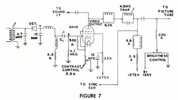
Complete video detector and video amplifier circuit.
