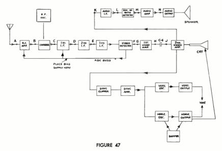
Block diagram of typical TV receiver.
