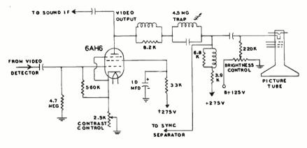
FIGURE 4 Typical video amplifier circuit.
