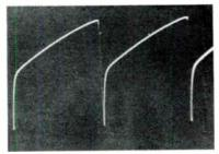
FIGURE 14 The waveform that would normally be present at the control grid of  $V_2$ , Fig. 13, when the circuit is functioning properly.
