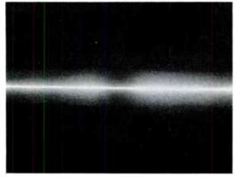
FIGURE 40 An image lacking a vertical deflection.
