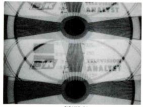
FIGURE 25 Loss of vertical synchronization.
