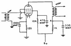
FIGURE 33 Screen by-pass capacitor can be checked with TV analyst.
