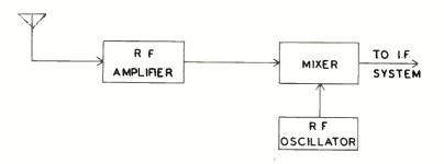
FIGURE 2 Black diagram of typical TV tuner.
