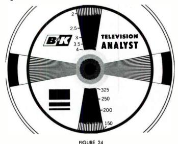
The test pattern shows that the frequency respanse of the receiver under test is only 2 mc.
