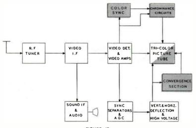
FIGURE 49 Block diagram of a color television receiver.
