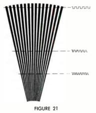
The frequencies represented by the various sections of the wedge increase as the distance from the center of the screen decreases.
