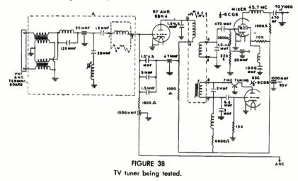
When a defective stage is found, the tube should be checked, if this has not been done already. If the tube is found to be good, voltage at the various tube elements should be measured next. This can be done quite readily by inserting an adapter between the tube and its socket. The lugs extending from each adapter pin then enable the serviceman to measure the voltage at each element.
