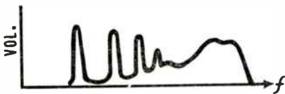
LINE AND BAND SPECTRA. Instantaneous content: here the sound is composed of individual tones superimposed on a broad spectrum band of noise.
