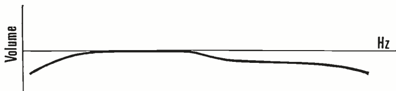
FREQUENCY RESPONSE. 1. Typical response for ribbon microphone. Characteristically this is smooth, but with marginal loss at high frequencies. The actual frequency at which this loss occurs depends on microphone dimensions.
