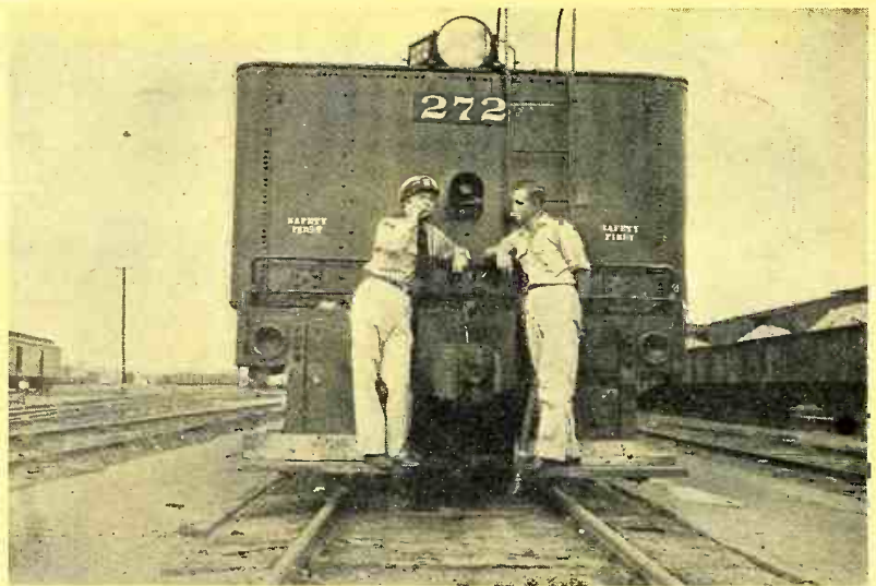
FIG. 6. A. C. NYGREN AND RUBE HOLSTROM OF THE F.E.C. TALK TO THE YARDMASTER FROM THE AUXILIARY SPEAKER AND HANDSET AT THE REAR OF NO. 272
