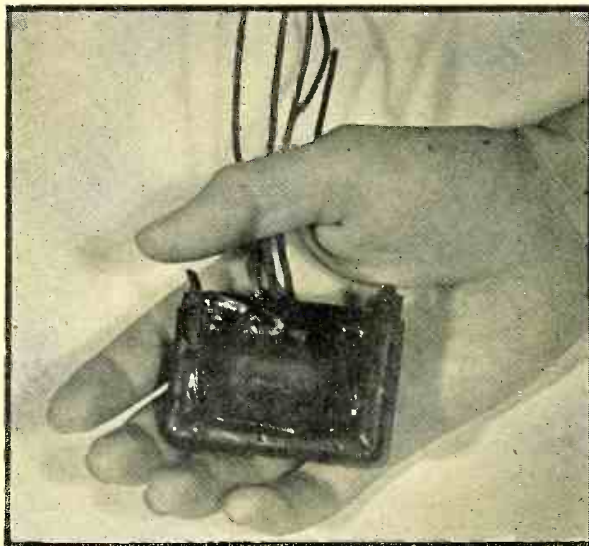
79-CENT OUTPUT TRANSFORMER FROM RADIO SET, ¾ LB.
