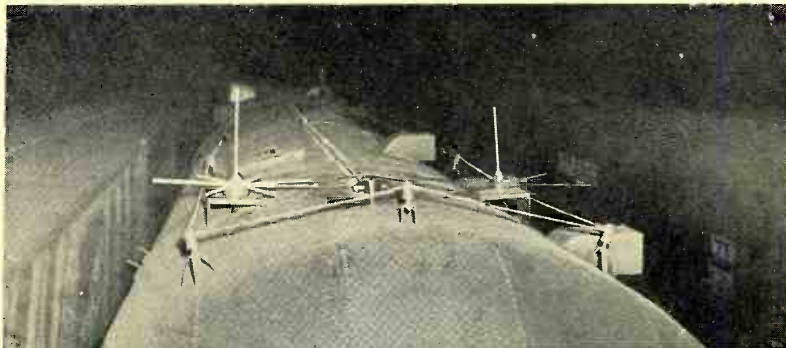
FIG. 10. TWO 160-MC. ANTENNAS MOUNTED ON ROCK ISLAND LABORATORY CAR
