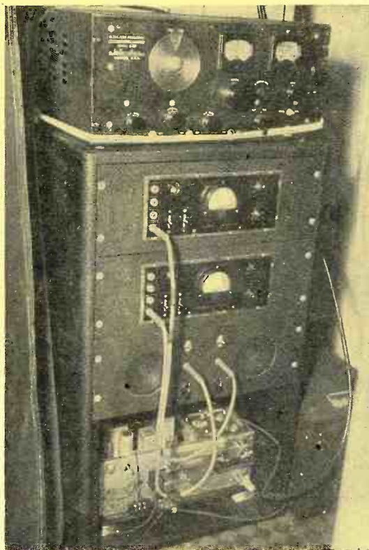
FIG. 7. VISUAL AND AUDIO EQUIPMENT USED ON THE ROCK ISLAND TEST CAR FOR MEASURING RADIO RECEPTION
