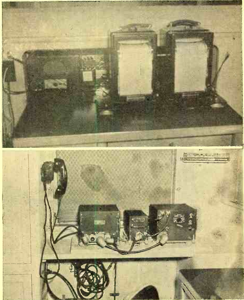
FIG. 8. ESTERLINE-ANGUS RECORDERS REGISTER RECEPTION CONTINUOUSLY. FIG. 9. COMMUNICATIONS COMPANY EQUIPMENT INSTALLED ON THE ROCK ISLAND
