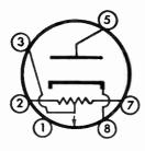
Fig. 9.21 Base connections of the 35Z5 rectifier tube. Prongs 2 and 7 are the heater terminals, prong 3 is the pilot-light tap.
