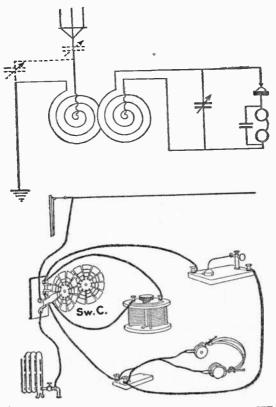
FIG. 44.—HOOK-UP FOR A CRYSTAL DETECTOR SHT WITH TWO SPIDERWEB COILS.
