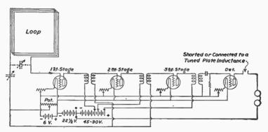
FIG. 81.—COMPLETE HOOK-UP FOR A LOOP AERIAL, THREE STAGES OF RADIO-FREQUENCY AMPLIFICATION AND A DETECTOR.
