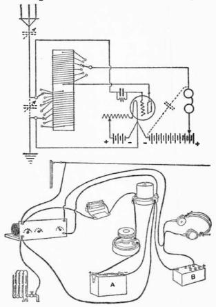
Fig. 63.—Diagram for home construction of a regenerative receiver with a tickler coll.
