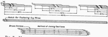
FIG. 7.-METHOD OF CONSTRUCTING A 40-FOOT LAMINATED MAST.
