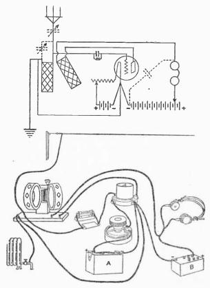
FIG. 64.—Hook-up for regenerative effect with two honeycomb coils.
