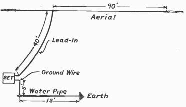
FIG. 4.—METHOD OF CALCULATING THE PHYSICAL LENGTH OF AN ABRIAL CIRCUIT.
