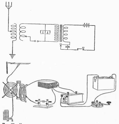
FIG. 89.-HOOK-UP FOR A COMPLETE SPARK COIL TRANSMITTING SET.
