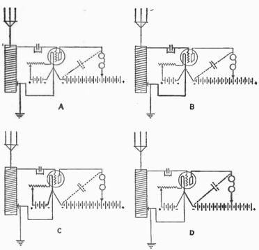
Fig. 49.—Four illustrations of the hook-up shown in Fig. 48. A shows the aerial circuit in heavy lines; B, the secondary of grid circuit in heavy lines; C, the filament circuit in heavy Lines; and D, the plate circuit in heavy lines
