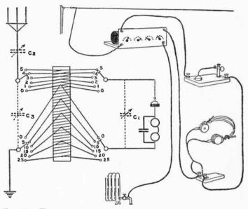
Fig. 33.—Hook-up for a tapped coil with two units switches and two multiple turns switches.
