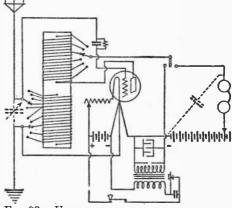
Fig. 93.—Use of a spark coll to increase the power of the receiver type of transmitter.
