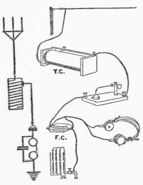
FIG. 16.—THE SIMPLE RECEIVING SET WITH A TUNING COIL AND A FIXED CON-DENSEL ADDED TO THE CIRCUIT.
