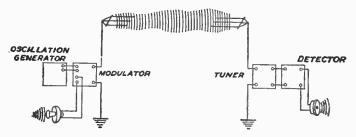
FIG. 53.-ESSENTIAL UNITS OF A RADIO TELEPHONE SYSTEM.
