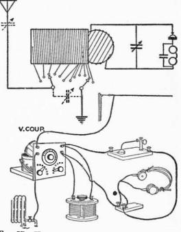
are sending on Fig. 37.—Hook-up for a variocoupler in a crysthe same wave - TAL DETECTOR SET.
