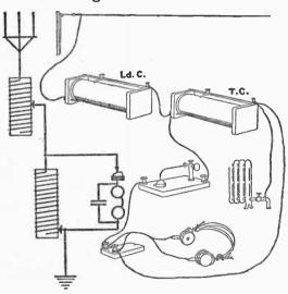
large enough to build up the wave length of the aerial to that of the station from which it is desired to receive, additional wire may be inserted in the aerial circuit by the use of what is known as a loading coil. Its hook-up is shown in Fig.
