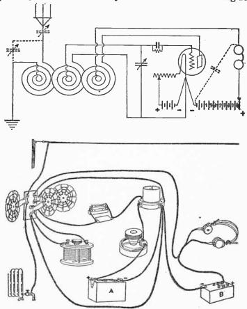
FIG. 66.—HOOK-UP FOR THREE SPIDERWEB COILS IN A REGENERATIVE SET.
