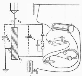
FIG. 31.-HOOK-UP FOR A DOUBLE SLIDE TUNING COIL.
