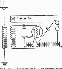
FIG. 56.-HOOK-UP FOR A REGENERATIVE SET USING A LOOSE COUPLER WITH A TICKLEB COIL.
