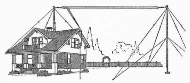
FIG. 14.—A COMPLETE INVERTED L TRANSMITTING AERIAL INSTALLATION, SHOWING MASTS, GUY WIRES AND INSULATORS, FLAT TOP, LEAD-IN, LIGHTNING SWITCH, GROUND WIRE, AND LIGHTNING GROUND.
