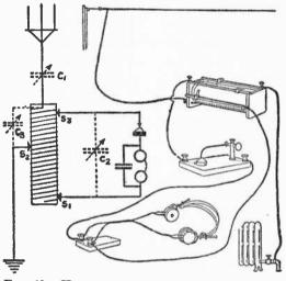
Fig. 40.—Hook-up for a three slide tuning coll in a crystal detector set.
