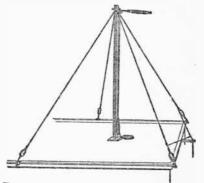
FIG. 6.—METHOD OF INSULATING AND GROUNDING GUY WIRES OF A POLE ERECTED ON THE ROOF OF A BUILDING.
