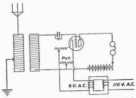
FIG. 54.--HOOK-UP FOR A VACUUM TUBE DETECTOR WITH THE FILAMENT HEATED FROM ALTERNATING HOUSE CURRENT
