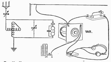
FIG. 46 .--- HOOK-UP FOR A VARIOMETER IN A CRYSTAL DETECTOR SET.
