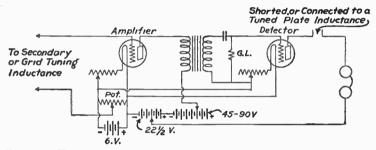
FIG. 80.—HOOK-UP FOR ONE STAGE OF RADIO-FREQUENCY AMPLIFICATION AND A DETECTOR.
