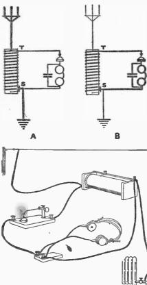
Fig. 21.—Circuits of the crystal detector hook-up. A. Primary in heavy lines. B. Specondary in heavy lines.
