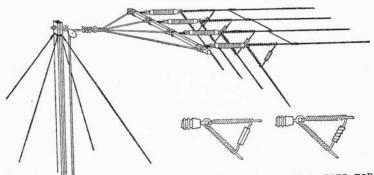
FIG. 9.—AERIAL WITH WOODEN SPREADERS REQUIRING INSULATORS FOR EACH WIRE. SMALL DRAWINGS SHOW APPROVED SLEEVES FOR SPLICING.
