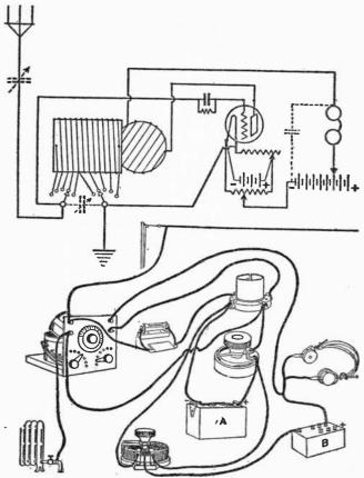
FIG. 62.-HOOK-UP FOR A VARIOCOUPLEE IN A REGENERATIVE SET.
