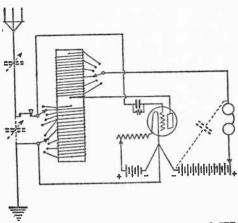
FIG. 92.—THE REGENERATIVE RECEIVING SET HOOKED UP AS A TRANSMITTER.
