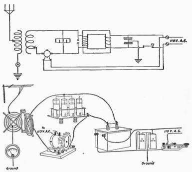
Fig. 90.—Hook-up for a rotary spark gap transmitter operating on 110-volt alternating current.
