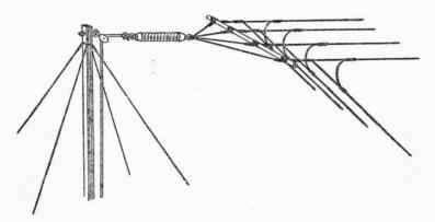
FIG. 8.—ABBIAL WITH METAL SPREADERS REQUIRING ONLY A SINGLE INSULATOR AT EACH END. NOTE METHOD OF CONNECTING THE LEAD-IN TO THE FLAT TOP. NOTE ALSO EASED OFF BENDS TO REDUCE BRUSH DISCHARGF IN TRANSMITTING.
