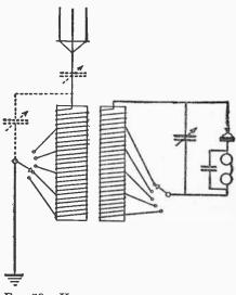
FIG. 38.—HOOK-UP FOR A CRYSTAL DETIRO-TOR SET WITH A TAPPED LOOSE COUPLER.
