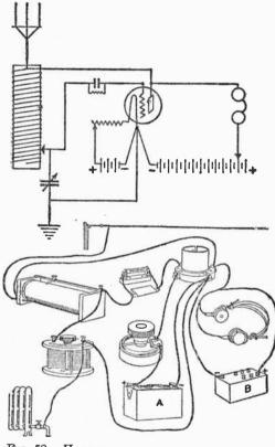
FIG. 58.—HOOK-UP FOR A SINGLE SLIDE TUNING COIL IN A REGENERATIVE SET.
