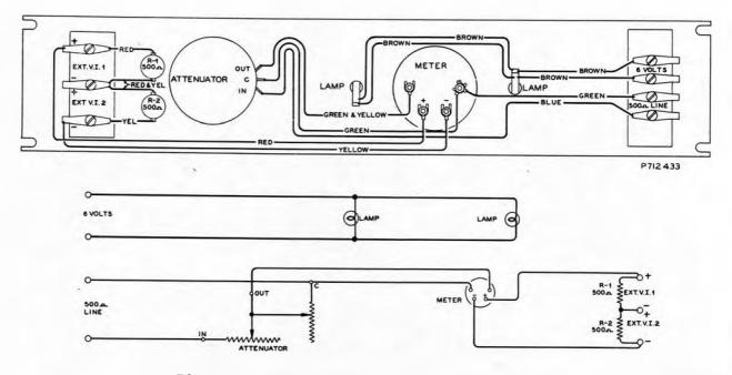
Figure 2 - Schematic and Wiring - MI-3115-A
