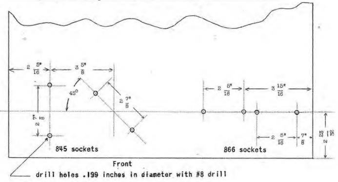
Figure 1 Layout of Mounting Holes for Porcelain Base Sockets in MI-4255-A
