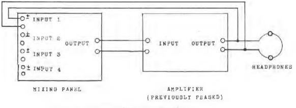
Figure 1 - Connections for Phasing
