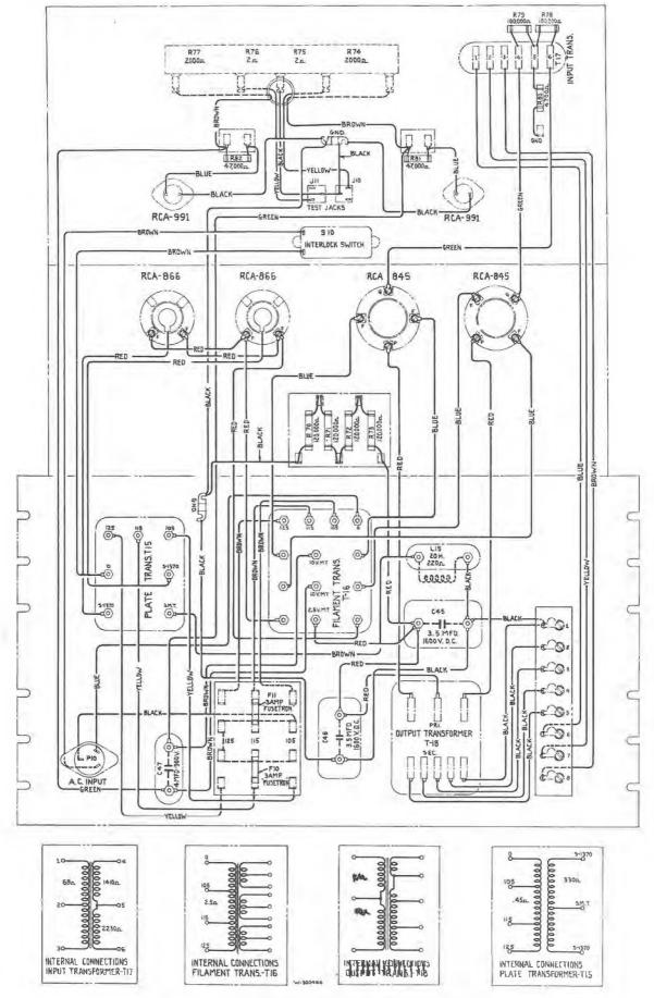
Figure 2 - Wiring Diagram - MI-4255A
