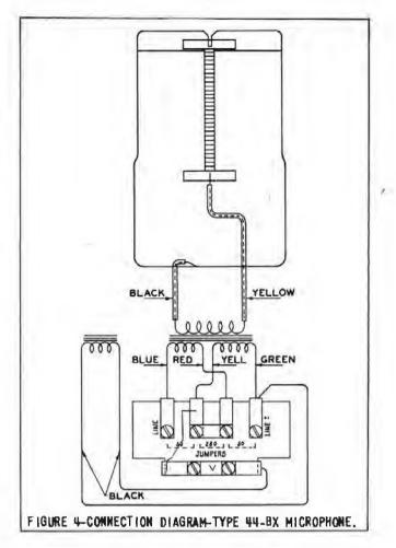
graved the number 50 (i.e., 50 ohms). See Figure 4. If the microphone is to feed a 250 ohm line, place the two small jumpers, one over the other, across the two center terminals (250 ohm). If the microphone is to feed a 50 ohm line, connect one of the jumpers across each pair of terminals marked 50. No change is necessary in microphone cable terminal connections. The cable should pass through the slot in the transformer housing. Solder the ground lead from the cable shield to the cable clamp.
