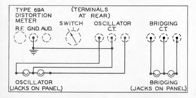
FIGURE 2 - INTERNAL WIRING (Connections K-841774)
