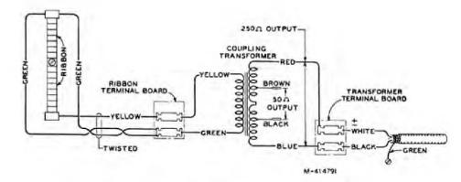
Figure 4—Schematic Wiring Diagram of Microphone
