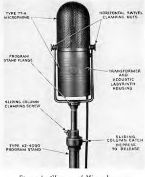
Figure 1—Close-up of Microphone on Program Stand
