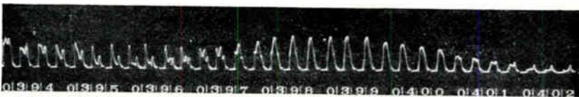
FIG. 6-34.—Section of the pulse-to-pulse record of the echo from a battleship on 9.2 cm. Pulse-recurrence frequency 333 pps, pulse length 1 \mu sec.
