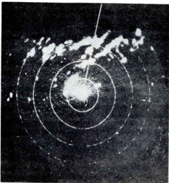
FIG. 7-17.—Localized precipitation preceding the hurricane of Sept. 14–15, 1944, as seen on the PPI of a 3-cm radar system at Provincetown, Mass., at 1015 hours, EST, Sept. 14. The small echo areas are part of larger “band” structures characteristic of this hurricane. Beamwidth 2^\circ , pulse length 1 \mu\text{sec} , 10-mile range marks. The white line points north.
