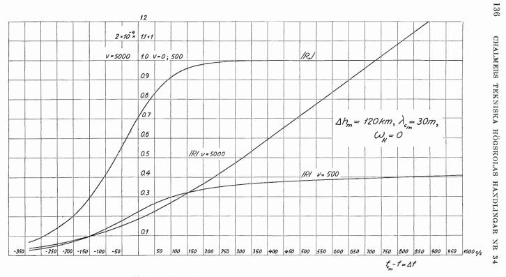
Fig. 30. The Reflection Coefficient of the Parabolic Layer.
