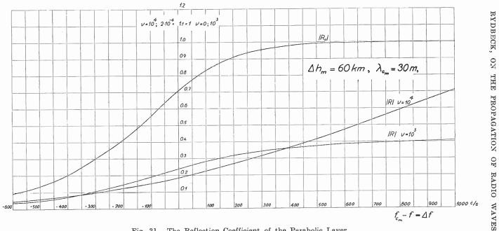
Fig. 31. The Reflection Coefficient of the Parabolic Layer.
