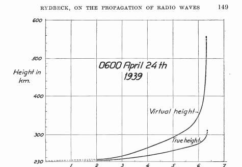
Fig. 43. Experimentally determined virtual and true heights.
