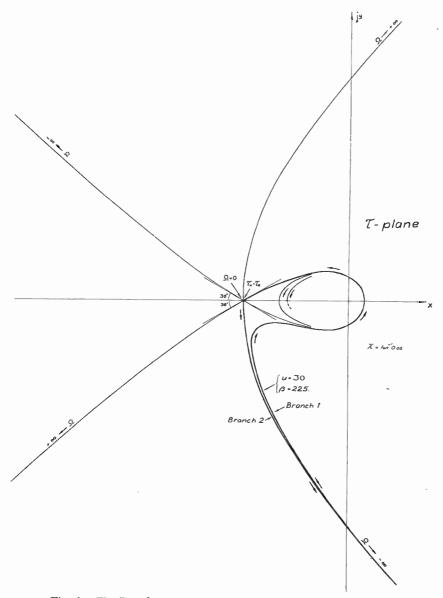
Fig. 9. The Im  $(\Omega_4) = 0$  contours through the stationary point. (Note:  $\tau_A$  means  $\overline{\tau}_A$ ,  $\Omega$  means  $-\Omega_3$ )
