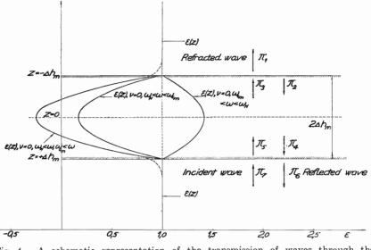
Fig. 4. A schematic representation of the transmission of waves through the inhomogeneous layer.
