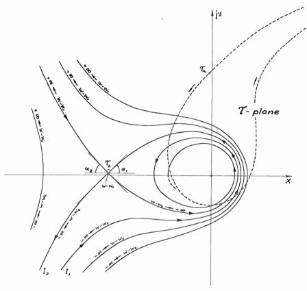
Fig. 8. The Im (W) = const. contours near the origin. [Note:  $W_0 = W(\tau_A)$ ]
