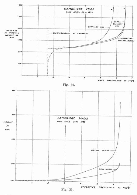
Fig. 30 shows the virtual height curve in the early morning a day later. The height correction is about the same as before. The virtual and true heights plotted against the »effective frequency» are shown
