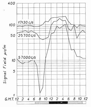
Fig. 27. Diurnal field strength data for transatlantic long wave transmission. Entire path in daylight. Entire path in darkness.
