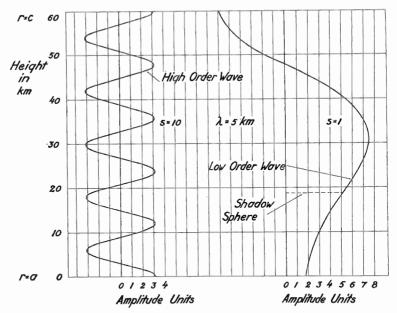
Fig. 26. The low and high order waves in the propagation of long vertically polarized radio waves.
