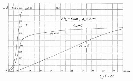
Fig. 33. The Reflection Coefficient of the Parabolic Layer.
