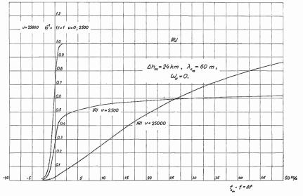
Fig. 32. The Reflection Coefficient of the Parabolic Layer.
