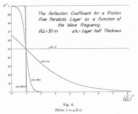
In order to demonstrate the character of relation (29) we reproduce in fig. 6 a plot of  $|R|^2$  for  $\omega_H = 0$ , as a function of  $x^2 = \frac{\omega^2}{\omega_{c_m}^2}$ , which has already been shown in earlier communications [3].
