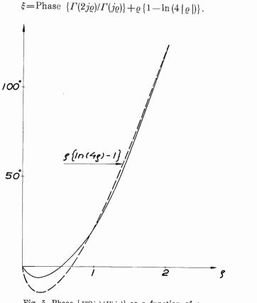
Fig. 5. Phase  $\{\Gamma(2j\varrho)/\Gamma(j\varrho)\}$  as a function of  $\varrho$ .
