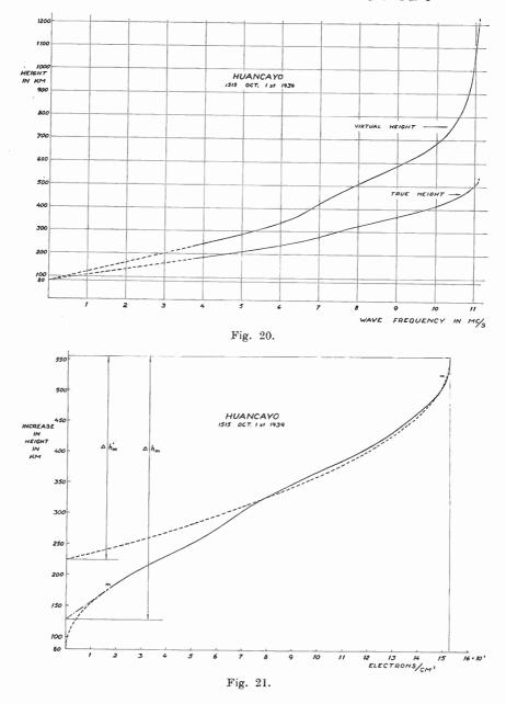
Fig. 20 indicates a very great expansion, the maximum true height being more than 500 km. Consequently the corresponding H value is great as indicated by Fig. 21. The approximate value is 165 km.
