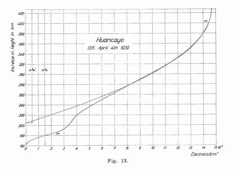
Fig. 13, showing the corresponding electron density distribution, indicates this even more clearly. The parabolic approximation is fairly good over an appreciable frequency range and it yields H about 105 km.
