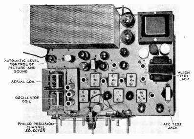
FIG. 8.9C. TOP VIEW OF THE PHILCO RECEIVER CHASSIS (Courtesy of Philco ('orp., Ltd.)
