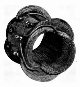
FIG. 3.6B. TYPICAL SADDLE INDUCTOR ASSEMBLY (Courtesy of E.M.I., Ltd.)
