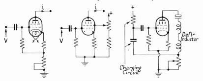
FIG. 4.10C. THREE METHODS OF TIME-BASE AMPLITUDE CONTROL
