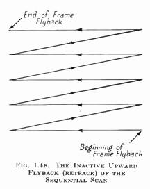
zig-zag path, called a "se figure. When the bottom vertical deflecting force reverts quickly to its original value (the "frame flyback"). The process is then repeated.
