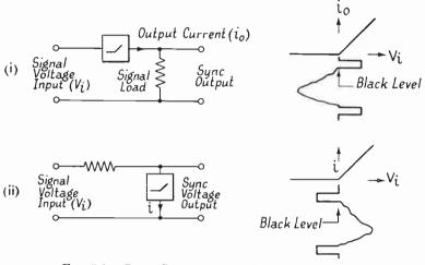
FIG. 5.4B. BASIC SYNCHRONIZING SIGNAL SEPARATORS
