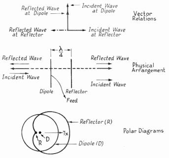
FIG. 9.3A. THE PRINCIPLE OF THE REFLECTOR
