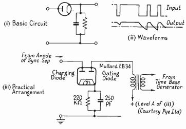
FIG. 5.6D. THE "DOUBLE" TIME-CONSTANT INTEGRATOR FRAMING-SIGNAL SEPARATOR
