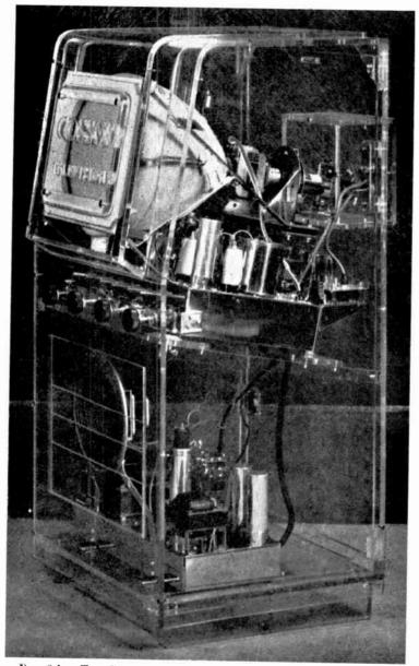
FIG. 8.1B. THE COSSOR MODEL 902 CONSOLE RECEIVER IN PLASTIC EXHIBITION CABINET (Courtesy of A. C. Cossor, Ltd.)
