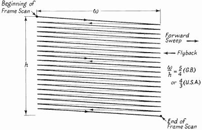
FIG. 1.4A. THE ACTIVE DOWNWARD PORTION OF A SIMPLE SEQUENTIAL OR PROGRESSIVE SCAN
