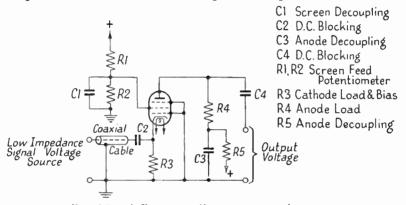
FIG. 2.8A. A PRACTICAL GROUNDED-GRID AMPLIFIER The component values employed will depend on the frequency and bandwidth of the signal.
