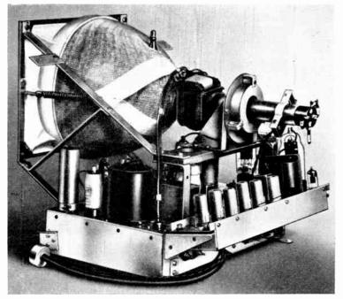
FIG. 3.2E. THE COSSOR MODEL 902 RECEIVER This illustration shows clearly the normal method of mounting a directlyviewed tube. Special features are the anti-implosion net and magnetic ion trap (near the tube base). (See also Fig. 8.1B.) (Courtesy of A. C. Cosmar, Ltd.)
