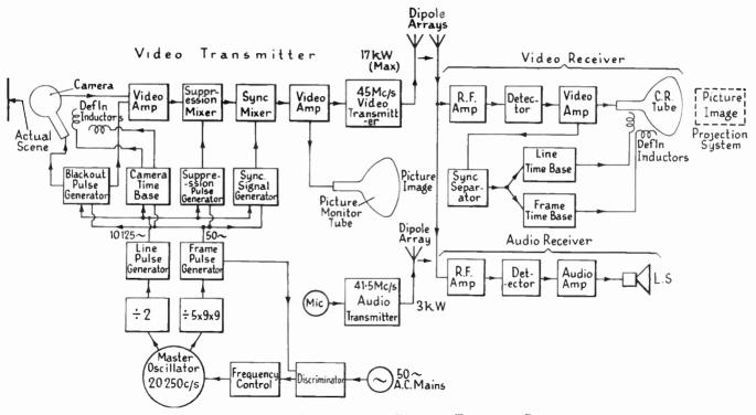
FIG. 1.10A. BLOCK SCHEMATIC OF A COMPLETE TELEVISION SYSTEM
