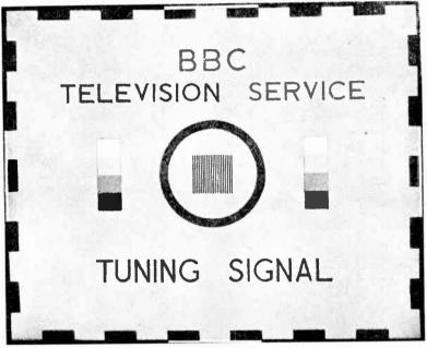
FIG. 10.3A. THE B.B.C. TEST CARD (Courdesy of "Electronic Engineering")
