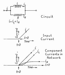
FIG. 2.3F. Application of a Linearly-rising Current to a Parallel LR Circuit
