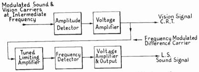
FIG. 7.4E. CARRIER-DIFFERENCE RECEPTION OF F.M. SOUND SIGNAL
