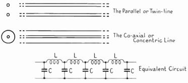
Fig. 9.4a. The Two Basic Forms of Feeder or Transmission Line and Their Equivalent Circuit
