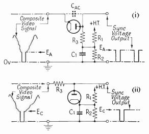
FIG. 5.4c. PRACTICAL DIODE SEPARATORS
