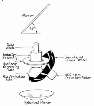
FIG. 11.3B. THE C.B.S. COLOUR PROJECTION SYSTEM
