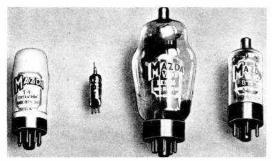
FIG. 2.6A. A GROUP OF VALVES DESIGNED FOR TELEVISION RECEPTION From left to right they are: a T41—thyratron: a D41—detector diode; a Pen 46—line time-base amplifier: a U22—high-voltage rectifier. (Courtesy of Edison Suran Electric Co., Ltd.)
