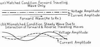
FIG. 9.4B. VOLTAGE AND CURRENT AMPLITUDE DISTRIBUTIONS ON A FEEDER FOR THE MATCHED AND SERIOUSLY MISMATCHED CONDITIONS
