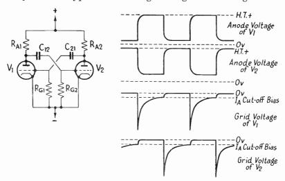
Fig. 4.7a. The Anode-coupled Multivibrator: Basic Circuit and Waveforms
