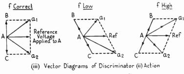
FIG. 7.4B. THE FREQUENCY-MODULATION DETECTOR OR DISCRIMINATOR
