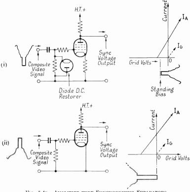
FIG. 5.4D. AMPLIFIER-TYPE SYNCHRONIZING SEPARATORS
