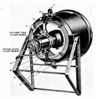
FIG. 3.8G. A PROJECTION TUBE MOUNTING (Courtesy of Phileo Corp., Ltd.)
