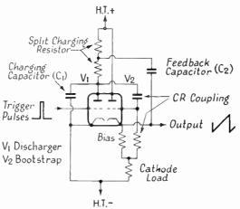
FIG. 4.11F. THE BOOTSTRAP LINEARIZED SAWTOOTH GENERATOR
