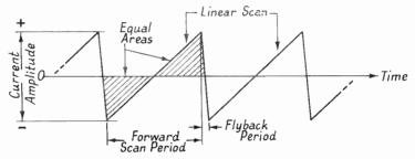
FIG. 4.1A. REQUIRED WAVEFORM OF THE SCANNING INDUCTOR CURRENT
