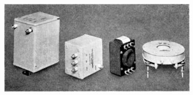
FIG. 3.6G. A GROUP OF PICTURE-TUBE AUXILIARY COMPONENTS From left to right they are: an E.H.T. transformer; a line output transformer; a scanning-inductor assembly; and a focusing-inductor assembly. (Courtesy of Haynes Radio, Ltd.)
