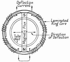
FIG. 3.6D. CROSS-SECTION OF A TOROIDAL DEFLECTION INDUCTOR
