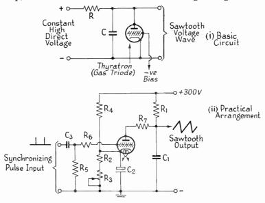
FIG. 4.4A. THE THYRATRON TIME-BASE (SAWTOOTH VOLTAGE WAVE) GENERATOR
