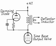
FIG. 4.10E. USE OF A DIODE FOR DAMPING THE LINE OUTPUT CIRCUIT
