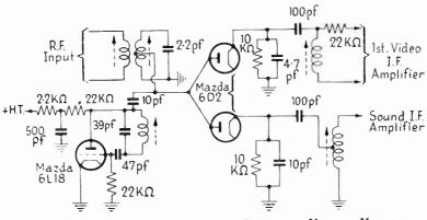
FIG. 6.9B. THE FREQUENCY-CHANGER CIRCUIT OF MURPHY MODELS V114, 116 (Conrtesy of Murphy Radio, Ltd.)
