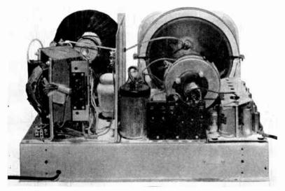
FIG. 8.3B. THE CHASSIS OF THE PVE MODEL B16T RECEIVER (Courtesy of Pye, Ltd.)
