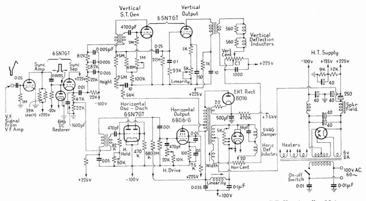
FIG. 8.7A. COMPLETE CIRCUIT DIAGRAM OF THE R.C.A. 7 IN. RECEIVER (1946), OMITTING THE R.F. UNIT (SEE FIG. 6.9D) (Courtesy of R.C.A., Ltd.)
