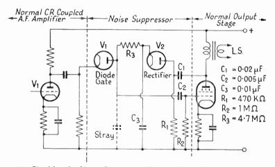
(ii) The Murphy Noise Suppressor Circuit. See also Fig 8.5c (V.10) (Courtesy Murphy Radio Itd
