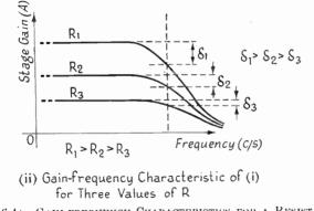
FIG. 6.4A. GAIN-FREQUENCY CHARACTERISTICS FOR A RESISTANCE-LOADED AMPLIFIER
