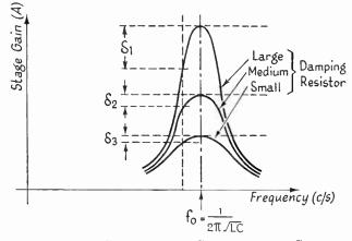
FIG. 6.4B. FORM OF CHARACTERISTIC GAIN-FREQUENCY CURVE FOR A TUNED-ANODE ('IRCUIT (C, L and R in Parallel) Amplifier for Three Values of R
