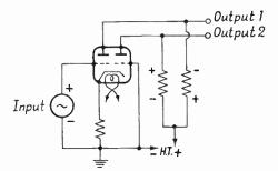
FIG. 2.12A. THE CATHODE-COUPLED DOUBLE-TRIODE AMPLIFIER
