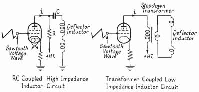
FIG. 4.10B. BASIC DEFLECTOR INDUCTOR COUPLING CIRCUITS
