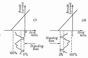
Fig. 6.4F. Alternative Operating Conditions for the Video Amplifier
