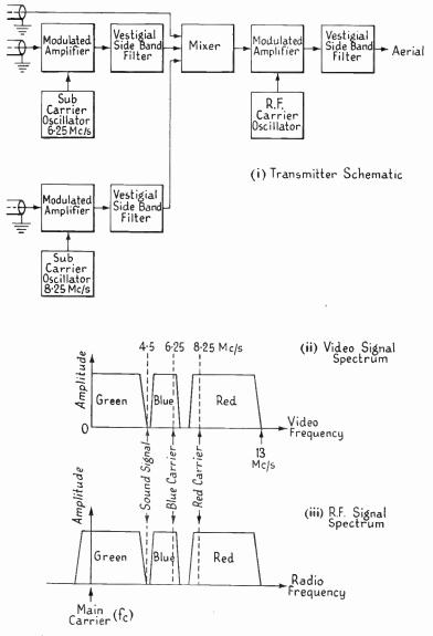
FIG. 11.4A. THE R.C.A. SIMULTANEOUS COLOUR TRANSMITTER (Courtesy of the I.R.E.)
