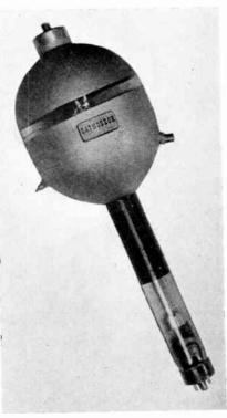
FIG. 10.3C. A STILL PICTURE GENERATOR TUBE (Courtesy of Cathodeon, Ltd.)
