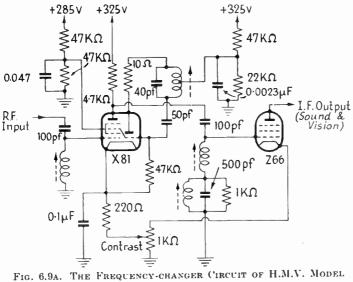
IG. 6.9A. THE FREQUENCY-CHANGER CIRCUIT OF H.M.V. MODEL 1804 RECEIVER
