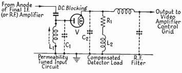
FIG. 6.6A. TYPICAL DETECTOR CIRCUIT
