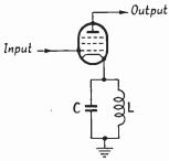
FIG. 6.8C. CATHODE-FEED-BACK REJECTOR
