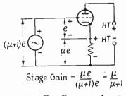
FIG. 2.9A. THE RELATIVE AMPLI-TUDES AND POLARITIES OF THE SIGNAL VOLTAGES IN A CATHODE FOLLOWER normal amplifier (i.e. one without a cathode load), because the increased voltage drop across the cathode load, in making the cathode follow in the same direction (positive) as the grid, restricts the actual change in grid-to-cathode p.d., which, of course, is the controlling factor in the amount of anode current change. The signs placed on
