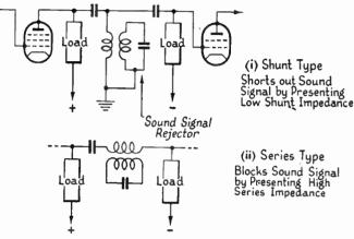
FIG. 6.8A. Two Methods of Rejecting the Sound Signal from the Vision Channel
