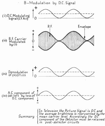
FIG. L.9B. MODULATION AND DEMODULATION-D.C. MODULATION SIGNAL
