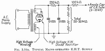
FIG. 3.10A. TYPICAL MAINS-OPERATED E.H.I. SOFFET
