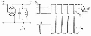
FIG. 5.6F. RESONANT FRAMING SIGNAL SHAPER
