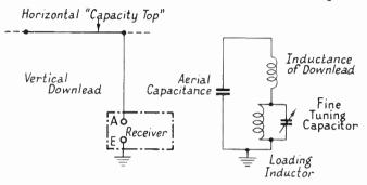
FIG. 9.1a. THE NORMAL BROADCAST (MARCONI) AERIAL AND THE Equivalent Circuit
