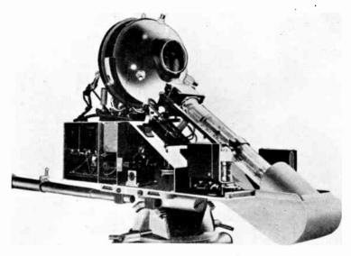
FIG. 1.3B. THE EMITRON ('AMERA WITH COVER REMOVED (Courtesy E.M.I., Ltd.)
