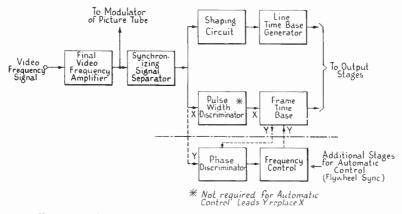
FIG. 5.3A. GENERAL SCHEMATIC OF THE SYNCHRONIZING SYSTEM
