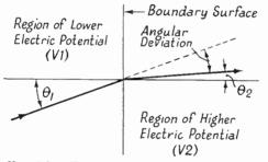
FIG. 3.1B. THE REFRACTION OF ELECTRONS
