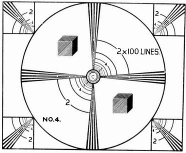
FIG. 10.3E. A TYPICAL RESOLUTION PATTERN (Contess of Cathodeon, Ltd.)
