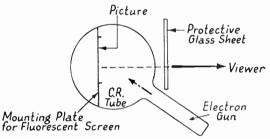
(ii) The Baird method of viewing the Fluorescent Screen from the Gun side. The oblique incidence of the Scanning Beam requires"keystone correction" of the raster, i.e. modulation of line amplitude at frame frequency, to produce rectangular shape
