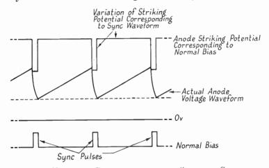
FIG. 4.9A. METHOD OF PULSE-TRIGGERING THE SAWTOOTH GENERATOR The positive-going grid pulse causes the critical anode potential to fall sufficiently to initiate the discharge (flyback) when the anode voltage has risen to the required level.
