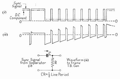
FIG. 5.6E. PARTIAL DIFFERENTIATION OF THE FRAMING SIGNAL
