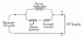
Control Circuit for Low Resistance Type Focus Inductor
