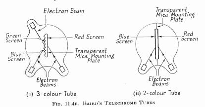
mica sheet, each side of which was scanned obliquely by separate beams arranged one on either side of the double screen. The mica mounting plate in the three-colour tube is corrugated to allow two distinct screens to be carried and a third gun is added, as shown in the diagram, Fig. 11.4F. The composite screen can be viewed from one side only because from the other side the image will appear reversed.
