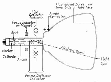
FIG. 1.6A. THE RECEIVER CATHODE-RAY PICTURE TUBE (Note that all inductors are outside the tube—their arrangement is shown schematically.)
