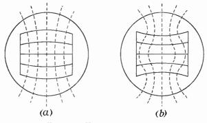
FIG. 3.6F. NON-UNIFORM FIELDS Type (a) produces a barrel and type (b) a pin-cushion-shaped raster.
