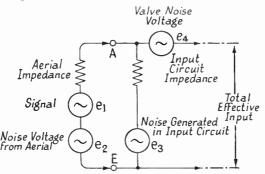
FIG. 6.10A. EFFECTIVE ARRANGEMENT OF THE THREE PRINCIPAL SOURCES OF NOISE VOLTAGE IN THE FIRST STAGE OF THE RECEIVER
