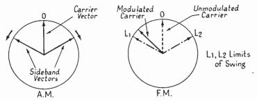
FIG. 7.4A. VECTORIAL COMPARISON OF AMPLITUDE AND FREQUENCY MODULATIONS
