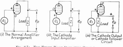
FIG. 2.7A. THE THREE BASIC OPERATING CIRCUITS OF AN AMPLIFIER VALVE
