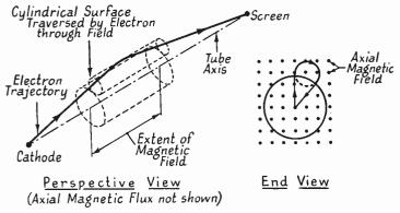
FIG. 3.4D. FOCUSING ACTION IN A SHORT MAGNETIC FIELD
