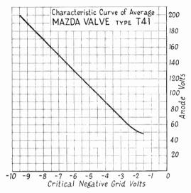
FIG. 4.3B. A TYPICAL THYRATRON GRID CONTROL (HARACTERISTIC (Courtesy of Edison Swan Electric Co., Ltd.)
