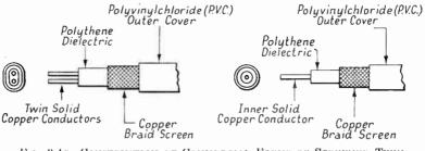
FIG, 9.4C. CONSTRUCTION OF COMMERCIAL FORMS OF SCREENED TWIN AND COAXIAL CABLE
