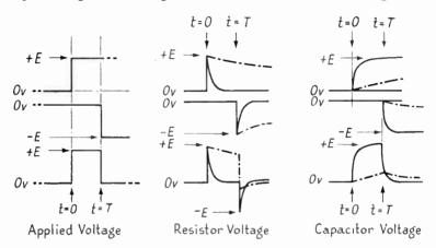
Fig. 2.4a. The Response of a Series CR to a Square Voltage Pulse, obtained by the Method of Superposition, for both Long (chain line) and Short (full line) Time Constants
