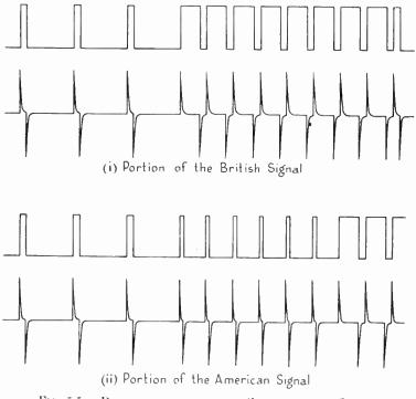
FIG. 5.5A. DIFFERENTIATION OF THE SYNCHRONIZING SIGNAL
