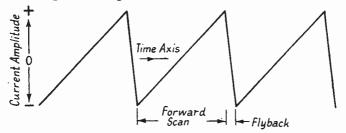
FIG. 1.6B. WAVEFORM OF THE SCANNING-INDUCTOR CURRENTS USED FOR BEAM DEFLECTION IN THE TRANSMITTER CAMERA AND THE RECEIVER CATHODE-RAY TUBE
