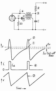
Fig. 4.6a. The Blocking-oscillator Type of Sawtooth Generator and its Characteristic Waveforms
