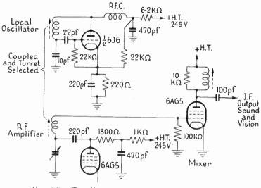
FIG. 6.9C. THE FREQUENCY-CHANGER ('IRCUIT OF THE PHILCO MODEL 48–1000 (Courtesy of the Phileo Corporation, Ltd.)
