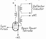
FIG. 4.12B. USE OF A TETRODE AS A SAWTOOTH CURRENT OSCILLATOR (After Sziklai, Reference 18.)
