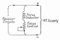
Control Circuit for High Resistance Type Focus Inductor
