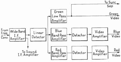
FIG. 11.4B. SCHEMATIC OF RECEIVER FOR SIGNAL OF SUB-CARRIER TYPE (Courtesy of the I.R.E.)
