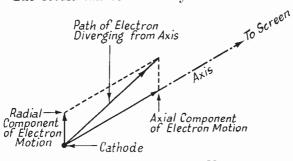
FIG. 3.4A. COMPONENTS OF ELECTRON MOTION IN THE CATHODE-RAY TUBE
