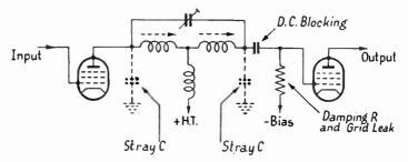
FIG. 6.7D. BRIDGED-T TYPE COUPLING NETWORK
