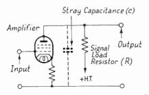
(i) Skeleton Circuit of Resistance Loaded Amplifier
