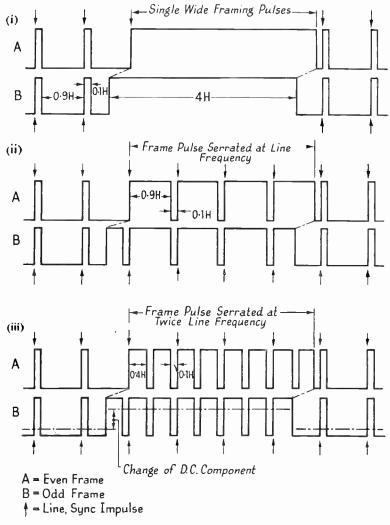
FIG. 5.1A. SYNTHESIS OF THE BRITISH SYNCHRONIZING SIGNAL
