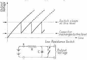
FIG. 4.2B. THE BASIC SAWTOOTH VOLTAGE-WAVE GENERATOR
