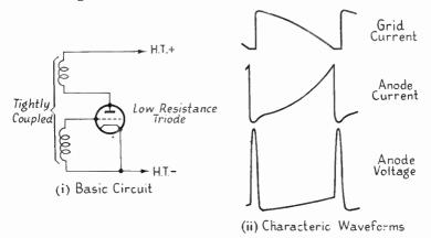
FIG. 4.12A. TRIODE SAWTOOTH CURRENT OSCILLATOR
