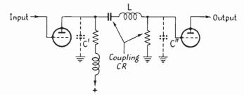
FIG. 6.4D. AN IMPROVED COMPENSATED COUPLING NETWORK An additional L separates the stray capacitance into two portions, C' and C".
