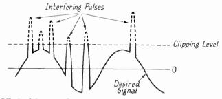
(i) Effect of Clipping Pulsating Interference at Fixed Level
