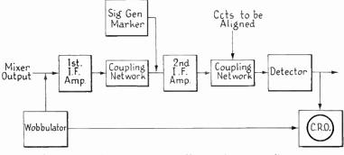
Fig. 10.2b. A Stage in the "Visual Alignment" of a Superhet Receiver
