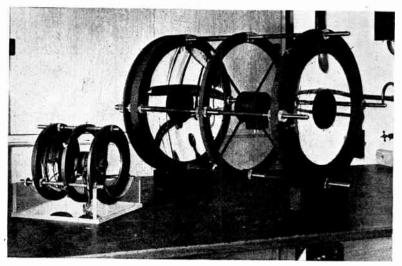
FIG. 3.8D. PROJECTION ASSEMBLIES FOR HOME RECEIVERS (LEFT) AND CINEMA EQUIPMENT (RIGHT) (Courtesy Dr. D. Starkie, "Endeavour," and I.C.I., Ltd.)
