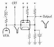
FIG. 5.4F. CATHODE-COUPLED, DOUBLE-TRIODE, NON-INVERTING SYNCHRONIZING AMPLIFIER
