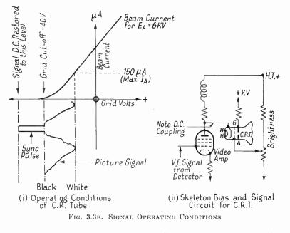
—the maximum beam current for this tube is specified by the manufacturer as 150  $\mu$ A.<sup>(3)</sup>
