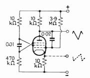
(ii) Practical arrangement for a Frame Base Generator of a Transitron-Miller combination (Courtesy Wireless World")
