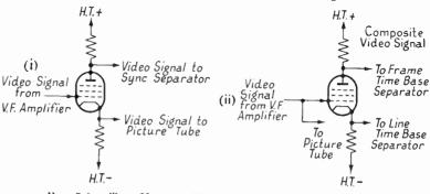
FIG. 5.4E. Two Uses of Cathode Coupling in the Video Output Stage
