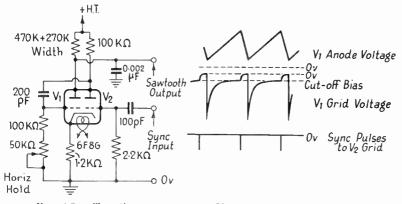
Fig. 4.7b. The Cathode-Coupled Multivibrator; a Practical Line Time-base Circuit (15:75 KC/8)
