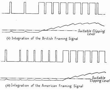
FIG. 5.6A. INTEGRATION OF FRAMING SIGNALS
