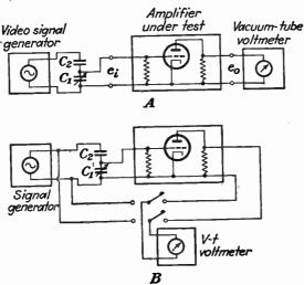
Fig. 141.—Methods of measuring amplifier gain: A, when the video signal generator is calibrated; B, substitution method for uncalibrated signal source.
