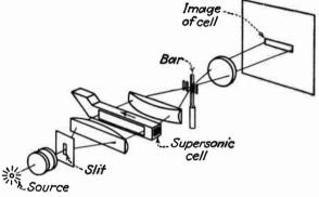
Fig. 310.—Basic light modulation method of the Scophony system of projection television. Light storage is employed to obtain an increase in optical efficiency of over 100 times.
