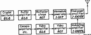
Ftg. 268.—Tube line-up of a typical 50-watt picture transmitter, station W2XVT, Passaic, N. J.
