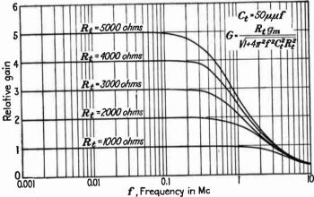
Fig. 121.—Effect on high-frequency response (uncompensated amplifier) of increasing the shunt resistance R<sub>i</sub>. While higher gain may be obtained thereby at low frequencies, the presence of the shunt capacitance places an upper limit on the gain at high frequencies.
