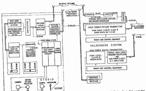
Fig. 272A.—Studio, relay, and main transmitting equipment of station W2XB, Albany, N. Y. (studio in Schenectady). All picture transmissions are handled by carrier after the initial modulator (center, left).
