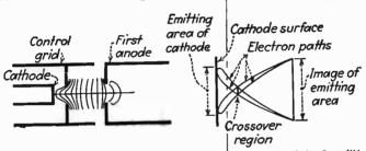
Fig. 62.—Equipotential contours and electron trajectories of the first ("immersion") electron lens of the gun shown in Fig. 61. Left, the lens system and the electric field lines, across which the electrons move. Right, paths taken by electrons as they leave the cathode surface. The crossover region is focused on the scanned surface by means of the second electron lens.
