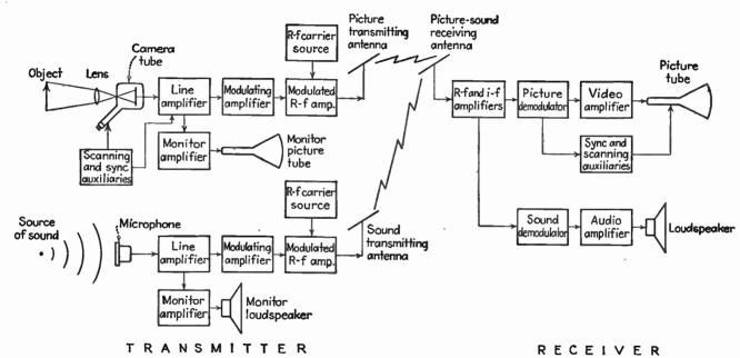
Fig. 7.—Elements of a typical television system.
