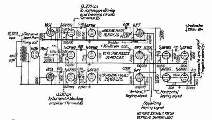
Fig. 254.—Horizontal shaping unit of the sync signal generator. This unit accepts 13,230-c.p.s. timing pulses from the timing unit (Fig. 251), and 60-c.p.s. keying signals from the vertical shaping unit (Fig. 255), and derives from them the composite sync signal with horizontal, equalizing, and serrated-vertical pulses. It produces also 13,230-c.p.s. blanking signals for the iconoscope and picture tube.
