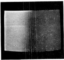
Fig. 292.—Horizontal scanning amplitude test at 13,230 c.p.s., obtained by method shown in Fig. 290.
