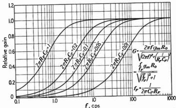
Fig. 132A.—Low frequency gain-frequency response curves of amplifier compensated with  $R_FC_F$  filter. The higher the RC product, the better the gain at low frequencies.
