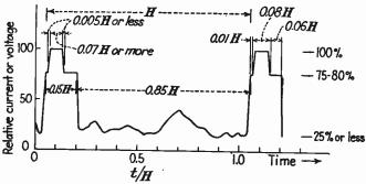
Fig. 99.—Dimensions of the blanking and synchronising signals (R.M.A. Standard) in terms of the line-scanning interval H (= 1/13,230th sec.).
