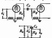
Fig. 122.—Uncompensated amplifier with equivalent low-frequency circuit.
