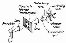
Fig. 47.—A simple method of electronic scanning, employing a cathode-ray tube as the light source. The lack of moving parts is an advantage but the available light is limited and the scanned area must be small.
