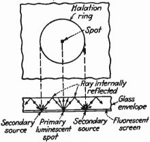
Frg. 206.—Halation due to total internal reflection in the glass face of the picture tube.
