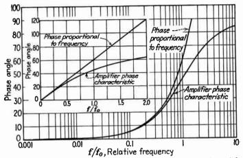
Fig. 120.—Phase-response characteristic of the uncompensated amplifier at high frequencies, compared with the linear (ideal) characteristic. Plotted in linear coordinates in inset, in logarithmic frequency coordinates in the larger diagram.
