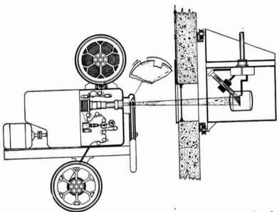
Fig. 259.—Projection system used with storage-type camera tubes for intermittent projection of motion-picture film. (From Lohr, "Television Broadcasting.")
