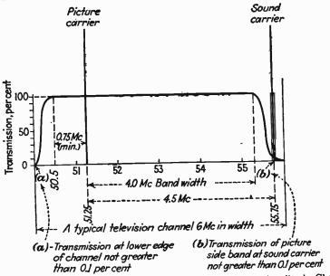
Fig. 813.—Reprint of R.M.A. Standard T-115, Transmitter Amplitude Characteristic, as defined by the R.M.A. Television Committee.
