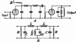
Fig. 184.—Top, capacitively coupled band-pass circuit and simple loaded circuit in cascade for compensating mid-band response. Bottom, combination circuit for developing similar compensation.
