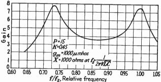
Fig. 181.—Band-pass response curve of circuit shown in Fig. 180A. The gain is directly proportional to the  $g_m$  of the tube and the value of X (after Seeley and Barden).
