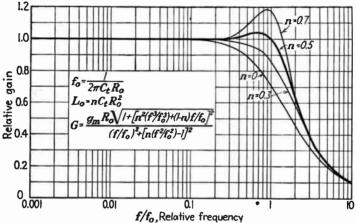
Fig. 126.—Amplitude-frequency response characteristics of the shunt-peaking compensated amplifier, for different values of the compensating inductance  $L_{\rm e}$ . The case for n=0 is the uncompensated case, whereas that for n=0.5 is that usually adopted in practice. Plotted as the magnitude of Eq. (147).
