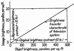
Frg. 33.—Contrast and tonal range. A brightness contrast of 10 to 1 in the object may be reproduced accurately in the image, although the absolute brightness of the image is reduced (cf. Fig. 197, page 336).
