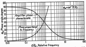
Fig. 124.—Phase-frequency characteristic of the uncompensated amplifier.
