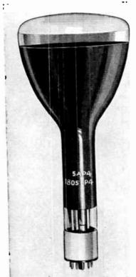
Fig. 199A.—Typical image-reproducing tube (picture tube), the type 5AP4.
