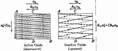
Fig. 20.—The odd-line method of interlaced scanning, now standard in the United States. The upward and downward scanning motions are of equal length (cf. Fig. 19) and the number of lines in each field is a whole number plus one-half (220½ lines for a 441-line pattern).
