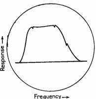
Fig. 298.—Typical oscillogram produced with circuit of Fig. 296. The notches are produced by the absorption in the marker circuits.
