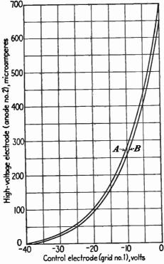
Fig. 204.—Beam current vs. control electrode voltage for electron gun in type 12AP4 picture tube: A, second-anode voltage 7000 volts; B, 6000 volts.
