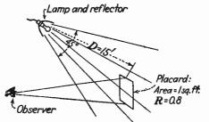
Fig. 30.—Illumination of a reflecting placard. The observed brightness depends on the distance D from the light source, and on the reflecting coefficient R, as well as on the geometry of the reflecting system.
