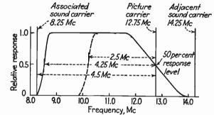
Fig. 178.—Response curve of a television i-f amplifier. The solid line has the maximum width practical within the channel limits, whereas the dotted line shows response limited to 2.5 Mc. to allow greater gain per stage and better signal-to-mask ratio, at the expense of picture detail.
