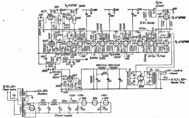
Fig. 251.—Complete circuit diagram of the timing unit (cf. Figs. 248, 249, and 250).
