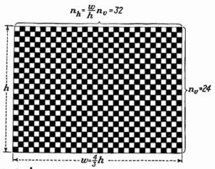
Fig. 14.—Relationship between vertical and horizontal resolution when picture-element spacing is equal in the two dimensions. The total number of picture elements is then  $\frac{4}{3} \times n_v^2$ , where  $n_r$  is the number in the vertical dimension and  $\frac{4}{3}$  is the ratio of the picture's width to its height.
