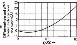
Fig. 77.—Difference between charge-time curve and linear slope (= 0.85). A nonlinearity of  $\pm 1$  per cent can be achieved if the charging time is restricted to 0.4RC or less, but the nonlinearity increases to  $\pm 5$  per cent if the charge is allowed to continue for t=0.7RC seconds.
