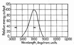
Fro. 39.—Spectral distribution of a typical "nonstandard" light source, for which the photoelectric response is to be computed.
