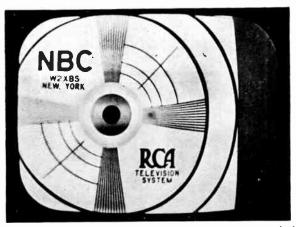
Fig. 238A.—Incorrect positioning due to excessive d-c component in horisontal scanning system.
