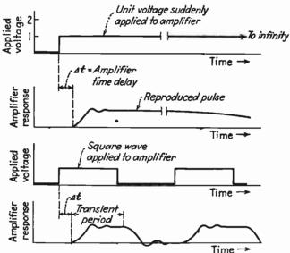
Fig. 138.—Amplifier response to a Heaviside unit voltage (above) and squarewave approximation (below) suggested by Bedford and Fredenhall for analysing transient response of video amplifiers.
