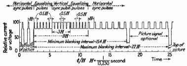
Fig. 100A.—The R.M.A. Standard Video Signal during the vertical blanking (field retrace) period, representing the beginning of the first field.
