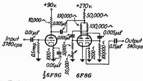
Fig. 249.—Typical multivibrator stage in the timing unit, used to obtain a division of 7 times. The first tube is the isolation amplifier, the second (double triode) the multivibrator proper.
