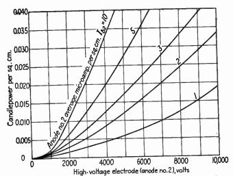
Fig. 2024.—Relationship of output brightness to accelerating voltage for various values of beam current (white-light phosphor, type P4).
