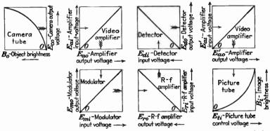
Fig. 195.--Transfer characteristics of the television system, so arranged that the output of one device coincides with the input of the following device. By following the arrows, the brightness of the object may be traced through the subsidiary signal voltages to the brightness of the received image. The relationship between these two brightnesses, the over-all brightness-transfer characteristic, is determined by the curvature of the subsidiary characteristics.
