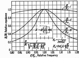
Fro. 166.—General impedance-frequency curves of the loaded tuned circuit. In r-f practice, the useful range usually extends from 0.95 to 1.05 fr.
