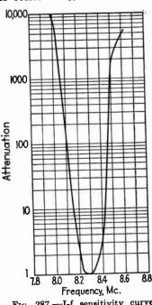
Fig. 287.—I-f sensitivity curve of sound channel of receiver shown in Fig. 284.
