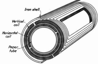
Fig. 289.—Internal construction of a typical magnetic deflection yoke. The axes of the two coils are at right angles to each other and to the axis of the picture tube.
