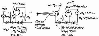
Fig. 42A.—Basic phototube amplifier circuit. The photoelectric current  $\Delta i_{pi}$  passes through the grid resistor  $R_0$ , producing a voltage  $\Delta e_g$  which is amplified to the value  $\Delta e_L$ .
