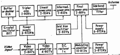
Fig. 269.—Tube line-up of a typical 1000-watt picture transmitter manufactured by the RCA Manufacturing Co.
