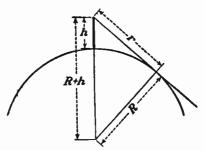
Fig. 149.—Geometrical relationship of antenna height to the horison distance.
