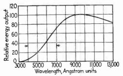
Fig. 34.—Spectral distribution of a standard tungsten incandescent lamp operated at 2870°K. The arrows mark the approximate limits of the visible region of the spectrum (violet, 4000 Angstroms, to red, 7000 Angstroms).
