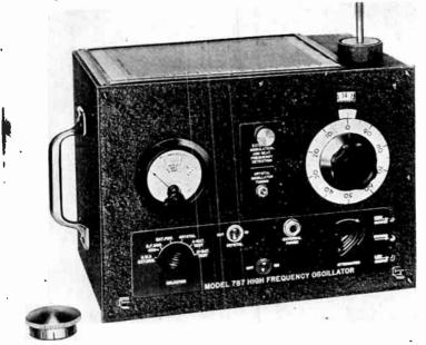
Fig. 306A.—External appearance of u-h-f signal generator, suitable use in method shown in Fig. 305.
