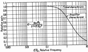
Fig. 118.—High-frequency amplitude-response characteristic of the uncompensated amplifier (Fig. 117) plotted in terms of the reference frequency  $f_o$  determined by the values of shunt resistance and capacitance in the coupling circuit.
