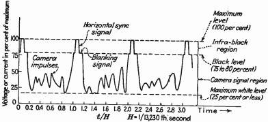
Fig. 98.—Three lines and blanking periods of the R.M.A. Standard Video Signal.
