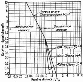
Fig. 153.—Empirical values of field strength within and beyond the horizon distance,  $r_{\lambda}$ .
