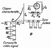
Fig. 217.—Separation of picture signal and sync pulses. The demodulated carrier signal is obtained by the method shown in A. This signal is then passed through a clipper stage which responds only to the positive peaks of the signal, which are the sync pulses, as shown in B.
