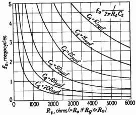
Fig. 119.—The reference frequency  $f_o$  in terms of the shunt capacitance  $C_i$  and resistance  $R_i$ .
