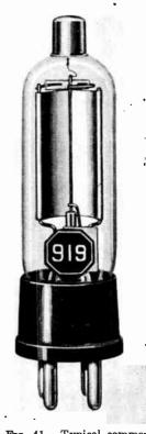
Fig. 41.—Typical commercial phototube. The hemicylindrical cathode, when illuminated, releases electrons which are collected by the central wire anode.
