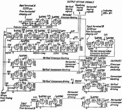
Frg. 255.—Vertical shaping unit of the sync signal generator. The 60-c.p.s. timing impulses from the timing unit are shaped to provide the keying signals used in the horizontal shaping unit (Fig. 254). Combined blanking signals (for the control amplifier, Fig. 244) are derived, as well as impulses for driving the iconoscope deflecting circuits and blanking the iconoscope scanning beam during retrace.
