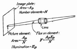
Frs. 32.—Light flux contained in a single picture element, computed from the illumination and the area of the element.
