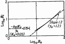
Fig. 198.—Transfer characteristic of Fig. 197 plotted in logarithmic coordinates. The gamma is the slope of the straight line (dashed) which most nearly fits the actual curve. The proportionality constant is determined from the intercept of the straight line with the  $\log_{10}B_0$  axis.
