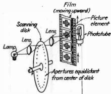
Frg. 45.—Light-source scanning of motion-picture film. In this arrangement, all the light is directed to each successive picture element, and subsequently collected by the phototube. When a multiplier phototube is used this method is capable of high-definition transmission with adequate signal-to-mask ratio.
