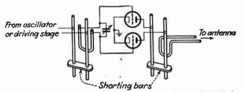
Fig. 156.—Typical push-pull r-f amplifier stage employing transmission-line segments as tuned circuits.
