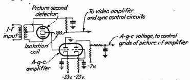
Fig. 225.—Typical automatic-gain-control circuit employing two stages of direct-coupled amplification.
