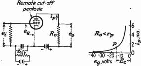
Fig. 137.—Typical distorting amplifier circuit used for obtained nonlinear reproduction ("gamma-control" amplifier). By adjusting the bias voltage  $E_{\epsilon}$  different portions of the  $i_v$ - $\epsilon_v$  operating characteristic may be chosen.
