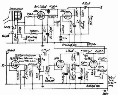
Fig. 242.—Complete diagram of iconoscope preamplifier.
