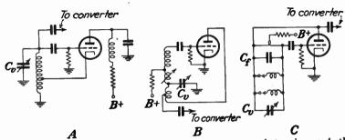
Fig. 176.—Oscillator circuits suitable for television superheterodynes: A, the floating-cathode circuit; B, center-tuned; C, shunt-inductance tuned. All are variations of the Hartley circuit. The capacitor  $C_v$  in each case is used as a trimmer.
