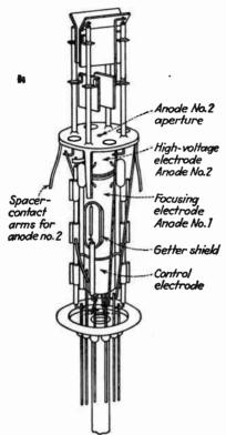
Fig. 199B.—Electron gun and deflecting structure of the 5AP4 picture tube.
