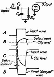
Fig. 253B.—The delay function in wave-shaping circuits. The delay circuit (top) produces a curved wave (B) from the initial square wave (A). The curved wave is clipped and the portion above the clip level is amplified, and then clipped again, resulting in a square wave delayed by the amount shown.
