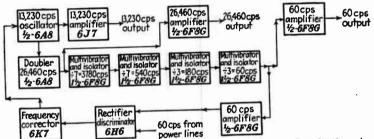
Fig. 248.—Block diagram of the timing unit of the synchronisation signal generator, which produces 60-c.p.s. and 13,230-c.p.s. timing impulses and coordinates them with the power supply.
