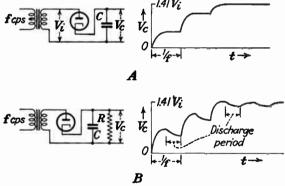
Fig. 209.—Effect of resistance load on ripple in high-voltage supply: A, voltage build-up across capacitor alone (no leakage); B, discharge through load resistor.
