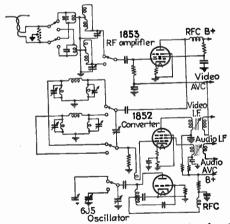
Fig. 177.—Input, r-f, converter and oscillator circuit of a typical television receiver, described by Lyman.
