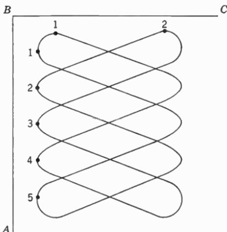
FIG. 20. Method of calculating frequency from Lissajous pattern.
