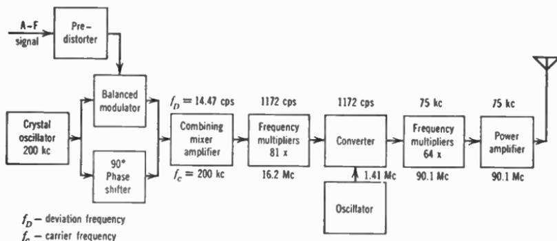
FIG. 6. Block diagram of Armstrong system transmitter.
