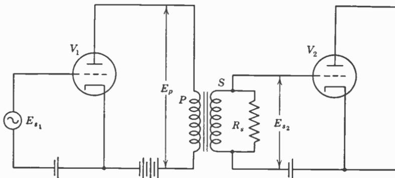
FIG. 9. Transformer-coupled amplifier.
