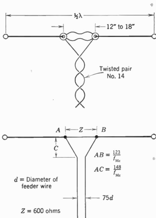
FIG. 16. Manner of connecting transmission lines to antennas to produce proper impedance match.
