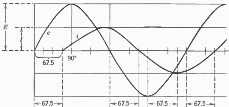
FIG. 13. Current and voltage in an inductive circuit where the maximum current lags behind the maximum voltage.
