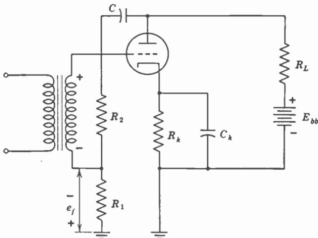
FIG. 20. A voltage-feedback circuit.
