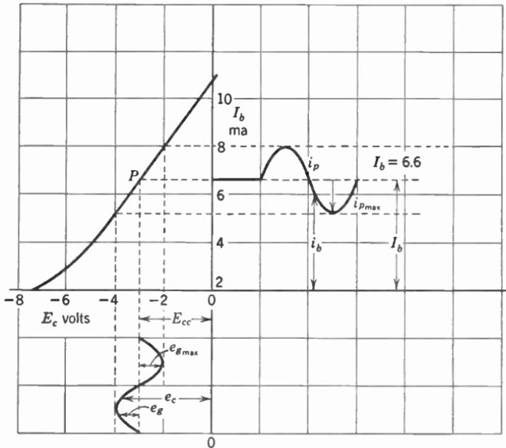
FIG. 2. Alternating voltages superimposed on the steady (bias) grid voltage produce a pulsating plate current which rises and falls from its steady (d-c) value.
