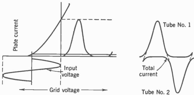
FIG. 15. Plate and total currents in a Class B push-pull amplifier.
