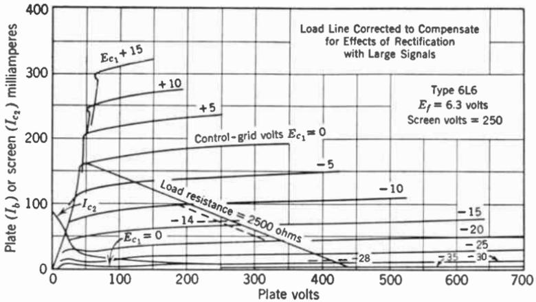
FIG. 16. Plate voltage-plate current curves of beam power tube.
