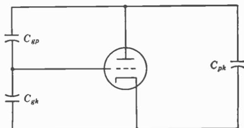
FIG. 6. Tube interelectrode capacitances.
