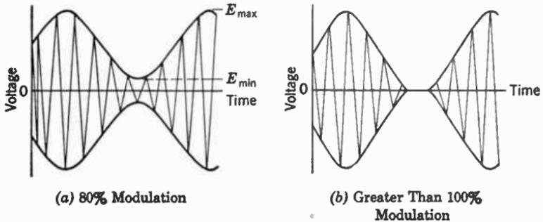
FIG. 22. Amplitude-modulated carrier as seen on a cathode-ray oscillograph.
