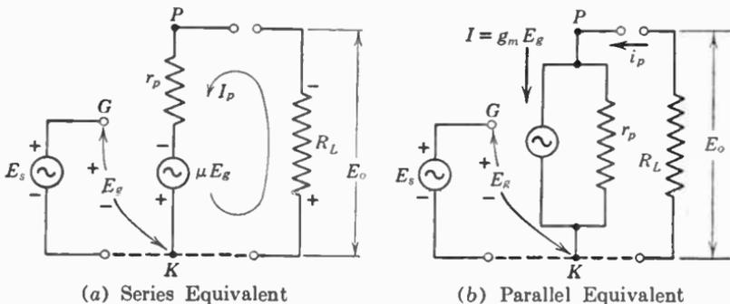
FIG. 4. A-c equivalent circuits of tubes. D-c elements are not shown. Dashed lines indicate connections for amplifier shown in Fig. 1.
