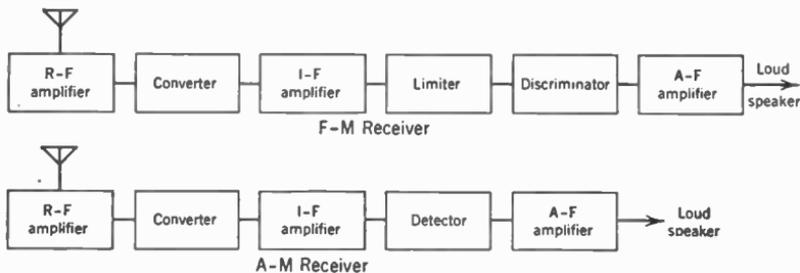
FIG. 7. Comparison of f-m and a-m receivers.
