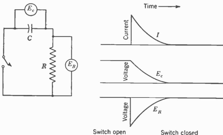
FIG. 2. In this figure the condenser is charged. When the key is closed, current flows through the circuit, building up a voltage across  $R$  which opposes  $E_c$ . When the charge in  $C$  has been dissipated, current ceases and  $E_c$  and  $E_R$  both become zero.
