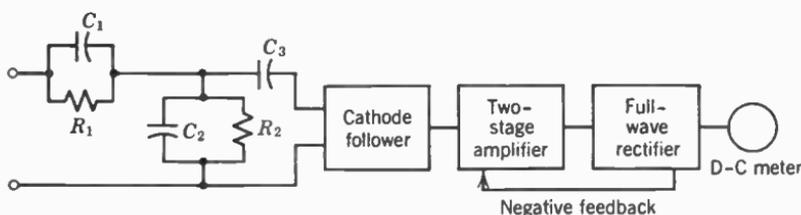
FIG. 9. Amplifier followed by diode rectifier.
