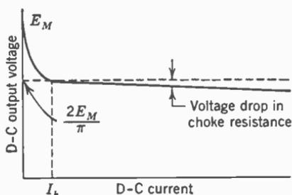
FIG. 14. Typical regulation curve for a choke-input filter.
