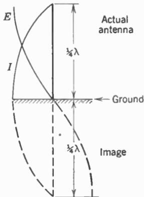
FIG. 8. Quarter-wave grounded antenna.
