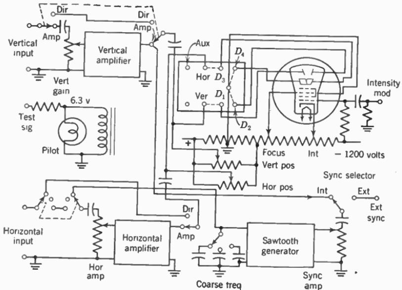
FIG. 16. Circuit of a typical cathode-ray oscilloscope.
