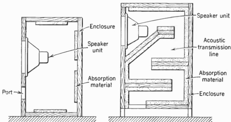
FIG 16. Bass reflex housing for improving low-frequency response of dynamic speaker.
