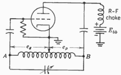
FIG. 4. Hartley oscillator. This is a "shunt-fed" circuit.
