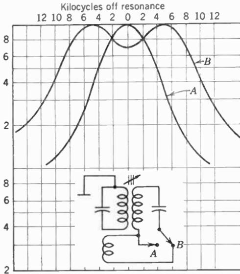
FIG. 11. Selectivity curve for two-position i-f transformer.
