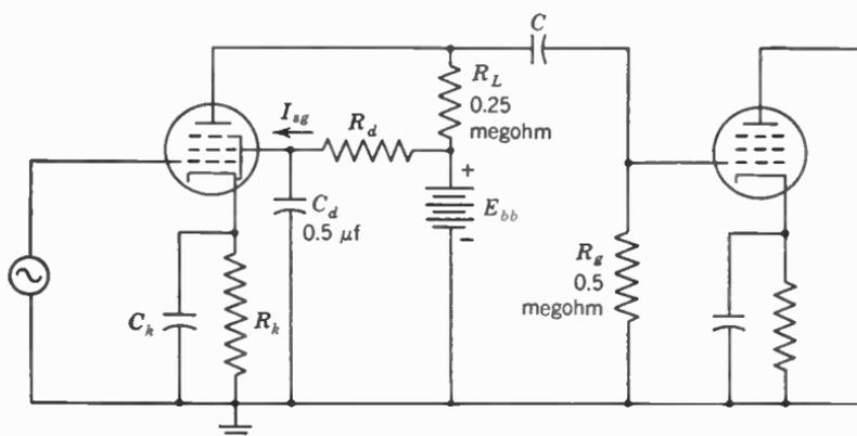
FIG. 7. Typical RC amplifier using pentode tube.
