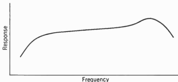
FIG. 10. Typical frequency response of a transformer-coupled amplifier.
