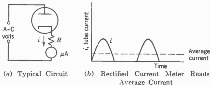
FIG. 6. Simple average-reading diode voltmeter. \*
