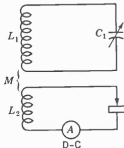
FIG. 3. A simple frequency meter.
