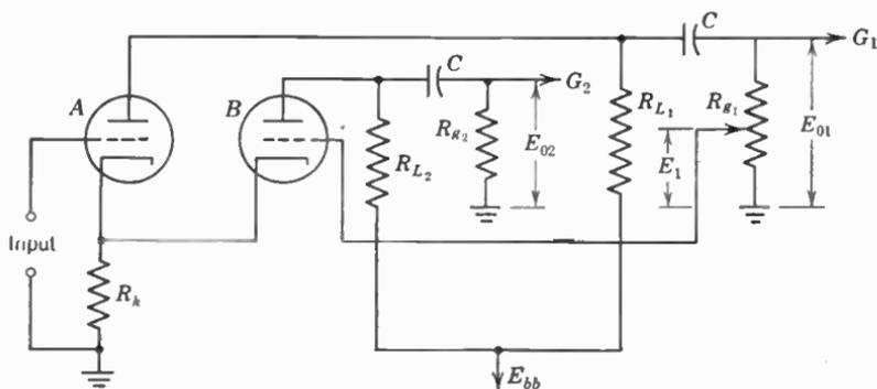
FIG. 17. A phase-inverter circuit used to drive a push-pull amplifier.
