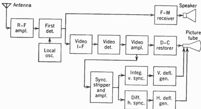
FIG. 7. Simplified block diagram of a typical television receiver.
