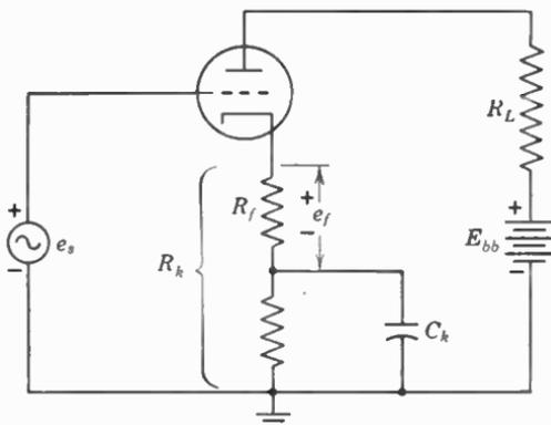
FIG. 19. Negative-feedback voltage is produced across resistor  $R_f$ . This is called current feedback.
