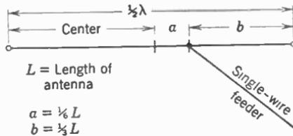
FIG. 18. Proper place to connect a single-wire feeder to an antenna for most efficient energy transfer.
