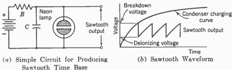
FIG. 13. Sawtooth generator.
