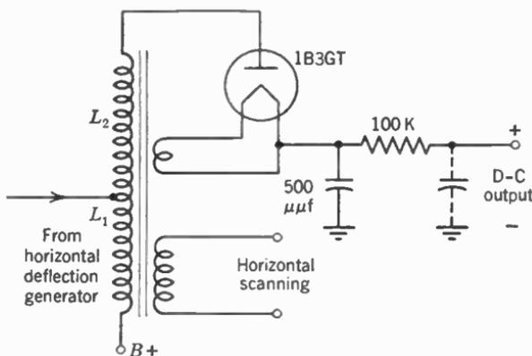
FIG. 10. Flyback power supply.
