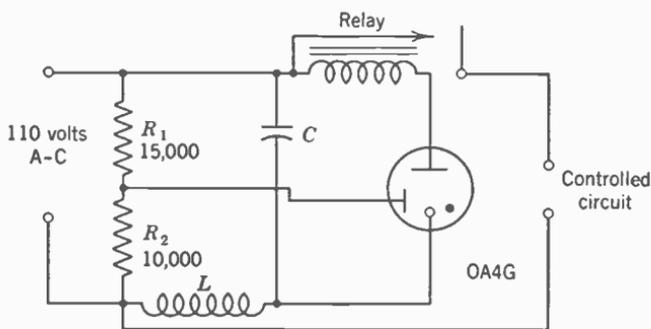
FIG. 4. Use of gas tube in a remote-control circuit.
