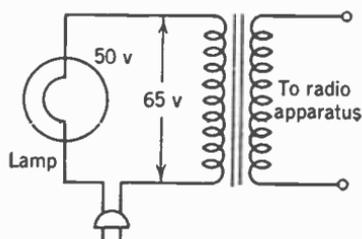
FIG. 19. Use of current regulator or ballast tube.
