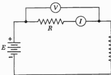
Fig. 12. Ammeter-voltmeter method of measuring resistance.
