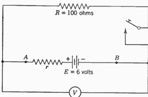
FIG. 19. In this diagram,  $r$  represents the internal resistance of the battery.
