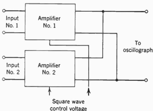
FIG. 23. Electronic switch for oscillograph.
