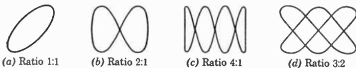
FIG. 19. Lissajous patterns resulting from application of signals of different frequencies on horizontal and vertical plates.
