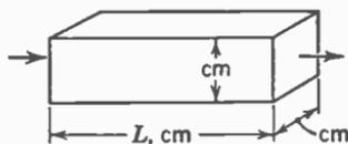
FIG. 4. Reluctance depends directly upon the length and inversely upon the area of the material.
