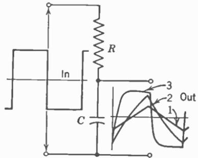
FIG. 5.  $RC$  integrating circuit.
