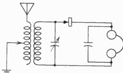
FIG. 1. Detector using a crystal as rectifier.
