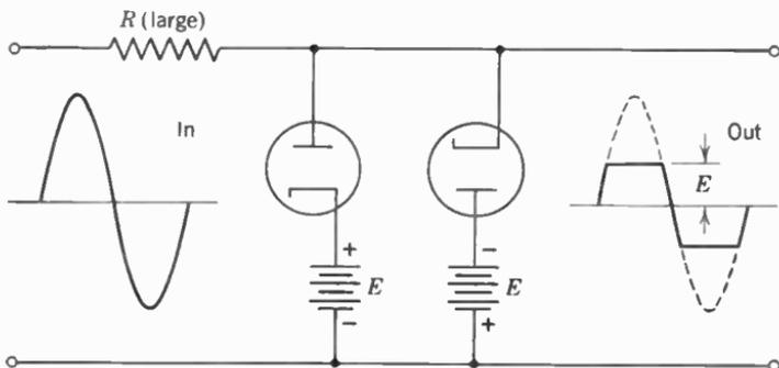
FIG. 9. Diode circuit which clips both peaks.
