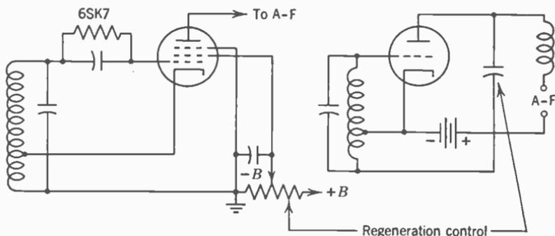
FIG. 3. Two feedback circuits for improving sensitivity of a detector.
