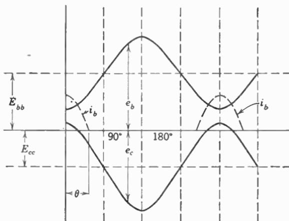
FIG. 3. Relations existing in Class C amplifier. The angle during which plate current flows is  $2\theta$ . The grid voltage magnitude is exaggerated here.
