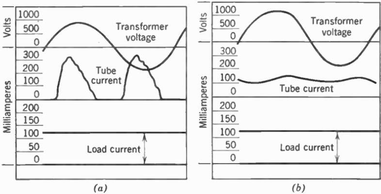
FIG. 12. High instantaneous current required by condenser-input filter (a) compared to the lower currents passed by the inductance-input filter (b).
