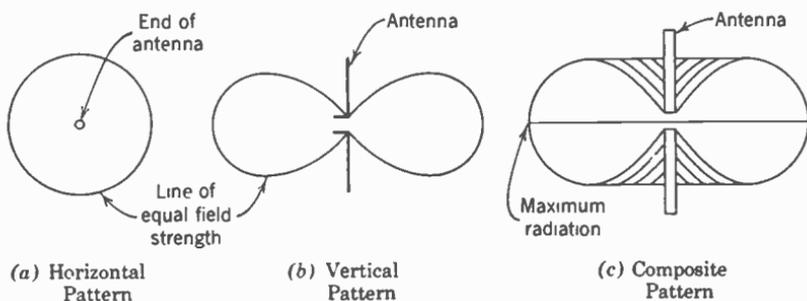
FIG. 10. Field patterns of an isolated half-wave dipole.
