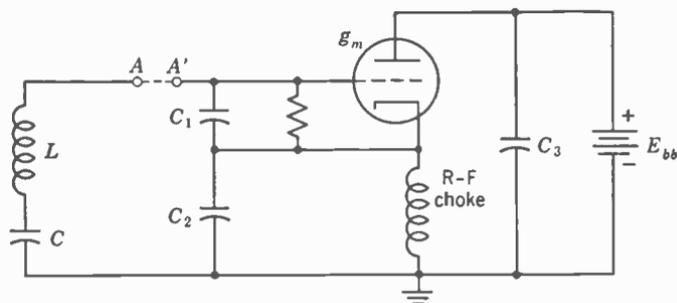
FIG. 7. A modified Colpitts oscillator. The impedance at  $A-A'$  has a negative resistance component equal to  $-X_{C_1}X_{C_2}g_m$ .
