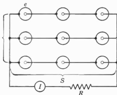
FIG. 22. A series-parallel arrangement of cells enables more current and more voltage to be obtained than from a single cell.
