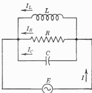
FIG. 27. In this parallel circuit  $I$  may be very small compared to the branch circuit currents  $I_L$  or  $I_C$ .
