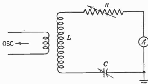
FIG. 5. When  $L$  is coupled loosely to an oscillator and  $C$  is varied, the current indicated at  $I$  will go through a maximum like that in Fig. 4.
