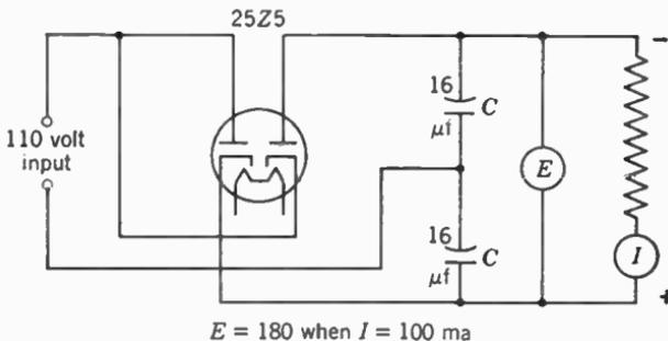
FIG. 8. A rectifier with two plates and two cathodes will double the voltage obtainable from a single diode.
