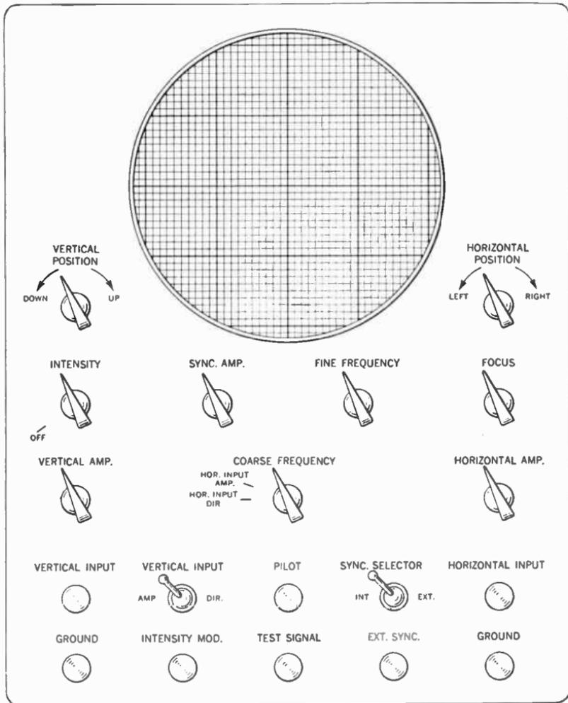
FIG. 15. Front panel of a typical cathode-ray oscillograph.
