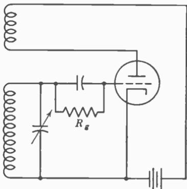
FIG. 1. Tuned-grid oscillator.
