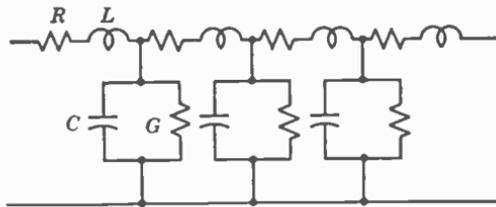
FIG. 1. Approximate equivalent circuit of a transmission line.
