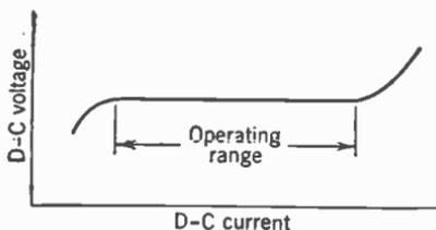
FIG. 18. Typical characteristics of a voltage-regulator tube.
