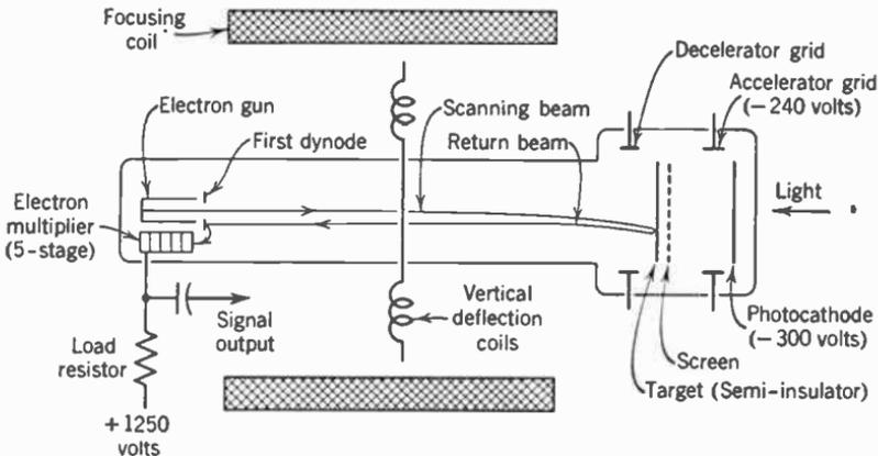
FIG. 3. Image orthicon, simplified diagram.
