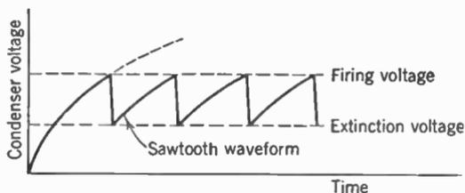
FIG. 16. Voltage waveform of relaxation oscillator of Fig. 15.
