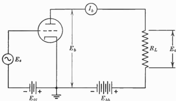
FIG. 1. Basic amplifier circuit with resistance load  $R_L$ .
