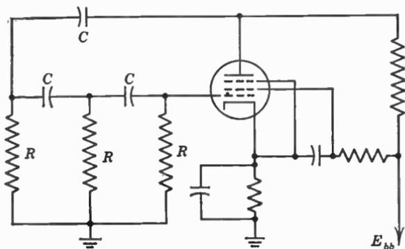
FIG. 17. Phase-shift oscillator.
