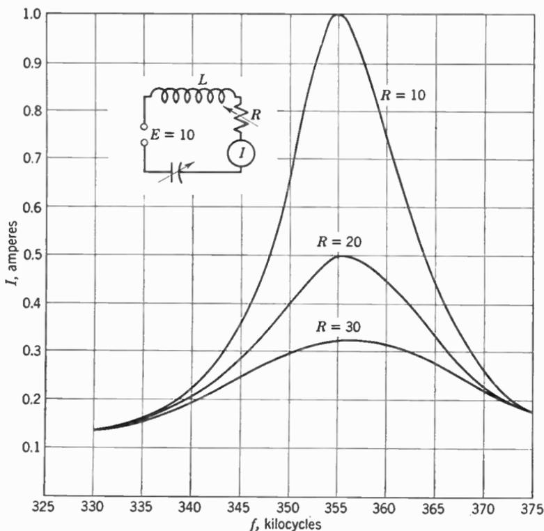
FIG. 10. Effect of resistance on a resonance curve. Note that the current far from resonance is not changed so much as the resonant current.
