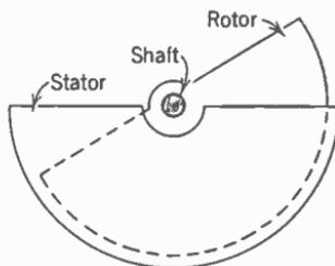
FIG. 2. Variable air condenser.
