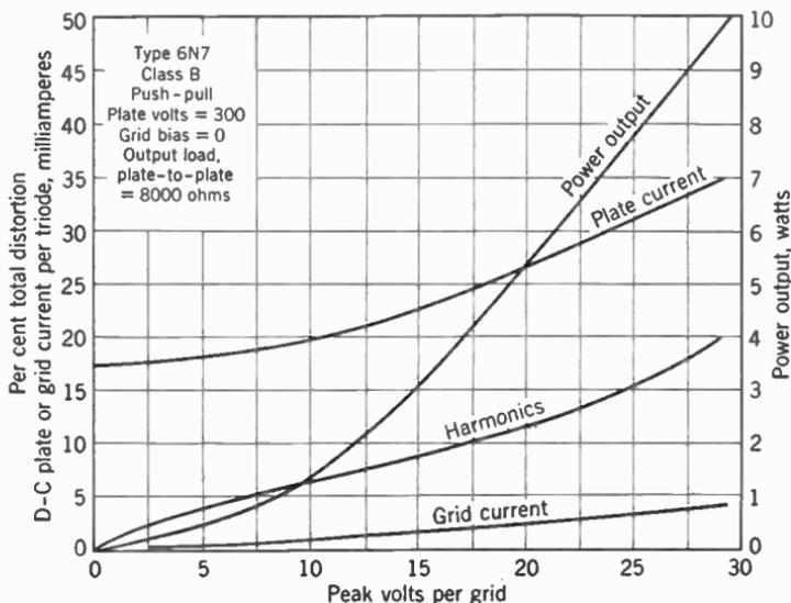
FIG. 16. Operating characteristics of a 6N7 Class B push-pull amplifier.
