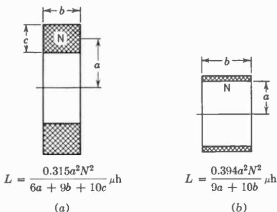
FIG. 4. Typical coil forms and formulas by which the inductance may be calculated. Dimensions are in centimeters.
