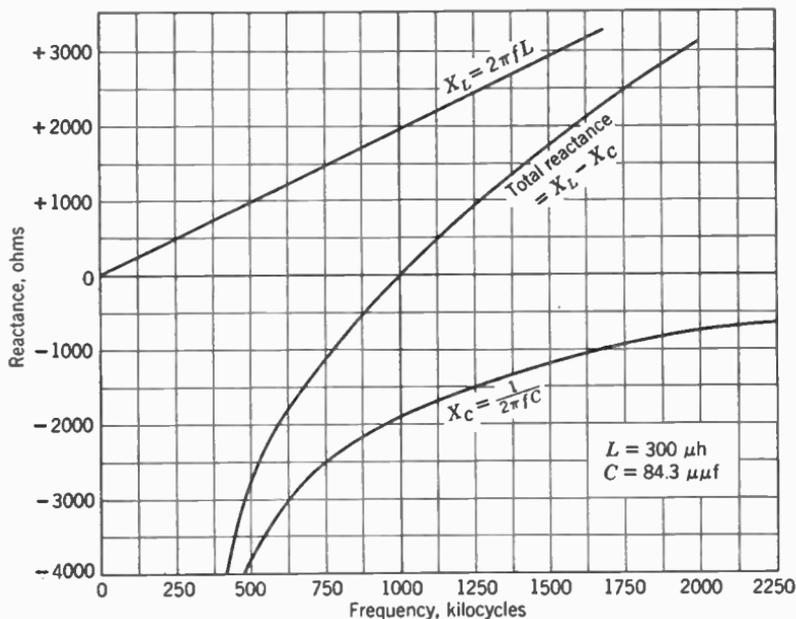
FIG. 9. A plot of the reactance of a coil and a condenser in series.  $X_L$  rises in direct proportion to  $f$ ;  $X_C$  rises inversely as  $f$ . The sum,  $X_L - X_C$ , changes from a high negative value where  $X_C$  is greater than  $X_L$ , through zero where  $X_L = X_C$ , to a high positive value where  $X_L$  is greater than  $X_C$ .
