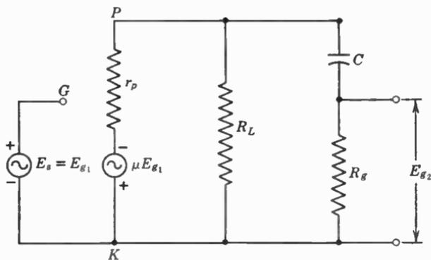
FIG. 3. A-c equivalent of circuit of Fig. 2.
