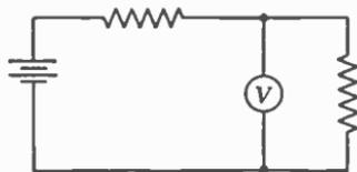
FIG. 8. Voltmeter goes across circuit being measured.
