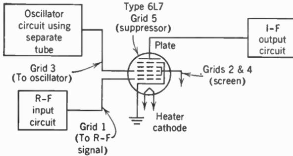
FIG. 8. Mixer tube and circuit useful at high frequencies.
