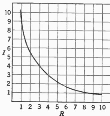
FIG. 5. Current is inversely proportional to the resistance, decreasing as the resistance increases.
