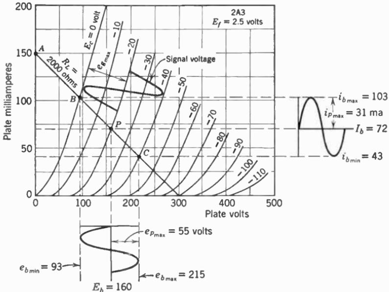
FIG. 7. The straight line AC is the load line. The value of plate current for various values of grid voltage is found along this line.
