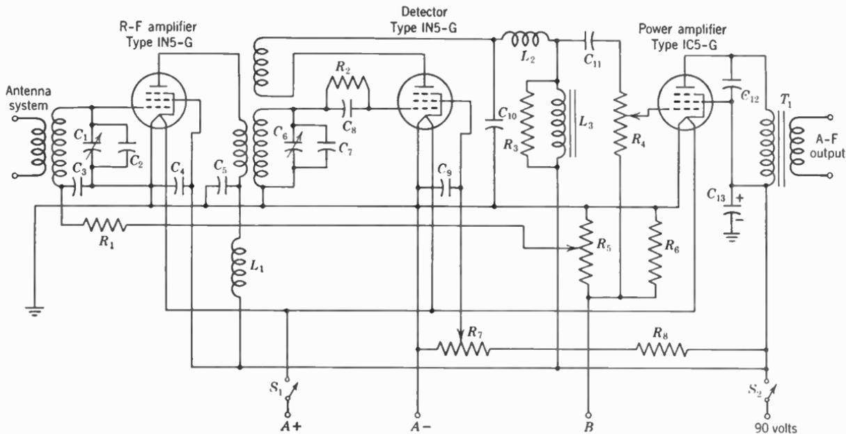
FIG. 4. Typical short-wave receiver using one stage of r-f amplification and a regenerative detector.
