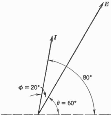
FIG. 15. Current leads the voltage at an angle  $\phi$  of  $20^\circ$ . Voltage is at  $60^\circ$  phase.
