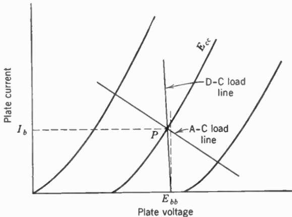
FIG. 11. D-c and a-c load lines for a transformer-coupled amplifier.
