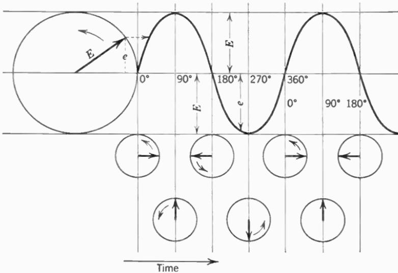
FIG. 1. As the vector  $E$  rotates, the vertical height,  $e$ , of the end of the vector varies according to the curve known as a sine wave. When the vector has the position as shown in the first small circle, the instantaneous value  $e$  is zero. At other times the instantaneous voltage has the other values as shown.
