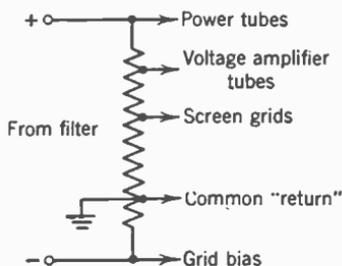
FIG. 15. Voltage divider for supplying various voltages to an amplifier.
