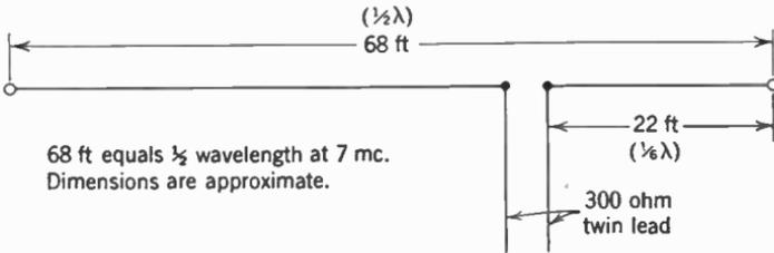
FIG. 17. Method of feeding a half-wave antenna with a 300-ohm line at 7 and 14 Mc.
