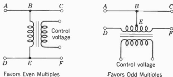
FIG. 13. Methods of injecting controlling voltages in multivibrator of Fig. 11.
