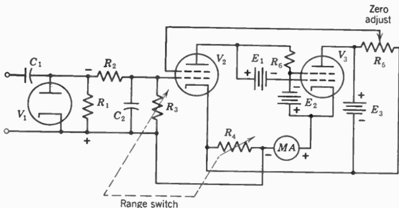
FIG. 8. Diode rectifier with d-c amplifier to enable the use of a more rugged indicating instrument.
