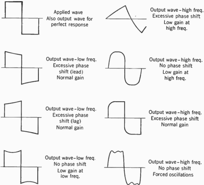
FIG. 14. Typical square-wave responses of a-f amplifiers.
