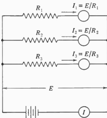
FIG. 11. A parallel circuit with meters to indicate the currents through the individual branches.
