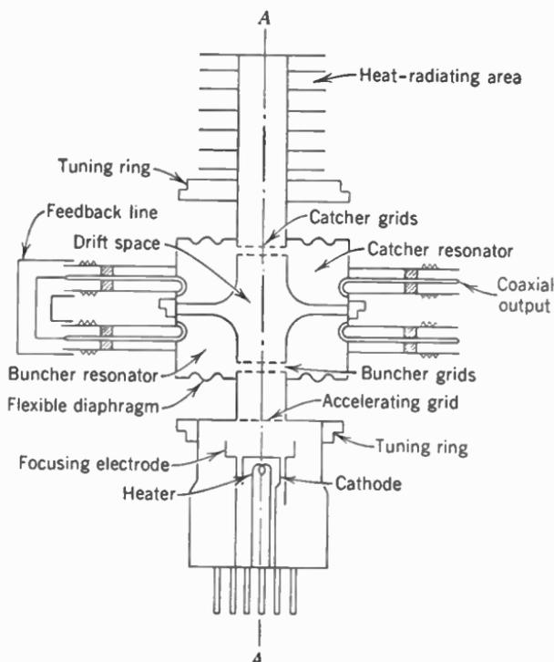
FIG. 8. Sectional view of the 410-R/2K30 klystron of Sperry, a tube of the velocity-modulation type which makes possible generation, amplification, and conversion of frequencies in the centimeter-wavelength region. The tube is 6 in. long overall.
