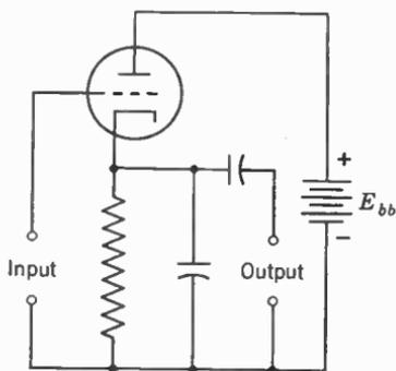
FIG. 13. Infinite input impedance detector.
