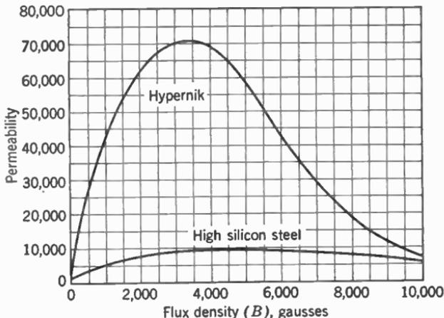
FIG. 10. Curves of two types of magnetic materials, showing how the permeability can be increased by use of alloys and heat treatment.
