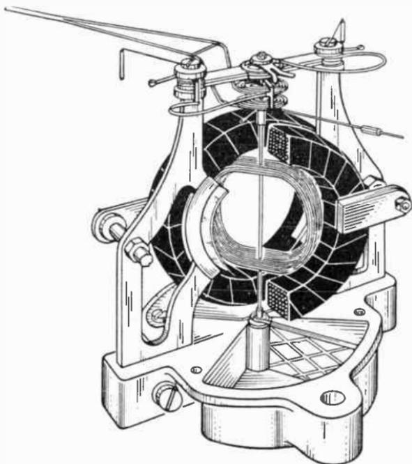
FIG. 6. Dynamometer type of instrument for alternating current.
