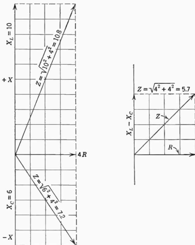
FIG. 22. At left is resultant of combining reactances and a resistance to form two  $Z$  vectors. At right, the two reactances have been added to form a net reactance of 4 ohms, which is then combined with a resistance of 4 ohms to form an impedance of 5.7 ohms.
