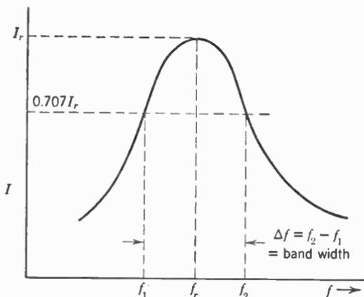
FIG. 19. The band width of a series-resonant curve is the number of cycles between points on the curve at which the current is equal to 0.707 times the maximum value,  $I_r$ .
