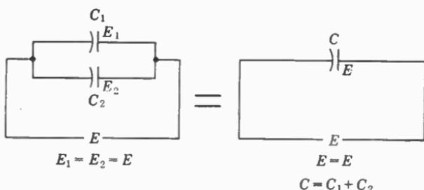
FIG. 8. Condensers in parallel.
