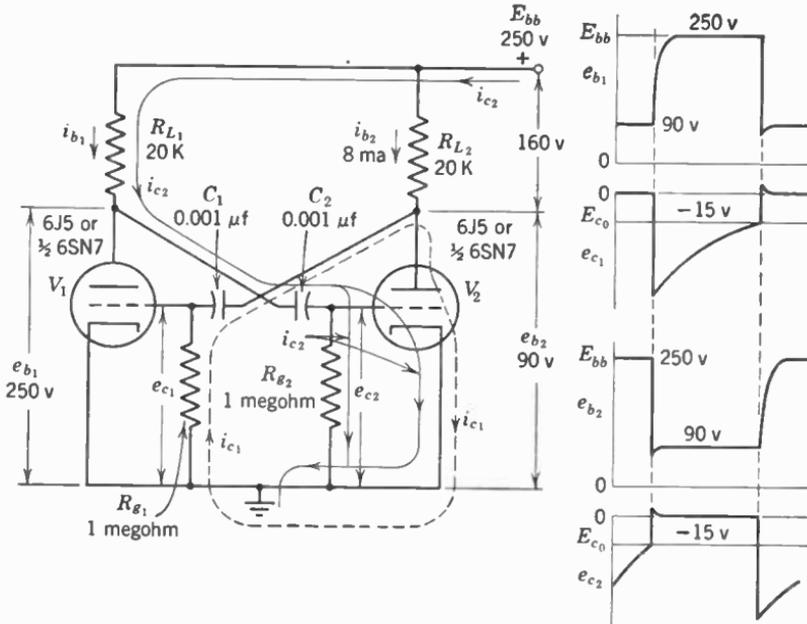
FIG. 12. Waveforms in a plate-coupled multivibrator.
