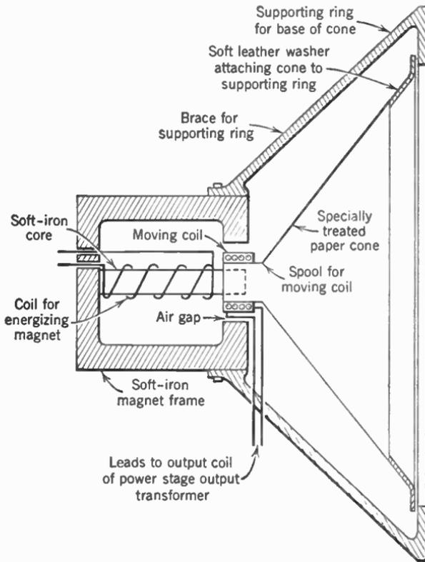
FIG. 14. Modern "dynamic" or moving-coil loud speaker.
