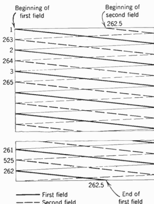
FIG. 1. Interlaced scanning sequence. Spacing between scanning lines is actually much closer than shown.
