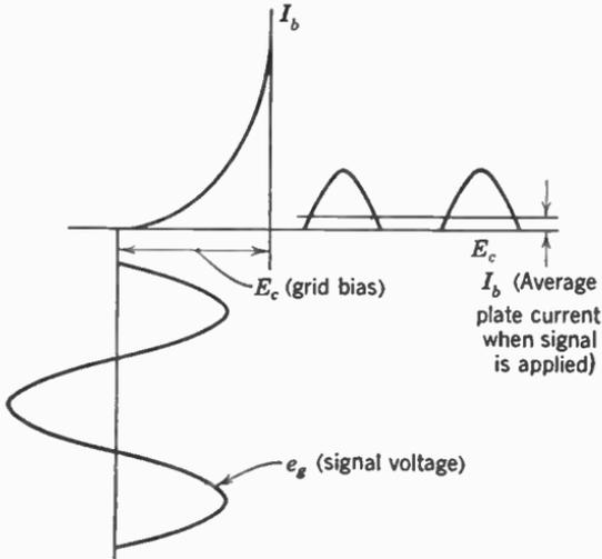
FIG. 3. When bias is well beyond cut-off, peaks of input voltage determine plate current.
