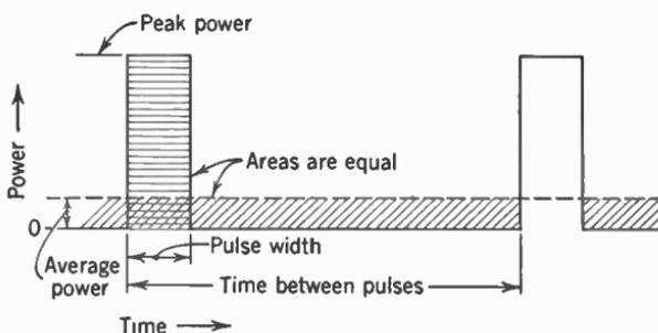
FIG. 4. High peak power does not mean high average power. In radar transmitters the time between pulses may be quite long compared to pulse time.
