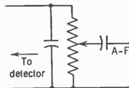
FIG. 11. Tapping the output of the detector puts stray capacitances across only part of the detector load, thus increasing the impedance of this load.
