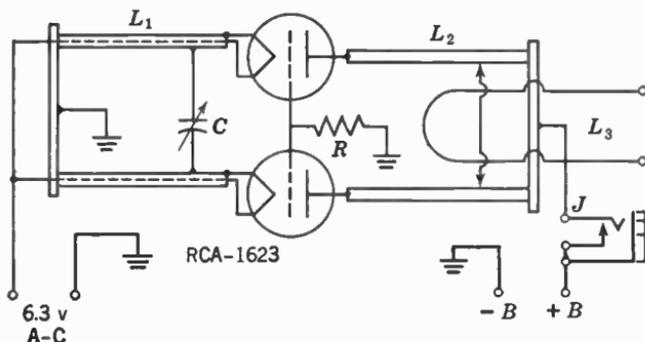
FIG. 3. A-c push-pull  $2\frac{1}{2}$ -meter, 45-watt oscillator, RCA-1623 tubes;  $C = 15 \mu\text{f}$ ;  $R = 1000$  ohms, 5 watts;  $L_1$  and  $L_2 = 12$ -in. lengths of  $\frac{1}{2}$ - and  $\frac{5}{8}$ -in. metal tubing, spaced 1 in. and  $1\frac{1}{8}$  in. between centers, respectively; plate voltage = 500 for CW; plate current = 200 ma.
