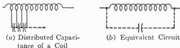
FIG. 21. "Distributed" capacitance exists between each pair of turns of a coil. This capacitance limits the usefulness of coils at high frequencies.
