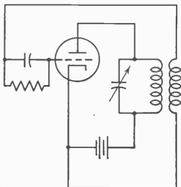
FIG. 2. Tuned-plate oscillator.
