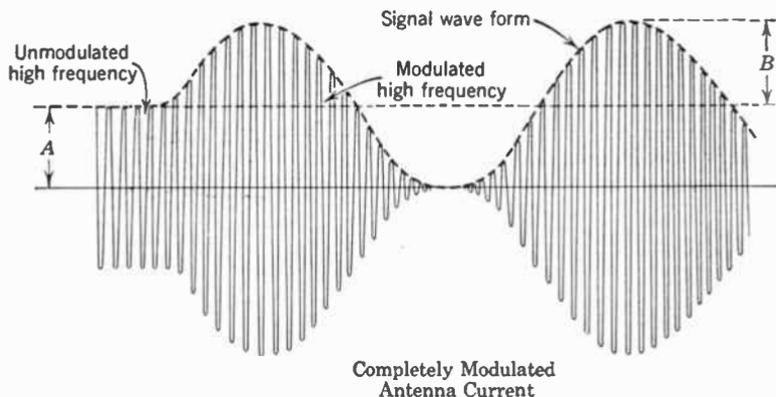
FIG. 6. Radio-frequency wave before and after modulation.
