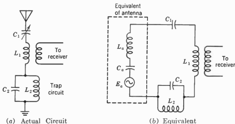
FIG. 15. The anti-resonant circuit in series with the antenna rejects undesired signals by making the series impedance to these signals very high.
