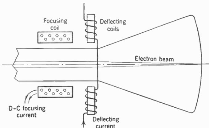
FIG. 11. Cathode-ray tube with magnetic focus and deflection.
