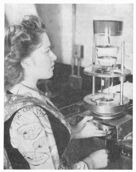
Fig. 2.14 Method of applying a coating of electrically conductive material to a cathoderay tube, creating an electrode upon the interior walls of the tube, which serves to accelerate the beam as well as to remove electrical charges from the walls of the tube.
