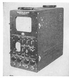
Fig. 9.16 The Du Mont type 5031-A mixer-amplifier and monitor. (Courtesy of Allen B. Du Mont Labs., Inc.)
