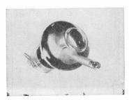
tion receiver in which it is used is illustrated in Fig. 8.79. The screen of this tube is 7.5 in. in diameter. It has projected images upon a screen measuring 15 by 20 ft.
