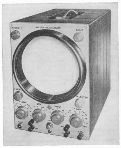
Fig. 3.15 R.C.A. type WO-56A cathode-ray oscilloscope. This is an example of an advanced type of test instrument available to the television engineer and technician. (Courtesy of Radio Corporation of America.)
