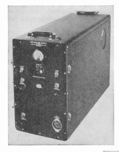
Fig. 9.18 Du Mont type 5029-A low-voltage power supply. (Courtesy of Allen B. Du Mont Labs., Inc.)
