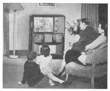
Fig. 8.81 An R.C.A. projection receiver incorporating the Schmidt optical system. (Courtesy of Radio Corporation of America.)
