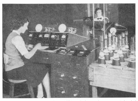
Fig. 2.36 Typical test console. The Du Mont cathode-ray tube must pass 18 electrical and 12 mechanical tests after manufacture. (Courtesy of Allen B. Du Mont Labs., Inc.)
