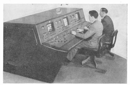
Fig. 9.25 Du Mont dual Iconoscope camera control console for film pickup. (Courtesy of Allen B. Du Mont Labs., Inc.)
