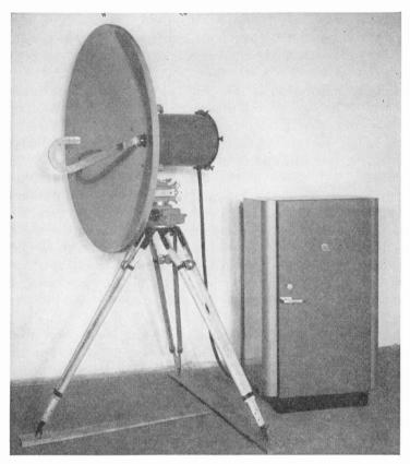
Fig. 9.27 R.C.A.'s microwave-link equipment for television relaying. (Courtesy of Radio Corporation of America.)
