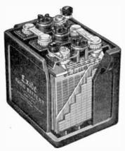
Fig. 42.—Cross-section of leadplate storage cell.
