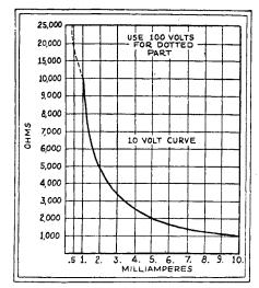
FIG. 26C—The 10-volt calibration curve. The dotted portion is for an applied voltage of 100.
