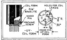
FIG. !!-Mounting coil-tubes to a plug-in base.
