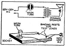
FIG. 4—Using a neon bulb as a help in centering speaker-cones.
