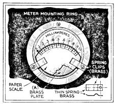
FIG. (1—The desired paper scale is pasted over a removable non-magnetic plate (A).
