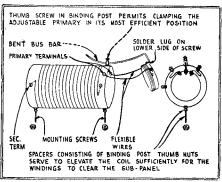
FIG. 14-A novel 3-circuit tuner.
