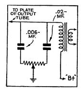
FIG. 4-A novel tone-control circuit.
