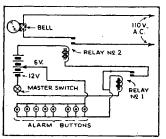
FIG. 28-Burglar alarm system using Ford cut-outs.
