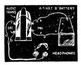
FIG. 6-Testing for noisy audio transformers.
