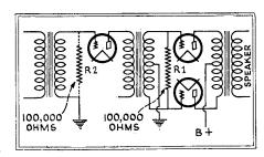
FIG. 4—These resistors give a solution of the persistent hum problem.
