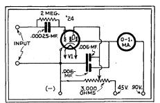
FIG. 15--Circuit of a Dynatron V.T. Voltmeter.
