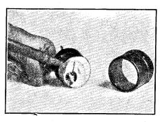
FIG. 9C—A voltmeter, with its case removed, undergoing the operation described by Mr. Nothelfer, which gives access to the basic milliammeter unit.
