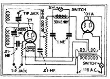
FIG. 2!—This oscillator, with home-made power transformer, is an extremely-compact and convenient device, modulated by the A.C. hum of the light line. A jumper is put across the lower tip jacks when the meter is not in circuit.
