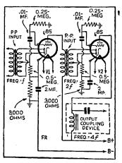
FIG. I—Circuit of frequency-doubling idea. Lower right, frequency quadrupled.
