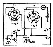
FIG. 4-Low-capacity condenser tester.
