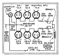
FIG. 5—Final connection of the series-parallel circuit C, Fig. 4.
