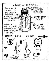
FIG. 22-Home-made photo-voltaic cell.
