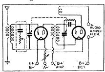
FIG. I-Design for a good volume control.
