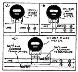
FIG. 3—How to figure wattage drain by use of the regular light-line power meter.
