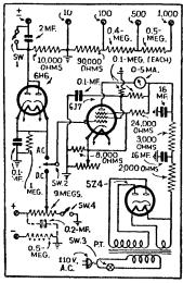
FIG. 14-A Versatile V.T. Voltmeter.
