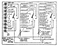
FIG. 24—A resistance-capacity box which saves time.
