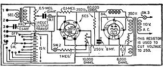
FIG. 16—Here is an improved version of the "Magic Eye" leakage tester described in March, 1936, Radio-Craft. Several features have been added, which make the apparatus much more adaptable.
