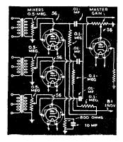
FIG. 4-Circuit of the low-cost mixer.
