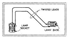
FIG. I—The dial-light is converted into a trouble-shooting lamp by the use of this simple adapter.
