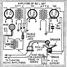
FIG. 2—The mechanical coupling of a pickup`to a magnetic speaker gives an input for an audio amplifier.
