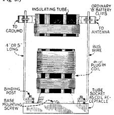
FIG. 4—A tube-base plug-in coil is easily equipped with an adjustable winding in this way.
