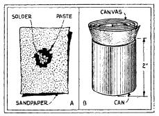
FIG. 5—The two accessories shown make it more convenient to do a good job of soldering.
