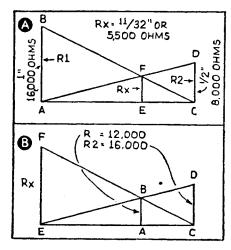
FIG. 4—Simple graphic calculating of parallel resistances.
