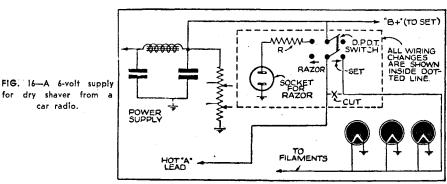
of the correct value to reduce the voltage delivered by the power supply to approximately 110 volts when the razor is running. This value must be found by experimentation.
