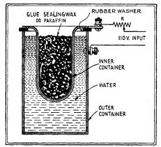
FIG. 7—An easily-constructed glue pot, recommended as an emergency construction design. It may be used regularly for light work.
