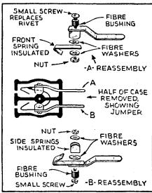
FIG. 21-The test-lamp adapter unit.
