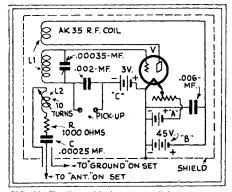
FIG. 20—The "portable broadcaster" is a very compact oscillator, built into a portable phonograph which gives modulation.
