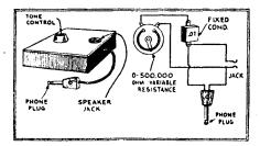
FIG. 3-The circuit of the portable tone-control box.
