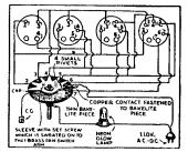
FIG. 4-A tube-short tester.
