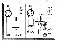
FIG. 26A, left—Theoretical circuit of the resistance calculator. FIG. 26B, right—Final circuit diagram of the calculator.
