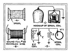
FIG. I—An additional inductance in shunt across a coil lowers the wavelength, if there is not too much self-capacity.
