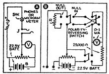
FIG. 19-Measures A.V.C. circuits accurately.
