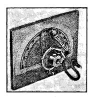
FIG. 2A-Homemade illuminated vernier dial
