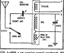
FIG. 6—With a set covering several wavebands, this switch makes it more convenient to change the aerial coupling.
