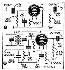
FIG. 5—Uses for old "tuning eye" tubes. target should be grounded when not used.
