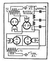
FIG. 11-Circuit of novel high-voltage power supply.
