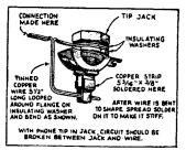
FIG. 6, above-Re-making a tip jack.
