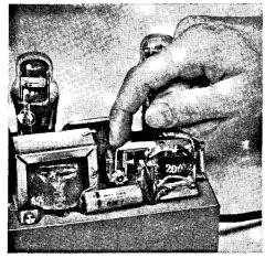
A close-up of the motor that turns the dual condenser
