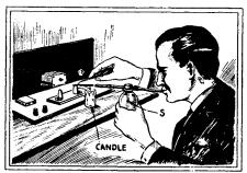
FIG. I—Biowpipes are obtainable from laboratory supply houses; but Mr. Kitchin takes this ingenious way to make one of light weight. (The bottle may be retained as a handle!)
