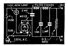
FIG. 18—A novel A.C.-D.C. "B" power supply, using a filament-type tube as rectifier.
