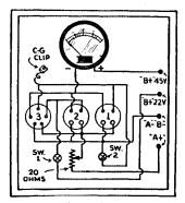
FIG. 2-A self-contained tube tester.
