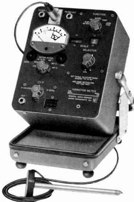
Figure 6-12. Type 1553 Vibration Meter shown with pickup connected.
