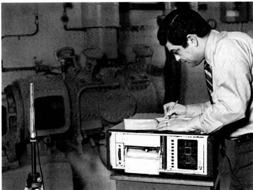
Figure 6-16. Type 1523 Graphic Level Recorder being operated with the Type 1523-P3 plug-in to make automatic stepped 1/3-octave-band analyses of compressor noise.
