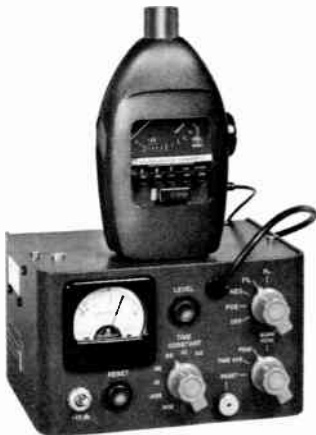
Figure 6-25. The Type 1565 Sound-Level Meter can be combined with a Type 1556 Impact Noise Analyzer to give direct readings on impulse-type noise.
