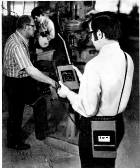
Figure 6-24. Type 1935 Cassette Data Recorder storing inputs from a GR 1933 SLM.
