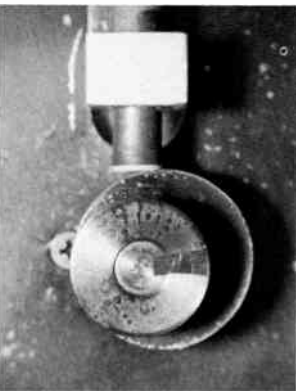
Figure 9-3. Sequence of photographs shows misbehaving cam and follower. The cam is rotating at 2000 rpm. The photographs were taken with stroboscopic illumination at different phases of the cam cycle to show the bouncing action when the cam rotates above a critical speed.
