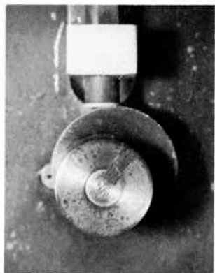
Figure 9-3. Sequence of photographs shows misbehaving cam and follower. The cam is rotating at 2000 rpm. The photographs were taken with stroboscopic illumination at different phases of the cam cycle to show the bouncing action when the cam rotates above a critical speed.
