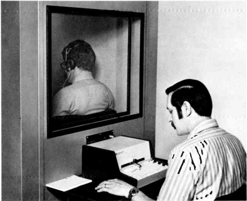
Figure 4-2. Automatic audiometer test showing a freshly recorded audiogram of actual hearing-acuity response. The subject is seated in the GR 1939 Audiometric Examination Room.
