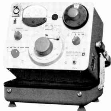
Figure 6-15. The Type 1564 Sound and Vibration Analyzer shown with selectivity characteristics.
