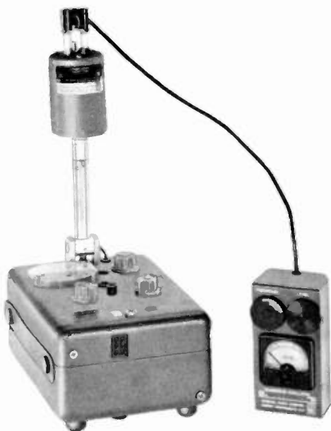
Figure 4-9. Type 1552-B Sound-Level Calibrator on the microphone of a sound-level meter for calibration. Type 1307-A Transistor Oscillator is audio source.
