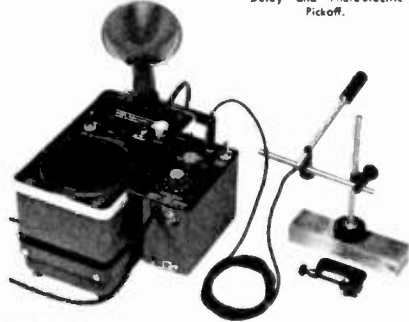
Stroboscac shown with Flash Delay and Photoelectric Pickoff.
