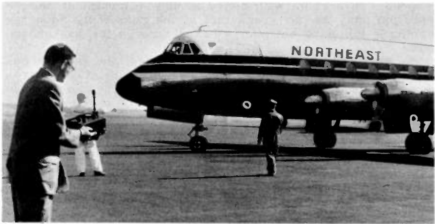
Figure 5-4. Sound-level meter being used to check noise at flight line.
