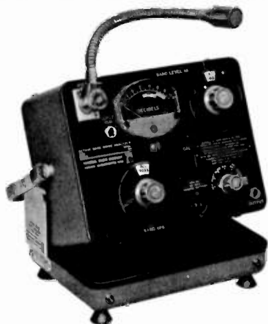
The Type 1558-A Octave-Band Noise Analyzer with the Type 1560-P6 Microphone Assembly.
