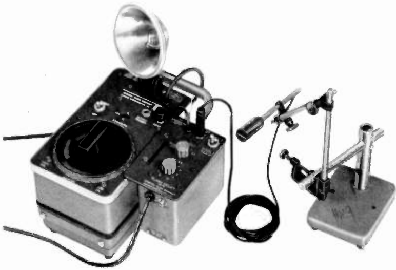
Figure 11-9. Type 1531-A Strobotac ® electronic stroboscope (left), Type 1531-P2 Flash Delay (attached to stroboscope), and Type 1536-A Photoelectric Pickoff.
