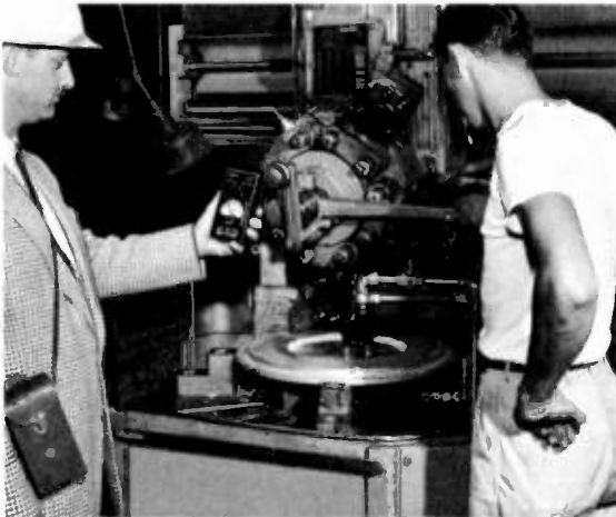
Figure 5-1. The Sound-Survey Meter being used for a preliminary investigation of machine noise.
