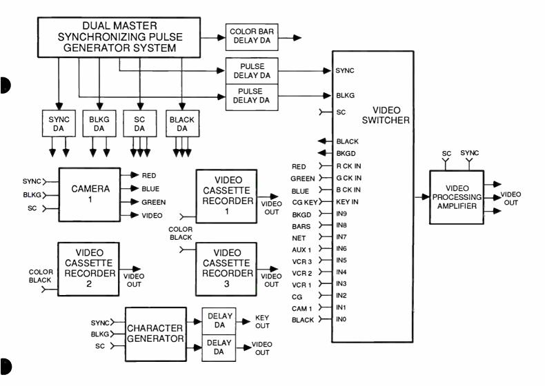
Composite Sync (CS) Horizontal and vertical sync pulses combined. Often referred to simply as "sync". Sync is used by source and monitoring equipment.
