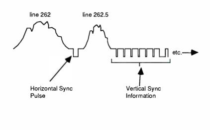
Horizontal Sync Pulse The synchronizing pulse at the end of each line that determines the start of horizontal retrace.
