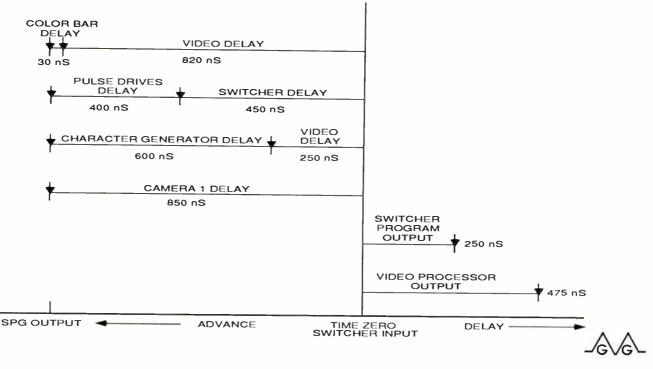
The sync and subcarrier required as external reference inputs for the video processing amplifier should come from the distribution amplifiers feeding the switcher. The video processing amplifier has sufficient timing range for both sync and subcarrier.
