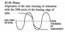
Reference subcarrier is **Positive Going** in Color Field 1 on even lines.
