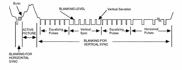
Equalizing Pulses A series of pulses occurring at twice the line frequency before and after the serrated vertical synchronizing pulse. Their purpose is to adjust the scanning sequence for proper interlace.
