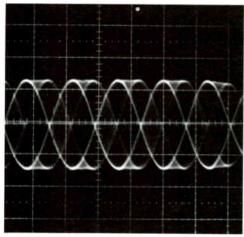
Video time base error is different than sync to subcarrier time base error. Sync to subcarrier time base error is seen when triggering a scope on the leading edge of sync and viewing color burst. What should be seen are two overlapping cycles of subcarrier that are not blurred. An example of sync to subcarrier time base error is shown in the accompanying oscilloscope photos.
