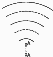
Fig. 11—End view of the vibrating string at A in Fig. 9. As it moves up and down over the distance AA it sends out air waves which carry some of its energy of vibration to the listener's ear
