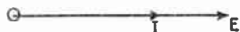
Fig. 50—Vectorial representation of the conditions in the circuit Fig. 43, where the current is in phase with the e.m.f. A convenient convention is to distinguish current vectors by filled-in arrow heads
