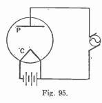
there is no plate current at all. Fleming realized the importance of this fact in that he called his tube a *valve*. This valve action of a diode, which causes it to make a current to flow in only one direction, is extensively used wherever a rectified current is wanted. In order to understand the general principle of the rectifying effect of a diode, we shall consider an alternating e.m.f. connected across the diode, from cathode to plate,
