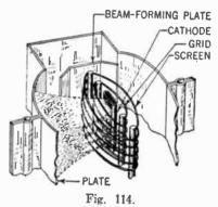
very efficient, since there is so little loss of current in the screen circuit. The tube also has a very high sensitivity, as is shown by the large amount of power it can deliver for a small grid voltage. It is therefore useful where a power tube is required.
