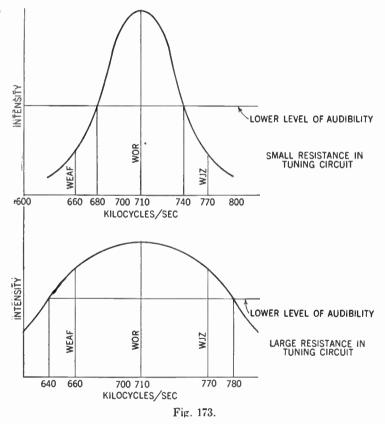
the resonant frequency. These two principles are sometimes combined in an antenna or aerial circuit so as to accept or reject certain frequencies.
