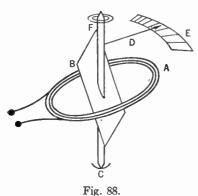
is shown in Fig. 88. A fixed coil, A, is mounted at an angle to the horizontal. At the center of this coil is a soft-iron vane, B, which is in a plane at right angles to the coil. The vane is mounted on a vertical shaft, C, which is free to turn on jeweled bearings. Attached to the shaft is a pointer, D, which moves over a scale, E. When an alternating current is sent through the coil, the vane of soft iron attempts to set itself along the lines of force that were
