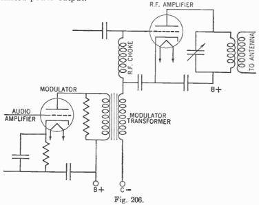
Grid-Bias Modulation.—The circuit for grid-bias modulation is illustrated by Fig. 206. It may be seen that here the primary coil of an audio transformer is connected to the plate of the modulator tube. The secondary coil of this modulator transformer is connected to the grid of the modulated amplifier. A radio-
