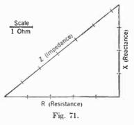
graphically, however, by the use of a diagram. Fig. 71 shows the method of adding a resistance and a reactance in series. The resistance is represented as a horizontal line drawn to scale. In the illustration, the resistance of 5 ohms is represented by a line 5
