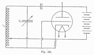
The Hartley Circuit.—Although there are many different oscillator circuits, nevertheless most of them are simply modifications of a few basic circuits. One of these latter, known as the Hartley circuit, is shown in Fig. 161. This is a self-oscillating circuit arranged on the magnetic feedback principle. Comparison of
