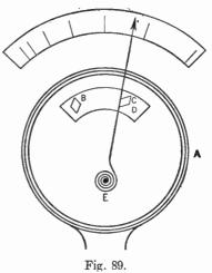
An alternating current flows in a fixed coil, A. Inside the coil are two soft-iron vanes. One vane, B, is fixed; the other, C, is attached
