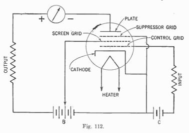
of the tetrode. This effect of secondary emission is overcome by the addition of a fifth element to the tube. The element so added is known as a *suppressor grid*. The tube is then known as a
