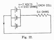
Three storage cells, each having an e.m.f. of 2 volts and an internal resistance of 0.03 ohm, are connected in parallel. A resistance of 0.4 ohm is then connected to this arrangement of cells. Find the current in the 0.4-ohm resistance and the potential across it. The total e.m.f. of all the cells is the same as for one cell; or,
