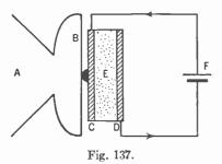
transmitter. A is the mouthpiece; B is a diaphragm; C and D are two polished carbon plates; E indicates loosely packed granules of carbon; F, a cell. The sound wave enters through the mouthpiece. Alternating condensations and rarefactions cause the diaphragm to vibrate back and forth with the same frequency as that of the
