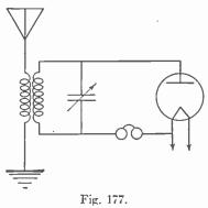
in consequence the detector will not function. Dirt and moisture also may spoil the contact with the crystal. Plainly, the functioning of a crystal is undependable. With the advent of the diode, crystals were replaced by twoelectrode tubes. A receiving circuit using a diode as a detector is shown in Fig. 177. The functioning of a diode as a rectifier has already been explained in the chapter on electronics. (See page 78.) This rectifying action,
