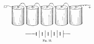
the total e.m.f. would be  $5 \times 1.5$  or 7.5 volts. This rule likewise applies to any other source of potential differences when arranged in series. Thus
