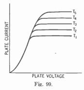
temperature of the cathode is increased, the rate of emission of electrons from the cathode is also increased. This results in a larger saturation, or emission, current. In Fig. 99 you may observe characteristic curves for the same diode, but in this instance the cathode is operated at different temperatures. Each curve is marked with the temperature at which the cathode is to be kept while the plate voltage is being changed.  $T_1$  is the lowest tempera-
