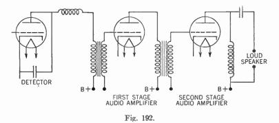
speaker, nevertheless it is also used for coupling the separate stages of the audio-amplifier. The diagram of a circuit that employs transformer coupling in the audio amplifier is shown in Fig. 192. The transformers have their primary coils and secondary coils
