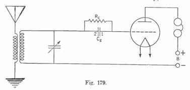
shown in Fig. 179 can be used. A fixed condenser,  $C_g$ , is connected to the grid. When the potential of the tuning circuit is negative, Plate 2 of the grid condenser is negative and electrons are driven
