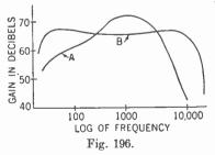
unequal amplification is most pronounced for the very low and very high frequencies. An amplifier that equally amplifies all frequencies over a given range is said to be *flat* over that range. Fig. 196 shows a frequency response curve for an amplifier that suffers from frequency distortion. This curve A is drawn
