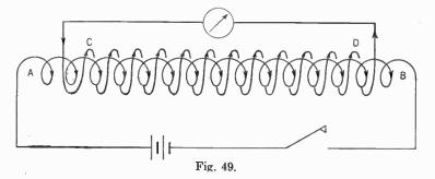
no electrical connection between the two coils. In this case of electromagnetic induction, an e.m.f. is induced in coil CD, due to the change of magnetic flux of the coil AB. It is important to realize that an e.m.f. is induced in CD only when there is a change in the current in AB. If there is a steady current in AB, there is no induction in CD. When the switch is opened, however, there is again a deflection of the galvanometer, but this time it is in the opposite direction.
