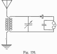
former coupling with the antenna-ground system is employed. The crystal is in series with the earphones. The alternating current from the tuning circuit is changed into a pulsating direct
