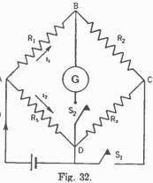
From these facts it follows that the potential difference between A and B must equal the potential difference from A to D. In a similar manner, the potential difference from B to C is the same as that from D to C. We can state this as follows:
