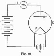
This circuit is called the *plate circuit*, or the *B circuit*. The high positive potential on the plate causes the electrons to move through the evacuated space to the plate. In Fig. 94 the milliammeter measures this plate current. If the plate is made negative,
