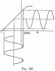
voltage. Fig. 197 shows the resultant of the signal voltage and the potential drop in the grid circuit when the grid is driven positive. In this illustration the distorted output signal is also shown. It is important that any amplifying tube be so operated that the grid will at all times be kept negative under the usual signal conditions.
