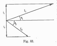
Fig. 82, resonance occurs when the impedance of the combination is a maximum, and the current through the combination is a minimum. This is shown by Fig. 83. Under the conditions of resonance for this circuit, the lagging current in the branch containing inductive reactance is equal to the leading current in the branch containing capacitive reactance.
