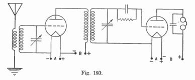
secondary of the antenna coupling. The amplifying circuit is inductively coupled to the detector circuit. Thus the incoming signal is amplified before it is rectified by the detector.
