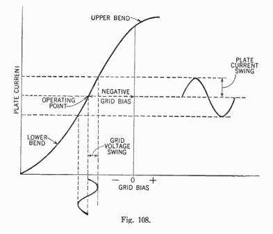
tortion of the signal. It will be observed that the plate-current swing is determined by means of the grid-voltage swing and the slope of the straight portion of the characteristic curve.
