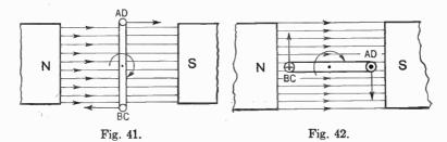
In Fig. 42 the same loop is shown after it has turned through 90°, and wire AD is moving down perpendicularly to the field. Making use of the three-finger rule, we find the e.m.f. directed out of the paper for AD, which we shall indicate by  $\odot$ . In the case of BC, the e.m.f is directed into the paper, and is indicated by  $\oplus$ .
