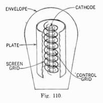
a cutaway section of a tube, which, in addition to the three electrodes (cathode, plate, and grid), has a fourth electrode that consists of a fine spiral, or mesh, of wire between the control grid and the plate. This tube, with its four electrodes, is known as a *tetrode*. The additional electrode of the tube is known as a *screen grid*. Since the latter is placed between the control grid and the plate, it acts as an electrostatic shield
