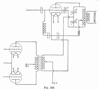
208 shows part of a cathode-modulated transmitting circuit. The audio excitation is introduced into the cathode circuit, and both grid bias and plate voltage vary during modulation. Because part of the modulation is obtained by the grid bias method, the plate efficiency of the modulated amplifier varies during modulation. The higher the percentage of plate modulation, the higher the efficiency of the modulated carrier wave.
