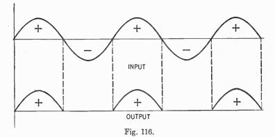
single ordinary type diode can produce only half-wave rectification.
