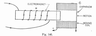
The Dynamic Loud-Speaker.-The dynamic loud-speaker has a moving-coil driving unit, the construction of which is shown by Fig. 146. A direct current flows through the coil of an electromagnet, M. The fluctuating current flows through the coil, C,
