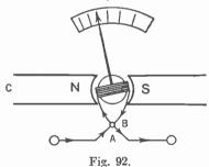
vanometer is connected between B and the cool junction of the thermocouple. A small direct current then flows through the galvanometer, thus causing a deflection of the pointer. Being nonuniform and crowded at the lower readings, the scale is therefore read with great difficulty in this area. Another disadvantage of this form of instrument is the burning-out of the thermocouple. This does not affect the rest of the instrument, however; the thermocouple can readily be replaced at small cost.
