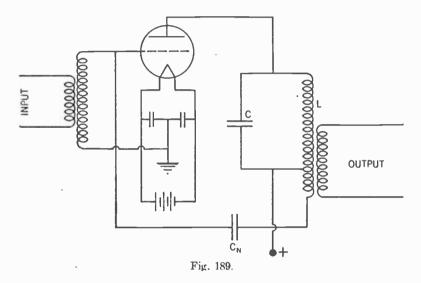
over a small range of frequencies. Many other circuits make use of plate neutralization, but most of them are merely modifications of the circuit shown in Fig. 189.
