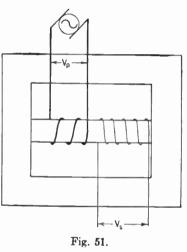
secondary coil. In the diagram, the secondary coil is shown to have more turns than has the primary coil. Such a transformer is known as a *step-up* transformer because the secondary voltage is greater than the primary voltage. If the secondary coil has fewer turns than has the primary coil, it will be a *step-down* transformer. The value of the secondary voltage can be found from the proportion
