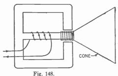
minimum of interference. An alternative method of setting a sufficient amount of air in vibration is by attaching a paper cone to such a driving unit as has just been mentioned.
