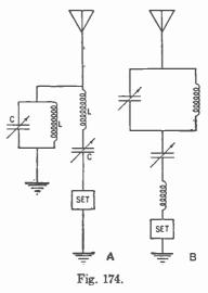
tuning circuit. When the rejector circuit is tuned to a given frequency, a large impedance is offered to the flow of this frequency, but all other frequencies can readily pass. The acceptor circuit works in the usual manner. A circuit of this type is called a *band-stop filter*. This device is used where a particularly strong station interferes with the reception of other stations.
