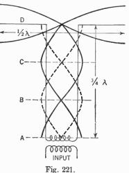
folded back upon itself. The length of such a transmission line may be any integral multiple of a quarter of a wave length. Fig. 221 shows a transmission line of  $\frac{3}{4}\lambda$  feeding into a half-wave antenna. Since the line is in resonance, the impedance is at a minimum. Also, there is no radiated field. Thus transmission loss from transmitter to antenna is greatly reduced.
