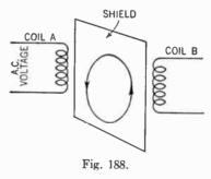
magnetic field. Thus coil B is protected from the influence of the magnetic field set up by the current in coil A. In a receiving set, the coils are either placed in separate metal cases, or certain parts of the circuit are shielded from those parts in which detri-
