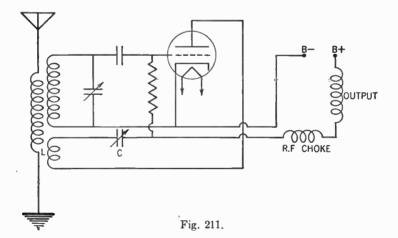
receiver that had high sensitivity. Owners of radios were eager to get stations that, because of their great distance, produced only feeble signals in the antenna ground system. Armstrong supplied the solution to this problem in the circuit shown in Fig. 211. The principal feature of the circuit is the coil, L, which is connected in
