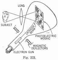
and a lens system. The photoelectric mosaic consists of a screen that is made up of a great number of microscopic photoelectric elements. By means of the lens, the subject (or picture) is focused upon the surface of the mosaic. Light falling upon the minute photoelectric cells causes electrons to be emitted by the photoelectric effect. Since the light over the mosaic varies according to the light that comes from different parts of the subject, the number of electrons
