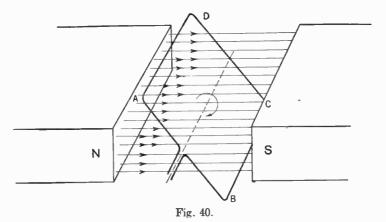
that picture their cross sections, since the wires are perpendicular to the paper. In Fig. 41 the loop is shown in a vertical position, and we observe that both AD and BC are moving parallel to the lines of force, and that the angle  $\theta$ , which we used in the formula, is 0. Hence the induced e.m.f. is 0 for this position of the loop.
