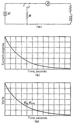
FIG. 2-64.—Characteristics of current and voltage vs time. (a) The circuit, (b) current vs time characteristics with switch in position 2, (c) voltage vs time characteristics with switch in position 2.
