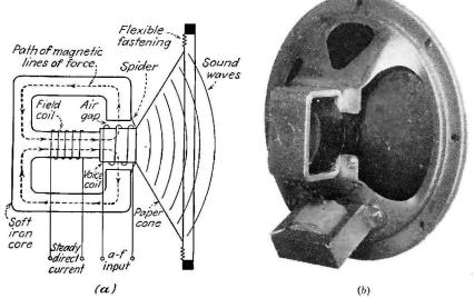
FIG. 12-13.—An electrodynamic loudpseaker. (a) Basic construction, (b) commercial loudspeaker. (Photograph courtesy of Jensen Radio Manufacturing Company.)
