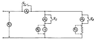
FIG. 15-1.-Correct method of connecting ammeters and voltmeters.
