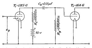
$$\begin{split} T_{1}-\mu = & 65, r_{p} = 240,000 \, \Omega, \ C_{gp} = 1 \, \mu \mu f, \ C_{gk} = 1.1 \, \mu \mu f, \ C_{pk} = 5.8 \, \mu \mu f \\ T_{2}-\mu = & 8.8, r_{p} = 10,700 \, \Omega, \ C_{gp} = 2.8 \, \mu \mu f, \ C_{gk} = 2.2 \, \mu \mu f, \ C_{pk} = 3.4 \, \mu \mu f \\ C_{w} = & 5 tray \ capacitance \ of wiring, etc. = 5 \, \mu \mu f \\ F_{10}, \ 8-29. \end{split}$$
