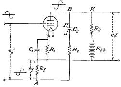
FIG. 8-19.- - A voltage-controlled negative feedback circuit.
