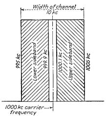
FIG. 13-3.—Illustration of the side bands and the channel width for a 1000-kc carrier wave that is being amplitude-modulated by audio frequencies ranging from 100 to 5000 cycles.
