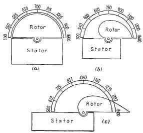
FIG. 6-3.—Frequency distribution obtained with three types of variable capacitors (a) Straight-line-capacity, (b) straight-line-wavelength, (c) straight-line-frequency.
