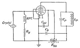
FIG. 10-19 .-- A crystal oscillator circuit using a pentode.
