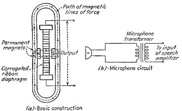
FIG. 12-10.- A velocity microphone and its circuit.
