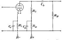
FIG. 8-26.—A simple plate decoupling circuit.
