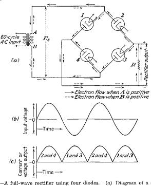
FIG. 11 7.—A full-wave rectifier using four diodes. (a) Diagram of a simple bridge-type rectif r circuit, (b) wave form of the input voltage, (c) wave form of the output current or voltage
