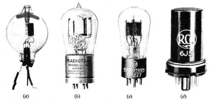
FIG. 4-23.—Development of triodes. (a) Early DeForest three-element tube, (b) early triode of the type UV-200, (c) early triode using an indirectly heated cathode, (d) modern triode with an indirectly heated cathode and metal tube construction. (Courtesy of RCA Manufacturing Co., Inc.)
