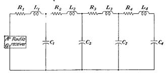
FIG. 3-6. -Electrical characteristics of the antenna circuit.
