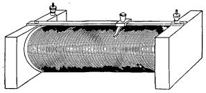
FIG. 3-10,-A slide-wire tuning coil.
