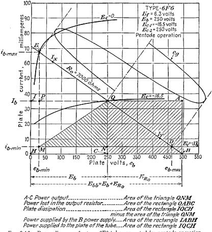
FIG. 9-16.—Power diagram of a type 6F6 tube connected for pentode operation.
