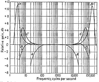
FIG. 8-23.—Relative gain vs frequency characteristics of a two-stage resistance-capacitance-coupled a-f amplifier with various amounts of feedback. Curve A, amplifier without feedback. Curve B,  $A\beta$  equal to -2 at mid-frequency. Curve C,  $A\beta$  equal to -10 at mid-frequency. Curve D,  $A\beta$  equal to -50 at mid-frequency.
