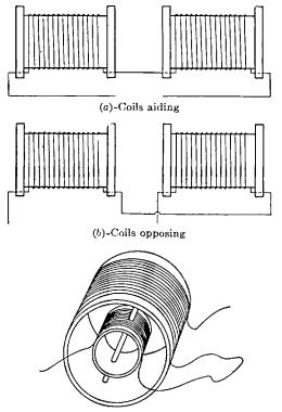
(c)-Variable coupling FIG. 2-9.—Two coupled inductors connected in series.
