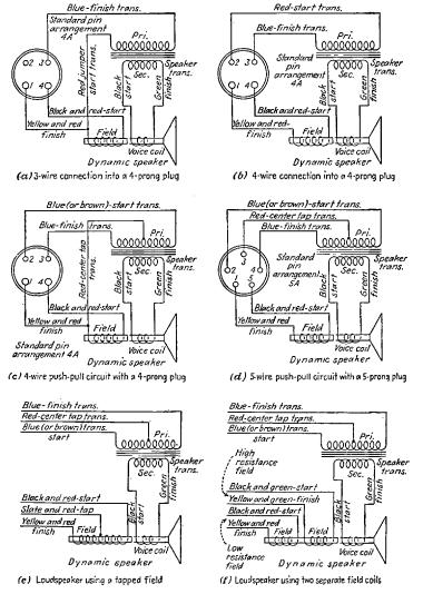
F1G. A-4.—Identification of electrodynamic loudspeaker leads. (Courtesy of P. R. Mallory & Co., Inc.)
