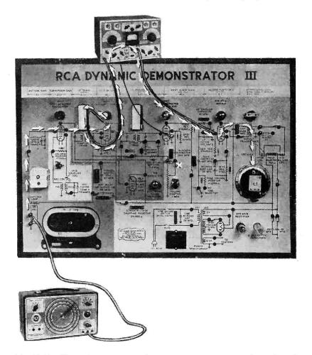
FIG. 15-30.—Illustration of signal-tracing technique. The arrows indicate the path of the signal from the antenna through the RCA Chanalyst to the loudspeaker, thus bridging the artificial defect at point *x*. (Courtesy of RCA Manufacturing Co., Inc.)
