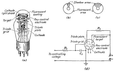
FIG. 14-15.—The tuning indicator. (a) Construction of the electron-ray tube, (b) indication when the receiver is properly tuned, (c) indication when the receiver is improperly tuned, (d) circuit connections. (Photograph courtesy of RCA Manufacturing Co., Inc.)
