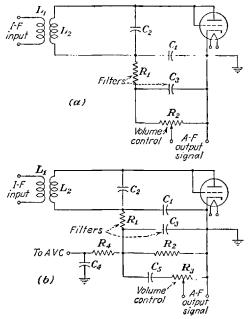
Fig. 5-6.—Diode-detector circuits. (a) Diode circuit with filter, (b) diode circuit with provision for obtaining voltage for automatic-volume-control.
