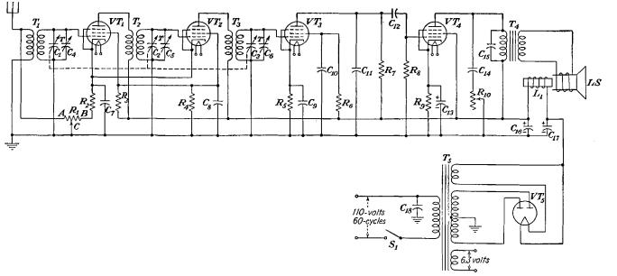
FIG. 14-9.—Circuit diagram of a five-tube, a-e operated, trf receiver.
