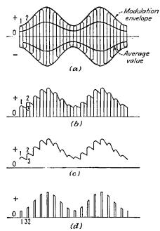
F10. 5-3.—Waveforms illustrating the operation of a diode detector circuit. (a) Modulated input voltage, (b) charging and discharging of the diode capacitor, (c) voltage across the diode capacitor, (d) diode plate current.
