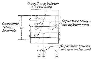
FIG. 2-26.—Distributed capacitances of a coil.
