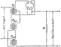
FIG. 11-2.-Circuit showing the connections of a voltage-regulating transformer.
