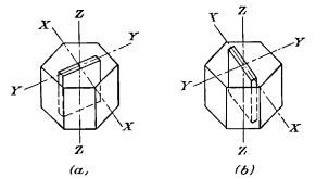
FIG. 10-15.—Methods of cutting a quartz crystal. (a) X-cut, (b) Y-cut.
