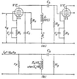
FIG. 7-12.—R-f amplifier circuit using untuned-impedance coupling. (a) Actual circuit, (b) equivalent circuit.
