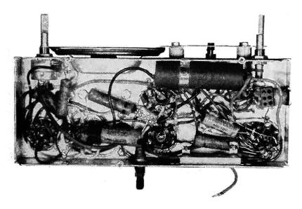
FIG. 14-17.—Bottom view showing the parts used in a radio receiver. (Courtesy of Philco Corporation.)
