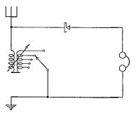
Fig. 3-12.—Circuit diagram of a simple crystal receiver using a variometer having a tapped secondary coil.
