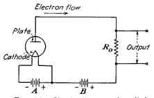
Fig. 4-9.—Circuit diagram of a diode showing the electron flow and the proper connections for the A and B power supplies.
