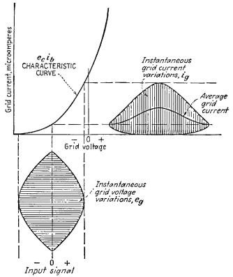
FIG. 5-14.- Grid circuit operating characteristics of a grid-leak detector.
