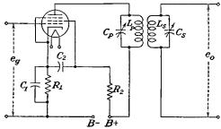
Fig. 7-16.--Typical band-pass amplifier circuit as used for the i-f amplifier in superheterodyne receivers.
