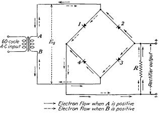
FIG. 11-9.--A full-wave contact-type rectifier bridge circuit.
