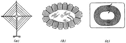
Fig. 3-5.—Three types of loop antennas. (a) Early loop antenna, (b) loop antenna used in modern receivers, (c) loop antenna used in modern receivers.
