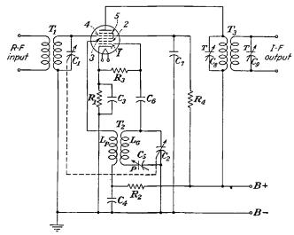
FIG. 14-11.—Frequency converter circuit using a pentagrid converter tube similar to the type 6A8.
