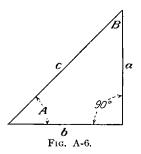
presented in the text makes it possible to solve all such problems by the use of right triangles. The following statements apply to any right triangle and are illustrated in Fig. A-6.
