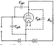
FIG. 4-28.—Interelectrode capacitances of a triode.
