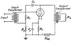
FIG. 9-25.—A voltage-controlled feedback-amplifier circuit as applied to a single-tube power amplifier.
