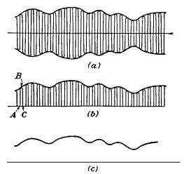
FIG. 3-17.—Waveform of a radio signal at various stages in a receiver. (a) As received by the antenna, (b) rectified current waveform at the detector, (c) a erage current output from the detector.
