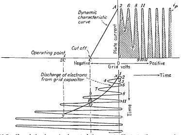
FIG. 10-7.—Use of the dynamic characteristic curve to illustrate the manner in which oscillations are produced.
