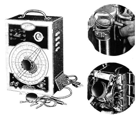
FIG. 15-28. —An L-C Checker and two of its applications. Left, the L-C Checker; upper right, checking the inductance of a coil; lower right, checking the capacitance of a capacitor in a receiver. (Courtesy of Aerovox Corporation.)
