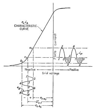
FIG. 7-4.—Distortion in a Class A operated voltage amplifier tube caused by using too large a bias.
