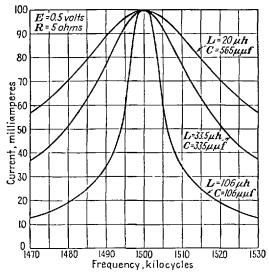
Fig. 2-42.—Resonance curves of a series tuned circuit showing the effect of the LC ratio on the slope of the curve.
