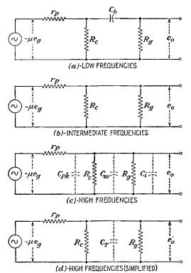
FIG. 8-6.—Equivalent electrical circuits at various audio frequencies for a resistancecapacitance-coupled amplifier circuit using triodes.
