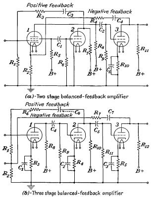
FIG. 8-25.---Several methods of obtaining balanced feedback.
