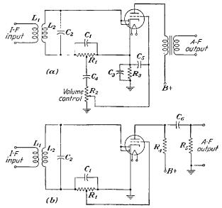
FIG. 5-7. Diode-detector circuits using duplex-diode-triodes. (a) Using cathode bias (resistor  $R_3$ ) for triode section, (b) using diode bias (portion of the diode load resistor  $R_1$ ) for the triode section of the tube.
