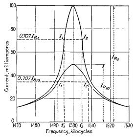
Fig. 2-41.—Resonance curves with the width of the band  $(f_2 - f_1)$  indicated.
