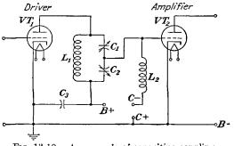
FIG. 13-12 .- An example of capacitive coupling.
