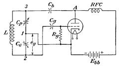
FIG. 10-10.-The Colpitts oscillator circuit.
