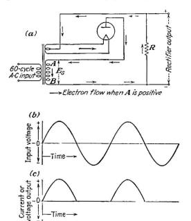
Fig. 11-5.—A half-wave diode rectifier. (a) The circuit, (b) wave form of the input voltage, (c) wave form of the output current or voltage.
