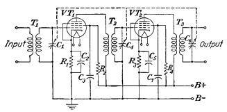
FIG. 7-24.- A two-stage tuned transformer-coupled r-f amplifier circuit.
