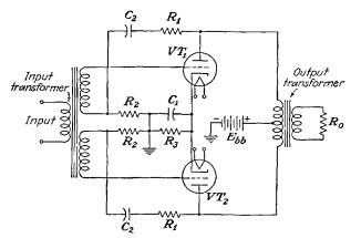
FIG. 9-26.- A push-pull amplifier circuit with voltage-controlled feedback.
