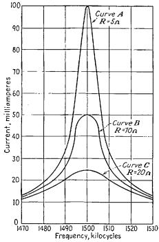
FIG. 3-14. Curves showing the effect of resistance upon the tuning circuit.
