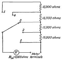
FIG. 15-3.—Circuit showing the application of a rotary switch and resistors to increase the voltmeter range by multiples of 2, 3, 4, or 5.
