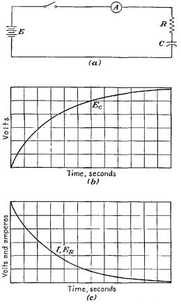
FIG. 2-65.—Characteristics of current and voltage vs time for a circuit containing resistance and capacitance. (a) The circuit, (b) capacitor volts vs time characteristics, (c) current and resistance volts vs time characteristics.
