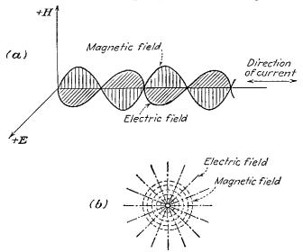
Fig. 13-24.—Illustration of the relations among the electric field, magnetic field, and the direction of current. (a) Viewed along the conductor, (b) end view.
