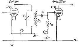
FIG. 13-13 .--- An example of impedance coupling.
