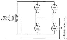
FIG. 11-16.—Parallel operation of two full-wave rectifiers.
