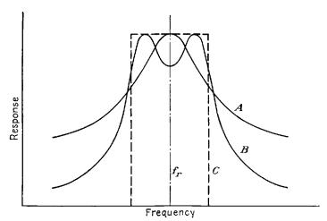
FIG. 7-15.—Response curves of typical amplifier circuits. Curve A, amplifier with a single tuned circuit. Curve B, amplifier with two tuned circuits that are tightly coupled. Curve C, the ideal response curve.
