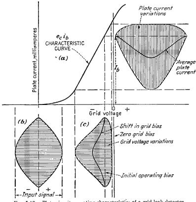
FIG. 5-13.—Plate circuit operating characteristics of a grid-leak detector.
