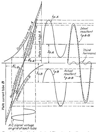
FIG. 9-21.-Graphical analysis of Class A push-pull operation.
