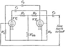
FIG. 15-23.-A simple multivibrator circuit.
