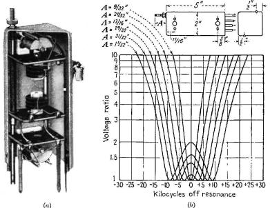
FIG. 7-17.—Illustration of variable coupling used for an i-f stage. (a) A variable roupling i-f transformer, (b) effect of various coupling values on the transmission characteristics of a single transformer as shown in (a). (Courtesy of Hammarlund Manufacturing Company, Inc.)
