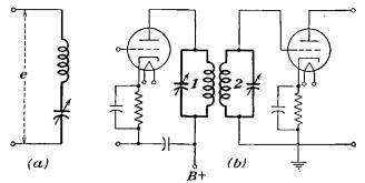
Fig. 2-35.—Typical resonant circuits. (a) Series resonant circuit, (b) 1-parallel resonant circuit 2- series resonant circuit.
