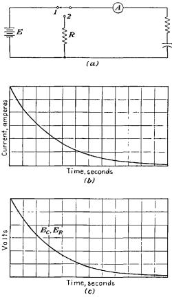
F10. 2-66.—Characteristics of current and voltage vs time. (a) The circuit, (b) current vs time characteristics with switch in position 2, (c) voltage vs time characteristics with switch in position 2.
