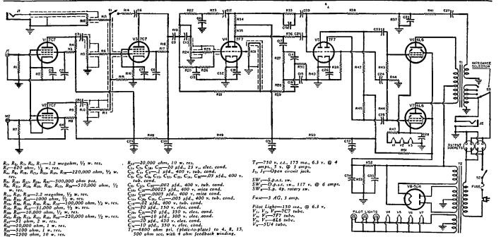
FIG. 9-11.—Circuit diagram of the audio-frequency power amplifier shown in Fig. 9-10. (Courtesy of Radio News.)
