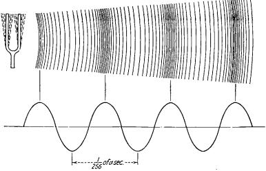
FIG. 1-8.—Propagation of sound waves.
