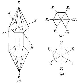
FIG. 10-14.—Quartz-crystal axes. (a) Symmetrical quartz crystal, (b) electrical axes, (c) mechanical axes.
