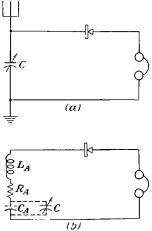
Fig. 3-13.— A simple crystal receiver circuit using a variable capacitor for tuning. (a) The circuit diagram, (b) the equivalent circuit.
