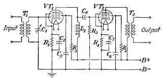
FIG. 7-25.—An r-f amplifier circuit using both impedance coupling and transformer coupling.
