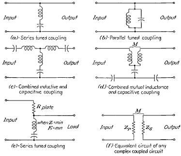
FIG. 2-54.—Typical complex-coupled circuits.
