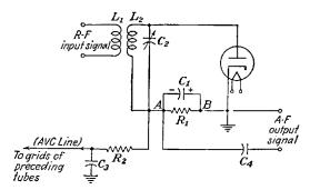
FIG. 5-21.-Diode detector with simple automatic voulme control.
