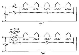
FIG. 4-6.—Methods of using a series dropping resistor in order to operate the heaters directly from a 110-volt line. (a) With a fixed resistor, (b) with an automatic ballast-regulating resistor.
