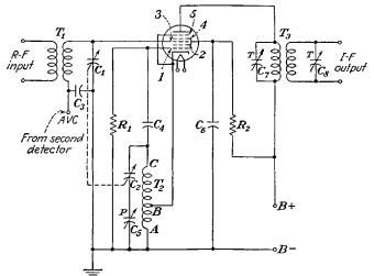
Fig. 14-12.—Frequency converter circuit using a pentagrid converter tube similar to the type 6SA7.
