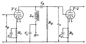
FIG. 8-9,-Impedance-coupled amplifier circuit using triodes.
