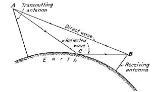
FIG. 13-42.-Direct and reflected waves at ultrahigh frequencies.
