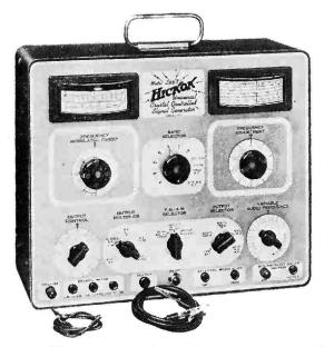
Ftg. 15-16.—A commercial universal crystal-controlled signal generator. (Courtesy of The Hickok Electrical Instrument Company.)
