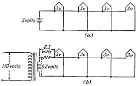
Fig. 4-4.—Circuits with heaters (or directly heated cathodes) connected in parallel. (a) Voltage of the heaters equal to the voltage of the power supply, (b) using a dropping resistor to compensate for the difference in power supply and heater voltages.
