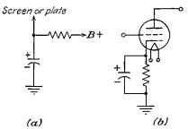
FIG. 2-52. —Resistor-capacitor filter circuits. (a) Filter action in the plate or screen-grid circuit, (b) cathode bias circuit.
