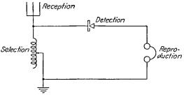
FIG. 3-2.--Schematic diagram of a simple crystal receiver.
