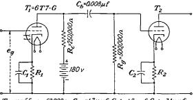
$T_{I} - \mu = 65, r_{P} = 62,000 n, C_{gP} = 1.7 \mu\mu f, C_{gk} = 1.8 \mu\mu f, C_{Pk} = 3.1 \mu\mu f$   $T_{2} - \mu = 120, C_{gP} = 1 \mu\mu f, C_{gk} = 3.5 \mu\mu f, C_{Pk} = 7.5 \mu\mu f$  $C_{uu} = Stray capacitance of wiring, etc. = 10 \mu\mu f$
