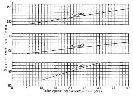
Fig. 11-31.—Operating characteristics of typical voltage-regulating tubes.
