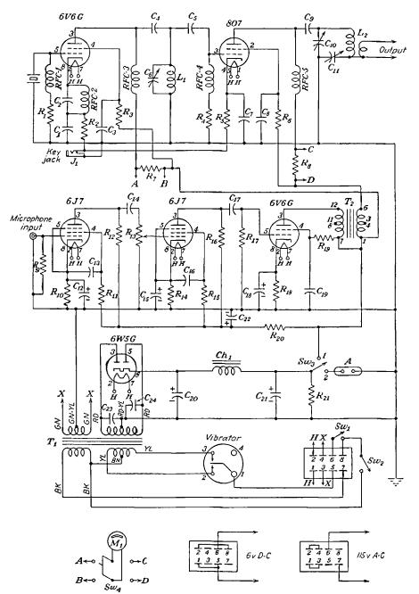
FIG. 13-16.—Circuit diagram of the transmitter illustrated in Fig. 13-15. (Courlesy of Thordarson Electric Manufacturing Division, Maguire Industries, Inc.)
