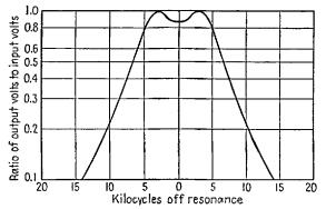
FIG. 7-18.—Curve showing variation of the ratio of output volts to input volts with changes in frequency.
