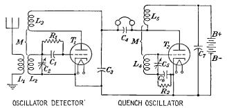
FIG. 5-20.—Separately quenched superregenerative detector circuit.
