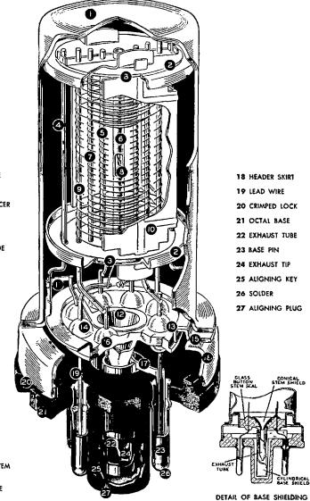
FIG. 4-26.—Structure of a single-ended metal tube. (Courtesy of RCA Manufacturing Co., Inc.)
