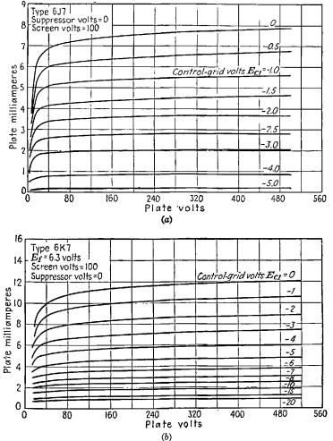
FIG. 4-31.—Family of plate characteristic curves for a pentode. (a) Type 6J7 tube with uniformly spaced grid, (b) type 6K7 tube with supercontrol grid.
