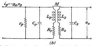
FIG. 7-20.-Single-stage i-f amplifier. (a) Actual circuit, (b) equivalent circuit.
