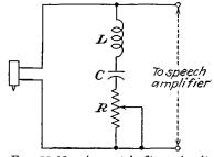
FIG. 12-19 .--- A scratch filter circuit.
