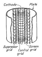
FIG. 4-33.—Cross-section view showing the construction of the electrodes of a supercontrol amplifier tube.
