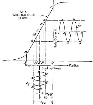
FIG. 7-2.—Operating characteristics of a voltage amplifier tube operated Class A.
