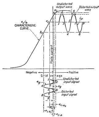
FIG. 7-7.—Distortion in a Class A voltage amplifier tube when operated with incorrect grid bias so that the grid is driven positive during part of each cycle.
