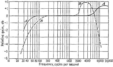
Fig. 8-16.—Relative gain vs frequency characteristics for a transformer-coupled audio-frequency amplifier. Curve A is for a circuit using a high-grade transformer, curve B is for a circuit using a low-grade transformer.
