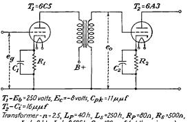
$L_{p}^{\prime}=0.1 h, L_{s}^{\prime}=0.625h, C_{p}^{\prime}=0.0\mu\mu f (at the primary), C_{p}^{\prime}=0.1 h, L_{s}^{\prime}=0.625h, C_{p}^{\prime}=0.0\mu\mu f (at the primary), Core-loss effect to be considered as negligible.$  $C_{w}^{\prime}=Stray capacitance of wiring, etc.=10 \mu\mu f (at the primary)$ Fig. 8-34.
