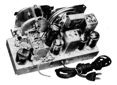
Fig. 14-16.—Top view showing the parts used in a radio receiver. (Courtesy of Philco Corporation.)
