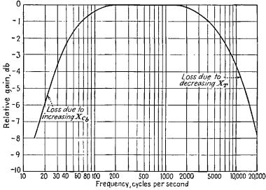
FIG. 8-5.—Relative gain vs frequency characteristics for a typical resistance-capacitancecoupled audio-frequency amplifier.
