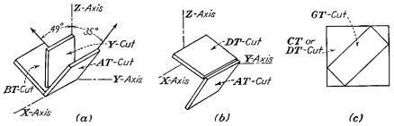
FIG. 10-16.—Crystal cuts having zero temperature coefficient. (a) AT- and BT-cuts (b) DT-cut, (c) GT-cut.
