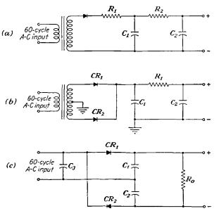
Fig. 11-18.—Several applications of contact rectifiers to rectifier circuits. (a) Half-wave rectifier, (b) full-wave rectifier, (c) voltage doubler.
