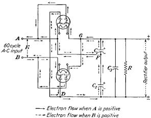
Fig. 11-13.--A full-wave voltage tripler circuit.
