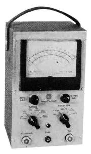
FIG. 15-9.—A Voltohmyst. (Courtesy of RCA Manufacturing Co., Inc.)
