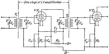
FIG. 7-19.-A single-stage i-f amplifier circuit.
