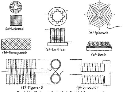
FIG. 2-14.-Various methods of winding high-frequency coils.
