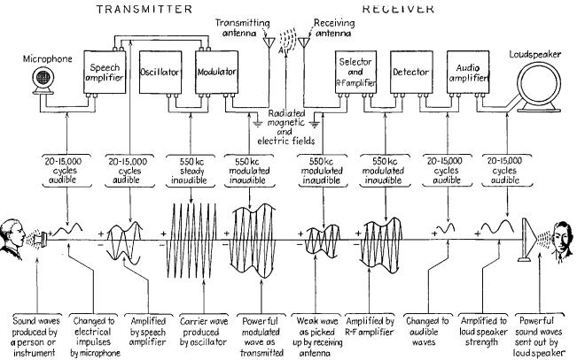
FIG. 1-11.-Radio-broadcasting operations from microphone to loudspeaker.
