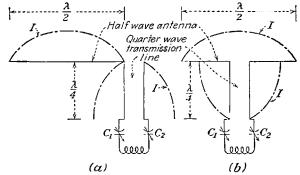
Fig. 13-36.—A half-wave antenna fed by a quarter-wave two-wire line. (a) Voltage-fed, (b) current-fed.
