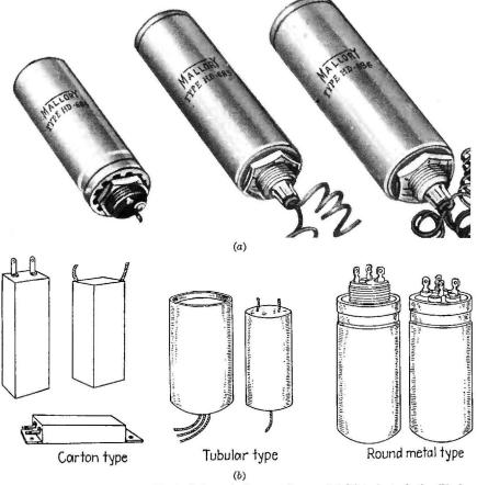
FIG. 2-23.—Typical electrolytic capacitors. (a) Wet electrolytic, (b) dry
