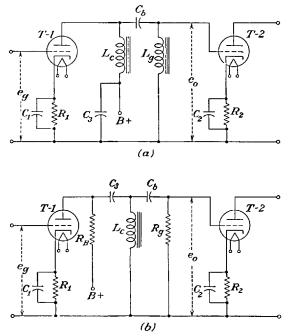
FIG. 8-12.---Applications of impedance-coupled amplifier circuits. (a) Double-impedance-coupled amplifier circuit, (b) impedance-coupled amplifier circuit with parallelplate-feed.
