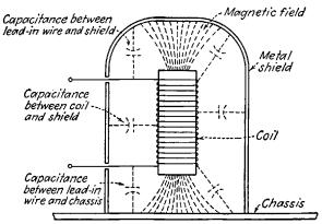
FIG. 7-26.— Illustration of the capacitance between the coil and its lead-in wires and the shield and chassis. The manner in which the magnetic lines from the coil cut the shield and chassis is also shown.
