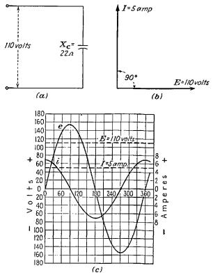
Fig. 2-19.—Methods of illustrating the leading current caused by capacitance. (a) The circuit, (b) vector diagram, (c) sine-wave diagram.
