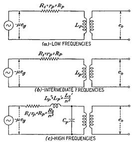
FIG. 8-14...-Simplified equivalent electrical circuits at various audio frequencies for a transformer-coupled amplifier using triodes.
