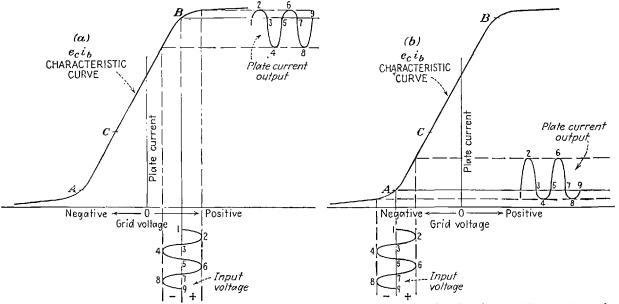
Fig. 5-8.—Operating conditions of a plate-detector circuit. (a) Operation at the upper bend of the  $e_c i_b$  curve, (b) operation at the lower bend of the  $e_c i_b$  curve.
