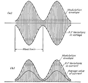
Fig. 5-1.—Detector action. (a) Input signal voltage, (b) current through the detector.
