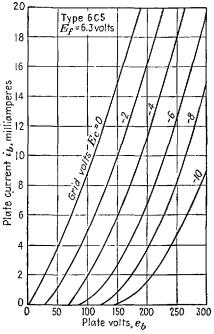
FIG. 4-19,-Plate characteristic curves.
