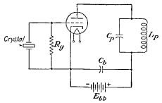
FIG. 10-18.-A simple crystal oscillator circuit.
