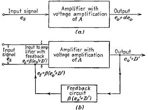
FIG. 8-17.—Block diagrams illustrating the principles of feedback. (a) Amplifier circuit without feedback, (b) amplifier circuit with feedback.
