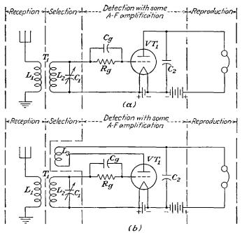
F10. 14-2.—Two single-tube receiver circuits. (a) Simple receiver circuit with a grid-leak detector, (b) simple receiver circuit with a regenerative detector.
