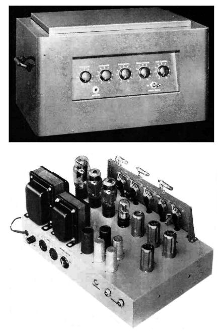
FIG. 9-10.-Commercial audio-frequency power amplifier. (Courtesy of Radio News.)
