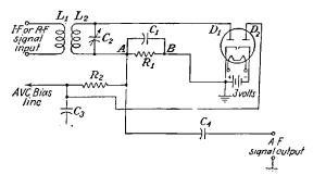
FIG. 5-22.-Diode detector with delayed automatic volume control.
