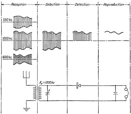
Frg. 3-20.—Diagram of a crystal detector receiving circuit and the type of current flowing through each of its parts.
