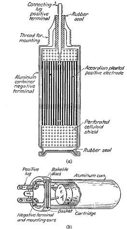
FIG. 2-22.—Cross-section view showing the construction of electrolytic capacitors. (a) Wet electrolytic, (b) dry electrolytic.
