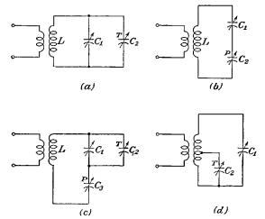
FIG. 6-12.—Trimmer and padder capacitors connected to produce bandspread and bandcompression.
