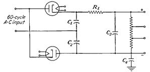
FIG. 11-27.--A transformerless power supply unit employing a voltage doubler rectifier,
