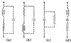
F1G. 2-43.—Equivalent circuits for the three kinds of circuit elements. (a) A resistor, (b) an inductor, (c) a capacitor used on direct current, (d) a capacitor used on alternating current.
