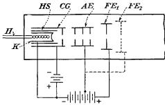
FIG. 15-19.—The electron gun of a cathode-ray tube.
