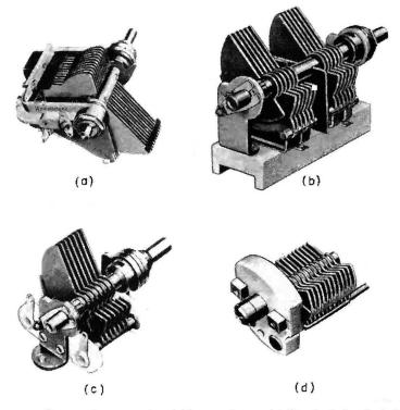
FIG. 2-24.—Commercial types of variable capacitors. (a) Standard-size single broadcast capacitor, (b) midget split-stator capacitor, (c) midget single capacitor, (d) micro capacitor. (Courtesy of Hammarlund Manufacturing Company, Inc.)
