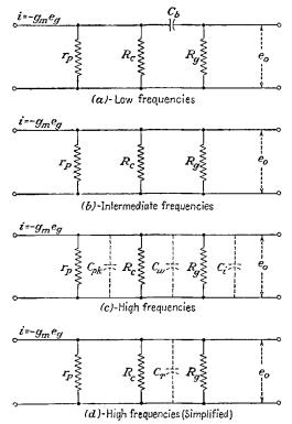
FIG. 8-8.—Equivalent electrical circuits at various audio frequencies for a resistancecapacitance-coupled amplifier circuit using pentodes.
