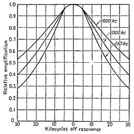
Fig. 14-7.—Curves showing the effect of frequency upon the selectivity of a typical trf amplifier stage.
