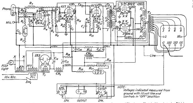
FIG. 12-23.—Circuit diagram of the 15-watt amplifier shown in Fig. 12-22. (Courtesy of Thordarson Electric Manufacturing Division Maguire Industries, Inc.)
