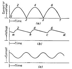
FIG. 11-19.—Filter action of a capacitor and an inductor. (a) Current or voltage output of a full-wave rectifier, (b) output from a capacitor, (c) output from an inductor.
