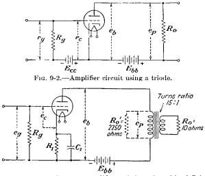
FIG. 9-3.- Triode power amplifier and the reflected load  $R_o'$ .
