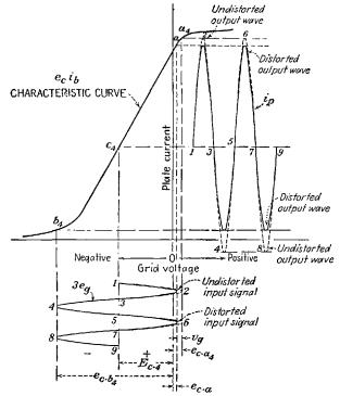
FIG. 7-8.—Distortion in a Class A voltage amplifier tube caused by applying too large an input signal.
