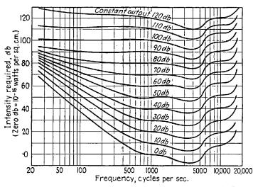
FIG. 8-3.—Curves illustrating how the relative amount of power required to produce a sound of equal intensity varies with the frequency. (Courtesy of Jensen Manufacturing Company.)
