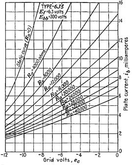
FIG. 9-8.—Dynamic characteristics for a type 6J5 tube.
