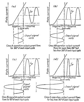
Fig. 7-1.—Curves showing the relation between the current flow in the output circuit and the input signal for various classifications of amplifier operation.
