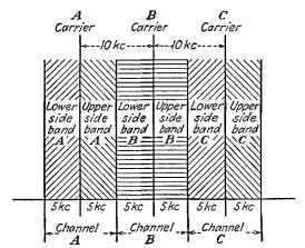
FIG. 6-2.-Relation between carrier wave, side bands, and channels.
