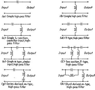
FIG. 2-46.--Typical high-pass filter circuits.
