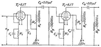
$T_{I}$  and  $T_{2}$ - $g_{m}$ =/225 $\mu$  mhos,  $r_{p}$ =/000000n,  $C_{gp}$ =0.005 $\mu\mu$ f,  $C_{gk}$ =/ $\mu\mu$ f,  $C_{pk}$ =/2 $\mu\mu$ f  $C_{w}$ =Stray capacitance of wiring, etc. = 10 $\mu\mu$ f (at each tube)
