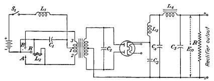
FIG. 11-28.—Circuit diagram of a power supply unit using a nonsynchronous vibrator.
