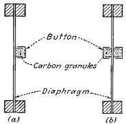
Fig. 12-4.—Basic construction of a carbon microphone. (a) Singlebutton type, (b) double-button type.
