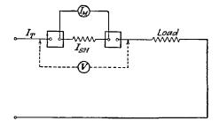
FIG. 15-2.—Proper connections for the use of a shunt with a millivoltmeter.
