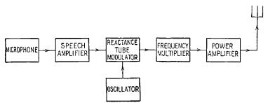
FIG. 13-9.-Block diagram of a frequency-modulated transmitter.
