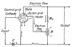
FIG. 4-27.—Circuit diagram for a tetrode showing the electron flow and the proper connection for the screen grid.
