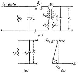
Fig. 7-21.- Band-pass amplifier circuit characteristics. (a) Equivalent circuit, constant-current-generator form, (b) parallel portion of the equivalent circuit, (c) vector relation of the currents and voltages of the circuit shown in (b).
