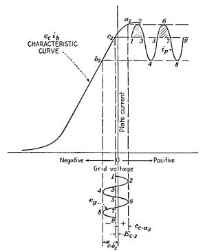
FIG. 7-5.—Distortion in a Class A operated voltage amplifier tube caused by using too small a bias.
