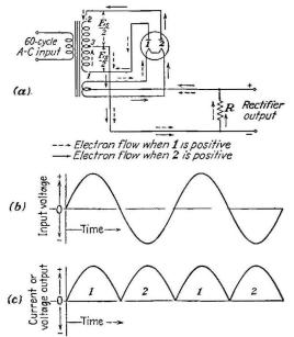
FIG. 11-6.—A full-wave diode rectifier using a center-tapped transformer. (a) The circuit, (b) wave form of the input voltage, (c) wave form of the output current or voltage.
