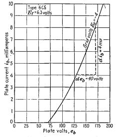
FIG. 4-20.—Method of determining the plate resistance of a tube. This curve is an enlarged segment of Fig. 4-19.
