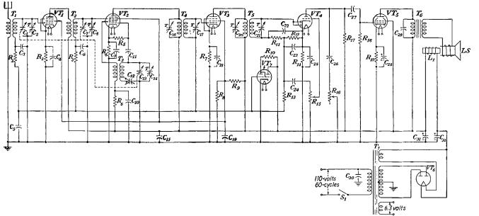
FIG. 14-13.—Circuit diagram of a seven-tube, a-c operated, superheterodyne receiver.
