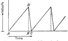
FIG. 15-21.—A saw-tooth linear time base.
