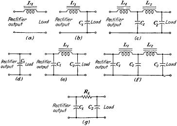
FIG. 11-20.-Types of filter circuits used with rectifiers.
