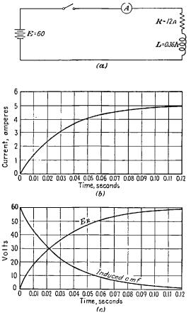
Fig. 2-63.—Characteristics of current and voltage vs time for a circuit containing resistance and inductance. (a) The circuit, (b) current vs time characteristics, (c) voltage vs time characteristics.
