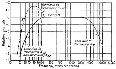
FIG. 8-11. Relative gain vs. frequency characteristics for an impedance-coupled audiofrequency amplifier. Curve A for a simple impedance-coupled circuit (Fig. 8-9), curve B for a circuit with a resonant section (Figs. 8-12a and 8-12b).
