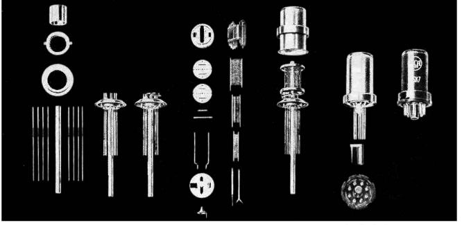
F16. 4-25.-Structural parts of a typical metal tube. (Courtesy of RCA Manufacturing Co., Inc.)
