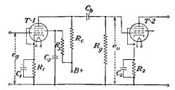
FIG. 8-7.-Resistance-capacitance-coupled amplifier circuit using pentodes.
