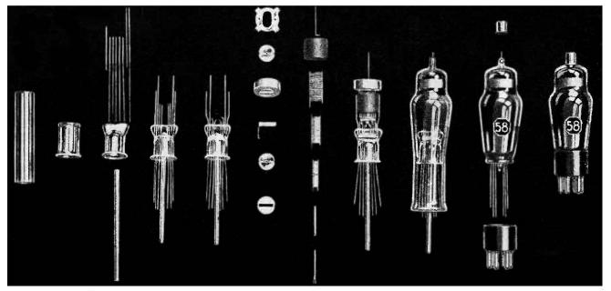
FIG. 4-15.-Structural parts of a typical glass tube. (Courtesy of RCA Manufacturing Co., Inc.)
