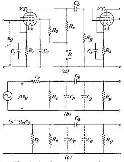
FIG. 7-13.—R-f amplifier circuit using resistance-capacitance coupling. (a) Actual circuit, (b) constant-voltage-generator form of equivalent circuit, (c) constant-current-generator form of equivalent circuit.
