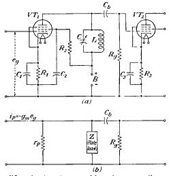
F10. 7-10.—R-f amplifier circuit using tuned-impedance coupling. (a) Actual circuit (b) equivalent circuit.
