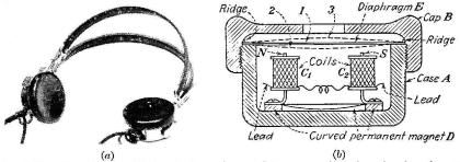
Fig. 3-19.—Earphones. (a) A set of earphones, (b) cross-section view showing the construction of an earphone.
