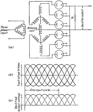
Ftg. 11-15.—A three-phase full-wave rectifier. (a) The circuit, (b) wave-form of the input voltage to tubes, (c) wave form of the rectified output voltage.
