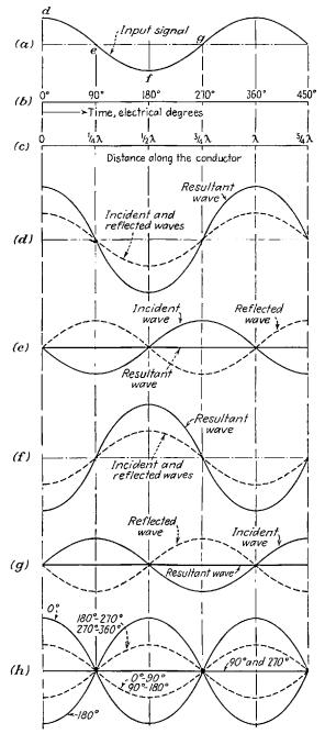
FIG. 13-33.—Curves showing the instantaneous current conditions existing along an openended conductor whose physical length is  $\frac{5}{4}$  the wavelength of the applied current.
