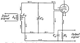
FIG. 5-4.-..Duplex-diode full-wave detector circuit.
