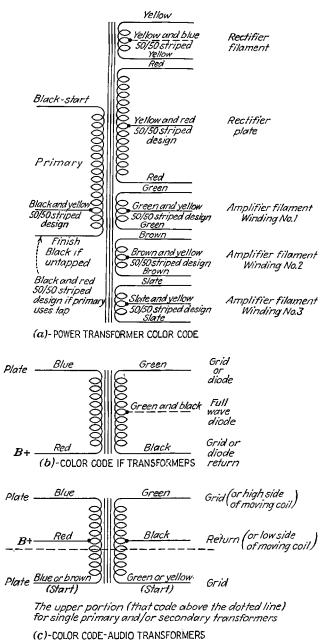
Fig A-5.-Identification of transformer leads. (Courtesy of P. R. Mallory & Co., Inc.)
