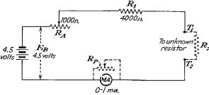
F1G. 15-4.—Circuit of a simple ohmmeter.
