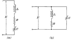
FIG. 2-36.-Equivalent circuits of typical resonant circuits. (a) Series, (b) parallel.
