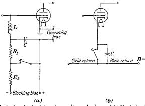
FIG. 13-7.—Methods of obtaining low-voltage keying. (a) Blocked-grid keying, (b) cathode keying.
