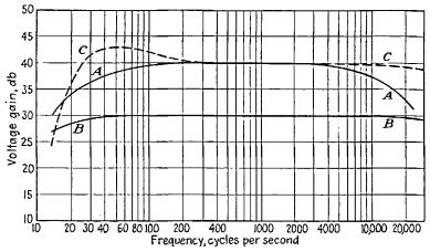
FIG. S-18.—Variation of voltage gain with frequency. Curve A for an amplifier without feedback, curve B for a similar amplifier with negative feedback, curve C for an amplifier with balanced feedback.
