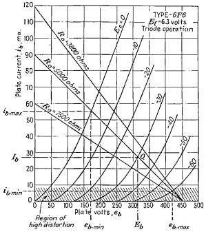
FIG. 9-13.—Distorted output caused by incorrect choice of load line, input signal voltage, or grid bias.
