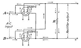
FIG. 11-8,—A full-wave duplex-diode bridge-type rectifier circuit.
