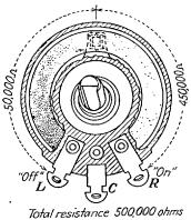
Fig. 2-5.—A carbon-type potentiometer with left-hand taper.
