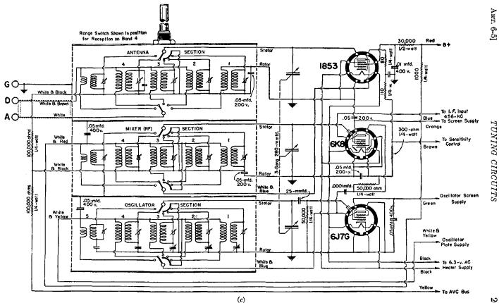
FIG. 6-11.—All-wave tuning unit. (a) The tuning unit, (b) coil assembly, (c) circuit diagram. (Courtesy of Meissner Manufacturing Division Maguire Industries, Inc.)
