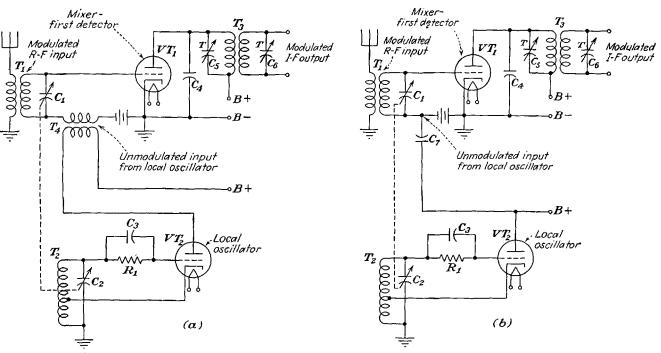
FIG. 14-10.-Simple frequency converter circuits. (a) Oscillator output inductively coupled, (b) oscillator output capacitively coupled.
