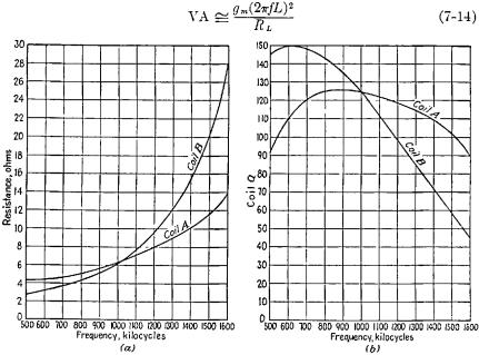
FIG. 7-11.-Effect of frequency on the characteristics of a coil. (a) Variation of coil resistance with frequency, (b) variation of coil Q with frequency.
