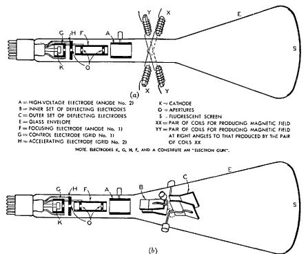
FIG. 15-18.—Schematic arrangement of the electrodes in a cathode-ray tube. (a) Electromagnetic deflection, electrostatic-focus type, (b) electrostatic deflection, electrostatic-focus type. (Courtesy of RCA Manufacturing Co., Inc.)
