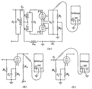
FIG. 15-10.—Methods of connecting the Voltohmyst for making radio circuit measurements. (a) F-m balance, (b) plate voltage, (c) a-f signal voltage.
