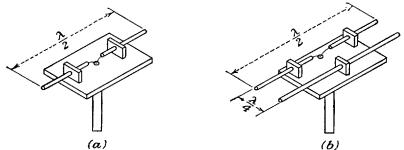
FIG. 14-19.—Antenna system for an f-m receiver. (a) Dipole antenna, (b) dipole antenna and reflector.
