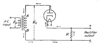
$\rightarrow$  Electron flow when A is positive Fig. 11-3.—A single-diode rectifier circuit.
