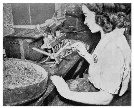
Fig. 1-4.—Photoelectric safety control. The light is reflected across the front and returned to the phototube by means of two mirrors shown in the foreground of the equipment. (Courtesy of RCA Manufacturing Co., Inc.)
