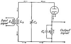
FIG. 5-2.—Simple diode detector circuit.
