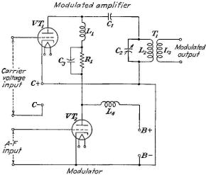
FIG. 13-11.-Basic circuit for obtaining plate modulation.
