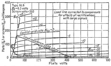
FIG. 4-35.-Family of plate characteristic curves for a beam power tube.
