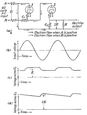
Ftg. 11-11.—A half-wave voltage doubler circuit. (a) The circuit, (b) wave form of the input voltage, (c) wave form of the voltage across  $C_1$ , (d) wave form of the voltage across  $C_2$  or the output voltage.
