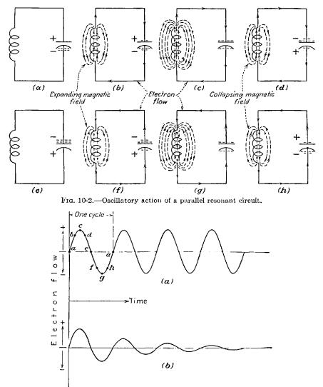
FIG. 10-3.—Flow of electrons in a tank circuit. (a) Theoretical flow, (b) actual flow.
