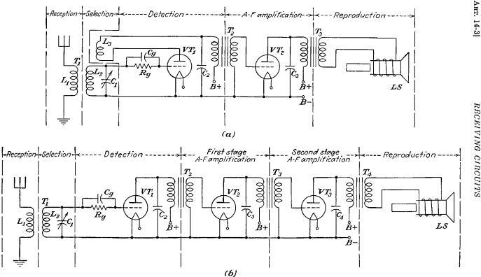
FIG. 14-4.-Two simple receiver circuits with a-f amplification. (a) Regenerative receiver with one stage of a-f amplification, (b) receiver with grid-leak detector and two stages of a-f amplification.
