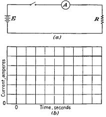
FIG. 2-62.—Characteristics of current vs time for a circuit containing only resistance. (a) The circuit, (b) current vs time characteristics.
