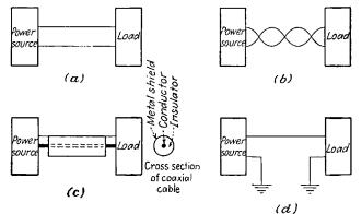
Fro. 13-34.—Four types of transmission lines. (a) Two-conductor open-wire line, (b) twisted-pair line, (c) coaxial line, (d) single-wire system.
