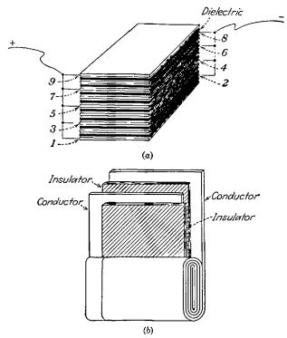
FIG. 2-20.—Typical construction of capacitors. (a) Mica-dielectric capacitors, (b) paperdielectric capacitors.
