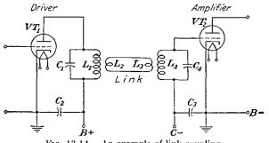
FIG. 13-14.-An example of link coupling.
