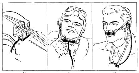
(a) (b) (c) Fig. 12-2.—Contact-type microphones. (a) For musical instruments, (b) throat microphone, (c) lip microphone.
