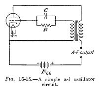
beat-frequency type (see Art. 10-2), (2) the resistance-capacitance type. A simple a-f oscillator circuit of the resistance-capacitance type is shown in Fig. 15-15. The output of this oscillator circuit has a constant amplitude and constant frequency. However, by the proper connection of additional circuit elements to this simple circuit a variable amplitude and variable frequency output can be obtained. The resistance-capacitance type a-f oscil-
