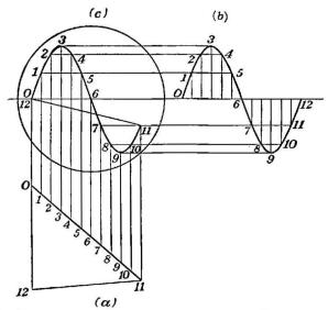
Fig. 15-24.—Pattern produced on the oscilloscope screen when the frequencies of the input voltage and the time base are equal and in phase. (a) Linear time base, (b) sine-wave input voltage, (c) pattern on the oscilloscope screen.
