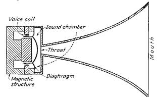
Fig. 12-14.—Basic structure of horn and driver unit. (Courtesy of Jensen Radio Manufacturing Company.)
