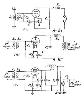
Fig. 5-9.—Plate-detector circuits. (a) Grid bias obtained by use of a C battery, (b) grid bias obtained by use of a cathode resistor, (c) grid bias obtained by use of a cathode resistor.
