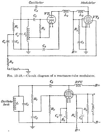
FIG. 13-19.—A reactance-tube modulator circuit using a type 6L7 tube.
