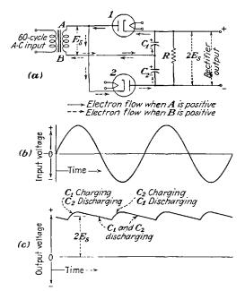
Fig. 11-10. -A full-wave voltage doubler circuit. (a) The circuit, (b) wave form of the input voltage, (c) wave form of the output voltage.
