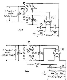
FIG. 14-22.—Discriminator circuits. (a) Split-secondary discriminator circuit, (b) phaseshift discriminator circuit.
