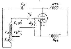
FIG. 10-11.—A modified Colpitts oscillator circuit.
