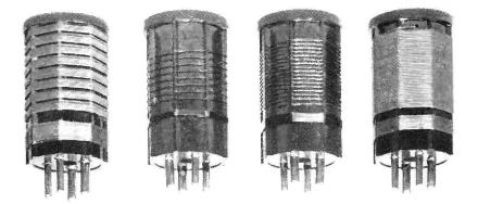
FIG. 6-6.—Set of plug-in coils. (Courtesy of Insuline Corporation of America.)
