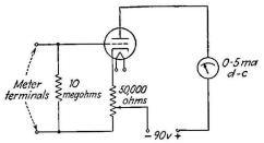
FIG. 15-11 .- A simple vacuum-tube voltmeter circuit.
