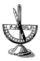
FIG. 5-28.—The dipping needle.
