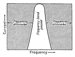
FIG. 12-10.-Characteristic curve for a simple band-pass filter circuit.
