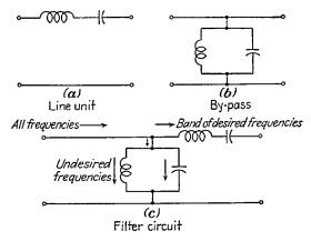
FIG. 12-11.—Basic units of a band-pass filter circuit.
