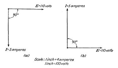
Fig. 10-11.—Vector representation of current and voltage: (a) current lagging the voltage by 90 degrees, (b) current leading the voltage by 90 degrees.
