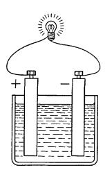
FIG. 3-3.—Simple cell delivering electrical energy to a lamp.
