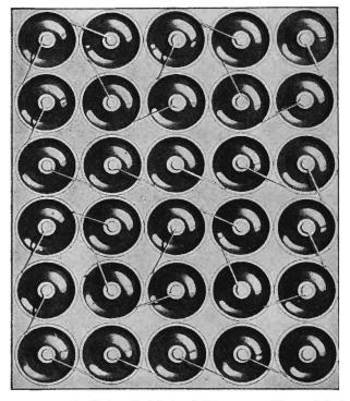
FIG. 3-12.—Arrangement of cells in cylindrical-cell B battery. (National Carbon Company.)
