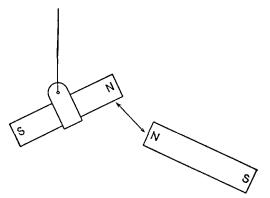
FIG. 5-8.—Repulsion between magnetic poles of like polarity.
