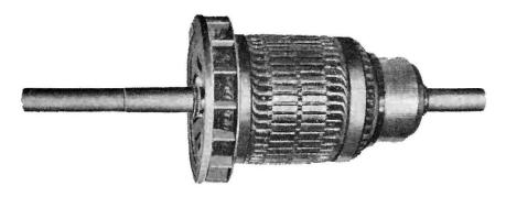
FIG. 7-19.—The armature of a d-c generator. (Westinghouse Electric Corporation.)
