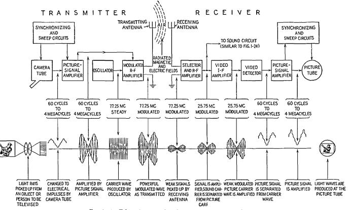
FIG. 1-25 .-- Telecasting operations from camera to picture tube.
