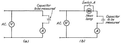
Fig. 9-31.—Impedance method of determining capacitance: (a) voltmeter-ammeter method, (b) voltmeter-ammeter method including a neon lamp to test for a short-circuited capacitor.
