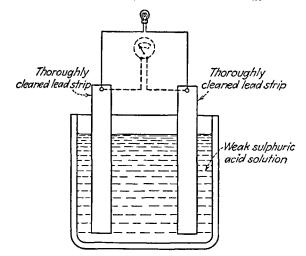
Fig. 3-16.—A simple cell of similar plates. The lamp and voltmeter show that no electrical energy is available.
