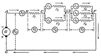
FIG. 4-13.-A series-parallel circuit.
