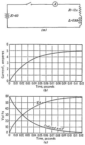
FIG. 12-38.—Characteristics of current and voltage vs. time for a circuit containing resistance and inductance: (a) the circuit, (b) current vs. time characteristics, (c) voltage vs. time characteristics.
