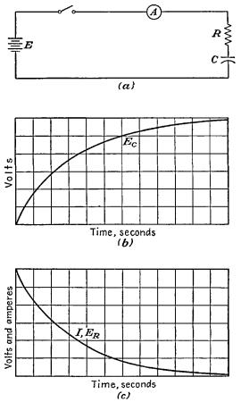
FIG. 12-40.—Characteristics of current and voltage vs. time for a circuit containing resistance and capacitance: (a) the circuit, (b) capacitor volts vs. time characteristics, (c) current and resistance volts vs. time characteristics.
