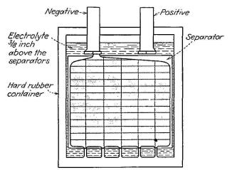
Fig. 3-30.—Cross section of a cell showing the electrolyte at the proper level.
