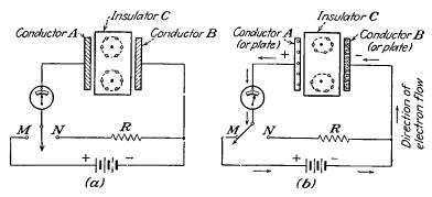
FIG. 9-1.—Principles of capacitor action: (a) capacitor in neutral electron state, (b) a charged capacitor.
