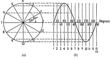
FIG. 7-6.-Wheel-diagram method of drawing a sine-wave voltage.
