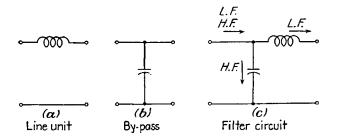
FIG. 12-7.-Basic units of a low-pass filter circuit.
