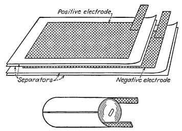
FIG. 9-21.—Construction of a dry-electrolytic capacitor. (P. R. Mallory & Co., Inc.)
