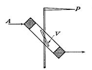
FIG. 6-13.—Essential parts of the Thomson inclined-coil instrument.
