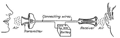
FIG. 1-12.--A simple telephone circuit. (American Telephone and Telegraph Company.)
