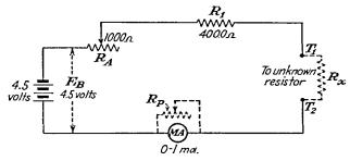
FIG. 6-32.—Circuit of a simple ohmmeter.
