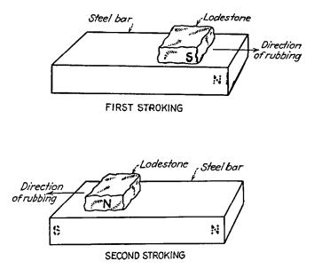
FIG. 5-3.-Making a bar magnet with a lodestone.
