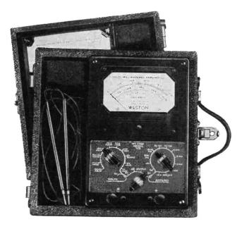
FIG. 6-23.—A combination a-c/d-c volt milliammeter illustrating an application of the complex scale. (Weston Electrical Instrument Corporation.)
