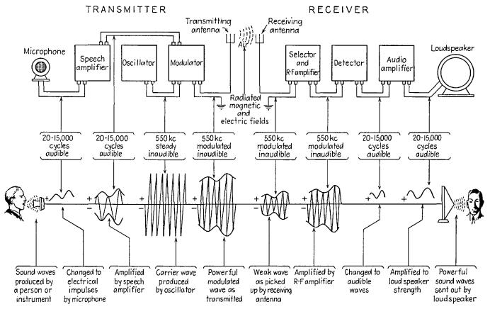
FIG. 1-24.-Radiobroadcasting operations from microphone to loudspeaker.
