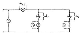
FIG. 6-20.-Correct method of connecting ammeters and voltmeters.
