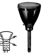
Cathode-ray tube, electromagnetic-deflection type.
