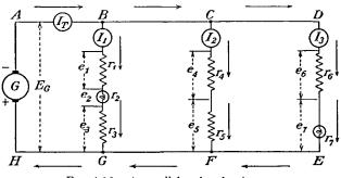
FIG. 4-16.---A parallel-series circuit.
