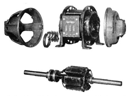
FIG. 7-16.-Disassembled view of an a-c generator. (General Electric Company.)
