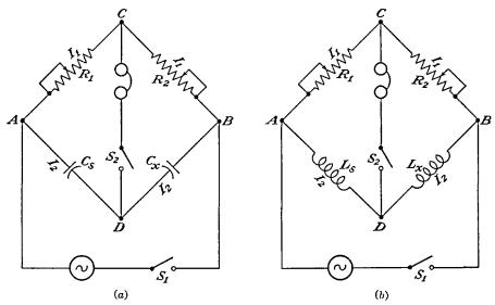
FIG. 6-38.—Basic a-c bridge circuits: (a) for capacitance measurements, (b) for inductance measurements.
