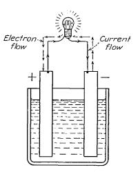
FIG. 3-4.—Electron flow vs. current flow.
