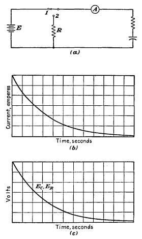
FIG. 12-41.—Characteristics of current and voltage vs. time: (a) the circuit, (b) current vs. time characteristics with the switch in position 2, (c) voltage vs. time characteristics with the switch in position 2.
