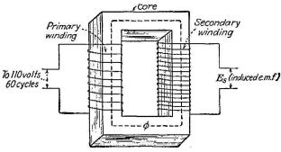
FIG. 7-21.-A fundamental transformer.
