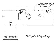
FIG. 9-32.—Impedance method of determining capacitance using a wattmeter, a voltmeter, and an ammeter.
