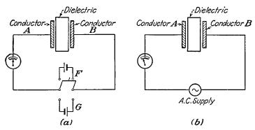
FIG. 9-2.—Effect of reversing the polarity at the terminals of a capacitor: (a) reversals produced by means of a switch, (b) reversals produced by connecting the capacitor to an a-c power supply.
