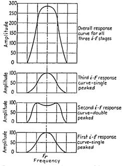
FIG. 12-34.—Wide pass band for the i-f response tance combination. These curcurve in an f-m receiver obtained by use of an cuits are generally referred to as over-coupled i-f transformer.  $B_{c}L$  and  $B_{c}C$  circuits
