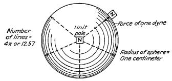
FIG. 5-16.-Magnetic field of a unit pole in a sphere two centimeters in diameter.
