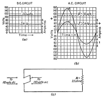
FIG. 10-1.—Direct current vs. alternating current characteristics: (a) current and voltage when the circuit is connected to a d-c power supply, (b) current and voltage when the circuit is connected to an a-c power supply, (c) the circuit diagram.
