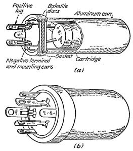
FIG. 9-22.—Construction of a fabricated-type dry-electrolytic capacitor: (a) Internal construction, (b) complete capacitor. (P. R. Mallory & Co., Inc.)
