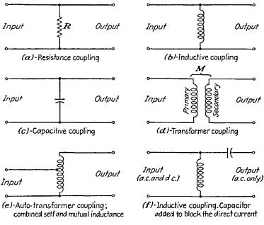
FIG. 12-23.-Types of simple-coupled circuits.
