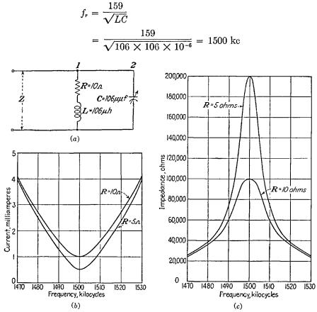
FIG. 11-8.—Parallel resonance: (a) a parallel resonant circuit, (b) current resonance curves (c) impedance resonance curves.
