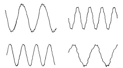
FIG. 7-7.-Several nonsinusoidal voltage waves recorded with the use of an oscillograph.
