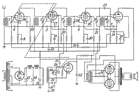
FIG. 9-33.—Circuit diagram of a typical superheterodyne receiver with its capacitors indicated by numbers.
