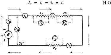
FIG. 4-6.-A series circuit.
