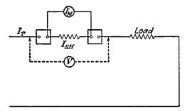
FIG. 6-25.—Proper connections for use of a shunt with a millivoltmeter.
