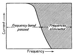
FIG. 12-6.—Characteristic curve for a simple lowpass filter circuit.
