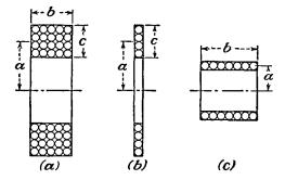
FIG. 8-5.—Types of inductance coils: (a) multilayer, (b) flat or pancake, (c) solenoid.
