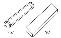
FIG. 8-17.—Conductors used for highfrequency currents: (a) hollow conductor, (b) flat-strip conductor.
