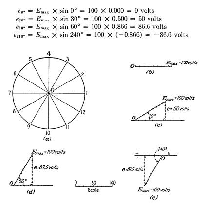
FIG. 10-9.—Vector representation of the wheel diagram: (a) the wheel diagram showing 12 equally spaced points, (b) vector representing point 1, (c) vector representing point 2. (d) vector representing point 3, (e) vector representing point 9.
