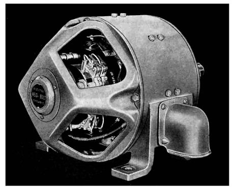
FIG. 7-20.-A d-c generator. (Electro Dynamic Works.)
