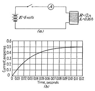
FIG. 8-7.—Time required for the current to build up in a circuit containing resistance and inductance: (a) the circuit diagram, (b) a graph showing the relation between current and time.
