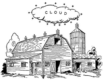
FIG. 2-8.—Application of the lightning rod.
