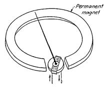
FIG. 5-23.—Ring magnet used in a meter.
