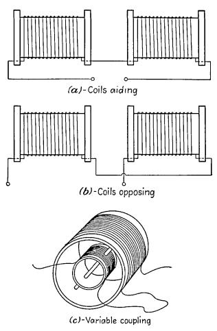
FIG. 8-10.-Two coupled inductors connected in series.
