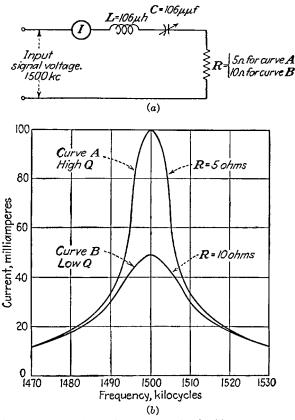
FIG. 11-4.—Series resonance: (a) a series resonant circuit, (b) resonance curves of the circuit shown in (a).
