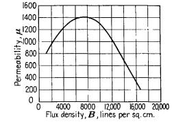
FIG. 5-36.—Permeability curve for cast steel.
