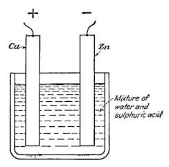
FIG. 3-2.—Simple voltaic cell.
