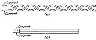
FIG. 8-20.—Noninductive wiring: (a) wires twisted to reduce the inductance, (b) wires placed parallel to one another to reduce the inductance.
