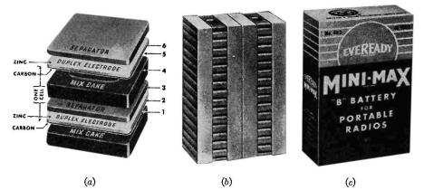
FIG. 3-14.—A miniature B battery: (a) arrangement of the parts of a cell, (b) 30 cells assembled in two stacks of 15 each, (c) the completed battery. (National Carbon Company.)
