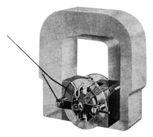
FIG. 6-8.—Mechanism of a commercial permanent-magnet moving-coil meter. (Weston Electrical Instrument Corporation.)
