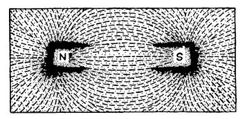
FIG. 5-11.-Magnetic field about a bar magnet illustrated by iron filings.
