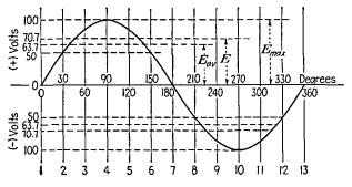
FIG. 7-8.—Relative values of an a-c sine-wave voltage.
