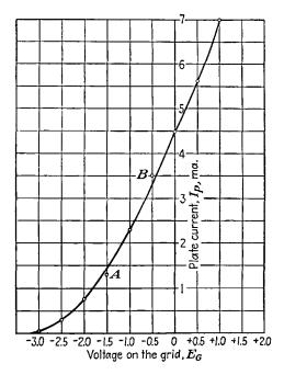
FIG. 11-3.—Curve showing the variation in the plate current of a tube with changes in the grid voltage. Commonly called an  $E_G I_P$  curve.
