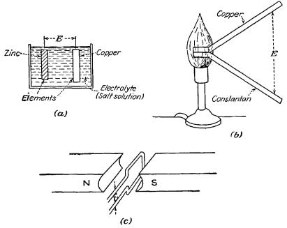
FIG. 2-13.—Three methods of obtaining an electric current: (a) chemical, (b) thermal, (c) magnetic.
