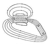
FIG. 5-14.—Path taken by magnetic lines when a magnetic substance is near the magnet.
