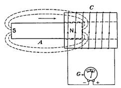
FIG. 7-3.—Electromotive force induced by magnetic lines cutting a conductor.
