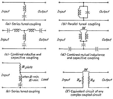
FIG. 12-24.-Typical complex coupled circuits.
