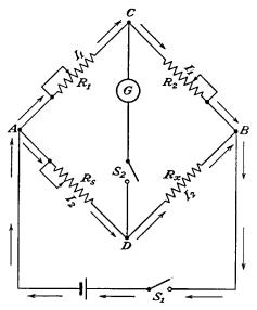
FIG. 6-37.—Wheatstone bridge method of measuring resistance.
