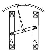
FIG. 6-16.—Essential parts of the dynamometer-type instrument.
