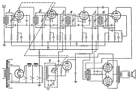
FIG. 11-14—Schematic diagram of a typical superheterodyne receiver with its resonant circuits indicated by heavy-line boxes.
