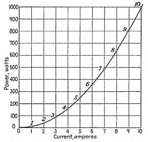
FIG. 11-2.—Curve showing the variation of power with current in a circuit whose resistance is 10 ohms.
