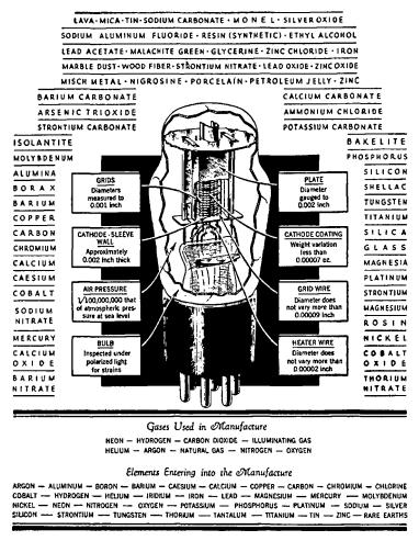
FIG. 2-1.—Materials used in the construction of radio tubes. (RCA Manufacturing Co., Inc.)
