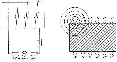
FIG. 8-1.—Alternating current flowing in a coil.
