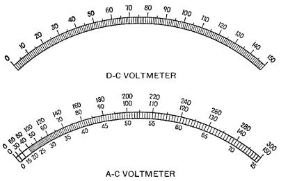
FIG. 6-22.—Meter scales: top, uniform scale; bottom, irregular scale.
