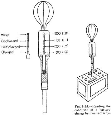
FIG. 3-24.-The hydrometer.
