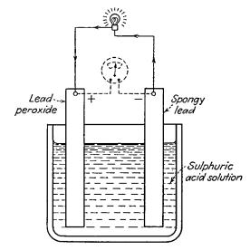
FIG. 3-18.—A simple cell delivering electrical energy to a lamp.
