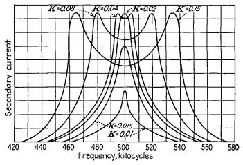
FIG. 12-30.—Curves showing the variation in secondary current with frequency for a bandpass circuit.
