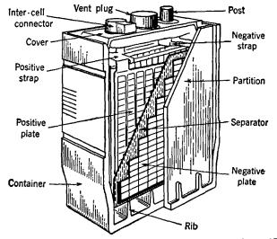
FIG. 3-23.-A complete cell cut away to show details of construction. (Electric Storage Battery Co.)
