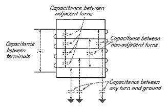
FIG. 9-14.-Distributed capacitances of a coil.
