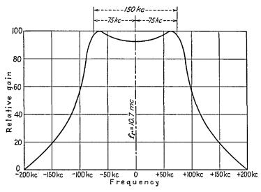
FIG. 12-33.-A double peak i-f response curve for an f-m receiver.
