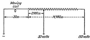
FIG. 6-21.—Internal circuit of a voltmeter having a 30- and 150-volt range.
