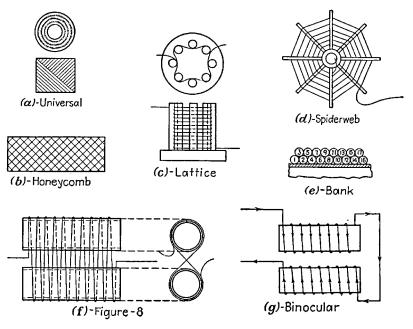
FIG. 8-13.—Various methods of winding high-frequency coils.
