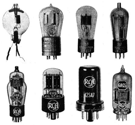
Fig. 1-14.—Evolution from the early De Forest tube to the modern vacuum tubes of more complex structure. (RCA Manufacturing Co., Inc.)
