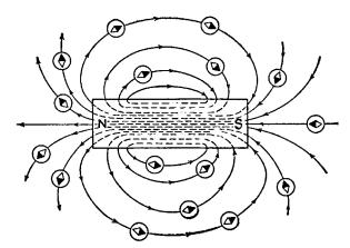
FIG. 5-12.---Magnetic field about a bar magnet illustrated by small compasses.
