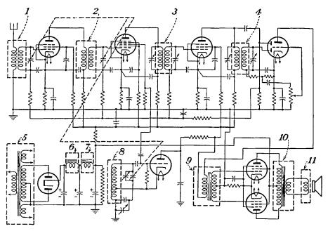
FIG. 8-21.--A typical superheterodyne circuit. The various inductors are shown enclosed in the heavy broken-line boxes.
