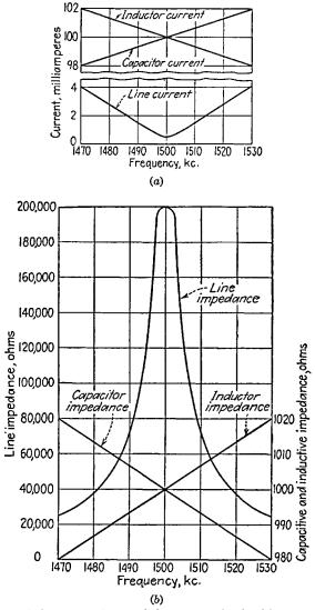
Fig. 11-9.—Characteristic curves of a parallel resonant circuit: (a) current curves, (b) impedance curves.
