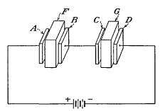
FIG. 9-12.-Effect of two capacitors connected in series.
