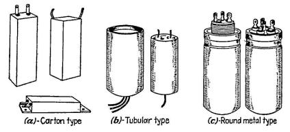
FIG. 9-25-Various forms of dry-electrolytic capacitors. (P. R. Mallory & Co., Inc.)
