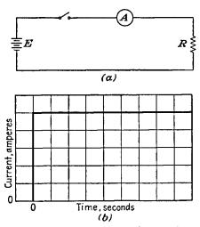
FIG. 12-37.—Characteristics of current vs. time for a circuit containing only resistance: (a) the circuit, (b) current vs. time characteristics.
