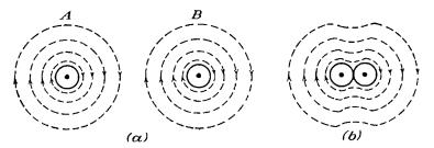
FIG. 5-34.—Magnetic fields about adjacent conductors of a coil carrying a current: (a) conductors separated, (b) conductors adjoining.
