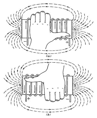
FIG. 5-35.--Left-hand rule for a coil: (a) electrons entering the coil at the right terminal, (b) electrons entering the coil at the left terminal.
