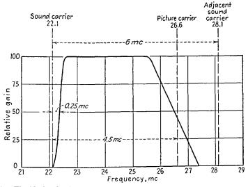
FIG. 12-35.—The ideal video i-f response curve for the reception of vestigial-side-band transmission of television signals.
