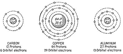
FIG. 2-2.-Structure of carbon, copper, and aluminum atoms.
