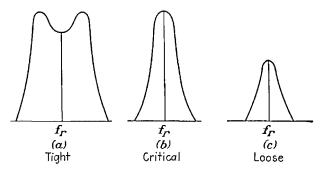
FIG. 12-25.- Response curves showing the effect of various amounts of coupling.
