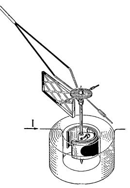
FIG. 6-15.—The concentric-type moving iron-vane mechanism. (Weston Electrical Instrument Corporation.)
