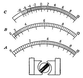
FIG. 6-11.—Meter scales produced by d'Arsonval instruments whose core and pole pieces have eccentric faces: A, effect of eccentricity on uniform scale; B, effect of eccentricity on square-law scale; C, effect of eccentricity on logarithmic scale.
