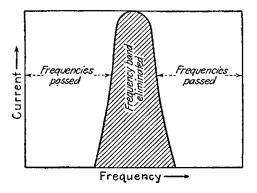
FIG. 12-12.-Characteristic curve for a simple band-stop filter circuit.
