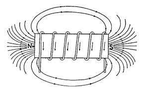
FIG. 5-32 .- Magnetic field about a coil carrying a current.
