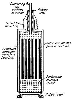
FIG. 9-18.—Cross-sectional view showing the construction of a commercial wet-electrolytic capacitor.
