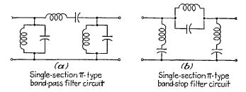
FIG. 12-19.—A  $\pi$ -type band-pass and band-stop filter circuits.
