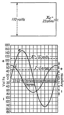
FIG. 10-3.—Voltage and current characteristics if a perfect capacitor were connected to an a-c power supply.
