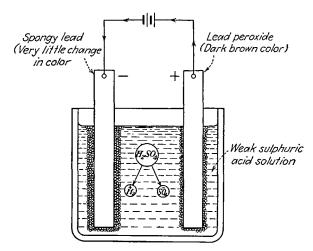
FIG. 3-17.—Forming the plates of a simple cell by passing a current through the cell.
