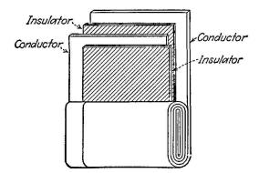
FIG. 9-5.—Typical construction of paper dielectric capacitors.
