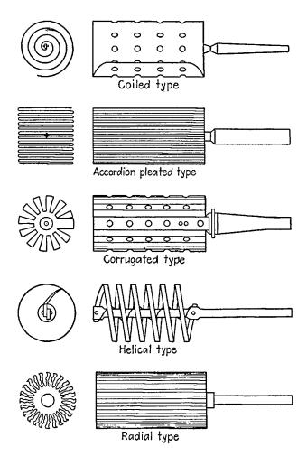
FIG. 9-20.-Types of construction used for the positive electrode.
