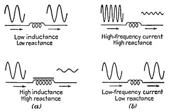
FIG. 12-3.—Effects of inductance and frequency on current flow: (a) variable inductance, constant frequency; (b) variable frequency, constant inductance.
