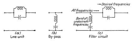
FIG. 12-13.-Basic units of a band-stop filter circuit.
