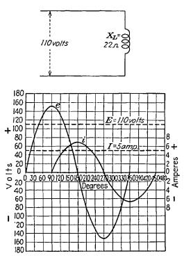
FIG. 10-2.—Voltage and current characteristics if a perfect inductor were connected to an a-c power supply.
