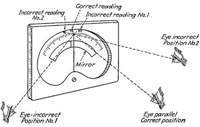
FIG. 6-24.—Errors possible in reading meters because of parallax.
