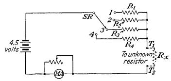
FIG. 6-34.—Diagram showing the use of resistors and switch to select the range of a multirange ohmmeter.
