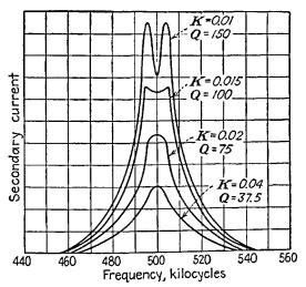
FIG. 12-31.—Characteristics of a band-pass amplifier circuit showing the effect of circuit Q on uniformity of response within the band being passed.
