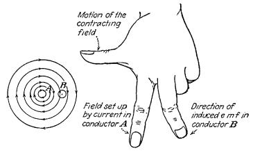
FIG. 8-4.—Voltage induced in conductor B when the current in conductor A is decreasing in strength: (a) direction of flow of electrons in conductor A, (b) left hand used to determine the direction of the induced emf.
