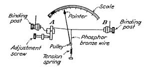
FIG. 6-3 .- Principle of the hot-wire meter. (Weston Electrical Instrument Corporation.)
