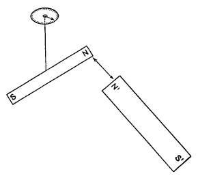
FIG. 5-9.-Measuring the force of repulsion by the torsion balance.
