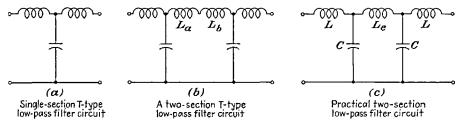
FIG. 12-14.—T-type low-pass filter circuits.
