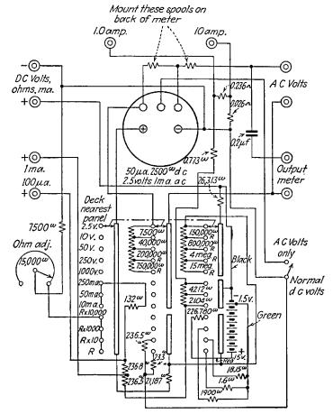
FIG. 6-36.—Schematic diagram of a combination meter. (Weston Electrical Instrument Corporation.)
