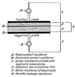
FIG. 9-28.—Factors affecting the equivalent series resistance of a dry-electrolytic capacitor. (P. R. Mallory & Co., Inc.)
