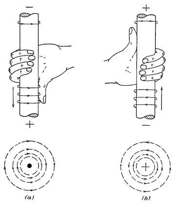
FIG. 5-30.—Left-hand rule for a wire carrying a current: (a) electrons flowing downward, (b) electrons flowing upward.
