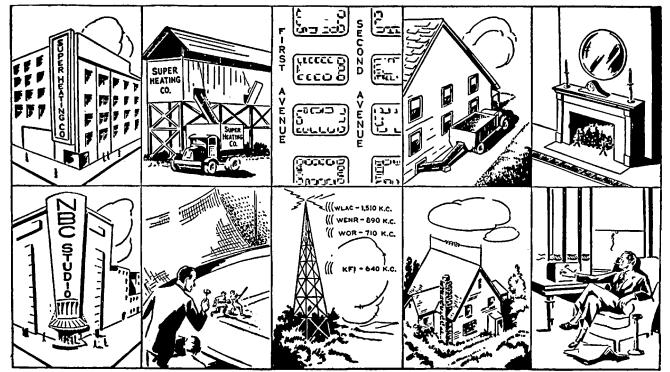
FIG. 1-23.-Comparison of delivery, receiving, and use of coal (top) with sending, receiving, and use of sound waves (below).
