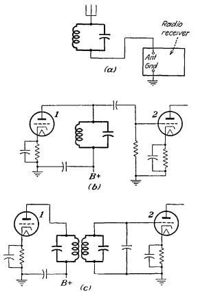
FIG. 11-10.—Applications of parallel resonant circuits in radio receivers.
