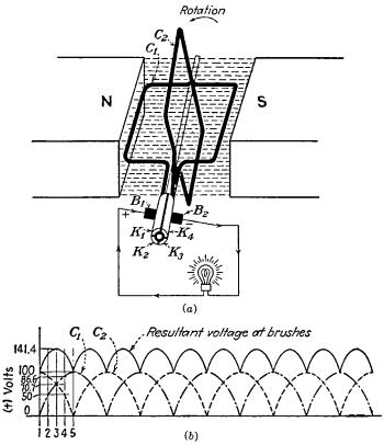
FIG. 7-13.—A two-coil d-c generator: (a) the generator, (b) voltage of the generator.
