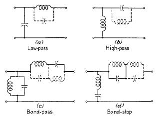
Fig. 12-21.—Shunt-derived m-type filter circuits. The dotted impedances are those added to the series unit to form the m-derived filter circuit.
