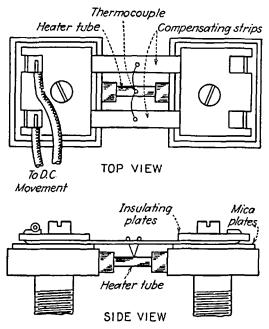
Fig. 6-5.—A compensated heating element of a thermocouple meter. (Weston Electrical Instrument Corporation.)
