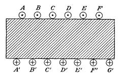
FIG. 5-33.—View showing the direction of the current in the conductors of the coil of Fig. 5-32.
