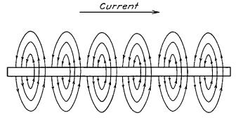
FIG. 5-31.-Magnetic field about a straight wire carrying a current.
