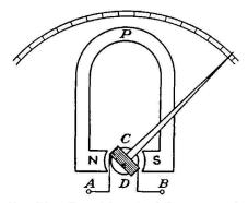
FIG. 6-7.—Essential parts of the permanentmagnet moving-coil meter.
