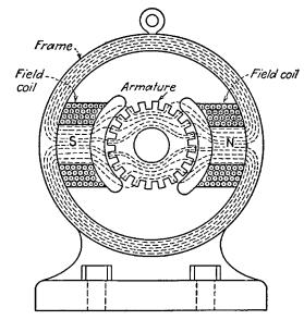
FIG. 7-15.—The magnetic circuit of a commercial two-pole generator.
