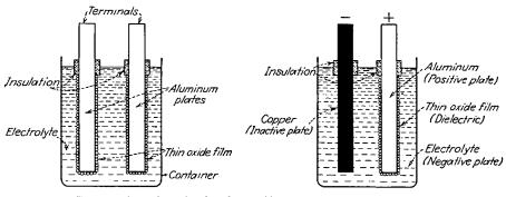
FIG. 9-16.—Construction of a simple electrolytic capacitor.
