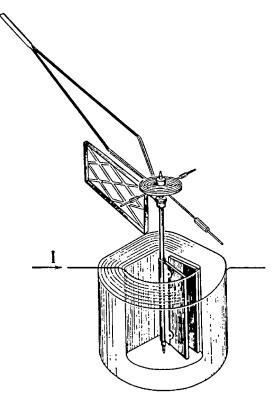
FIG. 6-14.—The radial-type moving iron-vane mechanism. (Weston Electrical Instrument Corporation.)
