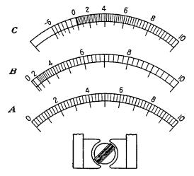
FIG. 6-10.—Meter scales produced by d'Arsonval instruments whose core and pole pieces have concentric faces: A, uniform scale; B, square-law distribution; C, logarithmic distribution.
