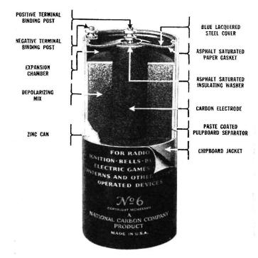
FIG. 3-6.—Cross-sectional view of the general-purpose dry cell. (National Carbon Company.)
