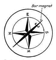
FIG. 5-26.-The simple compass.
