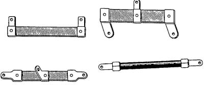
FIG. 4-2.-Wire-wound fixed resistors.
