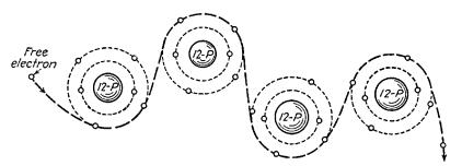
FIG. 2-3.—Path of a free electron in a carbon conductor.
