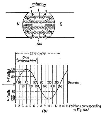
FIG. 7-5.—Induced emf of a conductor in the simple a-c generator.
