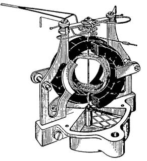
FIG. 6-17.—Cutaway view illustrating the construction of a commercial type of dynamometer mechanism. (Weston Electrical Instrument Corporation.)
