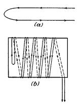
FIG. 8-19.—Noninductive winding: (a) a loop of wire, (b) a noninductively wound coil.
