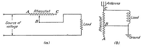
Fig. 4-23.—Circuits illustrating uses of rheostats: (a) rheostat in series with a load, (b) rheostat in parallel with a load.
