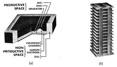
FIG. 3-13.—Construction of Layer-Bilt battery: (a) cross-sectional view of a cell, (b) stack of 15 cells. (National Carbon Company.)
