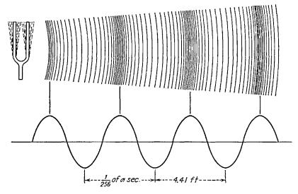
FIG. 1-21.—Propagation of sound waves.
