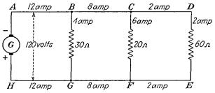
FIG. 4-10.-Current distribution of the parallel circuit shown in Fig. 4-9.
