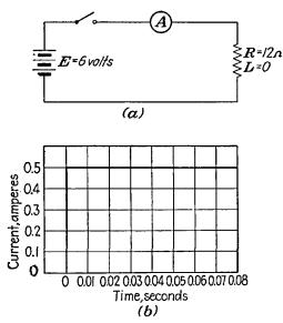
FIG. 8-6.—Time required for the current to build up in a circuit containing only resistance: (a) the circuit diagram, (b) a graph showing the relation between current and time.
