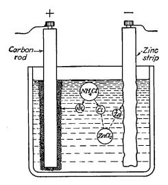
FIG. 3-5.—Chemical action of a simple cell.
