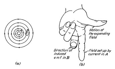
FIG. 8-3.—Voltage induced in conductor B when the current in conductor A is increasing in strength: (a) direction of flow of electrons in conductor A, (b) left hand used to determine the direction of the induced emf.
