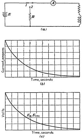
FIG. 12-39.— Characteristics of current and voltage vs. time: (a) the circuit, (b) current vs. time characteristics with the switch in position 2, (c) voltage vs. time characteristics with the switch in position 2.
