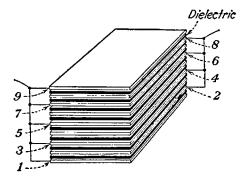
FIG. 9-3.-A parallel-plate capacitor.
