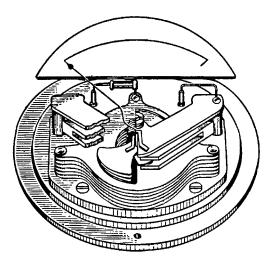
FIG. 6-2.—Internal construction of a commercial electrostatic voltmeter. (Weston Electrical Instrument Corporation.)
