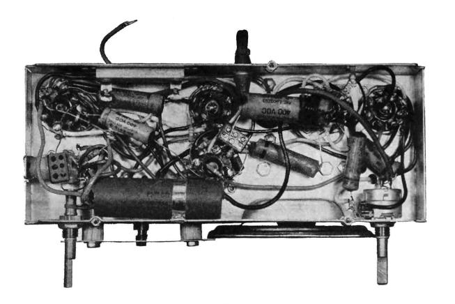
(b) FIG. 9-34.—Two views showing parts used in a radio receiver: (a) top view, (b) bottom view. (Philco Corvoration.)
