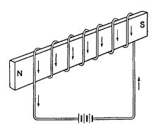
FIG. 5-4.—Magnetizing a steel bar by means of an electric current.
