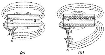
FIG. 5-17.—Magnetic induction: (a) nail A magnetized by induction, (b) nail B magnetized by contact with nail A.
