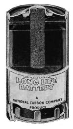
F16. 3-7.—Cross-sectional view of a size D unit cell. (*National Carbon Company.*)
