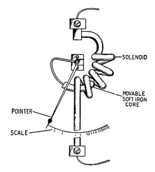
FIG. 6-12.—Early iron-vane instrument of the suction type. (Weston Electrical Instrument Corporation.)
