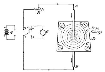
FIG. 5-29.--Magnetic field about a wire carrying a current.
