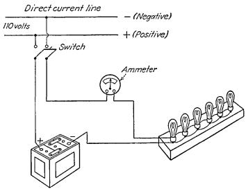
FIG. 3-26.—Charging a storage battery from a d-c power line.
