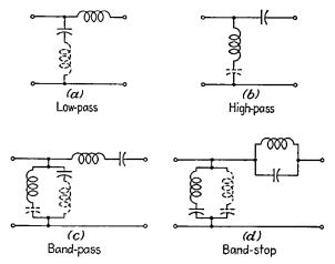
FIG. 12-20.—Series-derived m-type filter circuits. The dotted impedances are those added to the shunt unit to form the m-derived filter circuit.
