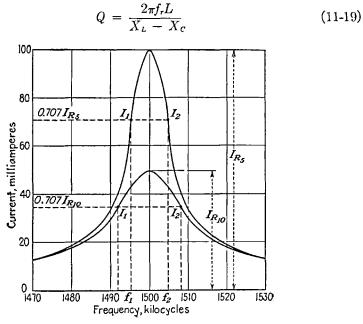
FIG. 11-5.—Resonance curves with the width of the band  $(f_2 - f_1)$  indicated.
