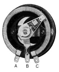
FIG. 4-26.—A wire-wound potentiometer with a left-hand taper.
