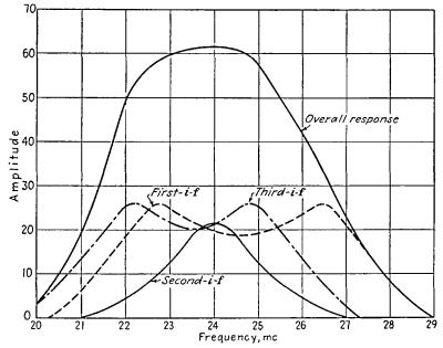
FIG. 12-36.—Wide pass band for the i-f response curve in the video section of a television receiver obtained by use of both stagger tuning and over-coupled i-f transformers.
