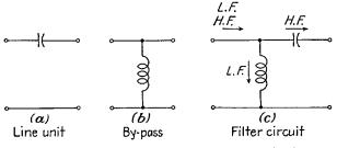
FIG. 12-9.—Basic units of a high-pass filter circuit.
