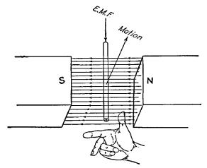
FIG. 7-2.—Fleming's right-hand rule for determining the direction of the induced emf.
