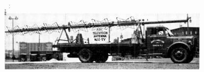
Fig. 13–38. A six-bay superturnstile antenna before erection. (Courtesy of American Broadcasting Company.)
