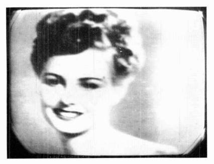
Fig. 3–17. The appearance of ion spot on the face of a cathoderay tube that employs electrostatic focus and magnetic deflection. The ion spot is the small, dark circular area over the subject's left evebrow. (Courtesy of Sylvania Electric Products, Inc.)
