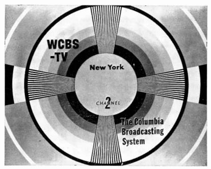
Fig. 10–9. A typical station test pattern. (Courtesy of Columbia Broadcasting System.)
