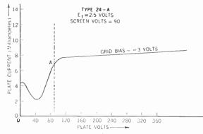
Figure 406. Plate-current — plate-voltage characteristic curve for the tetrode (type 24-A).
