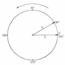
Figure 285. Vector diagram showing the current (I) lagging 30° behind the emf (E). Compare this diagram with the curve in Figure 282.
