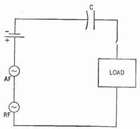
Figure 342. The resistor of Figure 341 has been replaced by a capacitor (*C*).
