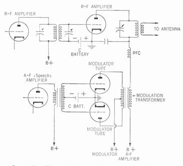
Figure 474. Plate modulation, transformer coupling. Neutralization is omitted for the sake of simplicity.
