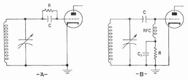
Figure 427. Methods of obtaining grid bias by the grid-leak-capacitor method. A—Series method. B—Shunt or parallel method.
