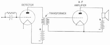
Figure 83. Diagram showing how the detector is coupled to the a-f amplifier by means of a transformer.
