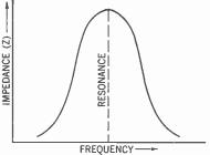
Figure 337. Resonance curve for the parallel resonant circuit with impedance (Z) plotted against the frequency (f). C and L are kept constant.
