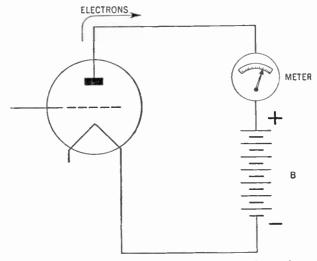
Figure 165. Meter connected in the plate circuit of the triode to show the flow of electrons.
