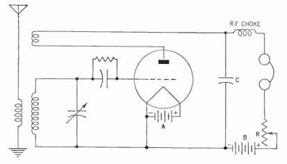
Figure 77. Three-circuit tuner using a fixed capacitor (C) of about 0.00025  $\mu$ f and a rheostat (R) of about 50,000 ohms to control the amount of feedback.
