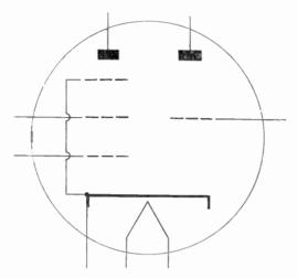
Figure 188. The 6F7 tube (one pentode-one triode).
