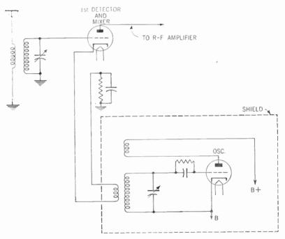
Figure 159. Circuit showing how current from the local oscillator is inductively coupled to the *cathode* of the first detector and mixer tube.
