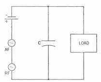
Figure 344. The capacitor (C) is now in parallel with the load and acts as a lowpass filter—that is, the low-frequency currents can pass to the load.
