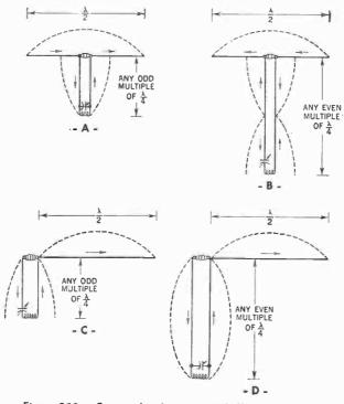
Figure 383. Current distribution on a half-wave antenna. A and B—The center-fed antenna. C and D—The end-fed antenna.
