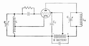
Figure 441. The electron-coupled oscillator.
