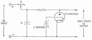
Figure 498. A saw-tooth oscillator using a thyratron tube.
