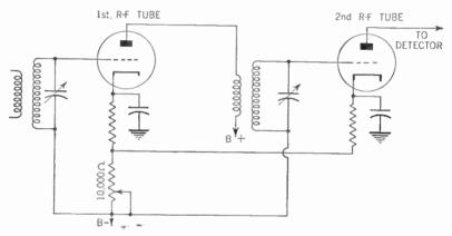
Figure 146. Circuit showing how the rheostat used as a volume control varies the grid bias of both radio-frequency tubes.
