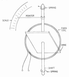
Figure 291. Diagram of the inclined-coil a-c meter.
