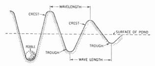
Figure 6. Sectional view of the pond showing what is meant by wavelength.
