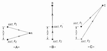
Figure 388. Diagrams explaining how the radiation pattern of Figure 387 is formed.
