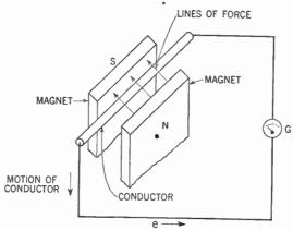
Figure 270. Diagram of a conductor cutting across lines of force between poles of a magnet.
