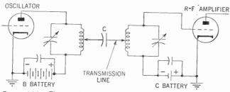
Figure 445. The matched-impedance transmission-line method of coupling.
