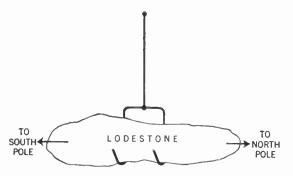
Figure 230. Figure showing how a freely swinging magnet turns so that its poles face the North and South Poles.
