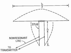
Figure 384. Current distribution on an antenna using quarter-wave matching stub.
