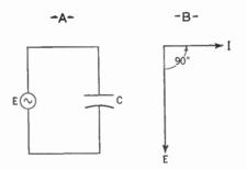
Figure 320. A—Circuit containing capacitance only. B—Vector diagram showing voltage (E) lagging 90° behind current (I).
