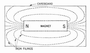
Figure 236. How to get a pattern of the lines of force around a magnet by the use of iron filings.
