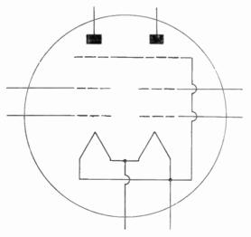
Figure 189. The 1E7-G tube (two pentodes).
