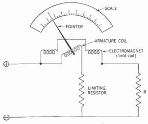
Figure 267. Circuit of wattmeter connected to measure power consumed by resistor (R).
