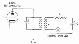
Figure 466. Circuit of the dummy antenna.
