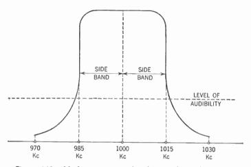
Figure 163. Ideal tuning curve for the superheterodyne receiver. Note that the side bands are fully received, but the unwanted stations are well below the level of audibility.
