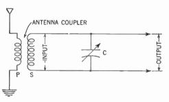
Figure 330. The tuning circuit of the radio receiver as a resonant circuit.
