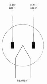
Figure 184. Diagram of a duo-diode tube. The type 80 is an example.
