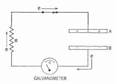
Figure 310. Capacitor discharging through resistor (R).
