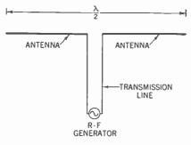
Figure 377. Transmission line connecting the r-f generator to the antenna.
