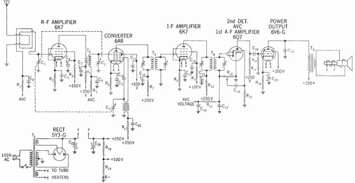
Figure 203. Circuit of a typical a-c superheterodyne receiver. On the opposite page is a list of values.
