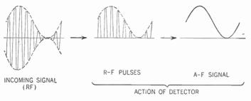
Figure 469. How the detector demodulates the incoming radio-frequency signal.
