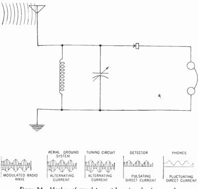
Figure 34. Hookup of complete crystal receiver showing wave forms of electric currents flowing in the various parts.
