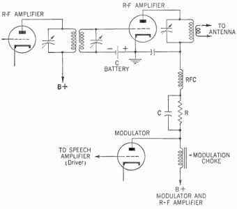
Figure 475. Plate modulation, choke coupling.
