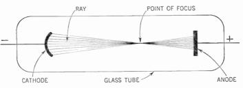
Figure 483. The cathode rays may be focused like light rays.
