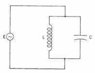
Figure 335. The parallel resonant circuit with inductance (L) and capacitance (C) in parallel.
