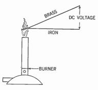
Figure 296. Diagram illustrating the principle of a thermocouple.
