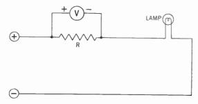
Figure 261. Circuit showing how the voltmeter is used to measure the potential drop across resistor (R).
