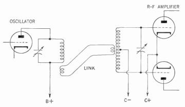
Figure 451. Method of coupling the oscillator to the push-pull radiofrequency amplifier by means of a link-coupled transmission line.
