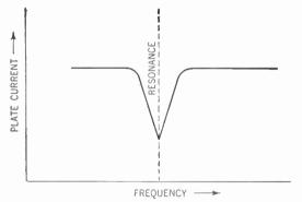
Figure 464. Graph showing the dip in plate current which indicates that the plate tank circuit is at resonance.
