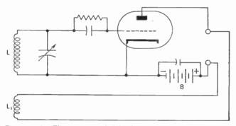
Figure 436. The output is fed back into the oscillatory circuit by means of an inductor ( $L_1$ ).
