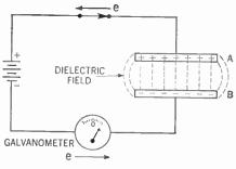
Figure 308. Capacitor being charged.
