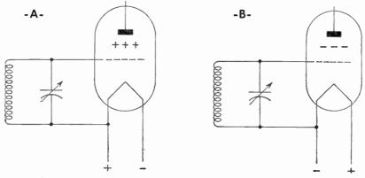
Figure 107. Circuits showing how alternating current flowing through the filament places an alternating charge on the grid of the tube.
