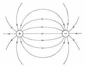
Figure 227. Lines of force between two opposite charges.
