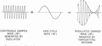
Figure 468. How the continuous carrier wave is modulated by the audio-frequency note.
