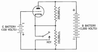
Figure 459. The blocked-grid method of keying.
