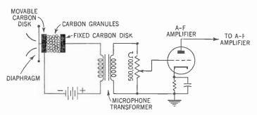
Figure 478. Hookup for the carbon-grain microphone.
