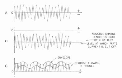
Figure 69. Graphs showing effect of placing a steady negative charge, or bias, on the grid of the triode.
