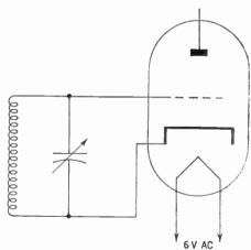
Figure 110. Circuit showing how the cathode is connected to the grid return.
