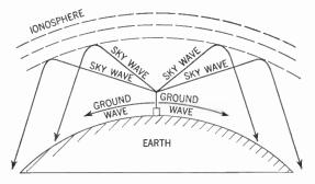
Figure 359. Diagram showing reflection of the sky waves from the ionosphere.
