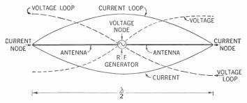
Figure 370. Diagram showing standing current and voltage waves on a half-wavelength doublet antenna.
