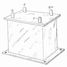
Figure 87. The Audio-frequency Transformer.
