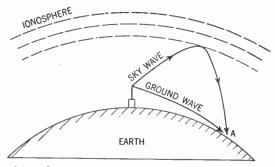
Figure 364. Diagram showing how fading is produced. The ground wave and the sky wave arrive at the same point (A) out of step (out of phase) and tend to neutralize each other. This condition causes the signal to fade out.
