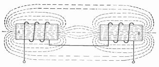
Figure 303. Inductors in series with their magnetic fields aiding each other. Note the windings are in the same direction on both coils.
