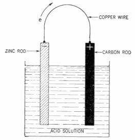
Figure 218. The voltaic cell.
