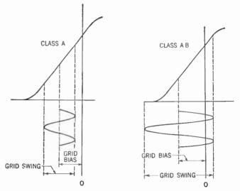
Figure 414. Graphs showing how a greater grid swing is possible with the class AB amplifier.
