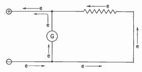
Figure 260. Circuit showing how a galvanometer is hooked up to measure the voltage of the line.
