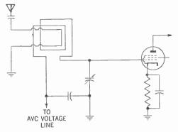
Figure 195. The loop antenna coupled to an external antenna.
