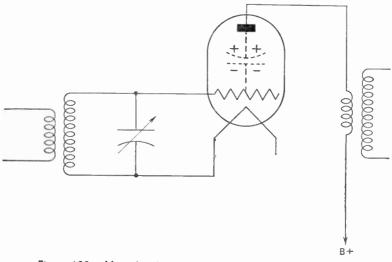
Figure 132. How the charge on the plate causes an opposite charge to be placed on the grid of the tube.
