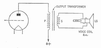
Figure 420. How the output transformer is used to match the impedance of the voice coil to the resistance of the tube.
