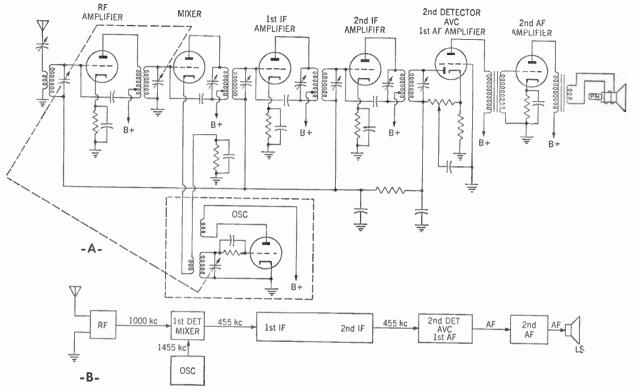
Figure 164. A—Circuit of the complete superheterodyne receiver. B—Block diagram showing arrangement of the component parts.
