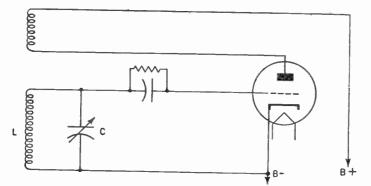
Figure 156. Circuit of the local oscillator. Note how it resembles the regenerative detector.
