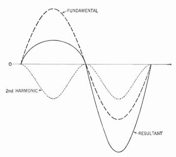
Figure 408. Graph showing the effect of adding the fundamental to the second harmonic which is below the X axis.
