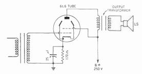
Figure 179. Circuit of beam power tube used as a power tube.
