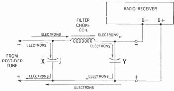
Figure 96. Hookup showing the filter system.
