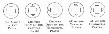
8. How may the cathode-ray oscillograph be used as a voltmeter?
