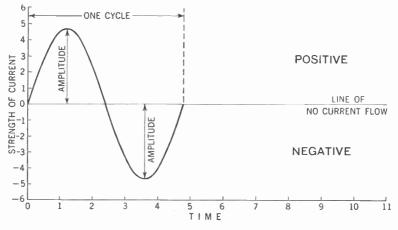
Figure 26. Graph showing curve or wave form of an alternating current. A curve whose current strength rises and falls in the smooth, even, and regular glide pictured here is called a *sine curve*.
