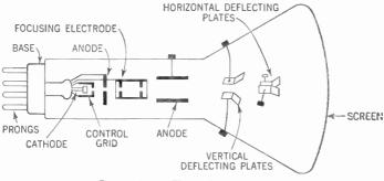
Figure 493. The cathode-ray tube.
