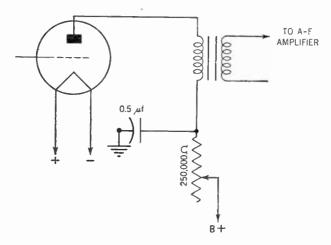
Figure 141. Circuit showing how a rheostat in the plate circuit is used to control volume. This device is unsatisfactory.
