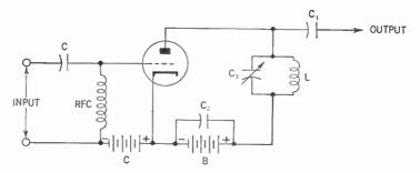
Figure 429. A stage of radio-frequency amplification. Note the resemblance to the audio-frequency stage in Figure 428.
