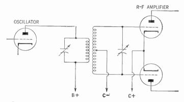
Figure 449. The inductive method of coupling a push-pull radio-frequency amplifier to the oscillator.
