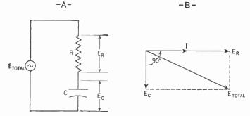
Figure 324. A—Circuit with resistance (R) and capacitance (C) in series. B—Vector diagram showing how the voltage drop across the resistor ( $E_R$ ) is added to the voltage drop across the capacitor ( $E_C$ ).
