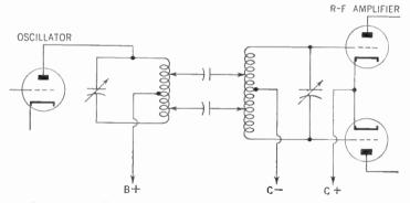
Figure 450. The matched-impedance transmission line method of coupling an oscillator to a push-pull radio-frequency amplifier.
