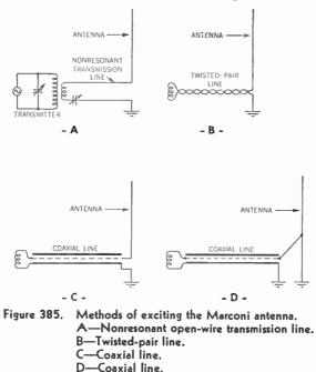
resonant transmission lines are used. Figure 385-A shows the antenna inductively coupled to the transmitter. Since the coupling coil increases the natural frequency of the antenna, a capacitor may be inserted to bring it back again to its desired value. Figure 385-B shows the twisted-pair line being used. In Figure 385-C, use is made of the coaxial line. A variation of this method is shown in Figure 385-D. Here, the transmission line is terminated on a point on the antenna
