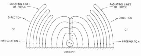
Figure 355. How lines of force are radiated when one end of the generator is connected to the ground.
