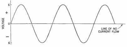
Figure 106. Wave form of alternating current used to heat the filament of the tube.
