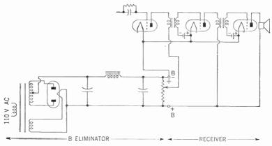
Figure 105. Completed B eliminator, showing how it is connected to the radio receiver.
