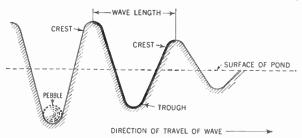
Figure 7. Sectional view of the pond. The heavy line shows the path of the wave going through one cycle.
