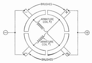
Figure 254. Diagram showing commutator connections for four-pole motor.
