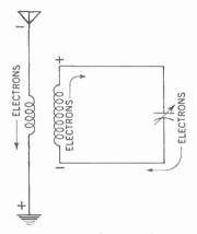
Figure 46. Diagram showing electrical charges and direction of electron flow in the aerial-ground system and tuning circuit during a half cycle of current flow. During the next half cycle, the charges and flow of electrons are reversed.
