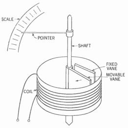
Figure 290. Diagram of the moving-vane a-c meter.
