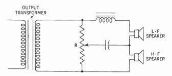
Figure 154. Circuit showing how tone control may be obtained through the use of high-frequency and low-frequency loudspeakers. The potentiometer (R) determines which speaker shall obtain the greater current.
