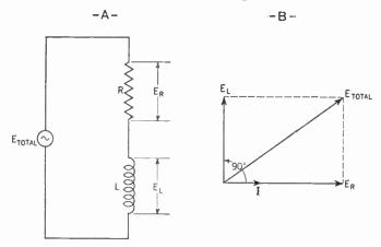
Figure 323. A—Circuit with resistance (R) and inductance (L) in series. B—Vector diagram showing how the voltage drop across the resistor  $(E_R)$  is added to the voltage drop across the inductor  $(E_L)$ .
