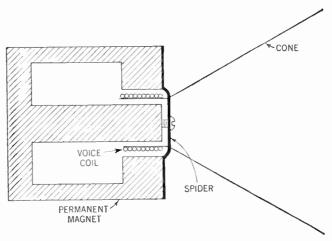
Figure 121. Diagram of a permanent-magnet dynamic speaker.
