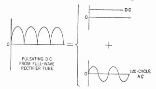
Figure 347. Wave-form diagram showing the pulsating direct current from the full-wave rectifier tube broken down into its two components, a steady direct current which goes to the radio set and a 120-cycle alternating current which is filtered out.
