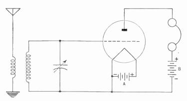
Figure 66. Diagram showing how alternating current from the tuning circuit places positive and negative charges on the grid of De Forest's tube.
