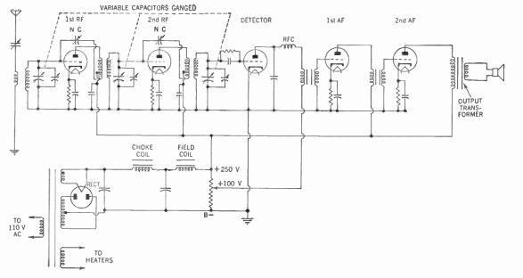
Figure 139. Circuit for a complete, tuned radio-frequency receiver.
