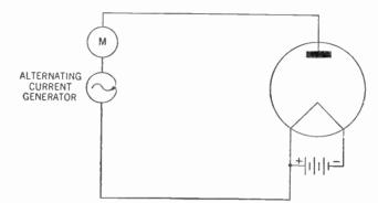
Figure 59. Fleming's experiment with an alternating-current generator connected to the plate of the tube. Electric current flowed through the meter only during the positive half of the alternating-current cycle.
