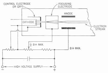
Figure 492. Voltage relationship between the various portions of the electron gun.
