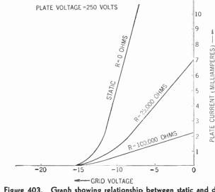
Figure 403. Graph showing relationship between static and dynamic curves for a 6J5 triode.
