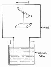
Figure 240. Showing how the magnetic field around a conductor carrying an electric current deflects the compass needle.
