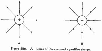
B—Lines of force around a negative charge.
