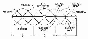
Figure 367. Sinusoidal distribution of current and voltage along an antenna. The Greek letter  $lambda(\lambda)$  is the symbol for wavelength.
