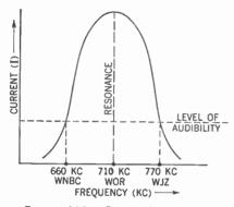
Figure 329. Curve of a resonant circuit showing the relationship of current (I) to changes in frequency. The inductance and capacitance of the circuit are kept constant.
