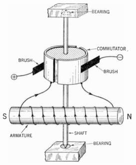
Figure 249. Figure showing the commutator and armature arrangement of the electric motor.
