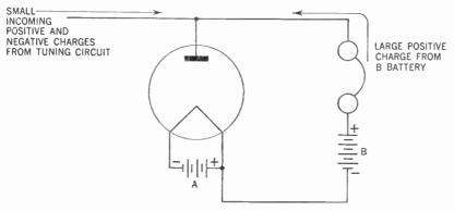
Figure 63. Diagram showing how the weak positive and negative charges placed on the plate of the diode are overwhelmed by the large positive charge placed on the same plate by the B battery.
