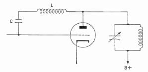
Figure 433. Circuit using direct plate-to-grid neutralization.
