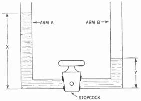
Figure 210. Diagram illustrating the fact that it is the *difference* of pressure which causes a fluid to flow through a tube.
