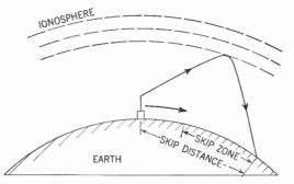
Figure 361. Diagram showing what is meant by skip zone. In this zone no signals are received.
