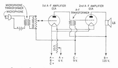
Figure 93. Diagram showing circuit of the public-address system.
