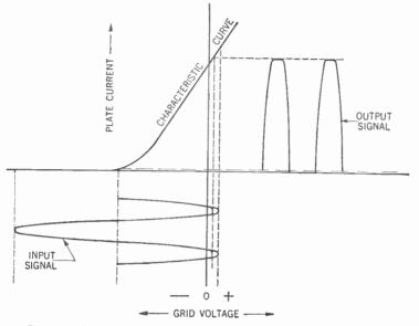
Figure 424. Distortion of the output signal in a class B amplifier. While this distortion would prevent us from using a single tube in class B as an audio-frequency amplifier, we can do so in the radio-frequency amplifier because of the "flywheel" effect.
