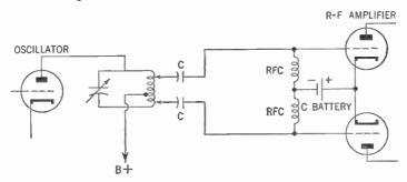
Figure 448. Direct or capacitive coupling for the push-pull radio-frequency amplifier.
