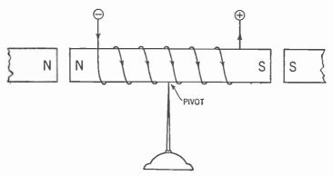
Figure 245. The electromagnet pivoted so that it may rotate between two fixed poles.
