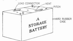
Figure 225. The lead-acid storage battery containing three cells connected in series.
