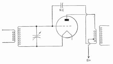
Figure 134. How a neutralizing capacitor (NC) is employed to eliminate the feedback due to the internal capacitance between the grid and plate of the tube.
