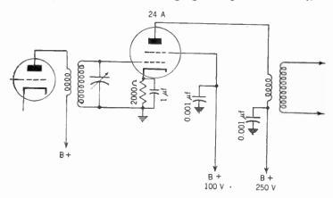
Figure 173. Circuit of a stage of radio-frequency amplification using the 24A type of screen-grid tube.
