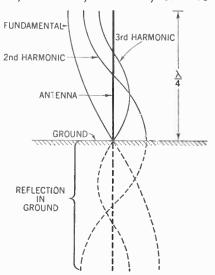
Figure 375. Voltage distribution on a quarter-wave Marconi antenna at the fundamental, 2nd harmonic, and 3rd harmonic frequencies. Only half the voltage wave is shown for the sake of simplicity. Note the voltage loop at the ground for the 2nd harmonic.
