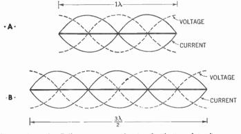
Figure 371. A—Full-wave antenna, showing distribution of standing waves of current and voltage. B—One-and-one-half wave antenna.
