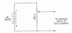
Adjust the oscillograph to place a 60-cycle sweep on the horizontal plates. Observe the location of the horizontal line. Move the potentiometer arm and notice changes of the image on the screen.
