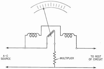
Figure 294. Diagram showing how the dynamometer type of meter is hooked into the circuit to read alternating voltage. (The effective current must be kept constant.)
