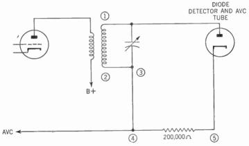
Figure 147. Circuit showing how the diode acts as a detector and automatic-volume-control tube.
