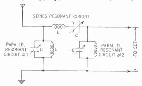
Figure 350. Diagram showing how series and parallel resonant circuits are used to allow signals of only one band of frequencies to pass. The band-pass filter.
