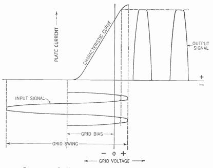
Figure 425. Graph showing relationship between the input and output signals in a class C amplifier.
