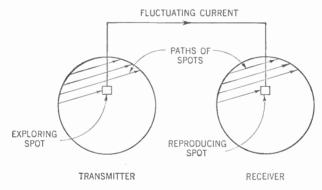
Figure 499. The basic principle of television. The two spots keep in step with each other.
