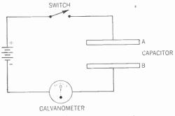
Figure 307. Capacitor ready for charging.
