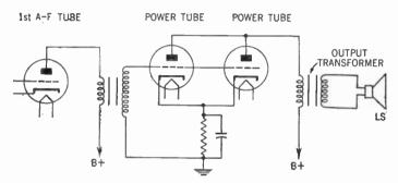
Figure 167. Circuit showing how two power tubes are connected in parallel to handle greater power.
