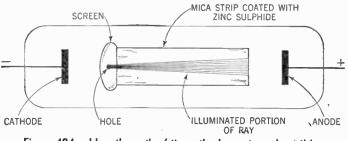
Figure 484. How the path of the cathode ray is made visible.
