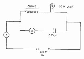
The value of the choke is 30 h at 200 ma. The capacitor is rated at 600 v working voltage. The ammeters are alternating-current meters. Note the readings of the two ammeters.
