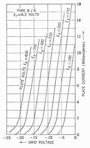
Figure 400. Family of transfer or mutual-characteristic curves for the triode (type 6J5).
