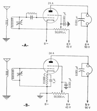
Figure 174. A—Circuit of a tetrode used as a grid-leak-capacitor detector. B—Circuit of a tetrode used as a cathode-bias detector.
