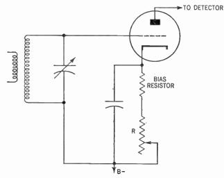
Figure 145. Circuit showing how a rheostat (R) is placed in series with the bias resistor to act as a volume control.
