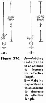
tor and the *distributed capacitance* of the antenna) give a total which is smaller than either, the natural frequency of the antenna is increased until once again it is in resonance with the signal frequency (Fig. 376-B).
