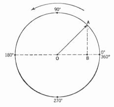
Figure 283. Diagram showing what is meant by a vector.
