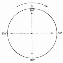
Figure 275. Figure showing degrees of a circle. If the complete circle is taken to stand for one revolution, then a quarter turn would amount to 90°, a half turn 180°, a three-quarter turn 270°, and a full turn or revolution 360°.
