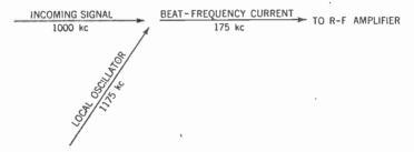
Figure 155. Diagram showing how the incoming signal mixes with the current produced by the local oscillator to produce the beat-frequency current.
