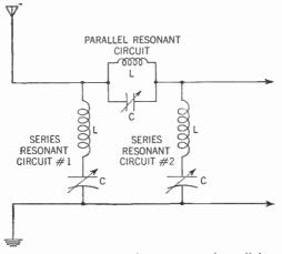
Figure 351. Diagram showing how series and parallel resonant circuits are used to stop signals of one band of frequencies from passing. The band-stop filter.
