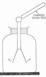
Figure 206. The effect of a charged rod on the gold-leaf electroscope.
