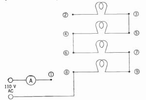
The lamps are each 110-volt, 50-watt. The ammeter is an alternating-current 0 to 5-amp ammeter.
