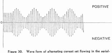
Figure 30. Wave form of alternating current set flowing in the aerialground system when the modulated radio wave shown in Figure 29-C passes across the aerial of the receiving set.
