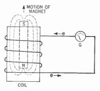
Figure 268. The magnet is plunged into the coil of wire. An electric current is induced in the coil.
