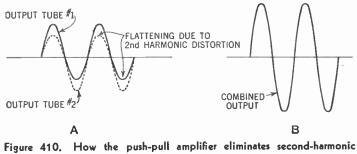
distortion. A—Graph showing output of each tube. B—Graph showing combined output of the output transformer. Note that the distortion has been eliminated.
