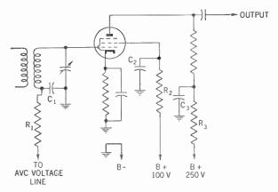
Figure 193. Circuit of a pentode amplifier showing the decoupling filters.
