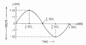
Figure 277. Curve showing relationship between time and the induced voltage.
