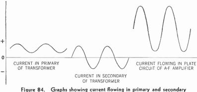
Figure 84. Graphs showing current flowing in primary and secondary of the transformer and in the plate circuit of the a-f amplifier. Note that the shape of all three curves is the same although the amplitudes vary.
