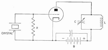
Figure 440. The crystal oscillator.
