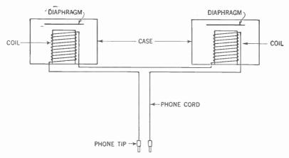
Figure 18. Diagram showing how a pair of phones are connected in series.
