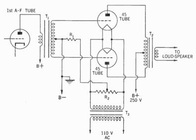
**Demonstration 2:** Build the push-pull audio-frequency amplifier shown on page 709:  $T_1$  is a push-pull input transformer;  $T_2$  is a push-pull output transformer;  $T_3$  is a 2.5-volt filament transformer;  $R_1$  is 400-ohm, 5 w;  $R_2$  is a 20- to 40-ohm center-tapped resistor; the power tubes are type 45.
