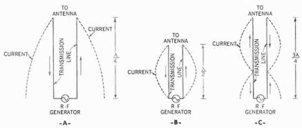
Figure 378. Standing waves of current on resonant transmission lines of various lengths.
