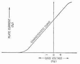
Figure 398. The grid-voltage — plate-current characteristic curve for a triode.
