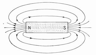
Figure 237. Pattern of lines of force around a magnet, showing the direction of the field.
