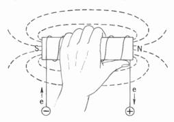
Figure 242. Method for determining the polarity of an electromagnet.
