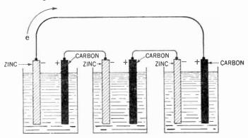
Figure 219. Three voltaic cells in series. Note that in series connections the + pole of one cell is always joined to the - pole of the next cell.
