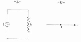
Figure 321. A—Circuit containing resistance only. B—Vector diagram showing voltage (E) and current (I) in phase.
