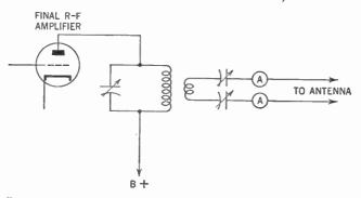
Figure 454. One method of coupling the final radio-frequency amplifier to a center-fed Hertz antenna.
