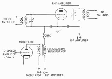
Figure 476. Grid modulation, transformer coupling.
