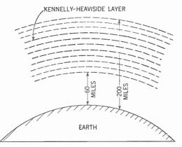
Figure 357. Diagram showing the Kennelly-Heaviside layer above the surface of the earth.
