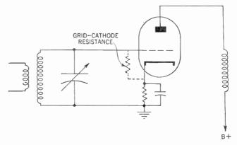
Figure 426. Diagram showing that the grid-cathode resistance of the tube is in parallel with the tuned circuit.
