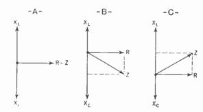
Figure. 333. Vector diagrams showing effect of frequency changes on a resonant circuit when the resistance (R) is large.
