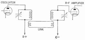
Figure 446. The link-coupled transmission line.
