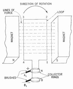
Figure 274. The loop after a three-quarter turn.
