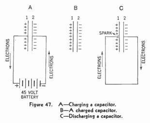
Now obtain a capacitor whose capacitance is about 1 microfarad  $(1 \mu f)$  and connect it to a 45-volt battery for a few seconds. Disconnect the battery. By means of a piece of wire, connect one plate of the capacitor to the other. You will notice a spark jump from the end of the wire to the second plate of the capacitor just as you are about to touch them together.
