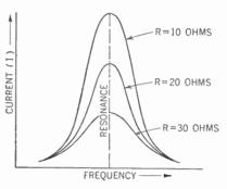
Figure 334. Resonance curves showing changes produced by changes in resistance (R). Inductance and capacitance are kept constant.
