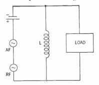
Figure 345. The inductor (L) is now in parallel with the load and acts as a high-pass filter—that is, the highfrequency currents can pass to the load. current is bypassed to the ground through the capacitor in Figure 136, Part I, by means of this filter system.
