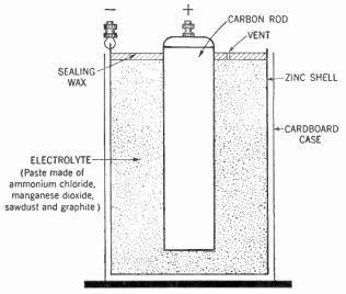
Figure 221. Cross-sectional view of the dry cell.
