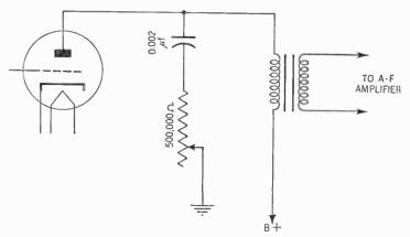
Figure 152. Circuit showing how a rheostat is connected in series with the capacitor to control the amount of high-frequency current filtered out.
