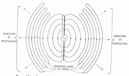
Figure 354. Diagram showing how the trapped lines of force are radiated or propagated.
