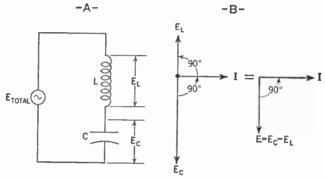
Figure 326. A—Circuit diagram with inductance (L) and capacitance (C) in series.
