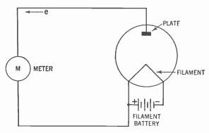
Figure 56. Diagram showing Edison's experiment.
