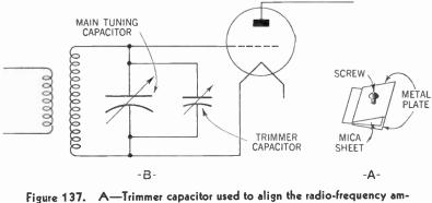
Figure 137. A—Trimmer capacitor used to align the radio-frequency amplifier stages. B—Circuit showing how the trimmer is connected across the main tuning capacitor.
