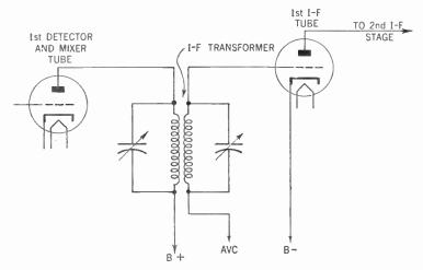
Figure 161. Circuit of the intermediate-frequency transformer.
