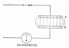
Figure 309. Capacitor fully charged. The battery has been removed.
