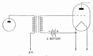
Figure 112. Circuit showing a C battery connected in the grid circuit of an amplifying tube.
