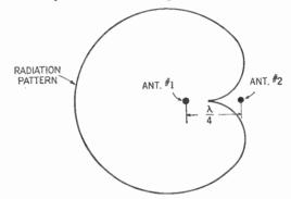
Figure 390. Unidirectional pattern (cardioid) for two vertical, halfwave antennas, a quarter wave apart and with currents 90° out of phase.
