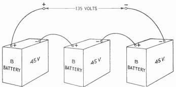
Figure 222. Circuit showing three B batteries connected in series.
