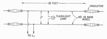
The terminals of the flashlight lamp are soldered to two bare copper wires that slide on the Lecher wires. As the lamp is moved over the wires, it glows brightly at some points and goes out at others, depending upon whether it is passing a loop or node of the standing wave.
