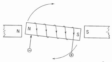
Figure 246. Looking down on the top of the electromagnet. Since like poles repel, the electromagnet is rotated in a clockwise direction.
