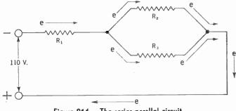
Figure 216. The series-parallel circuit.
