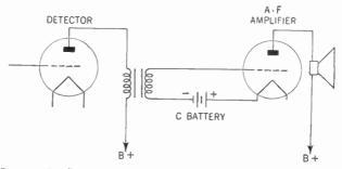
Figure 85. Diagram showing how a C battery is connected in the grid circuit of the amplifier tube.
