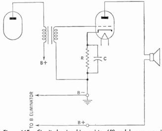
Figure 115. Circuit showing bias resistor (R) and bypass capacitor (C).
