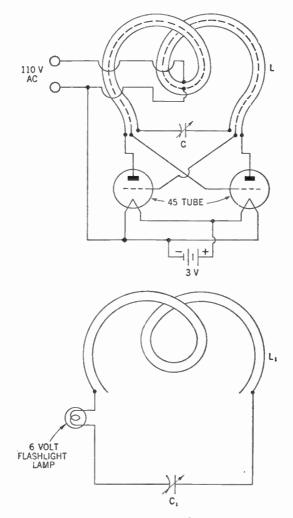
nance with the oscillator. Change C to vary the frequency of the oscillator. The flashlight lamp goes out, and  $C_1$  must be adjusted again before the lamp lights up again.
