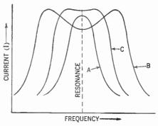
Figure 340. Resonant curves showing the effect of coupling. Curve A—Loosely coupled. B—Tightly coupled. C—Compromise between A and B.
