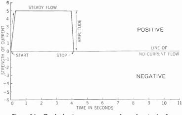
Figure 24. Graph showing curve or wave form of a steady direct current.
