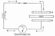
Figure 311. The effect of placing a dielectric (such as mica) between the plates of a fully-charged capacitor.
