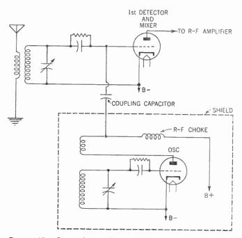
Figure 160. Circuit showing how a small fixed capacitor is used to couple the current from the local oscillator to the grid of the first detector and mixer tube.
