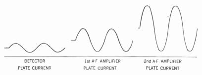
Figure 81. Graphs showing plate current in the detector, the first audio amplifier, and the second audio amplifier.
