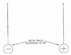
Figure 212. Figure showing two oppositely charged balls suspended far apart in air. Although there is a potential difference between them, no current flows because the resistance of the path between them is too great.
