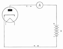
Figure 394. Circuit to show relationship between plate current and plate voltage.
