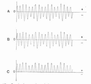
Figure 65. Graphs showing flow of electric current in various parts of the triode circuit.
