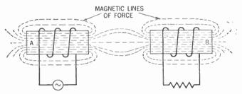
Figure 302. Diagram showing magnetic coupling between two inductors.
