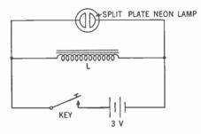
L is a 15- to 30-henry choke. Close the key. Since the neon lamp requires about 70 v before it lights up, no light appears. Now open the key quickly. The neon lamp flashes.
