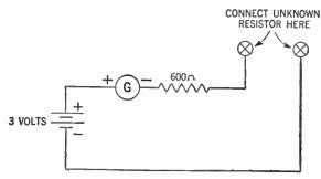
Figure 265. Circuit of the ohmmeter.
