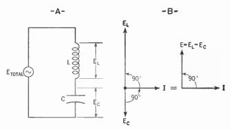
Figure 325. A—Circuit diagram with inductance (L) and capacitance (C) in series.
