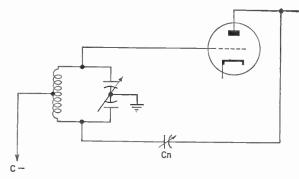
Figure 432. Circuit showing grid neutralization.
