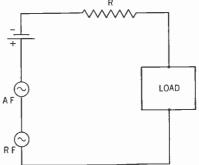
Figure 341. A battery, a low-frequency (af) generator, and a highfrequency (rf) generator supplying current to a load through a resistor (*R*).
