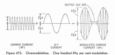
Since we are seeking the greatest amount of variation. modulation less than 100 per cent means we are not getting the most efficient utilization of the radiated power. On the other hand, overmodulation produces distortion. It can be readily seen that 100 per cent modulation is desirable.
