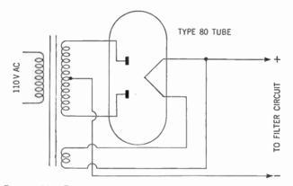
Figure 102. Type 80 rectifier tube with one filament and two plates. This tube is used for full-wave rectification.
