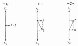
Figure 332. Vector diagrams showing effect of frequency changes on a resonant circuit when the resistance (R) is small. A—Resonance. B—Frequency reduced. Slightly off resonance. C—Frequency increased. Slightly off resonance.
