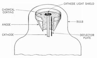
Figure 487. The tuning-eye tube.
