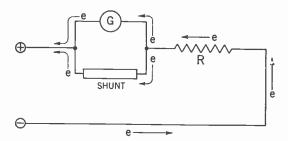
Figure 259. Circuit showing how an ammeter (galvanometer plus shunt) is used to measure the current flowing through the resistor (R).
