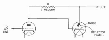
Figure 489. Circuit showing how the tuning-eye tube is connected to the automatic-volume-control line.
