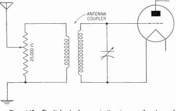
Figure 142. Circuit showing how a potentiometer across the primary of the antenna coupler is used as a volume control.
