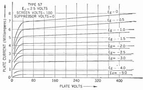
Figure 407. Family of plate-current — plate-voltage characteristic curves for the pentode (type 57).
