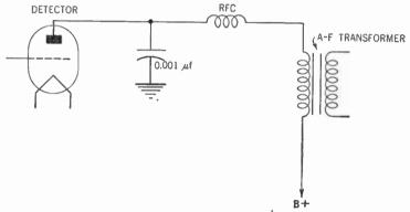
Figure 136. How a radio-frequency choke coil (*RFC*) and bypass capacitor are used to keep stray radio-frequency currents from leaking into the audio-frequency amplifier and power supply.
