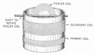
Figure 75. Three-circuit tuner showing arrangement to vary the coupling between the secondary coil and the tickler coil.
