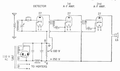
Figure 111. Radio circuit showing the use of a B-battery eliminator and cathode-type tubes.
