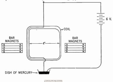
The coil consists of about 25 turns of bell wire. Both ends are bared. One end is connected to a piece of thin copper wire (No. 30 or finer) which suspends the coil. The other end dips into a small dish of mercury. A 6-volt battery is connected to the coil through the thin wire at one end and the mercury at the other.
