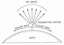
Figure 356. Diagram showing how a transmitting station sends out ground and sky waves.
