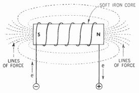
Figure 243. Diagram showing, by use of a soft-iron core, how lines of force of an electromagnet are concentrated at the poles.
