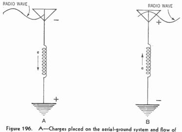
Figure 196. A—Charges placed on the aerial-ground system and flow of electrons as one half cycle of the radio wave passes the aerial. B—Charges and flow of electrons as the next half cycle of
