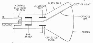
Figure 491. The basic diagram of the cathode-ray tube.
