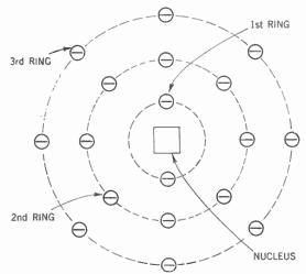
Figure 208. Picture of an atom of argon, showing the nucleus surrounded by the first three completed rings of planetary electrons.
