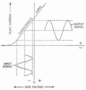
Figure 412. Graph showing relationship between the input and output signals in a class A amplifier.
