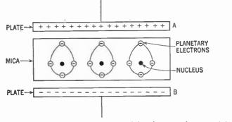
Figure 313. Distortion of the orbits of the planetary electrons of the atoms of the mica as a result of charging the capacitor plates.
