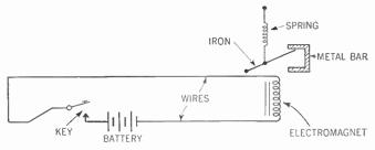
Figure 244. How the electromagnet is used in the telegraph.
