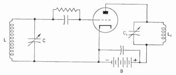
Figure 439. The tuned-grid tuned-plate oscillator.
