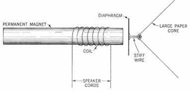
Figure 19. Diagram showing how an earphone is converted to a loud-speaker.
