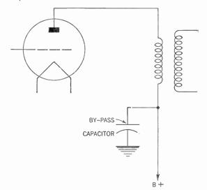
Figure 135. How a fixed capacitor is used to bypass any radio-frequency current leaking across the B supply.
