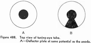
B-Deflector plate at lower potential than the anode.
