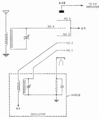
Figure 183. Complete circuit showing the pentagrid converter as the first detector, mixer, and oscillator tube in the superheterodyne receiver.
