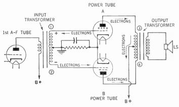
Figure 168. Circuit showing how two power tubes are connected in push-pull.
