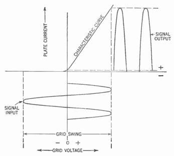
Figure 416. Graph showing how the special class B tubes operate on zero grid bias.
