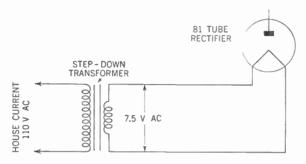
Figure 99. Step-down transformer used to heat the filament of the rectifier tube.
