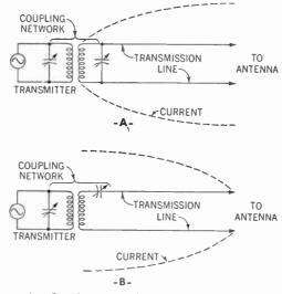
Figure 381. A—Coupling network with a current node at input end of the transmission line. B—Coupling network with a current loop at input end of the transmission line.
