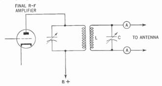
Figure 455. One method of coupling the final radio-frequency amplifier to an end-fed Hertz antenna.
