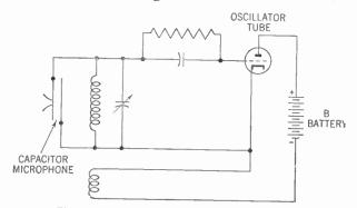
Figure 481. Theoretical circuit of the frequency-modulation transmitter.
