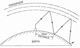
Figure 360. Diagram showing what is meant by skip distance.
