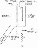
Figure 500. The iconoscope,
