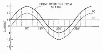
Figure 288. Curve showing the result of adding alternating and direct currents.
