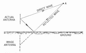
Figure 392. Diagram showing the effect of the ground upon the vertical radiation pattern of an antenna.
