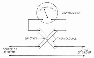
Figure 297. Diagram of the thermocouple ammeter.
