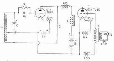
C is a 0.00035- $\mu$ f variable capacitor, C<sub>1</sub> is a 0.00025- $\mu$ f fixed capacitor, C<sub>2</sub> is a 0.002- $\mu$ f fixed capacitor; R<sub>1</sub> is 50,000 ohms; RFC is 33 turns of No. 32 double-cotton-covered wire on a  $\frac{1}{2}$ -in. dowel; L is a broadcast-band coil, L<sub>1</sub> is a 30-henry choke; T is the microphone transformer.
