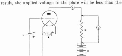
Figure 402. Circuit for obtaining the dynamic characteristic curves of a triode.
