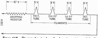
Figure 118. Diagram showing how the dropping resistor and the filaments of the rectifier, detector, and first and second audio-frequency amplifier tubes are connected in series across the 110-volt house line.
