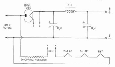
Figure 120. Diagram showing the circuit of the complete ac-dc power supply. The symbol 15h stands for a filter choke coil of 15 henrys.
