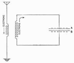
Figure 51. Diagram showing how the capacitor got its charge.
