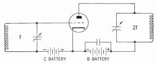
Figure 452. Circuit of the frequency multiplier. The plate tank circuit is tuned to a harmonic of the frequency to which the grid tank is tuned.
