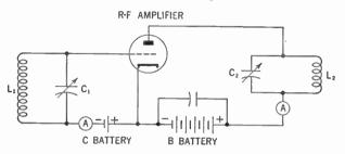
Figure 463. Diagram showing how direct-current milliammeters are hooked into the grid and plate circuits of the radio-frequency amplifier to test for resonance.
