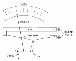
Figure 295. Diagram of a hot-wire ammeter.
