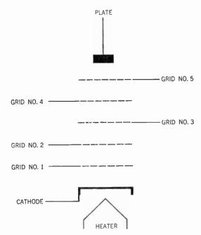
Figure 181. Diagram showing the arrangement of electrodes in the pentagrid converter tube.
