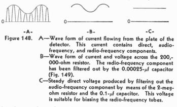
200,000-ohm resistor has the same wave form as the current and, therefore, is not suitable as bias for the grids of the radiofrequency tubes, where a steady bias is required. Therefore, we must filter out the radio- and audio-frequency components, leaving a steady direct voltage which may be applied to the grids.
