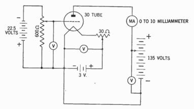
(a) Keeping the grid bias fixed, vary the plate voltage and draw the  $I_p$ - $E_p$  characteristic curve.
