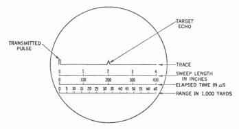
Figure 501. Trace on face of cathode-ray tube showing pips.
