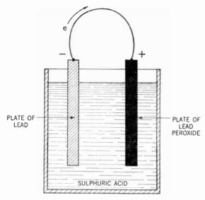
Figure 223. The lead-acid storage cell.
