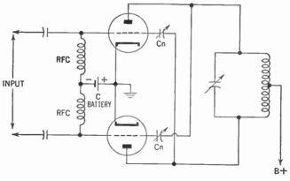
Figure 461. Circuit showing how neutralizing capacitors  $(C_n)$  are hooked up to neutralize a push-pull radio-frequency amplifier.
