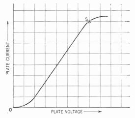
Figure 395. Graph showing the characteristic curve of the diode.
