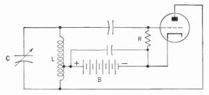
Figure 438. The Hartley oscillator.
