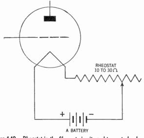
Figure 140. Rheostat in the filament circuit used to control volume. 219
