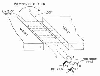
Figure 273. The loop after a half turn.
