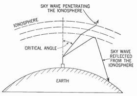
Figure 358. Diagram showing the critical angle. Sky waves of a certain frequency, striking the ionosphere at an angle less than the critical angle, penetrate and do not return to earth.
