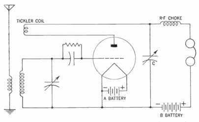
Figure 76. Three-circuit tuner using a variable capacitor (C) to control the amount of feedback. The inductor marked R-F Choke is a small coil of wire used to force some of the plate energy through C.
