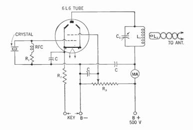
Close the key. The transmitter is now oscillating. This condition is indicated by the drop in plate current as shown on the milliammeter. If a 2-watt neon lamp is touched to the plate-circuit tank coil, the lamp will glow. Observe the caution against connecting this set to an antenna.
