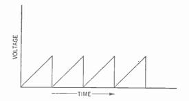
Figure 496. Wave form of the output of a saw-tooth oscillator.
