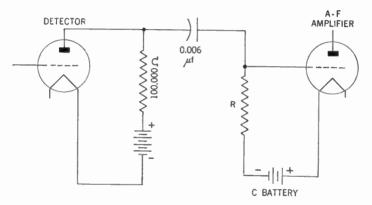
Figure 91. Diagram showing how grid resistor (R) is placed in the circuit.
