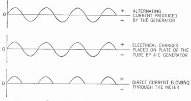
Figure 60. Graph showing the effect of connecting an alternating-current generator to the plate of Fleming's tube.
