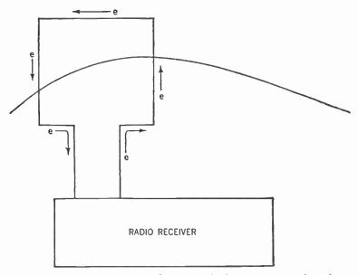
Figure 201. The flow of electrons in the loop is sent into the radio receiver and the signal is heard.
