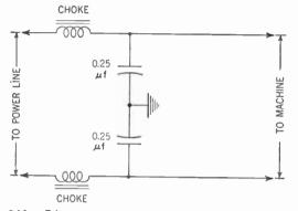
Figure 363. Filter circuit to prevent radio-frequency currents set up by a sparking machine from traveling back into the power lines.
