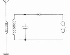
Figure 53. Diagram showing crystal detector and phones substituted for the loop of wire.
