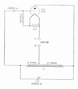
$L_1$  is 25 turns of No. 14 double-cotton-covered wire on a cardboard tube 3 in. in diameter.
