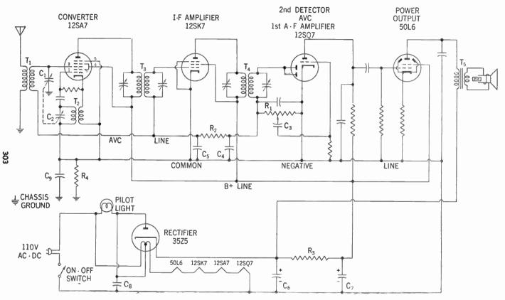
Figure 202. Circuit diagram of a typical ac-dc superheterodyne receiver.
