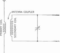
Figure 39. Diagram showing how an antenna coupler or transformer is connected in the radio receiver. Note that the path of the aerial-ground system no longer passes directly through the tuning circuit.
