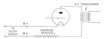
Figure 104. Circuit showing use of a dropping resistor to obtain the lower B voltage required for the plate of the detector tube.
