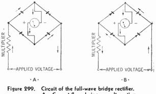
Figure 299. Circuit of the full-wave bridge rectifier. A-Current flow during one alternation. B-Current flow during the next alternation.
