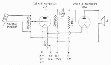
Figure 94. Diagram showing circuit of the electrical phonograph.
