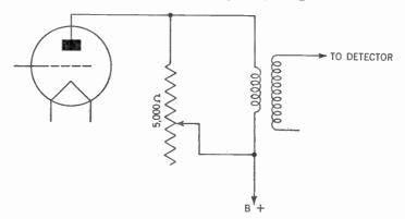
Figure 143. Circuit showing how a rheostat connected across the primary of the last radio-frequency transformer is used as a volume control.
