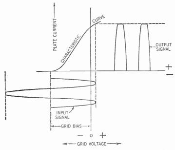
Figure 437. Graph showing how plate current goes up as the grid bias approaches zero.
