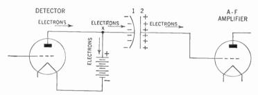
Figure 88. Diagram showing how a fixed capacitor is used to couple the amplifier tube to the detector.
