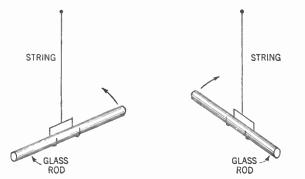
Figure 204. How two glass rods that have been rubbed with a silk cloth repel each other.
