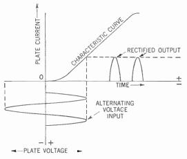
Figure 396. How the characteristic curve of the diode is used to show the relationship between the voltage input and the current output.
