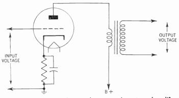
Figure 166. Diagram showing what is meant by a stage of amplification.
