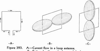
B—Pattern for the vertical arms of the loop. C—Pattern for the horizontal arms of the loop.
