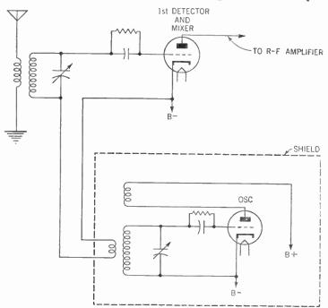
Figure 158. Circuit showing how current from the local oscillator is inductively coupled to the first detector and mixer circuit. The dotted lines showing that both variable capacitors are connected to each other are omitted from this diagram for the sake of clarity.
