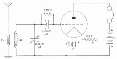
Figure 73. Diagram of the complete receiving set using the triode as a detector. The symbol 2 MEG, over the grid leak stands for 2 megohms. The symbol  $30\Omega$  over the rheostat stands for 30 ohms.
