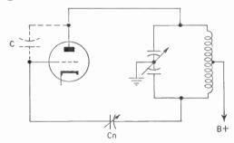
Figure 431. Circuit of a radio-frequency amplifier showing the neutralizing capacitor ( $C_n$ ). This is an example of plate neutralization.
