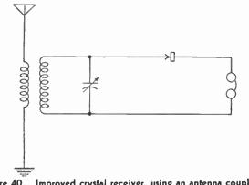
Figure 40. Improved crystal receiver, using an antenna coupler. This set will tune sharper than that of Figure 22.
