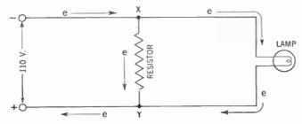
Figure 215. The parallel circuit. Here the electrons have more than one path to follow.
