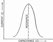
Figure 328. Graph showing the effect on the current (I) as the capacitance of the variable capacitor of Figure 327 is changed. The inductance and frequency are kept constant.
