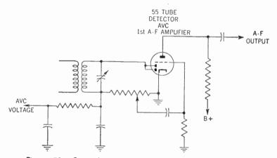
Figure 150. Circuit showing how the type 55 tube is used as a detector, automatic volume control, and first audio-frequency amplifier.
