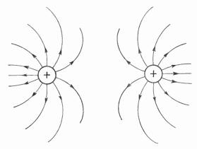
Figure 228. Lines of force between two similar charges.
