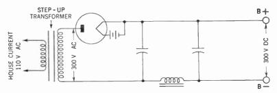
Figure 98. B-battery eliminator using a step-up transformer.
