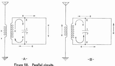
sure 52. Parallel circuits. A—Flow of electrons during a half cycle. B—Flow of electrons during the next half cycle.
