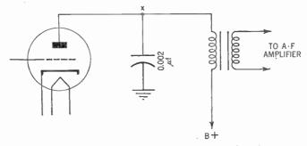
Figure 151. Circuit showing how a capacitor is used to filter out some of the high-frequency current.
