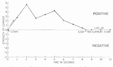
Figure 25. Graph showing curve or wave form of a fluctuating direct current. Note that the current strength may assume different values at different times.
