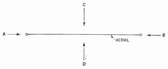
Figure 198. Diagram showing why signals from directions A and B will be heard louder than signals from directions C and D. The radio waves coming from A and B set up a difference of electrical pressures in the aerial.
