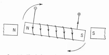
Figure 248. Now the direction of current flowing into the electromagnet is reversed. This reverses the poles of the electromagnet and, since now like poles are facing each other, the electromagnet is again rotated in a clockwise direction.
