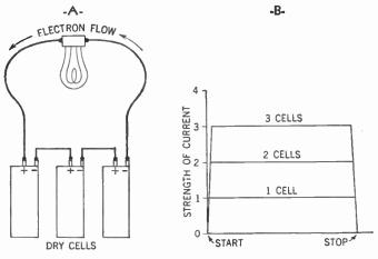
Figure 43. A—Three dry cells connected in series. B—Graph showing flow of current from one, two, and three dry cells, respectively.
