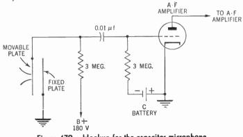
Figure 479. Hookup for the capacitor microphone.
