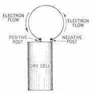
Figure 42. The dry cell is a sort of pump sending electrons streaming from the negative post to the positive post when a path is furnished.
