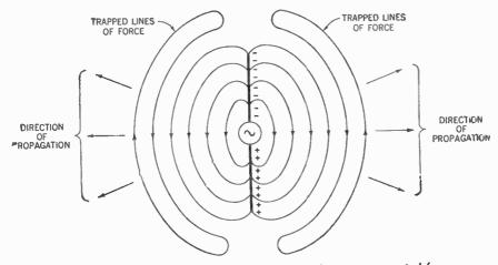
Figure 353. Diagram showing how lines of force are prevented from returning to the antenna.
