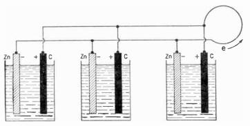
Figure 220. Three voltaic cells in parallel.
