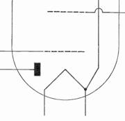
Figure 185. The 1H5-G tube. One diode—one triode.
