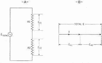
Figure 322. A—Circuit containing two resistors (R<sub>1</sub> and R<sub>2</sub>) in series. The voltage drop across each (E<sub>R1</sub> and E<sub>R2</sub>), when added together, will give the total voltage (E) of the circuit.
