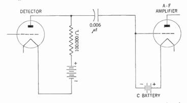
Figure 90. Diagram showing how the C battery is connected in the grid circuit of the amplifier tube.
