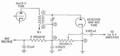
Figure 149. The complete AVC circuit.
