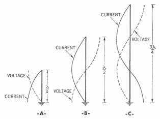
Figure 373. Marconi-type antennas of different lengths. A-Quarter wave. Note that the voltage node is at the
