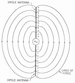
Figure 352. Diagram of the dielectric field around a dipole antenna.
