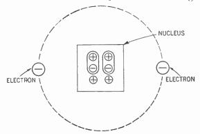
Figure 207. The helium atom, showing two electrons revolving around the nucleus. The nucleus contains two protons and two neutrons. The positive charge of the nucleus is just balanced by the two electrons. Hence, the atom has a neutral charge.
