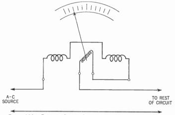
Figure 293. Diagram showing how the dynamometer type of meter is hooked into the circuit to read alternating current.
