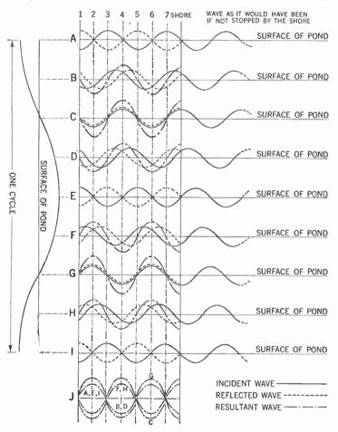
Figure 368. A to I—Diagram showing how standing waves are set up in water. Each section of the diagram is an eighth of a cycle later than the preceding one.
