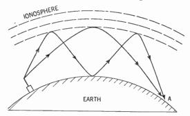
Figure 365. Another cause of fading. Here two sky waves arrive at the same point (A) out of step.
