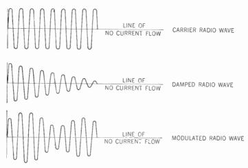
Figure 28. Graphs showing the wave forms of a continuous, damped, and modulated radio wave. Note that in all three waves shown here the frequencies are the same. Only the amplitudes vary.
