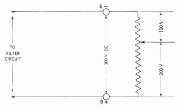
Figure 103. Diagram showing how a potentiometer is hooked up as a voltage divider.
