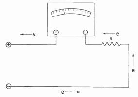
Figure 258. Circuit showing how the galvanometer is used to measure the electric current flowing through a resistor (R)
