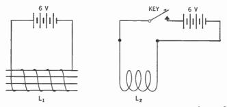
$L_1$  corresponds to the field coil of the dynamic speaker. It consists of about 300 turns of bell wire wound on a soft iron core and it is held in a fixed position.  $L_2$  corresponds to the voice coil of the dynamic speaker. It consists of about 30 turns, air wound, with a diameter of about 1 in. It is suspended so that it is free to move.
