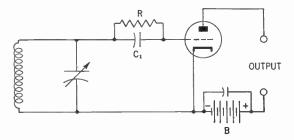
Figure 435. A class C amplifier is hooked across the simple oscillatory circuit.
