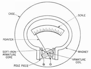
Figure 257. Diagram of the moving-coil or D'Arsonval galvanometer.
