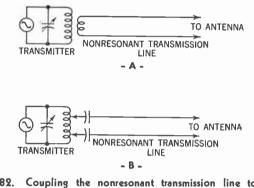
Figure 382. Coupling the nonresonant transmission line to the transmitter. A—Inductive coupling. B—Capacitive coupling.
