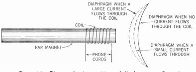
Figure 16. Diagram showing positions of diaphragm as a fluctuating current flows through the electromagnet of the phones. The bending of the diaphragm is greatly exaggerated in this drawing.
