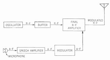
Figure 477. Block diagram showing the relationship of the components of a radio-telephone transmitter (high-level modulation).
