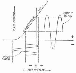
Figure 411. Distortion of the signal due to overloading.
