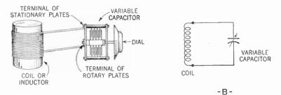
Figure 13. Hookup showing how coil and variable capacitor are connected to form the tuning circuit. Figures A and B are identical, A being the pictorial method of showing the circuit, whereas B is the schematic method using symbols.
