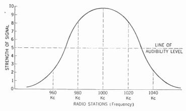
Figure 35. Graph or tuning curve showing what happens when a receiver tunes broadly. Note that unwanted radio stations at 980 and 1020 kc come in well above the line of audibility level. This means that three stations may be heard at the same time.
