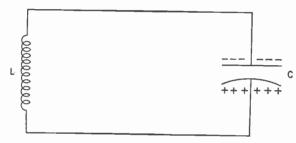
Figure 434. A simple oscillatory circuit.
