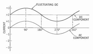
Figure 289. Curves showing how a fluctuating direct current may be broken down to its steady d-c component and its a-c component.
