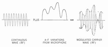
Figure 470. How the voice currents in the microphone circuit modulate the carrier wave.
