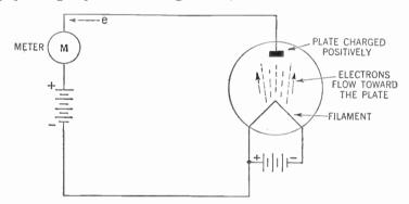
Figure 57. Fleming's experiment with a positive charge on the plate of the tube. The meter showed that an electric current was flowing through it.
