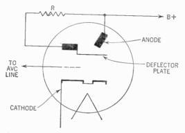
Figure 490. How the triode and tuning eye are connected in one envelope.
