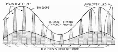
Figure 55. Graph showing how the capacitor levels off the peaks and fills in the hollows between the pulses of direct current coming from the detector. Note that the resulting curve resembles the envelope quite closely.
