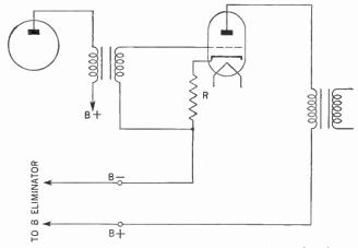
Figure 114. Circuit showing how a bias resistor (R) is used to obtain grid bias.
