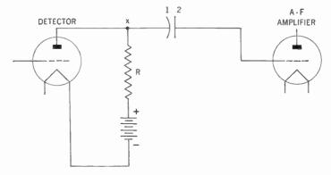
Figure 89. Diagram showing how plate resistor (R) is placed in the circuit.
