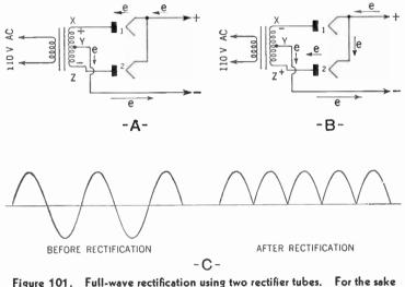
Figure 101. Full-wave rectification using two rectifier tubes. For the sake of simplicity, the complete filament circuits and the circles in the tube symbols are omitted. A—Electron flow during one half cycle. B—Electron flow during the next half cycle.
