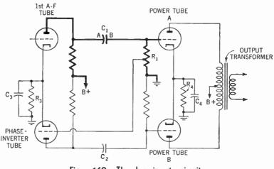
Figure 169. The phase-inverter circuit.
