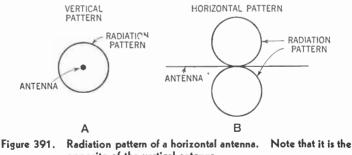
Figure 391. Radiation pattern of a horizontal antenna. Note that it is the opposite of the vertical antenna. A—Vertical pattern. B—Horizontal pattern.
