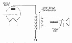
Figure 122. Diagram showing how a step-down transformer (output transformer) is used to couple the voice coil of the permanent-magnet dynamic speaker to the plate circuit of the second audio-frequency tube.
