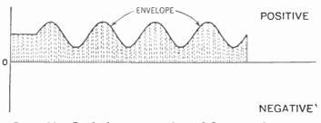
Figure 33. Graph showing wave form of fluctuating direct current through the phones. This wave form is indicated by the envelope. Note that the envelope has the same shape as the fluctuating direct current from the microphone in Figure 29-A.
