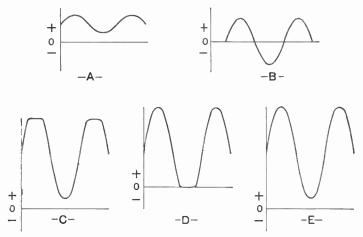
Figure 86. Graphs showing effects of grid bias.
