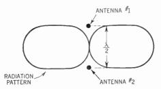
Figure 387. The horizontal pattern of two vertical half-wave antennas, a half wave apart, with their currents in phase.
