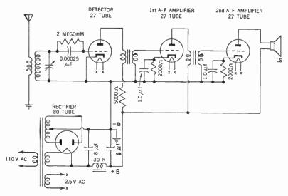
Figure 116. Diagram showing the circuit of an all-electric receiving set.
