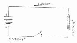
Figure 49. Hookup of coil, key, and battery to illustrate self-induction.
