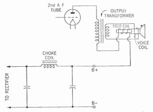
Figure 124. Diagram showing how current is obtained from the power supply to operate the field coil of the electromagnetic dynamic speaker.
