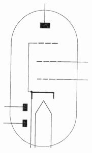
Figure 190. The 2A6 tube (two diodes—one triode).
