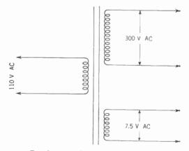
Figure 100. Transformer with two secondaries to step up the voltage for the plate supply and to step down the voltage for the filament of the rectifier tube.
