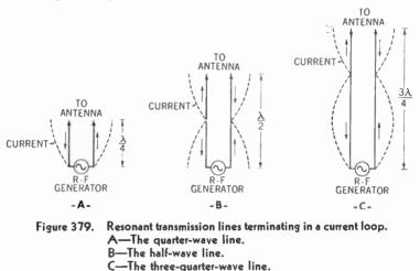
transmission line has current nodes at each end, but the other has current loops. What determines whether we have a node or loop at the ends?
