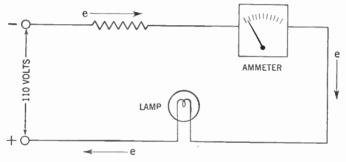
Figure 214. The series circuit. Electrons can follow only one path from negative to positive.
