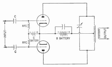
Figure 447. The push-pull radio-frequency amplifier.
