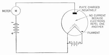
Figure 58. Fleming's experiment with a negative charge on the plate of the tube. The meter showed that no electric current was flowing through it.
