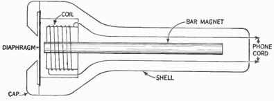
Figure 15. Construction of a telephone receiver.
