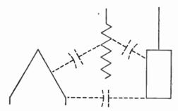
Figure 131. Diagram showing the capacitive effect existing between the electrodes of the triode. The result is the same as if small capacitors were connected between the electrodes.
