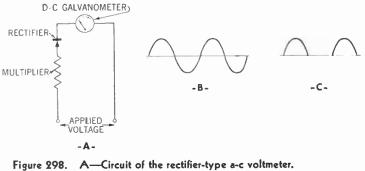
ure 298. A—Circuit of the rectifier-type a-c voltmeter. B—Wave form of the applied voltage. C—Wave form of the voltage entering the galvanometer.
