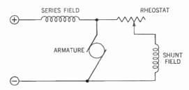
Figure 256. Hookup showing how a rheostat (R) is used to vary the speed of the compound motor.
