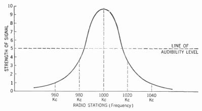
Figure 36. Graph or tuning curve for a sharply tuning receiver. Note that all unwanted radio stations fall below the line of audibility level.
