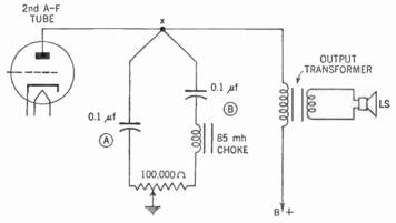
Figure 153. Circuit showing a treble-bass tone control.
