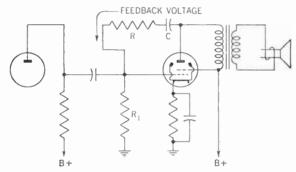
Figure 423. Circuit showing inverse feedback in the audio-frequency amplifier. The values of R and  $R_1$  determine the amount of feedback.
