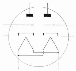
Figure 187. The 6C8-G tube (two triodes).
