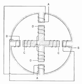
Figure 253. A four-pole motor with two sets of field and armature windings.
