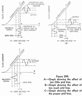
Figure 399-C shows the correct grid bias to be used for the amplifier tube. It is neither too large nor too small. The output closely resembles the input signal. You will notice that we operate on the straight-line portion of the curve.
