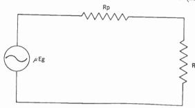
Figure 418. The equivalent circuit for an amplifier.
