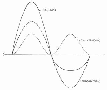
Figure 409. Graph showing the effect of adding the fundamental to the second harmonic which is above the X axis.
