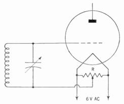
Figure 108. Circuit showing the use of a 20- to 40-ohm center-tapped resistor (R) to reduce hum.
