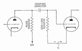
Figure 422. Resistance coupling for audio-frequency amplification.
