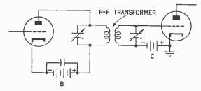
Figure 430. Circuit of a transformer-coupled radio-frequency amplifier.
