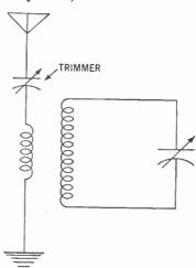
Figure 138. Use of trimmer capacitor to adjust the aerial to the radio receiver.
