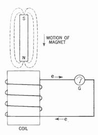
50 turns of wire wound in the shape of a cylinder about 2 inches in diameter. Now plunge the north end of a permanent magnet into the
