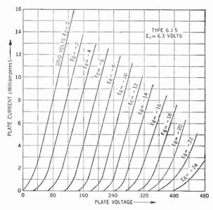
Figure 401. Family of plate characteristic curves for the 6J5 triode.
