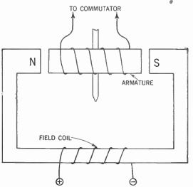
Figure 250. Diagram showing how an electromagnet is used to supply the field of a motor.
