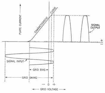
Figure 415. Graph showing relationship between the input and output signals in a class B amplifier.
