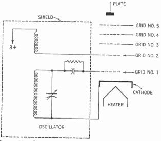
Figure 182. Circuit showing how cathode, grid No. 1, and grid No. 2 of the pentagrid converter are used as a triode for the oscillator section of the superheterodyne receiver.
