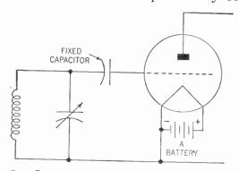
Figure 71. Diagram showing how a fixed capacitor is connected to place a negative charge, or bias, on the grid of the triode.
