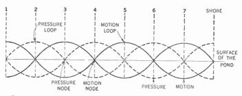
Figure 369. Diagram showing standing waves of pressure and motion in water.
