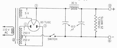
The power transformer should be able to deliver about 250 v on either side of the center tap. The rectifier tube is a type 80. The filter capacitors are 8  $\mu$ f at 450 v direct-current working voltage. The choke is an ordinary 30-henry choke coil. The voltage divider is 15,000 ohms rated at 25 w. Connect a 2-watt split-plate neon lamp in series with a magnetic speaker and test as follows:
