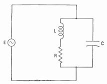
Figure 336. The parallel resonant circuit. The resistance is usually found in the inductive branch of the circuit.
