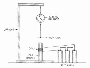
Figure 14. Apparatus used to show that a varying electric current passing through an electromagnet will exert a varying pull on an iron disk.
