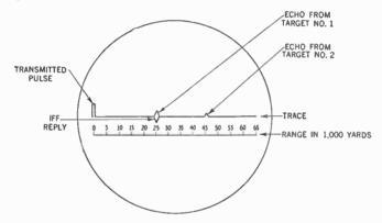
Figure 502. Trace showing two targets, one of which (the nearest) is friendly, as indicated by the IFF reply.
