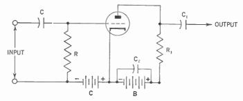
Figure 428. A stage of resistance-coupled audio-frequency amplification.
