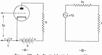
Figure 405. A—Circuit of the triode as an amplifier. B—The equivalent circuit of A.
