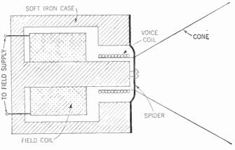
Figure 123. Diagram of an electromagnetic dynamic speaker. The field coil replaces the permanent magnet of the PM dynamic speaker.
