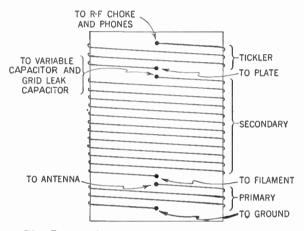
Figure 79. Diagram showing construction and connections of the threecircuit tuner.
