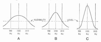
Figure 127. A—Tuning curve with one tuned circuit. Notice that stations at 990 kc and 1,010 kc are heard when the set is tuned to 1,000 kc.
