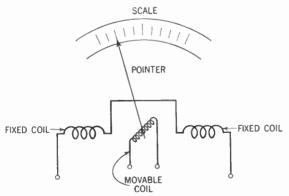
Figure 292. Diagram of the dynamometer principle.
