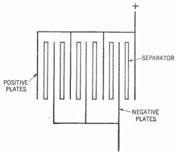
Figure 224. The lead-acid storage cell showing how the plates are hooked up.
