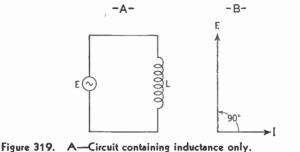
B—Vector diagram showing current (I) lagging 90° behind voltage (E).
