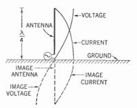
Figure 372. The quarter-wave Marconi antenna, showing current and voltage distribution. Note that this antenna corresponds to the halfwave Hertz antenna. Only half the current and voltage waves is shown here for the sake of simplicity.
