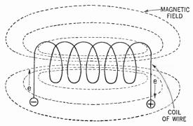
Figure 241. The magnetic field around an electromagnet.
