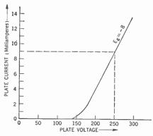
Figure 404. Plate-current — plate-voltage characteristic curve for the 6J5 triode. Grid bias is —8 volts.
