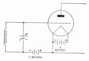
Figure 70. Diagram showing how a C battery is connected to place a negative charge, or bias, on the grid of the triode. The completed diagram would include the earphones and B battery connected as in Figure 66.
