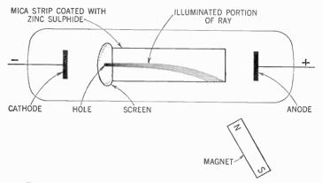
Figure 485. How the electron stream is deflected by a magnet.
