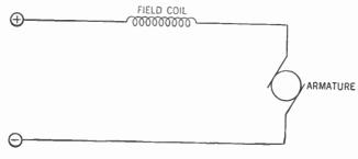
Figure 252. Hookup of a series motor.
