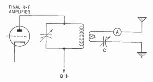
Figure 453. Method of coupling the final radio-frequency amplifier to a Marconi antenna.
