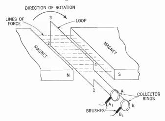
Figure 271. A simple alternating-current generator. It consists of a single loop of wire rotating in the magnetic field between two poles of a . magnet.
