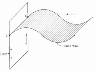
Figure 199. Loop with flat side facing the oncoming radio wave. Since the flows of electrons in the two vertical parts are equal in strength and opposite in direction, they cancel each other out.
