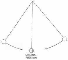
Figure 48. Diagram of pendulum illustrating oscillatory motion.
