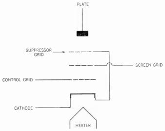
Figure 176. Arrangement of electrodes in the pentode tube.
