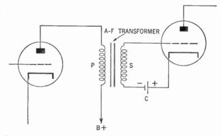
Figure 421. How the audio-frequency transformer is used to match the output of one tube with the input of the next.
