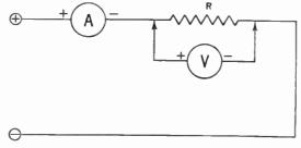
Figure 262. The voltmeter-ammeter method of finding the resistance of R.
