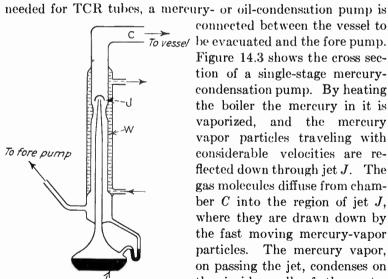
Fig. 14.3.—Single-stage condensation pump.
