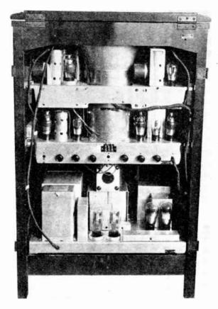
Fig. 1.23.—(b) Television receiver, rear view.
