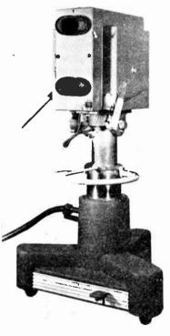
Fig. I.8.—Iconoscope camera.
