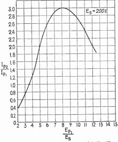
Fig. 9.22.—Variation of  $I_{p^2}/I_{p^1}$  with  $E_{p^1}/E_s$ .
