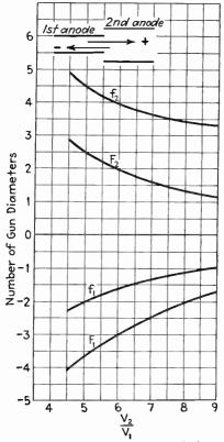
Fig. 6.14.—Optical constants vs. voltage ratio for  $d_2/d_1 = 1.5$ .
