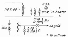
Fig. 9.23.—Circuit for cathode activation.
