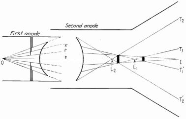
Fig. 7.3.—Imaging in the presence of spherical aberration.
