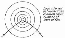
Fig. 10.7.—Magnetic field of two bar magnets.
