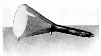
Fig. 11.7.—Experimental tube for determination of willemite potential.
