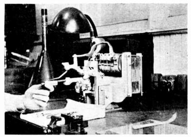
Fig. 14.9.—Photograph of a 1-kw. spot-welder.
