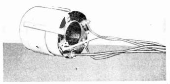
Fig. 13.32.—Improved magnetic deflecting yoke with air-core windings enclosed in iron tube.
