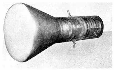
Fig. I.29.—Photograph of a 9-in. image tube.
