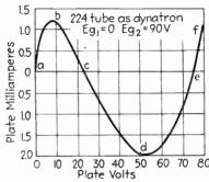
Fig. 13.5.—Dynatron characteristics of 224 tube.
