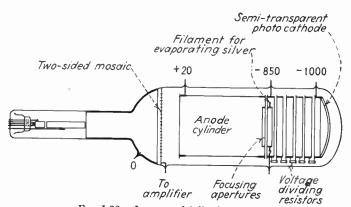
Fig. I.32.—Image-multiplier iconoscope.
