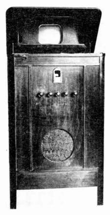
Fig. I.23.—(a) Television receiver, front view.
