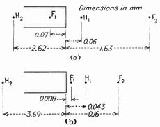
Fig. 6.20.—(a) cardinal points of immersion lens of Fig. 6.19(A). (b), cardinal points of immersion lens of Fig. 6.19(B).
