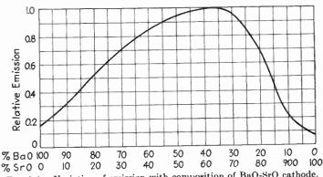
Fig. 2.4.—Variation of emission with composition of BaO-SrO cathode.
