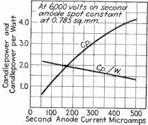
Fig. 11.3.—Luminescent efficiency of green willemite as a function of current.
