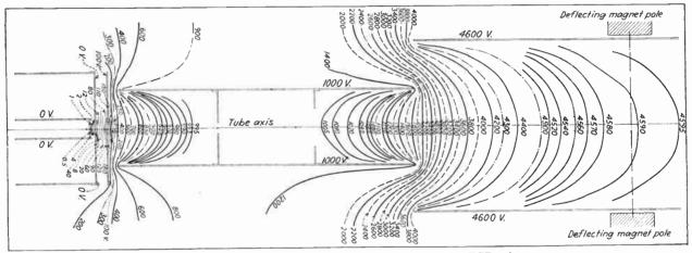
Fig. 4.1.—Electrode system and equipotential lines of a TCR tube.
