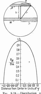
Fig. 9.18.—Distribution of ning line of a deflected circular spot of uniform intensity.
