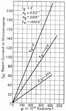
Fig. 9.12.—Variation of  $I_{p2}$  with  $\varphi$  for three values of  $E_{\varrho}$ .
