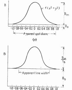
Fig. 9.19.—Distribution of intensity; (a) along diameter of stationary spot, (b) along width of scanning line.
