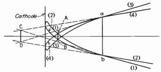
Fig. 6.21.—Beam crossover in proximity of cathode.
