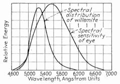
Fig. 11.1.—Spectral characteristic of green willemite.
