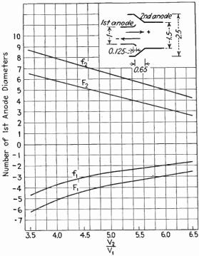
Fig. 6.9.—Variation of optical constants with voltage ratio.
