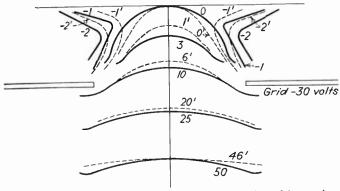
Fig. 7.13.—Effect of space charge on potential distribution of immersion lens.
