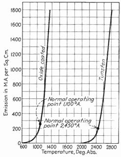
Fig. 2.3.—Variation of emission with absolute temperature.
