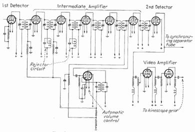
Fig. I.22.—Receiver picture channel.
