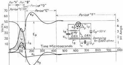
Fig. 13.17.—Detailed performance of blocking oscillator.
