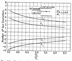
Fig. 6.7.—Variation of optical constants with voltage ratio.
