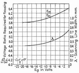
Fig. 9.20.—Variation of  $\lambda$  and  $E_{p2}/E_{p1}$  with  $E_{q}$ .
