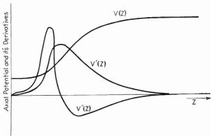
Fig. 4.3.—Axial distribution of potential and its derivatives.
