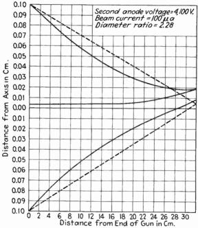
Fig. 7.17.—Effect of space charge on paraxial electron trajectories in image space.
