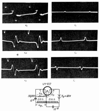
Fig. 13.18.—Oscillographic study of performance of blocking oscillator with constants shown.
