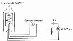
Fig. 14.6.—Connections for thermocouple gauge.
