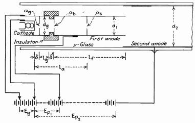
Fig. 9.1.—The electron gun.
