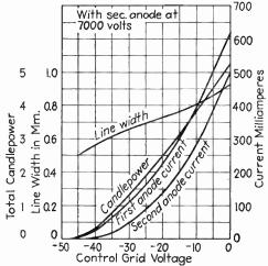
Fig. 12.9.—Operating characteristics of TCR tube.
