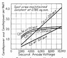
Fig. 11.2.—Luminescent efficiency of green willemite as a function of voltage.
