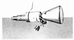
Fig. 12.3.—Five-inch TCR tube with magnetostatic focusing and all-magnetic deflection.
