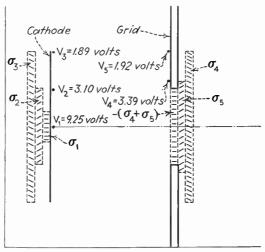
Fig. 7.15.—Approximate distribution of charge induced on cathode and grid by beam.
