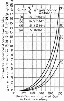
Fig. 7.6.—Transverse spherical aberration vs. beam diameter.
