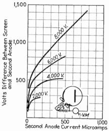
Fig. 11.6.—Secondary-emission characteristics of willemite on a platinum screen.
