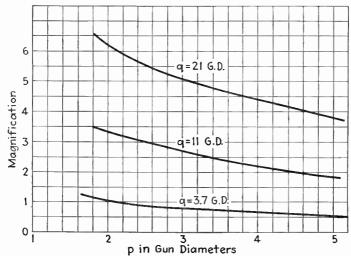
Fig. 6.15.—Magnification vs. object distance for  $d_2/d_1 = 1.5$ .
