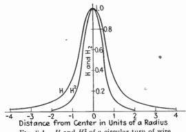
Fig. 8.4.—H and  $H^2$  of a circular turn of wire.
