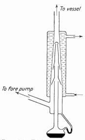
Fig. 14.4.—Triple-stage mercury-condensation pump.
