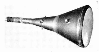
Fig. 12.1.—Nine-inch TCR tube for all-electric deflection.
