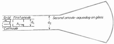
Fig. 6.1.—Cross section of a TCR tube.
