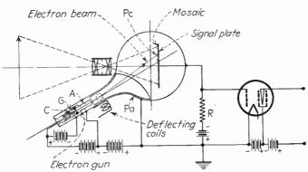
Fig. I.6.—Iconoscope and its circuit.
