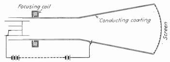
Fig. 1.35.—Magnetostatic electron microscope.
