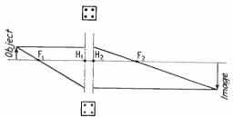
Fig. 8.1.—Focusing with a short coil.
