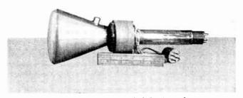
Fig. I.4.—TCR tube with deflecting yoke.
