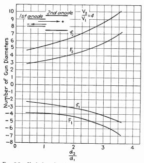
Fig. 6.8.—Variation of optical constants with diameter ratio.
