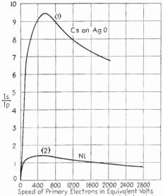
Fig. 2.5.—Secondary emission of Cs on AgO and Ni surfaces.
