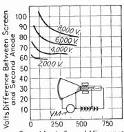
Second Anode Current Microamps Fig. 11.8.—Secondary-emission characteristics of willemite on Pyrex glass screen.
