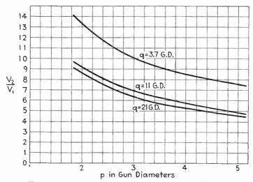
Fig. 6.16.—Voltage ratio vs. object distance for  $d_2/d_1 = 1.5$ .
