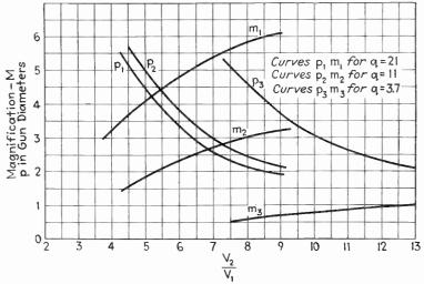
Fig. 6.13.—Magnification and object distance vs. voltage ratio.
