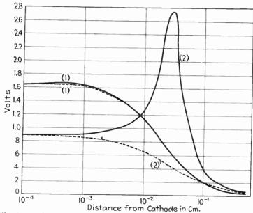
Fig. 7.14.—Curve (1), potential distribution along axis due to a disk of charge located near cathode. Curve (2), potential distribution along axis due to charges induced on cathode by disk. Curve (2)', potential produced by the charges induced on cathode by the cylinder of charge producing curve (2).
