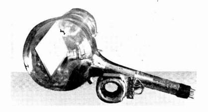
Fig. I.7.—Iconoscope with deflecting yoke.
