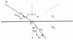
Fig. 3.1.—Electron refraction and reflection at plane surface.
