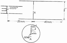
Fig. 7.4.—Gun useful in determination of spherical aberration.
