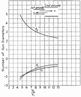
Fig. 6.18.—Position and focal lengths of thin lens vs. voltage ratio.
