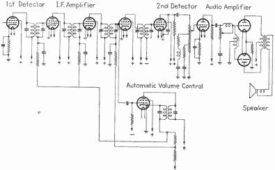
Fig. I.21.—Receiver sound channel.
