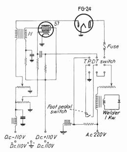
Fig. 14.10.—Circuit of a thyratron-controlled welder.
