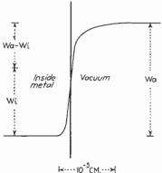
Fig. 2.2.—Potential barrier of a clean metal surface.
