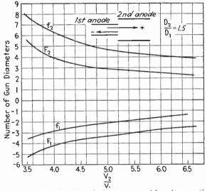
Fig. 6.6.—Variation of optical constants with voltage ratio.
