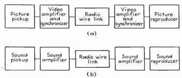
Fig. I.1.—(a) Block diagram of television-communication system. (b) Block diagram of sound-communication system.
