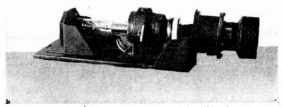
Fig. 12.6.—Typical mounting for projection TCR tube.
