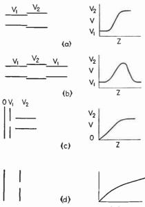
Fig. 5.3.—Types of electrostatic lenses.
