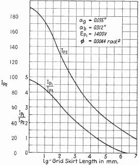
Fig. 9.17.—Variation of  $I_{p2}$  and  $I_{p1}/I_{p2}$  with  $l_g$ .
