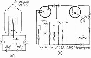
Fig. 14.7.—Ionization gauge, (a) connected with galvanometer, (b) connected with direct-current amplifier and milliammeter.
