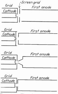
Fig. 6.22.—Electrode systems of immersion lenses used in TCR tubes.
