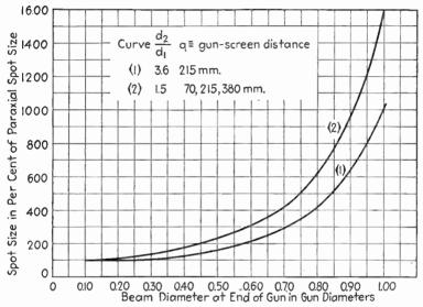
Fig. 7.9.—Minimum spot size vs. beam diameter.
