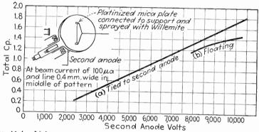
Fig. 11.4.—Light output vs. second-anode voltage for willemite on a platinized mica screen.
