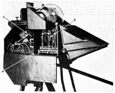
Fig. I.25.—General arrangement of parts in a television camera.
