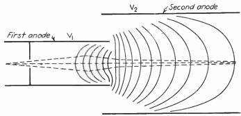
Fig. 3.2.—Equipotential line plot of two cylinders.
