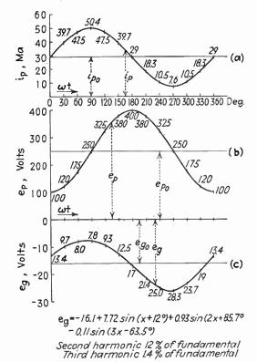
Fig. 13.28.—Inverse method applied to distortion analysis.
