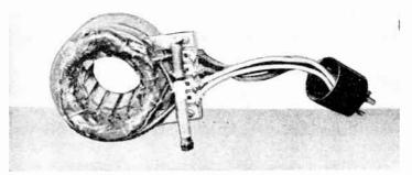
Fig. 13.31.—Improved magnetic deflecting yoke with iron core.
