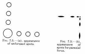
Experimentally, it is simpler to determine the transverse spherical aberration, and Fig. 7.4 shows the type of gun useful in the determination of that type of aberration. Figure 7.5(a) represents the appearance of the spots on the screen when  $V_2 = V_1$ . If there were no spherical aberration, all the spots would, on focusing, unite to form the small paraxial-image spot.
