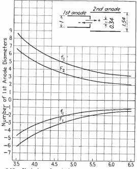
Fig. 6.10.—Variation of optical constants with voltage ratio.
