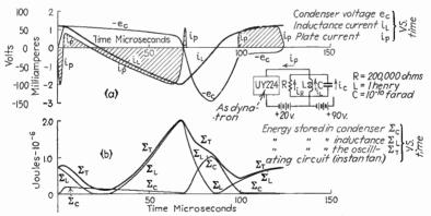
Fig. 13.6.—Detailed performance of a dynatron oscillator.
