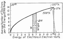
Fig. 2.1.—Distribution of energy of free electrons in nickel at 0°A, 300°A, and 1500°A.
