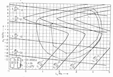
Fig. 13.14.—Isocline solution of a multivibrator.
