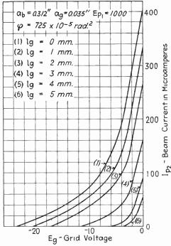
Fig. 9.16.—Variation of  $I_{F^{\ddagger}}$  with  $E_{\emptyset}$
