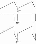
Fig. 13.22.-Voltage wave required to force a saw-tooth wave of current through (a) resistance, and inductance in series.
