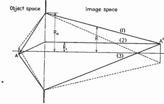
Fig. 7.16.—Paraxial electron focusing with negligible space charge.
