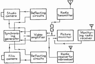
Fig. I.24.—Block diagram of television transmitter.
