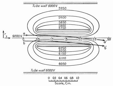
Fig. 10.10.—Symmetrical electric deflecting field.
