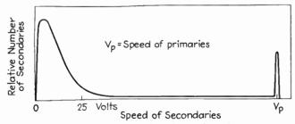
Fig. 2.6.—Speed distribution of secondary electrons.
