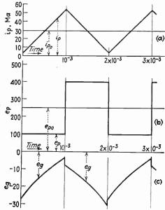
Fig. 13.30.—Inverse method applied to saw-tooth wave shape.
