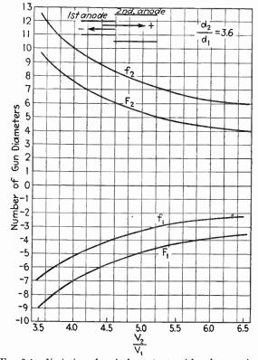
Fig. 6.4.—Variation of optical constants with voltage ratio.
