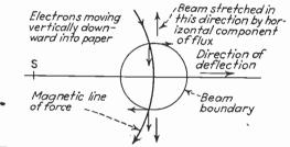
Fig. 10.8.—Beam defocusing by magnetic deflecting field.
