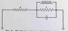
FIG. 8. Electrical equivalent of the light valve.
