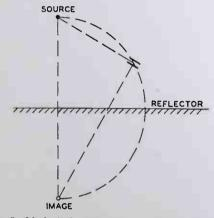
Fig. 5-Method of reducing effect of interfering waves with velocity microphone.
