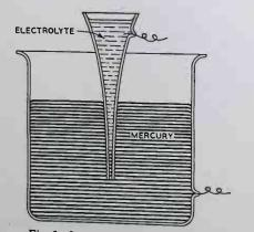
Fig. 3-Latour capillary microphone.
