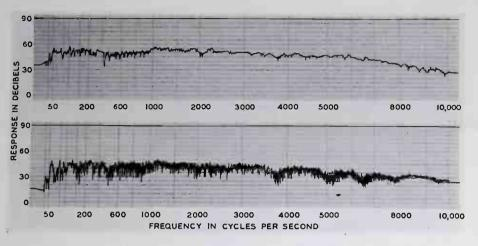
Fig. 9—Loudspeaker and microphone response curves taken at different distances in the same room.
