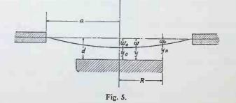
Referring to Fig. 5, if V is the potential between the plate and the diaphragm, and T, the tension of the membrane, we have
