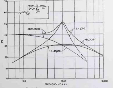
FIG. 1. Response of a simple resonant system.
