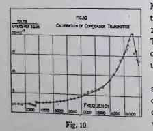
Measurements were made in this manner for frequencies from 160 to 18,000 cycles per second. The general shape of the curve obtained by plotting these values is shown in Fig. 10.
