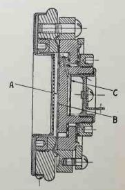
Fig. 1. Sectional view of the electrostatie transmitter.
