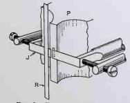
FIG. 2. The single-ribbon type of light valve; R, the ribbon; J, the aperture jaws.
