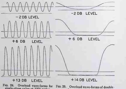
single-plane valve at 1000 cycles. Plane valve for 100 cycles.
