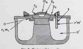
FIG. 9. Moving coil transmitter.
