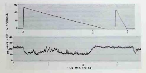
Fig. 8-Decay of an undamped and damped tuning fork, and a record of street noise.
