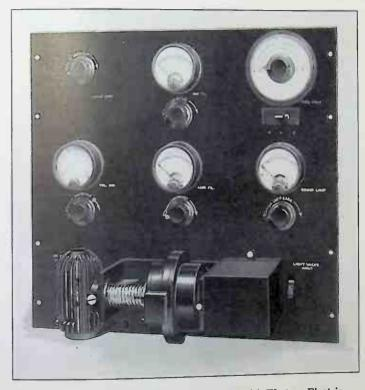
FIG. 24. Separate valve tuning unit supplied with Western Electric recording equipment.
