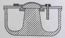
Fig. 1-Moving coil microphone.
