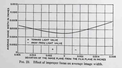
It is, therefore, apparent that either the azimuth adjustment of the light valve or the focal adjustment of the objective lens, or both, are important factors that may seriously affect the quality of reproduced sound records. If the analysis of light valve action given in Part II is to hold, the average image width assumed must be consistent with the azimuth and focus conditions.
