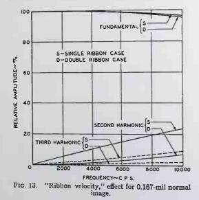
than for the double-ribbon valve, but the situation on harmonic distortion remains relatively much the same.
