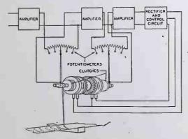
Fig. 1-Schematic drawing of level recorder.
