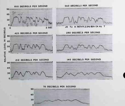
Fig. 6-Level variations in speech at different recording speeds.
