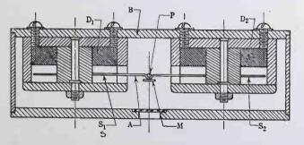
FIG. 3-SECTIONAL VIEW OF DIFFERENTIAL A-C. GALVANOMETER
