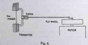
placed over the diaphragm as shown in the figure, thus forming an airtight enclosure. Connected to this was a cylinder containing a piston. The connecting rod was long compared with the stroke of the piston so that with the motor running, the piston was given practically a simple harmonic motion. The fly wheel was fairly heavy and the connecting rod was made of stiff tubing, so that but little vibration was noticeable even when the motor ran at the highest speed.
