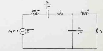
FIG. 2. Circuit diagram for receiver or transmitter.
