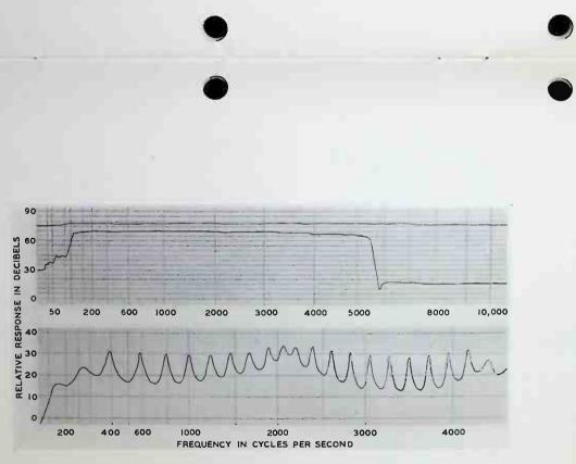
Fig. 10—Upper record: Output characteristic of heterodyne oscillator, and transmission characteristic of a 100-5500-cycle band-pass filter. Lower record: Harmonic resonance in an air column.
