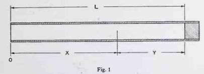
resented by  $Z_2 = R_2 + iX_2$  per unit area. Under these conditions, the pressure, p, at any point in the tube at a distance x from O, is by analogy with the electrical transmission line
