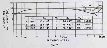
designated as 5000 instead of 10,000 c.p.s., k = 0.5, the curves will remain unchanged in form but the ordinates will be raised 6 db. The form of any of the curves of Fig. 7 will, of course, not be changed if all the corresponding constants are changed proportionally, although the absolute value of the velocity per unit of force will vary inversely with the magnitude of these constants.
