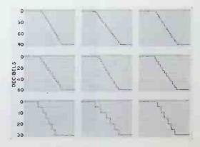
Fig. 5-Calibrations of the 30-, 60- and 90-db ranges in five db steps.
