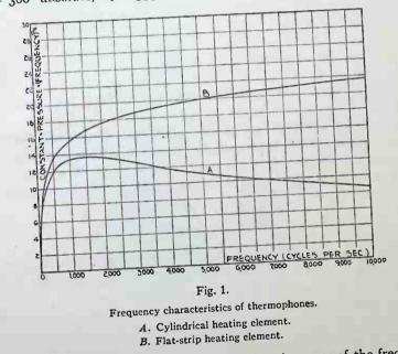
In Fig. 1 the products of pressure and the 3/2 power of the frequency are plotted as a function of frequency. The curves thus show the amount of deviation from a simple 3/2 power relation. It appears that as telephone receivers the two types of instruments produce approximately the same amount of distortion and so neither possesses an advantage in
