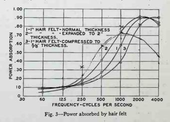
type. After measurements on several samples it was evident that concordant results could not be expected as the absorption varied considerably with the packing of the felt. This point is illustrated by the curves shown in Fig. 3. These curves were all obtained on the same piece of hair felt but with different degrees of packing. It is thus evident that a felt which has become loosened by handling may have an absorption frequency characteristic quite unlike that of a new piece.
