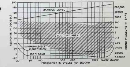
Fig. 2-Operating range of moving coil microphone.
