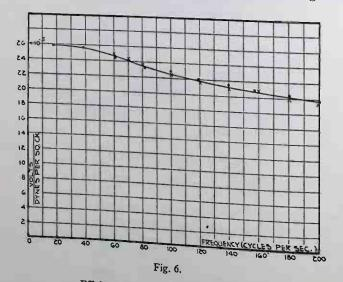
Efficiency of electrostatic transmitter. •Values obtained with the pistonphone. × Values obtained with the thermophone. Nol. XIX.
