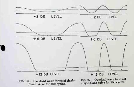
might be expected would be a simple cutting off of the negative troughs of the wave whenever the ribbons were sufficiently displaced so as to cut off all light. This assumes that, in the main, modification of the overload distortion, due to photographic considerations and due to non-linearity of valve displacement for excessive movements of the ribbon, might be neglected.
