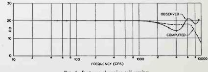
FIG. 6. Response of moving coil receiver.
