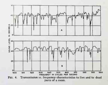
to have a characteristic as irregular as this one, we should probably conclude that the system would be incapable of transmitting speech intelligibly. As a matter of fact we should be correct in our conclusion, for this curve was taken in a room that was acoustically so reverberant that it was almost impossible to carry on a conversation between the sending and the receiving points.
