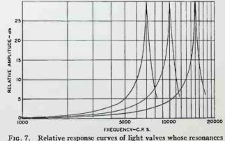
FIG. 7. Relative response curves of light valves whose resonances occur at 7000, 10,000, and 15,000 cycles.
