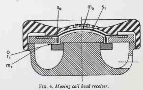
is of the self-supporting ribbon type, the construction of which has been described previously.<sup>1</sup> It is rigidly attached to the base of the domed portion of the diaphragm. The radial magnetic field is derived from a permanent magnet. The mass of the diaphragm plus that of the coil corresponds to  $m_0$  in Fig. 2, the stiffness of the diaphragm to  $s_0$  and the mechanical resistance to  $r_0$ .
