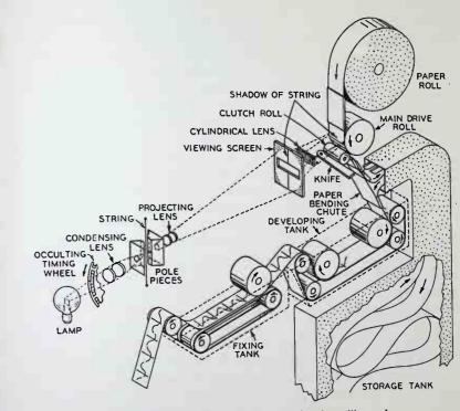
Fig. 8-Diagrammatic arrangement of Curtis oscillograph.
