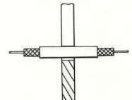
SLEEVING OVER WIRE WITH NO PRESSURE ON CHASSIS.
