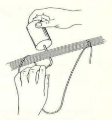
Step B. Thread tool under cable and and grasp cord near tool.
