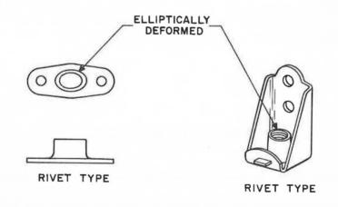
Figure 3-15. Two Lug Anchor<br/>Rivet Type All-Metal<br/>Lock NutFigure 3-16. Right Angle<br/>Rivet Type All-Metal<br/>Floating Lock Nut
