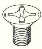
SLIVERS OR LOOSE FLAKES ON TOP OF HEAD
