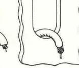
SLEEVING OVER WIRE WITH PRESSURE ON CHASSIS.
