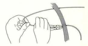
When Cutting an End of Cord, Leave 1/8 inch Outside Knot
