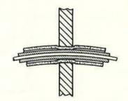
SLEEVING OVER WIRE INSTEAD OF PROTECTION ON CHASSIS. PRESSURE ON WIRE.
