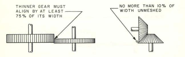
Figure 4-5. Alignment Limits for Spur Gears and for Bevel Gears
