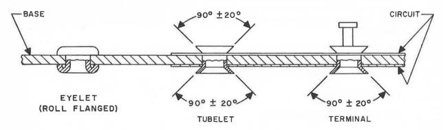
Figure 5-1. Eyelet, Tubelet and Terminal on a Board
