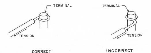
Figure 1-13. Avoiding Tension on Soldered Joint
