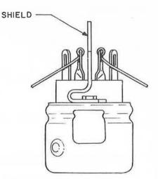
WIRES AND TERMINALS ADJACENT TO SHIELD PROPERLY POSITIONED
