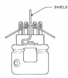
WIRES AND TERMINALS ADJACENT TO SHIELD NOT PROPERLY POSITIONED
