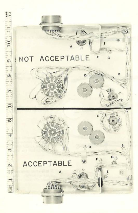
Figure 1-6. Cable Dress and Routing
