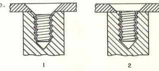
Figure 3-2B. Using Flathead Screws on a Thin Panel
