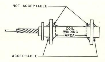
Figure 1-23. Cementing Terminals to Coil Form
