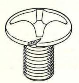
LARGE, OPEN FRACTURES EXTENDING HALFWAY OR MORE THAN HALFWAY TO THE RECESS
