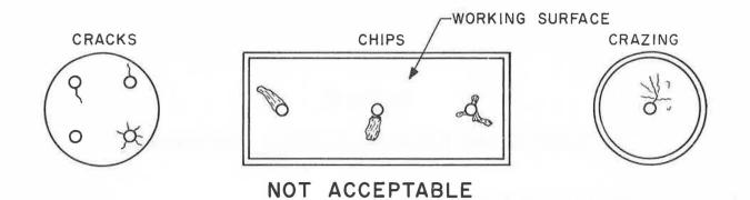
Figure 4-1. Cracks, Chips and Crazing around Sealed Terminals
