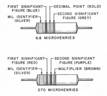
It is significant to note that there have been isolated instances when, for no apparent reason, the manufacturer has not followed this marking code. If there is any question or doubt about the value of a choke, it should be checked by actual measurement on a suitable bridge.
