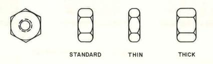
Figure 3-10. Nut Thickness
