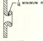
CHASSIS EXTRUDED TO PROVIDE PROPER RADIUS.
