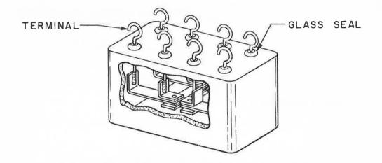
Figure 4-20. Construction of a Sealed Relay
