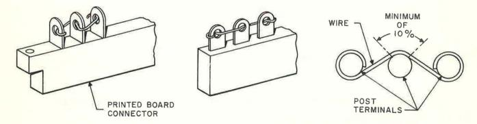
Figure 1-12. Threading Terminals with Wire
