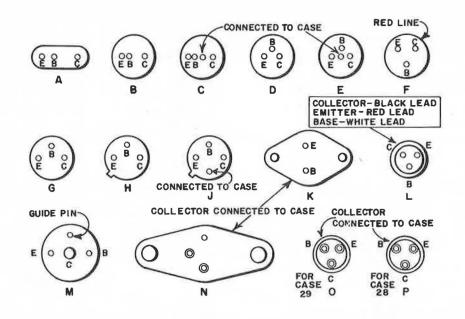
NOTE: MANY MANUFACTURERS CONNECT ONE OR ANOTHER OF THE LEADS TO THE CASE STRUCTURE, SO THE INDIVIDUAL TRANSISTOR SPECIFICATION SHEET SHOULD BE REFERRED TO BEFORE CONNECTING THE TRANSISTOR INTO A CIRCUIT, ESPECIALLY FOR BASE DIAGRAMS B, G, & H.
