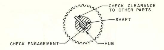
Figure 4-21. Pin Engagement and Clearance Checks
