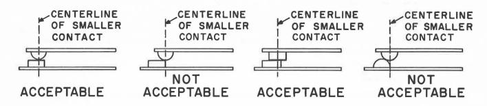
Figure 4-17. Contact Alignment for Low Current Applications
