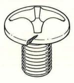
OPEN, ANGULAR FRACTURES ON EDGE OF HEAD
