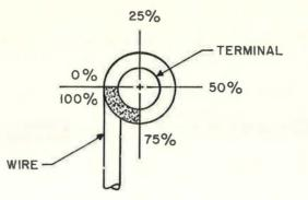
Figure 1-9. Mechanical Wrap on Post
