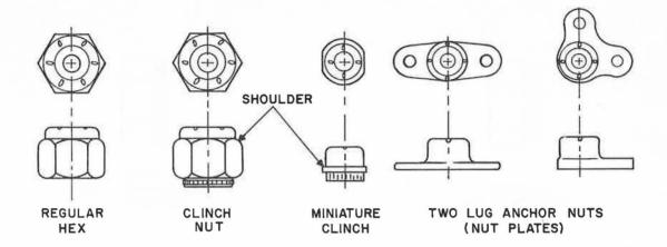
Figure 3-14. Common Elastic Stop Nuts
