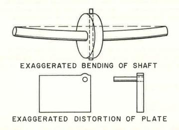
Figure 4-22. Distortion Caused by Improper Pinning
