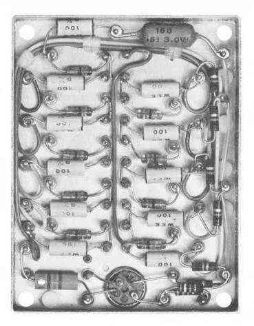
Figure 2-3. Example of Wired Assembly
