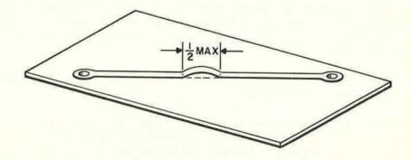
Figure 5-3. Lifted Circuitry Repairable Maximum
