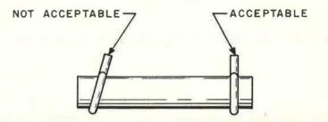
Figure 1-22. Mounting of Ring Terminals
