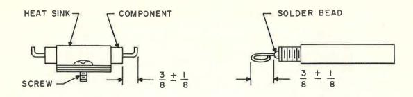
Figure 1-16. Component Leads as Terminals
