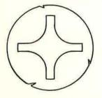
SLIGHT "FRACTURES" NOT EXTENDING HALF-WAY TO RECESS AND NOT AFFECTING USEABILITY
