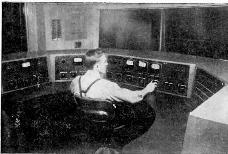
Fig. 1-1(B). The control console of Fig. 1-1(A). The master panel is in the middle with studio panels on either side.
