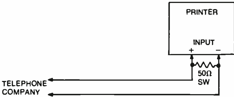
Fig. 6-8. When there is no way to adjust the signal current, add a resistor across the input of the printer to provide a shunt path for part of the signal current.
