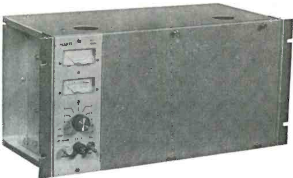
Fig. 7-14. The station may use a microwave unit instead of telephone lines for the interconnecting link. Shown is the Marti STL-8F transmitter unit, operating in the 950 MHz band.
