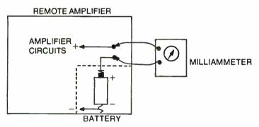
Fig. 7-11. Measure the current drain of a remote amplifier in full operation. Save the figures for later reference.
