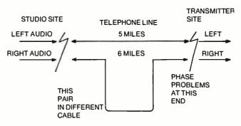
Fig. 7-12. If two audio circuits run in different cables, there can be different path lengths, which will mean phase problems in stereo.
