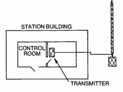
Fig. 1-1. Combined studio-transmitter arrangement. This is the simplest form and requires the least equipment.
