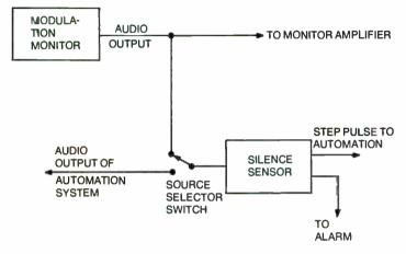
Fig. 8-5. Monitor the audio after the modulation monitor with the silence sensor.
