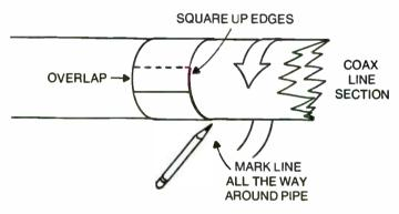
Fig. 10-6. Mark the pipe all the way around. Use a stiff piece of paper as a guide.
