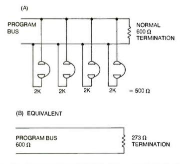
Fig. 4-18. Impedances in parallel figure the same as resistors. Here, the four earphones will cause double loading of the bus.
