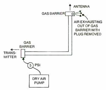
Fig. 10-9. Bleed the line by opening the plug at the end.
