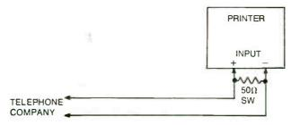
Fig. 6-8. When there is no way to adjust the signal current, add a resistor across the input of the printer to a provide a shunt path for part of the signal current.
