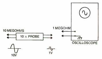
Fig. 13-3. A 10X probe on oscilloscope will provide circuit isolation, but also reduces signal amplitude to instrument.
