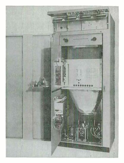
Fig. 9-20. Harris MW-1, solid-state AM transmitter with the front door and access panels open, showing the simplicity of layout and easy access for maintenance.
