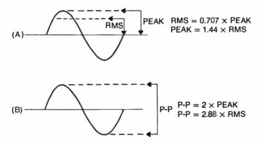
Fig. 13-2. The RMS and peak-to-peak values of a sine wave.
