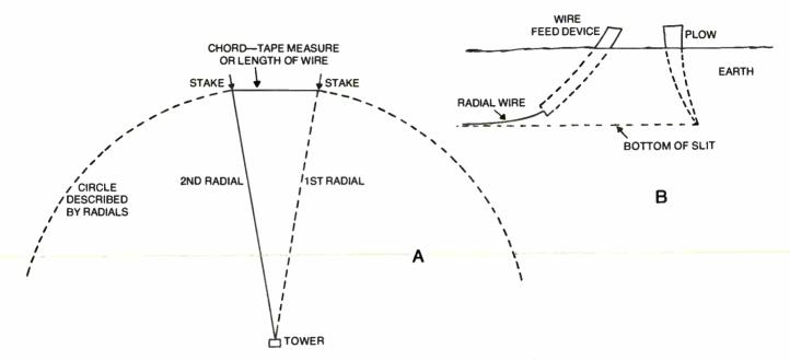
Fig. 11-2. Installing the ground system. (A) Plot out the ground system using one radial wire and either a tape measure or a wire the length of a chord to determine each terminating point. (B) Slit the soil and lay the radial wire in the bottom of the slit.
