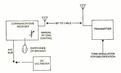
Fig. 14-10, Setup for measurement of out-of-band radiations. Depending upon how well the receiver is shielded, you may have to move away from the transmitter site up to 1 mile.
