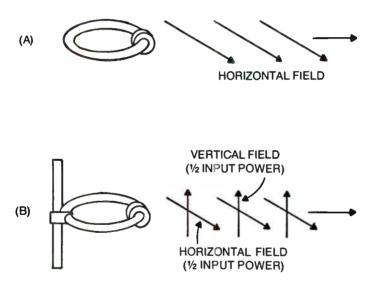
Fig. 11-3. (A) A single FM antenna bay has a power gain of 1 and radiates a horizontal field. (B) Adding vertical polarization will divide the bay input power into each field so that the gain in each field is 0.5.
