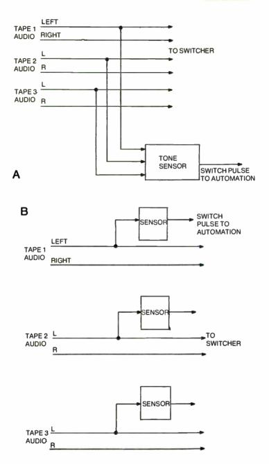
Fig. 8-3. Two different ways the control tones of music machines are handled. In A, one sensor handles all machines, and in B, each machine has its own sensor.
