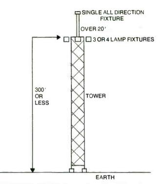
Fig. 11-6. High-intensity light system requires lights at the top of tower and at different intermediate heights on towers above 300 ft. If antenna projects above tower more than 20 feet, then an omnidirectional lamp must be used on top of the projection.
