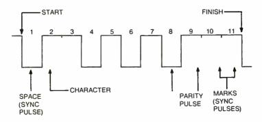
Fig. 6-7. ASCII 8-level code. The full 11-pulse group is used to define one character.
