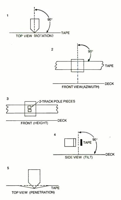
Fig. 5-16. The five conditions of head positioning which must be met in head alignment.
