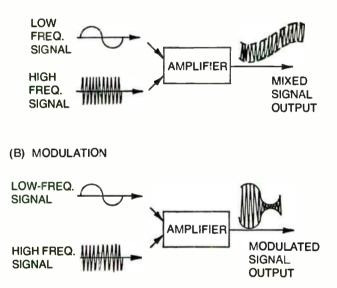
Fig. 4-14. Intermodulation distortion is a modulation process-not mixing.
