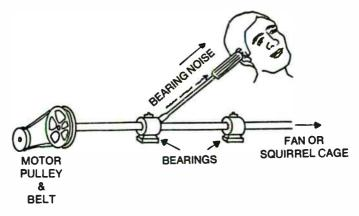
Fig. 9-10. Use a long screwdriver as a stethoscope to detect bad bearings.
