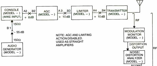
Fig. 14-4. Draw a block diagram of the equipment lineup and signal levels. Label each block and the jacks.
