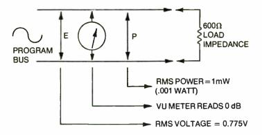
Fig. 4-2. The broadcast standard reference level is a measurement of power in a program circuit, with a specific 600-ohm load impedance. This is designated as 0 dBm (the small m means milliwatt reference).
