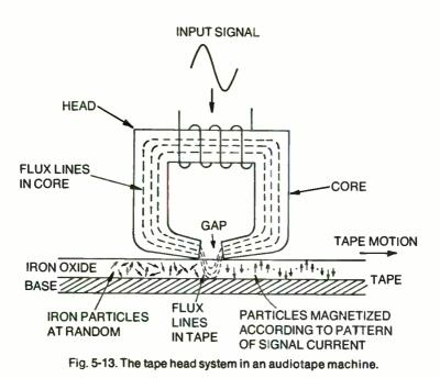
and a low-frequency portion of the tape is subjected to the signal for a longer period of time than high frequencies, and have a chance to penetrate deeper into the iron layer.
