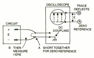
Fig. 13-7. Making DC voltage measurement with the oscilloscope. Use DC coupling and short the probe to ground for reference. Distance between zero reference and deflection of trace is directly proportional to the DC voltage.
