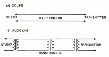
Fig. 7-13. A DC line is a metallic wire pair. An audio line might have transformers in it.
