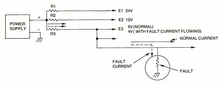
Fig. 4-15. Fault in circuit can increase current through R3, causing a higher voltage drop and lowering voltage bus E3. All circuits fed by E3 will be affected.
