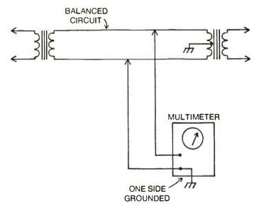
Fig. 13-5. The unbalanced input of meter can short out half of a balanced circuit. This will affect both the circuit and the readings. To avoid this, float meter case.
