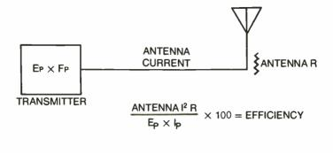
ORIGINAL: ANTENNA R = 50  $\Omega$  P = I<sup>2</sup> R = 1000W ANTENNA I = 4.47 A
