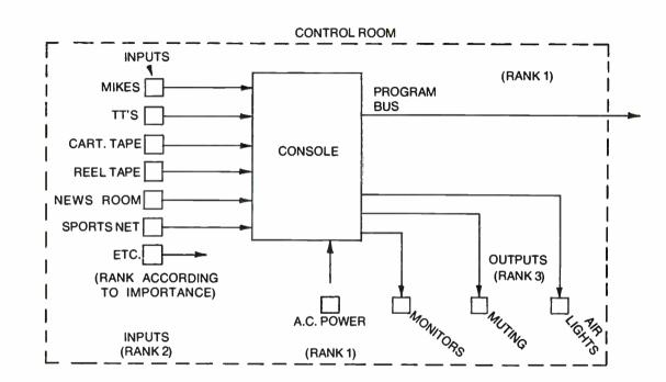
Fig. 1-8. Typical minor subsystem of the studio area. This is similar to a regular block diagram, except placement should be according to importance of role.
