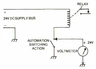
Fig. 13-11. Automation switches the "low" side of a circuit. Without current flow, the supply voltage will be measured at the "low" end of the coil.
