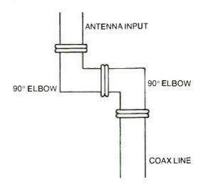
Fig. 10-4. Use two 90-degree elbows at the base of the antenna.
