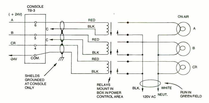
Fig. 3-2. Schematics are needed for specific sections to show the necessary installation data. Notice the information on shields, parts location, and other data. take place, it is important that the diagrams are altered at the same time, not at some later date. Making changes to the drawings as the work progresses does tend to make the drawings look a bit shop-worn, but they are accurate!
