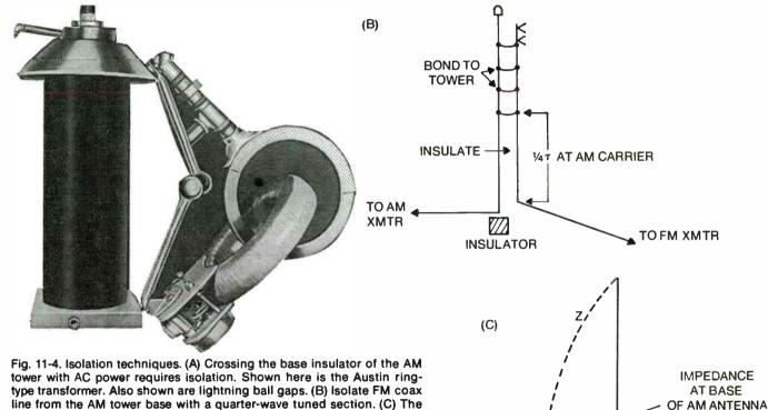
type transformer. Also shown are lightning ball gaps. (B) Isolate FM coax line from the AM tower base with a quarter-wave tuned section. (C) The quarter-wave section presents infinite impedance to the AM carrier. (Photo courtesy Harris Corporation.)
