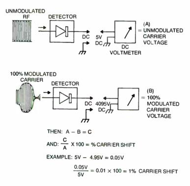
Fig. 14-9. Carrier shift is the change in rectified DC voltage out of the detector between the unmodulated and modulated-carrier conditions.
