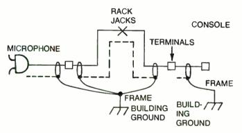
Fig. 3-9. Plan the control of shield grounding ahead of time.
