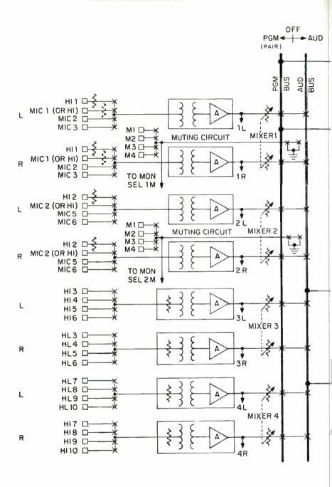
Fig. 5-2. Block diagram of the RCA BC-15 console.
