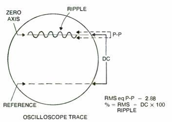
Fig. 13-8. Use the scope to measure and compute the ripple on a DC bus. Ripple must be RMS value.
