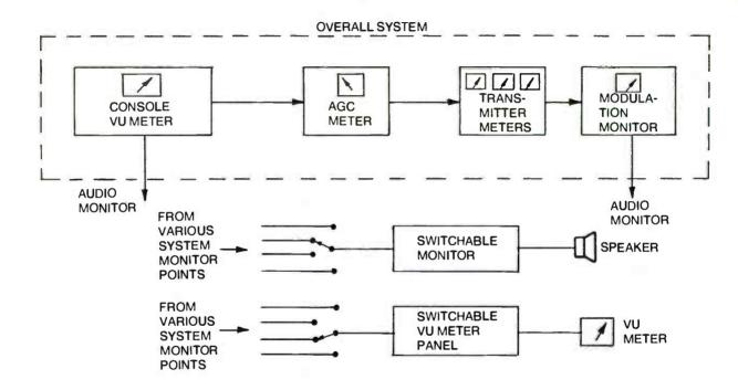
Fig. 2-13. Use the system's normal metering and monitoring when signal tracing.
