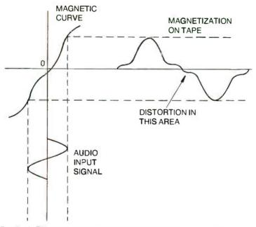
Fig. 5-14. Effects of the magnetic properties of the head and tape cause distortion near the zero-crossing line.
