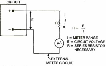
Fig. 13-6. When adding a panel meter to make a voltmeter, add enough series resistance to limit current through meter and drain from circuit. Use Ohm's law to figure resistance.
