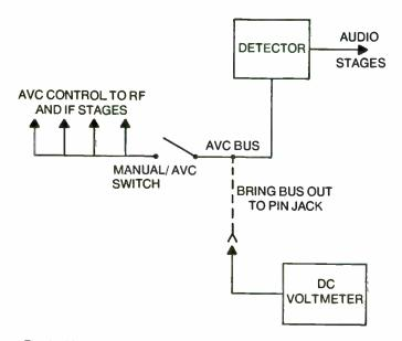
Fig. 14-11. Modify the receiver so that AVC bus can be measured.
