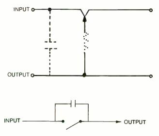
Fig. 4-16. Oxidation on jack "normal" contacts can create high series resistance and form a small capacitor. This is equivalent to an open circuit with a small capacitor across it. Only the very high audio frequencies will get through. This additional 1% will add to the system's total distortion, and this may push the system out of FCC tolerances, even though that 1% would not be discernible by itself.
