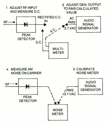
Fig. 14-13. To measure AM noise on FM carrier: (1) Measure DC output of the peak detector. (2) Compute 0.707 of this DC value and set output of signal generator to this value. (3) Use this AC signal to calibrate the noise meter. (4) Connect calibrated noise meter to detector to measure any modulation components on carrier. For example shown, RF was adjusted to obtain 3V.
