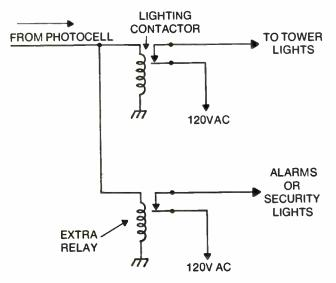
Fig. 12-6. Check other relays that may operate from the photocell.
