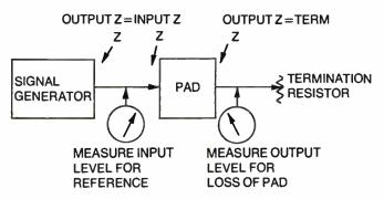
Fig. 4-21. Test setup to measure loss value of homemade pad.
