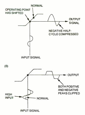
Fig. 4-12. Two ways amplitude distortion can occur: In A, stage operating point has changed on its input-output curve, causing output to be non-linear. In B, input signal is too high, causing stage to be driven into clipping.
