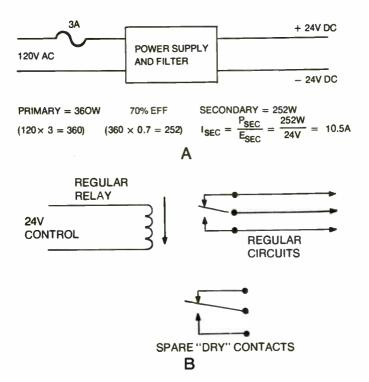
Fig. 5-5. Modifications to console. (A) Method of roughly calculating the maximum lead current of a power supply. (B) "Dry" contacts have no other circuits connected to them.
