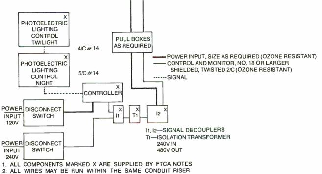
3. WIRING MAY BE RUN IN ANTENNA MAST-6 INDIVIDUAL CONDUCTORS
