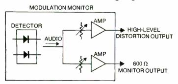
Fig. 14-12. The distortion output of the monitor often uses different circuitry than the audio monitor output.
