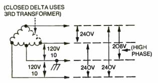
Fig. 3-12. Typical open-delta secondary connections for a 3-phase system. One transformer provides a 120V single phase. Voltages shown are the design parameters.
