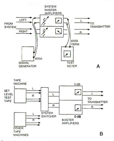
Fig. 8-2. Set the levels of the master amplifiers first (A), and then (B) the individual tape machines.
