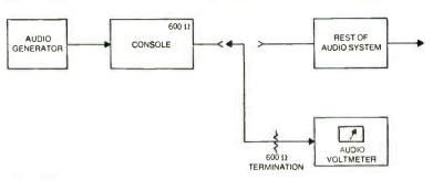
Fig. 14-8. Use the audio voltmeter to measure output of each unit in chain. Add proper termination to input of voltmeter.
