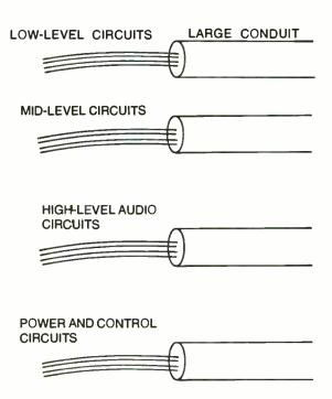
Fig. 3-7. Segregate cables by signal levels.
