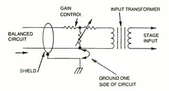
Fig. 4-27. When a T-pad gain control is used ahead of the transformer on a balanced circuit, it may be necessary to ground one side and run unbalanced.
