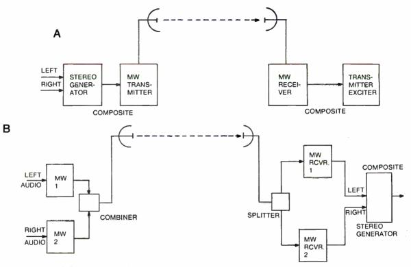
Fig. 7-19. Two ways to send stereo over the STL in A, as composite, in B, as the left and right audio.
