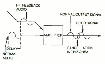
Fig. 4-10. RF feedback to the audio that is delayed can cause an echo effect.
