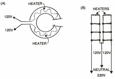
Fig.11-9. Each element of the FM antenna has a heater mounted internally. All heaters are connected in parallel. Divide load on both sides of a 230V circuit.
