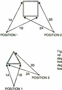
Fig. 12-9. Transit should be set up at two different positions 90 degrees apart. On a triangular tower, this may be less than 90 degrees. Check opposite legs of tower in each position.
