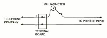
Fig. 6-10. Break one side of circuit and insert milliammeter in series with line to measure signal current.
