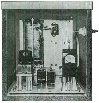
Fig. 11-1. The AM antenna must be matched to the transmission line at the base of the tower. Shown is a unit that contains a full T-network that can handle 1250W. (Courtesy Harris Corporation.)
