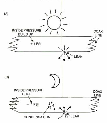
Fig. 10-8. An air dielectric line without pressurization and with a leak will breathe.
