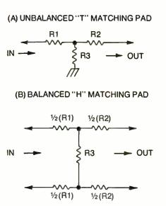
Fig. 4-20. To make a balanced pad from a T-pad calculated resistor values, divide R1 and R2 in half for each side of the circuit (R3 remains the same).
