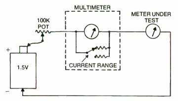
Fig. 13-4. To check unknown scale of a meter, use the ammeter section of a multimeter as a comparison. Start with a high-resistance value in the pot.
