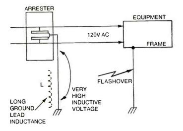
Fig. 3-10. The inductance of the long ground lead at the transient frequency generates dangerously high inductive voltages that arc over to adjacent units.
