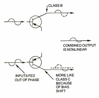
Fig. 4-13. Class B push-pull stages must be kept balanced. If bias should shift one half of the push-pull circuit so that one stage acts more like Class C, the combined output will be nonlinear.
