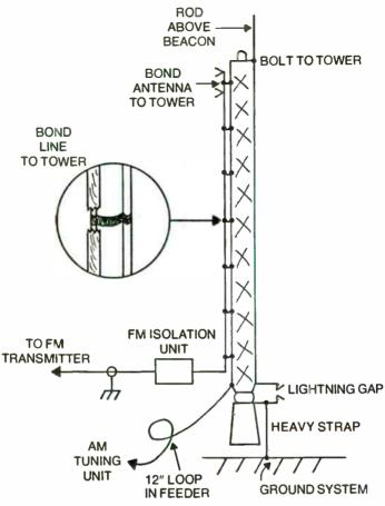
Fig. 11-10. Standard lightning protection.
