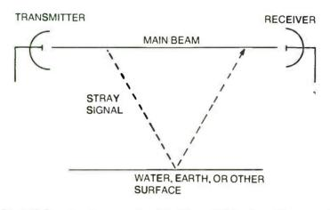
Fig. 7-16. Beam tends to spread out, and stray signal reflects off surfaces and back into beam with the wrong phasing.
