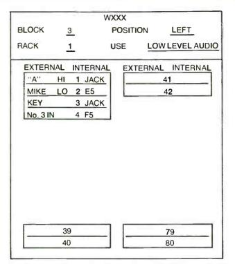
Fig. 3-4. Typical audio terminal block sheet. List all the terminals even though they may be spares at the moment.
