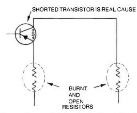
Fig. 2-7. Defective parts are not always the real cause. In this case, the shorted transistor burned out the resistors.
