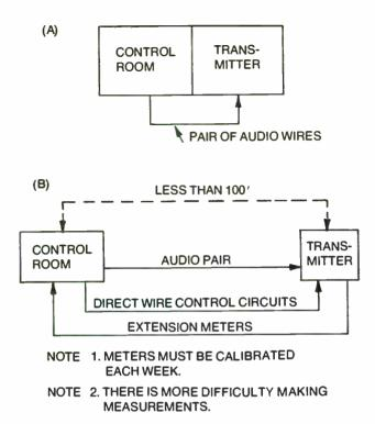
Fig. 1-10. Moving the transmitter out of direct visual view and control by the operator increases station complexity and requires more circuitry and routines. In A, the simple system requires nothing more than a pair of audio wires. In B, there must also be wire control circuits and extension meters. The further away the transmitter is moved, the more complex it becomes.
