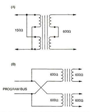
Fig. 4-22. When windings on a transformer are strapped in parallel, they usually provide one-fourth the impedance value of the series strapping. When two separate transformers are strapped in parallel, the impedance is halved.
