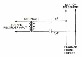
Fig. 6-2. A simple, direct connection can be made to regular telephone circuit, but use isolation.
