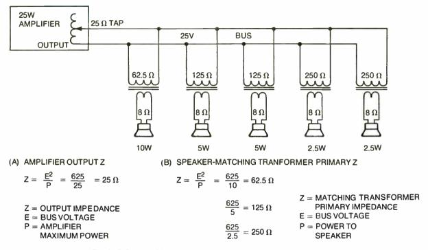
Fig. 6-13. Design of 25V system with "unmarked" components. Compute output impedance tap of amplifier, and use universal output transformers at each speaker.
