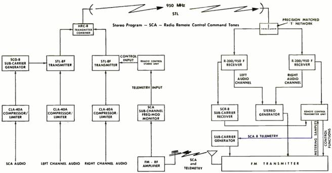
Fig. 7-18. Full over-the-air remote control for FM radio. (Courtesy Marti Electronics, Inc.)
