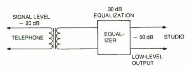
Fig. 7-2. When heavy equalization is done, the output of the equalizer may be at a low level.
