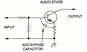
Fig. 4-25. Bypass the emitter to base at the transistor if this won't upset stage.
