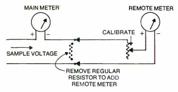
Fig. 9-18. When the remote meter and calibrating resistor are in series with the main meter, they are difficult to calibrate; the remote will affect the main meter.
