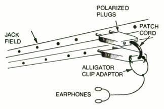
Fig. 2-14. When there is no multiple on a jack, use a patch cord to substitute for the jack "normals." Use earphones with alligator clips and attach to screws at rear of patch plug.
