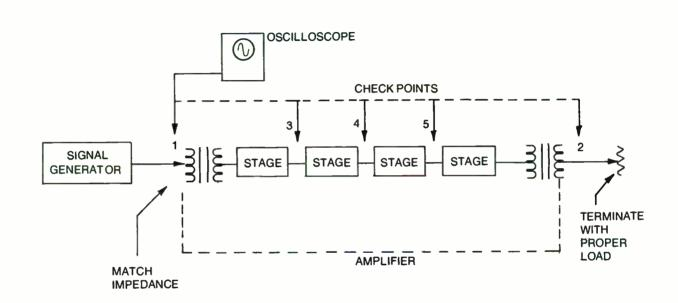
Fig. 2-11. Signal tracing. Measure the input first, then the output, then stage to stage.
