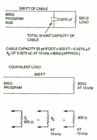
Fig. 4-17. Cable capacitance will shunt the high-frequency response. In the example, even a properly terminated cable will have a rolloff at the upper frequencies when the cable is very long.
