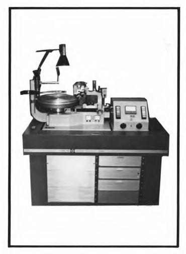
A Neumann VMS70 Cutting Lathe, the most common lathe found today.
