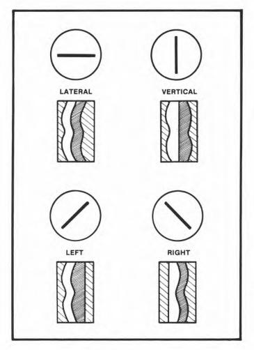
Oscilloscope patterns with matching groove types.
