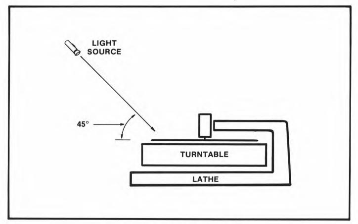
Correct physical procedure for observing light patterns.
