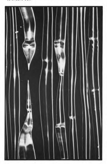
Out of phase material can make a cutterhead "lift out," thereby breaking the groove. The lift out shown here is unacceptable.
