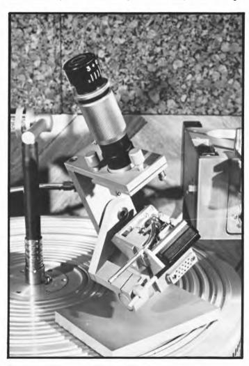
A second, smaller microscope is used to mount the cutting stylus in the cutterhead.
