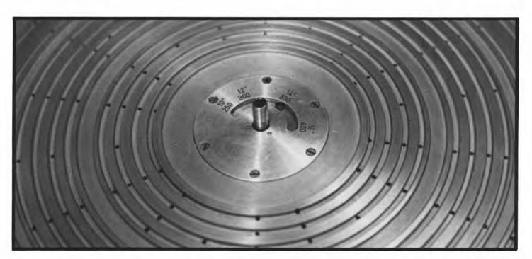
Close-up of the turntable of a Neumann Lathe, showing disc size selector and vacuum holes for disc hold-down.
