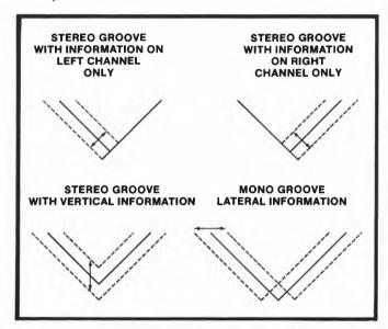
Westrex kept the 90° relationship of lateral to vertical but rotated the axis 45° to the plane of cut. This system made **physical** compatibility a reality. In addition, rumble is generally more pronounced in the vertical plane. The 45/45 system rumble is identical in both channels and lower by about 3 DB overall.
