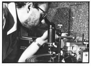
Each disc is spot-checked through the microscope after cutting.
