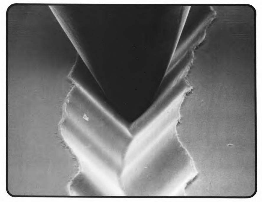
Playback stylus resting in a groove (1,000 magnification). Severe "horns" are visible at the top of each groove wall, typical of an inferior pressing. (Photo courtesy Stanton Magnetics)
