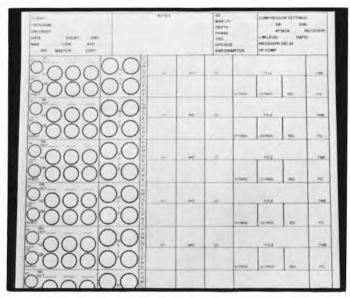
Typical mastering setting sheet, allowing the engineer to repeat his settings at a later date.
