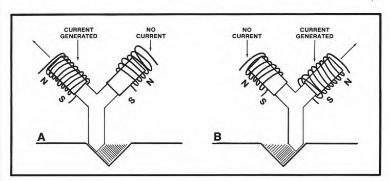
A playback stylus translates the stereo groove back into two distinct signals. "A" shows right channel output; "B" shows left channel output.
