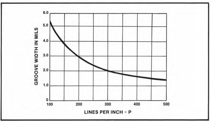
Groove width versus lines per inch. Average groove width
