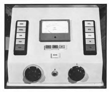
Control Section of a Neumann Lathe, showing turntable speed indicator, lathe function control and L.P.I. Meter.
