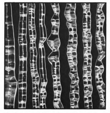
Complex groove geometries can often cause pressing problems. The vinyl must fill every nook and cranny, much like hot butter on an English muffin.
