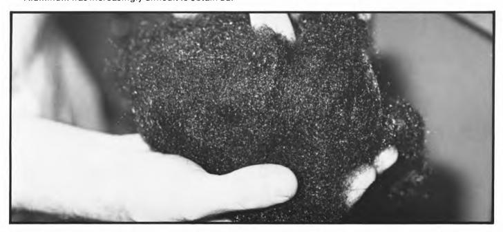
The waste acetate that is cut out of the groove is called "chip". By means of a vacuum system, it is sucked into a receptable for disposal.
