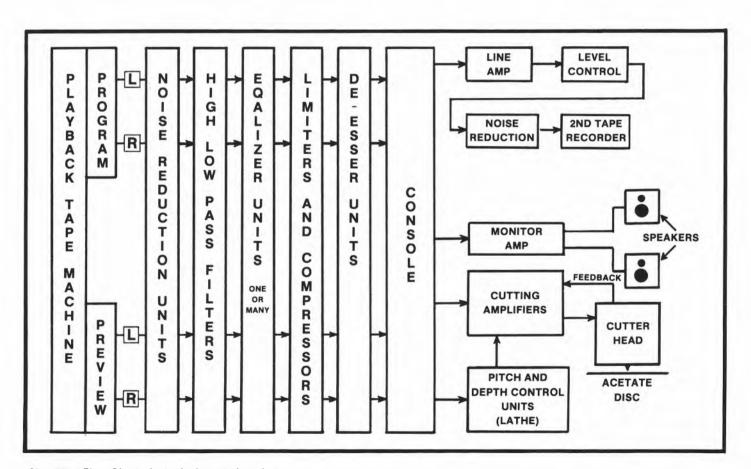
Simplified Flow Chart of a typical mastering chain.
