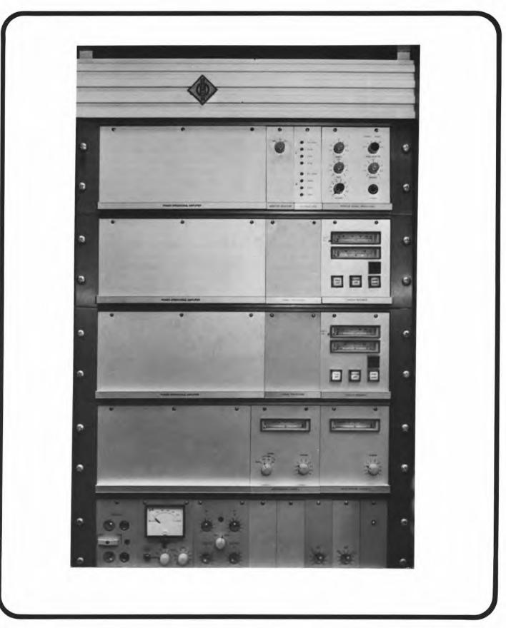
The output of the Mastering Console is fed into the cutting amplifiers, which in turn drive the cutterhead.
