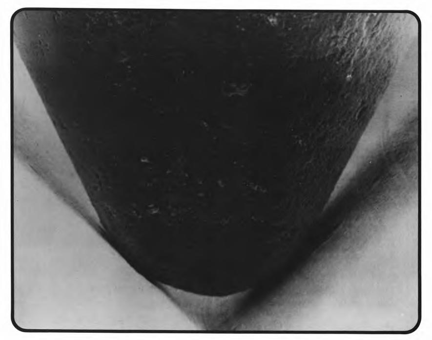
A spherical playback stylus resting in a record groove in playing position (10,000 magnification). (Photo courtesy Stanton Magnetics)
