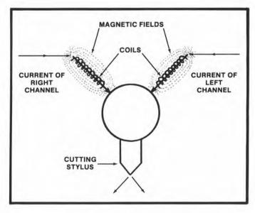
Simplified view of a stereo cutterhead.
