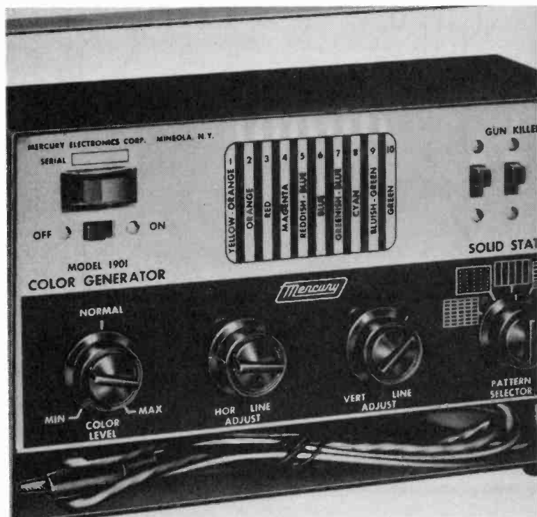
Fig. 2-8. Mercury's 1900-1901 inexpensive color-bar generator produces variable size lines and dots.
