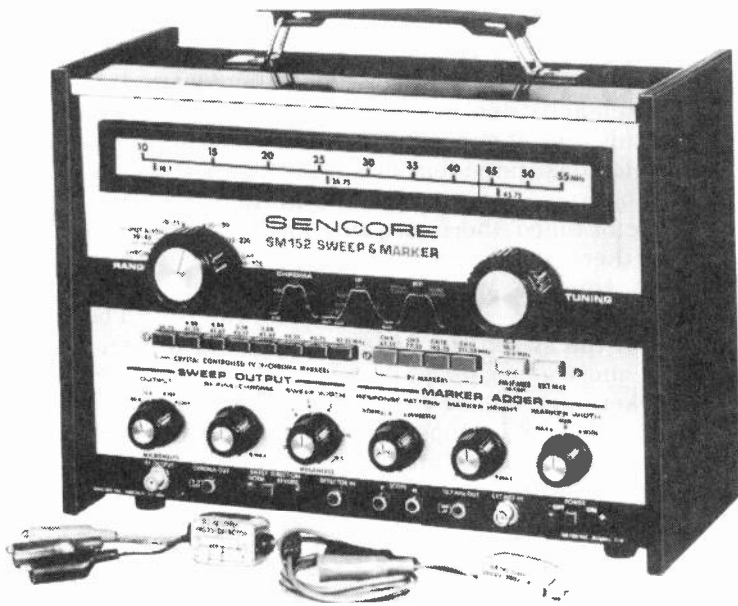
Fig. 14-18. Varistor tuned SM152 Sencore sweep, crystal-controlled marker generator with ranges from 10 MHz to 900 MHz. It contains 13 close frequency crystals with both vertical and horizontal markers, virtually flat output. ($459)
