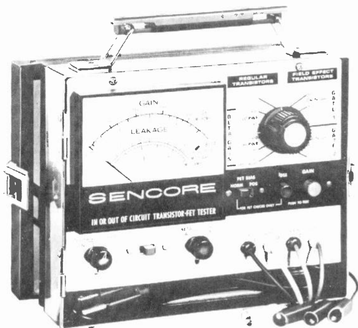
Fig. 14-15. Sencore's TF17 circuit transistor checker is handy for FETs and bipolars when you're in semiconductor trouble.
