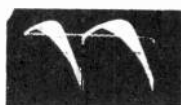
64 PW800-C 9V P-P Vert Rate Vert Input to Red and Green Conv Coils
