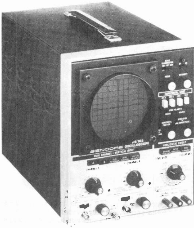
Fig. 14-22. Dual-trace, triggered and free-run sweep, Sencore PS163 scope with front panel vector inputs; deflection factor to 5 millivolts, sweep to 100 nanoseconds. ($495)
