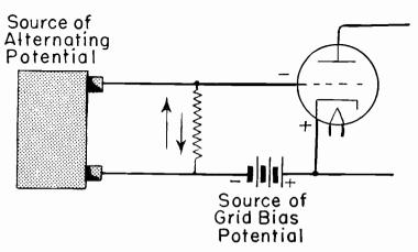
Fig. 17-5.—A grid bias potential furnished by a battery.
