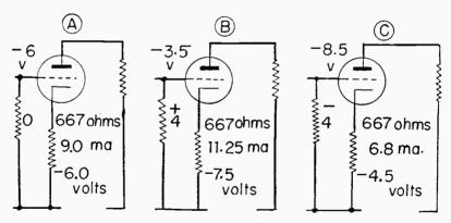
Fig. 17-10.—These potentials and currents would exist if the cathode-bias did not alter the values of plate current.
