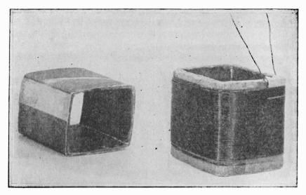
Fig. 20-11.—The bobbin on which the windings are placed.
