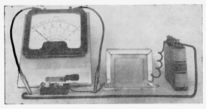
Fig. 12-12.—Experimental setup for observing some effects of self-induction.
