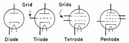
Fig. 15-13.—The symbols for four types of tubes.
