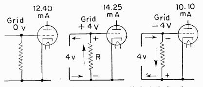
Fig. 17-3.—Grid potentials and plate currents with the 4-volt alternating signal potential.
