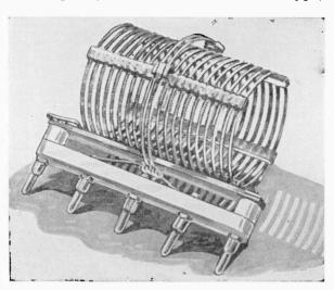
Fig. 14-4.—An air-core coil or inductor used at high frequencies.
