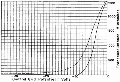
Fig. 18-11.—Transconductance of a remote-cutoff pentode (broken line) and of a sharp-cutoff pentode (full line).
