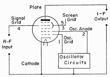
Fig. 18-20.—Connections for one kind of pentagrid converter.
