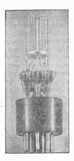
Fig. 15-6.—With the plate removed we see the several grids.
