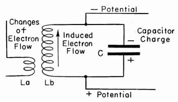
Fig. 19-12.—The induced electron flow and the accompanying potentials in a tuned coupled circuit.
