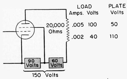
Fig. 18-5.—Changes of current and potential in the plate circuit of a screen-grid tube.
