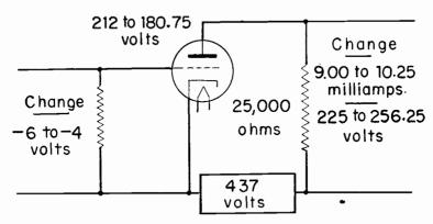
Fig. 16-19.—Operating conditions with a 25,000-ohm load.
