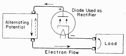
Fig. 15-16.—A heater-cathode type of diode used as a rectifier.
