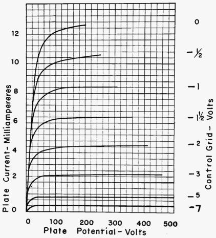
Fig. 18-8.—Typical plate characteristics for voltage amplifying pentodes.
