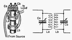
Fig. 19-13.—Two tuned circuits having mutual inductive coupling.
