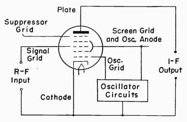
Fig. 18-21.—Connections for another type of pentagrid converter.
