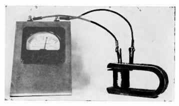
Fig. 12-7.—Moving the coil into the magnetic field induces current in one direction.
