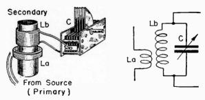
Fig. 19-10.—Mutual inductive coupling with tuned secondary winding.
