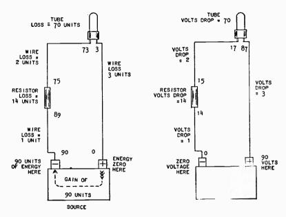
Fig. 11-10.—Energy is added to electrons in the source, and ost in the external circuit.
