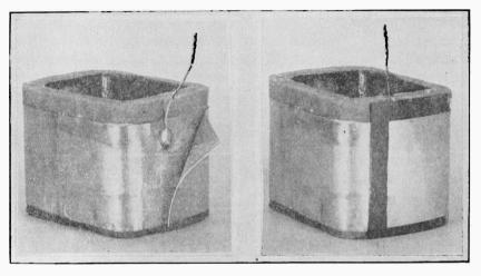
Fig. 20-13.—The electrostatic shield and its connection lead.
