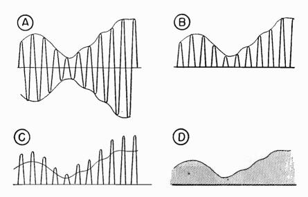
Fig. 18-16.—How a diode detector separates the low-frequency modulation from the high-frequency signal.
