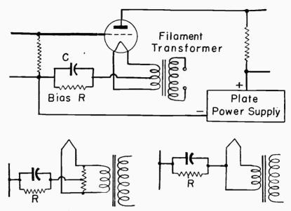
Fig. 17-15.—Obtaining a cathode-bias with a filament-cathode type of tube.
