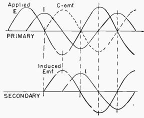
Fig. 20-20.—Phase relations in primary and secondary windings.
