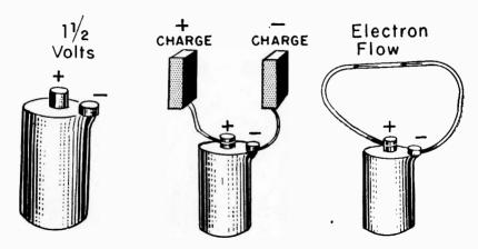
Fig. 11-7.—A source of emf will produce electric charges and cause electron flow.
