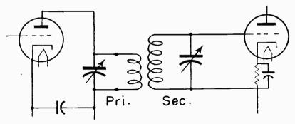
Fig. 20-4.—Coupling by means of a double-tuned transformer between amplifier tubes.
