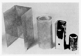
Fig. 14-17.—Shielding enclosures and cans.
