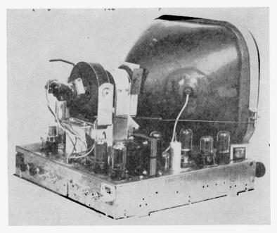
Fig. 11-3.—Service controls and adjusters for controlling picture quality are accessible at the rear of this chassis.
