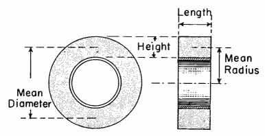
Fig. 14-22.—How and where to measure the dimensions of a multi-layer coil.
