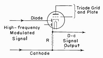
Fig. 18-15.—Connections to a diode used as a detector.
