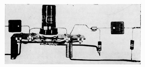
Fig. 11-9.—Principal parts of a resistance-capacitance coupling system, which may be referred to as a circuit.
