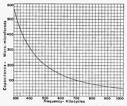
Fig. 13-21.—How the capacitance is varied when tuning to various frequencies.
