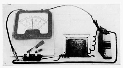
Fig. 12-15.—With the coil out of circuit there will be no "inductive kick."
