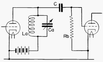
Fig. 19-6.-- A tuned impedance coupling for radio frequencies.
