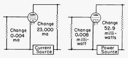
Fig. 16-17.—Current amplification (left) and power amplification (right) with the triode.
