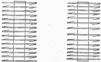
Fig. 18-10.—At the right is the grid wire spacing for a variable-mu pentode. for use where there are no great variations of control grid potential.
