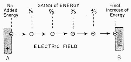
Fig. 15-21.—When electrons move through an electric field they gain energy if movement is from positive to negative.
