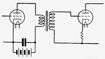
Fig. 20-26.—An audio transformer for coupling between amplifier tubes.
