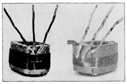
Fig. 20-17.—The center-tapped winding for the tube heaters.
