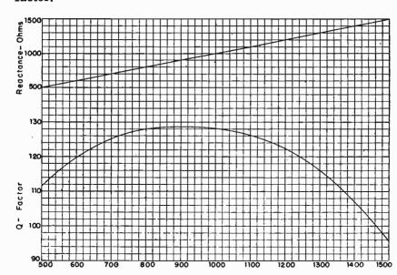
Fig. 14-10.—Reactance (top) and Q-factor (bottom) of the single layer coil.
