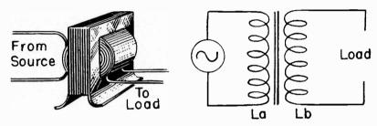
Fig. 19-9.—Mutual inductive coupling in an iron-core transformer.
