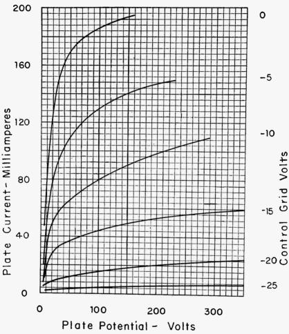
Fig. 18-12.—Plate characteristics for a typical power pentode.
