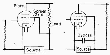
Fig. 18-3.-Connections for the screen grid.
