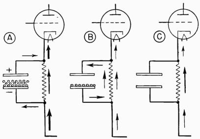
Fig. 17-13.—The action of a smoothing capacitor or bypass capacitor used with the hias resistor.
