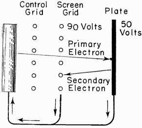
Fig. 18-6.—Secondary emission in a screen grid tube.
