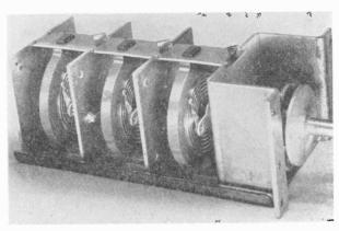
Fig. 14-3.—The spiral inductors or coils in this unit are used for several different television tuners.
