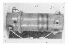
Fig. 14-5.—Tuning coils supported in insulating tubing.
