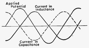
Fig. 12-31.—Lagging inductive current and leading capacitive current are in opposite phase with reference to each other.
