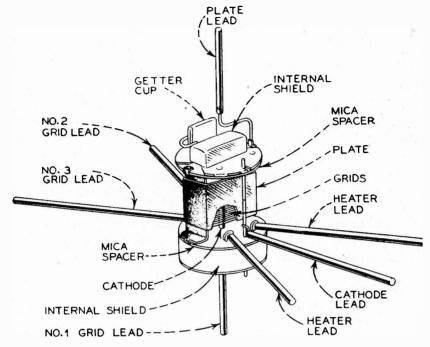
Fig. 18-23.—Internal structure of an RCA acorn pentode.
