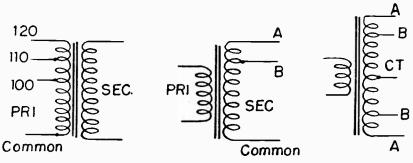
Fig. 20-23.—Voltage toos on primary and secondary windings.
