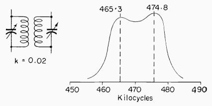
Fig. 19-16.—Double-hump resonance with coupled tuned circuits.
