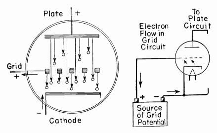
Fig. 15-27.—When the grid is made positive it attracts electrons just as does the positive plate.
