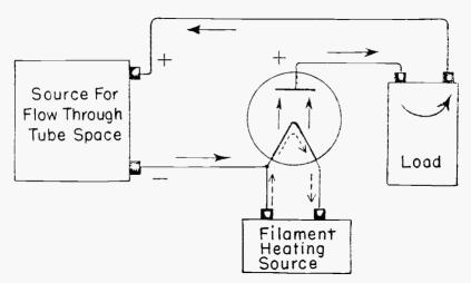
Fig. 15-15.—Connections for a diode tube having a filament-cathode.
