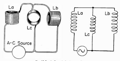
Fig. 19-7.-A direct inductive coupling.
