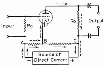
Fig. 17-8.—Bias obtained from the source of plate potential and current.
