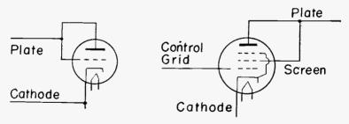
Fig. 18-17.—A triode connected as a diode (left), and a pentode connected as a triode (right).
