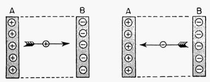
Fig. 15-18.—Charges are attracted toward other charges which are of opposite polarity.
