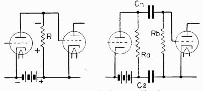
Fig. 19-3.—Resistance coupling between amplifier tubes.
