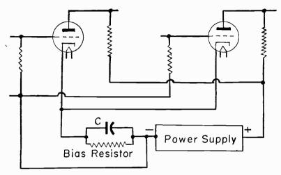
Fig. 17-14.—A single cathode-bias resistor used with several tubes.
