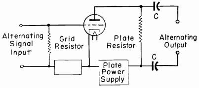
Fig. 17-1.—A stage of amplification using a triode tube.
