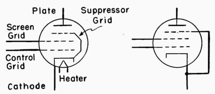
Fig. 18-7.—Symbols for pentodes; showing the five elements.
