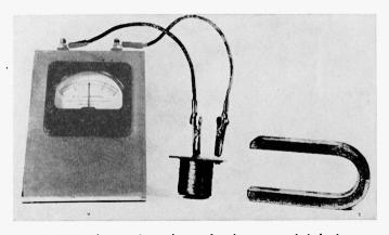
Fig. 12-6.—The experimental setup for electromagnetic induction.
