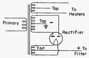
Fig. 20-7.—The center tap connections on the secondary windings of the power transformer.
