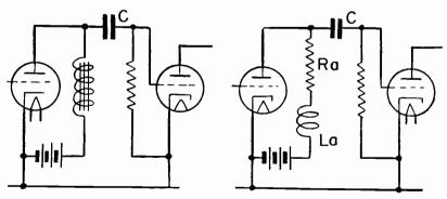
Fig. 19-5.—An audio-frequency impedance coupling (left) and a coupling with compensation for high frequencies (right).
