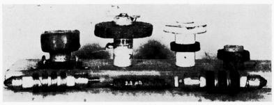
Fig. 14-15.—R-f chokes used wherever high-frequency alternating currents are to be opposed.
