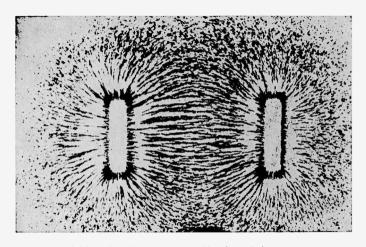
Fig. 12-4.—The field of the electromagnet is like that of the permanent magnet.
