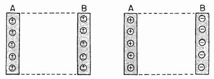
Fig. 15-17.—The charges at the right are produced by transfer of electrons.
