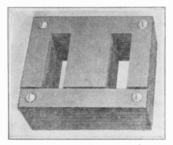
Fig. 20-8.—The core of the power transformer.
