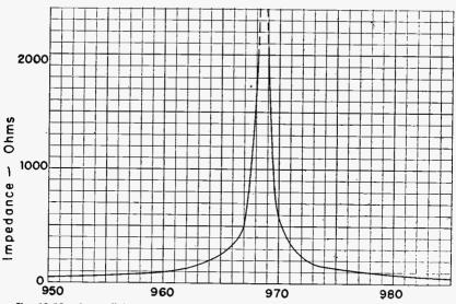
Fig. 13-18.—A parallel resonant circuit has high impedance at the resonant frequency.
