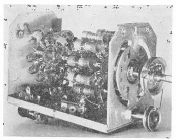
Fig. 13-20.—A television tuner containing adjustable inductors.
