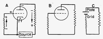
Fig. 18-1.—The grid and the plate, with vacuum between them, act as a capacitor.
