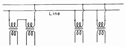
Fig. 20-21.—Primaries in series and in parallel on the line.
