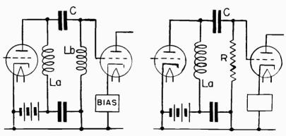
Fig. 19-4.—Impedance coupling with air-core coils.
