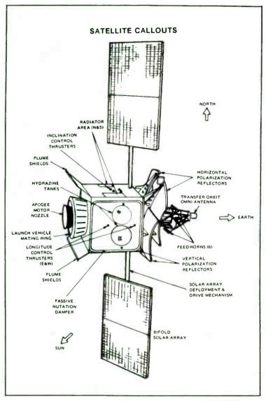
Fig. 1-16. The anatomy of a communications satellite, in this case an RCA Satcom satellite (courtesy RCA Government Systems Division).
