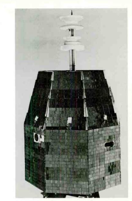
Fig. 1-6. The Relay satellite weighed 169 pounds—less than the first Sputnik (courtesy NASA).
