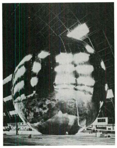
Fig. 1-4. The Echo satellites were nothing but large metallized balloons off of which signals were bounced. This was one of several space communication techniques that were discarded in favor of geosynchronous satellites (courtesy NASA).
