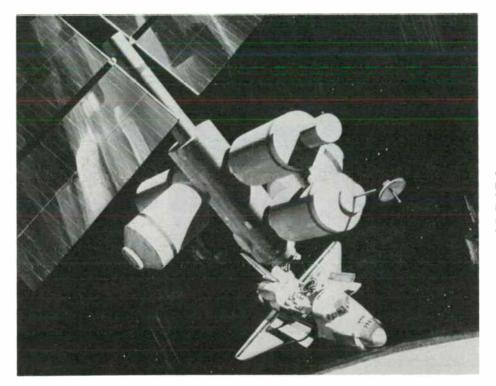
Fig. 1-20. The space shuttle can eventually be used to carry up the parts for entire manned communications satellites that will be assembled in low earth orbit and boosted up to geosynchronous orbit (courtesy NASA).
