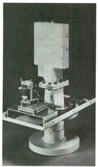
Fig. 5-1. The low-noise amplifier, down converter, and rotatable feed assembly from a Heathkit home earth station (courtesy Heathkit).
