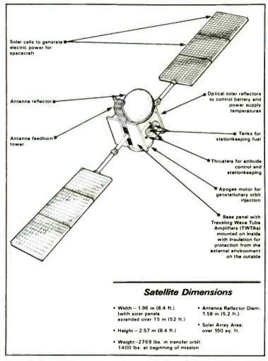
Fig. 1-22. The GSTAR communications satellite from GTE will be used primarily for business communications (courtesy GTE).
