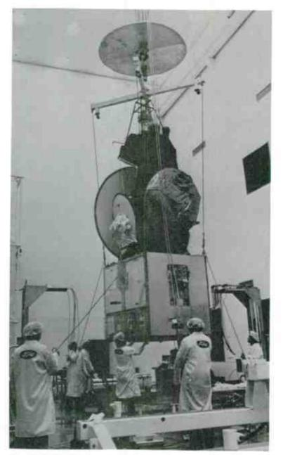
Fig. 1-10. Intelsat V being readied for launch. The satellite can handle 12,000 two-way telephone calls and two color television channels at the same time (courtesy NASA).
