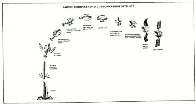
Fig. 1-17. The various stages that an RCA Satcom satellite goes through from lift-off to operation in orbit (courtesy RCA Government Systems Division).
