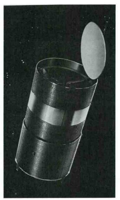
Fig. 9-1. Westar IV has the capacity to handle 24 channels of television simultaneously.
