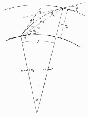
FIG. 1. Geometry of the refraction of radio waves.
