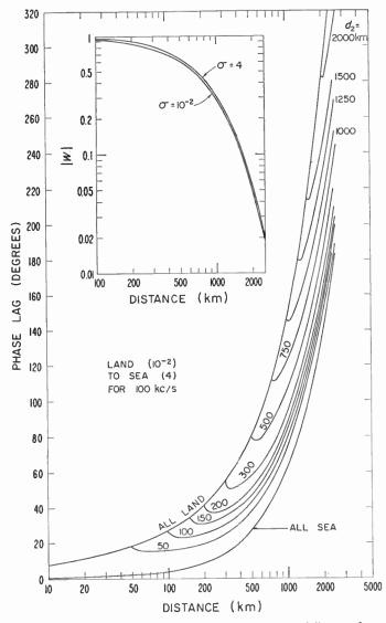
FIG. 12. Amplitude and phase of the relative field as a function of distance for propagation from land to sea.
