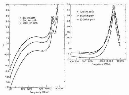
FIG. 14. Values of b and m in the regression line y = mx+b, where y is the logarithm of the total path absorption, x is the logarithm of the absolute humidity, b is the value of y when the absolute humidity is 1 g/m<sup>3</sup>.
