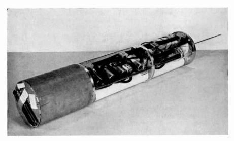
FIG. 9. A view of the 400 Mc/s light-weight refractometer as developed by Deam, complete with the exception of the removal of the aluminum cylindrical covers.
