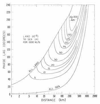
Fig. 9b. Phase of the relative field corresponding to conditions of Fig. 9a.
