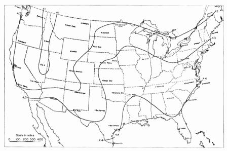
FIG. 17. August values of 300-mile propagation path absorption loss (in db) to be exceeded 1 per cent of the time for a frequency of 10 Gc/s.
