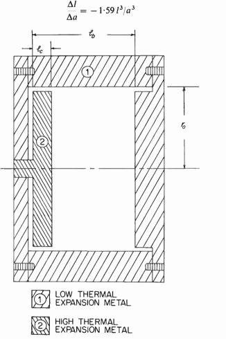
FIG. 6. Parts and assembly sketch of temperature compensation technique employed in the microwave cavities of the Crain refractometer.
