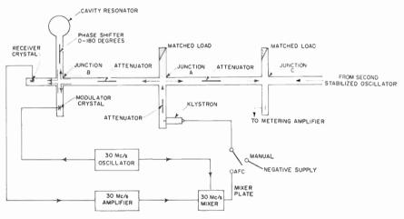
FIG. 4. Block diagram of the basic stabilized oscillator unit employed for all models of the Crain refractometer.
