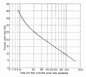
FIG. 24. Excess path loss due to rainfall versus hours per year at Mobile, Alabama. (After Hathaway and Evans, 1959.)
