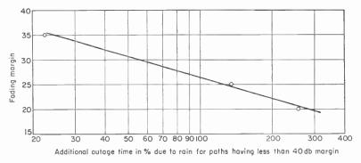
FIG. 25. Additional outage time expected for 11 Gc/s systems having a fading margin less than 40 db.
