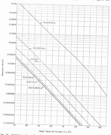
FIG. 11. Common values of total gaseous atmospheric absorption for elevations greater than 75 000 ft.
