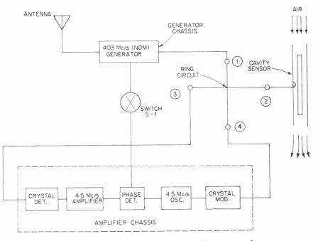
FIG. 10. Block diagram of the basic circuit of the 400 Mc/s Deam refractometer.
