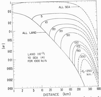
Fig. 10a. Amplitude of the relative field of the ground wave as a function of distance for propagation from land towards the sea. The coast line is a distance  $d_2$  from the transmitter (which is on the land).
