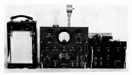
FIG. 2. A view of a typical model of the Crain 9 400 Mc/s refractometer showing from left to right the recorder, refractometer proper and power supply. The measuring cavity with its frequency perturbation screw is above the refractometer while the top part of the reference cavity can just be seen to the left of the measuring cavity. Later models made use of higher speed recorders to obtain fluctuation data.
