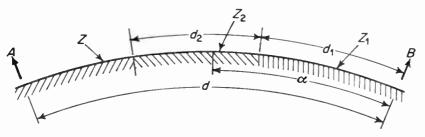
FIG. 8. Three-section path on a spherical earth.
