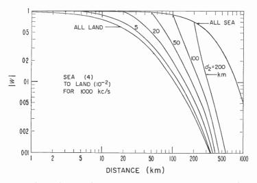
FIG. 11. Amplitude of the relative field of the ground wave as a function of distance for propagation from sea towards the land. The coast line is a distance  $d_2$  from the transmitter.
