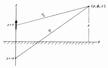
FIG. 1. Cylindrical coordinate system  $(\rho, \phi, z)$  showing location of source dipole with respect to impedance boundary.
