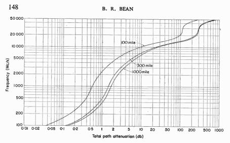
FIG. 21. Combined rain and gaseous absorption to be exceeded 1 per cent of the time.
