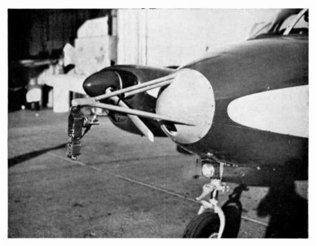
FIG. 8. A view of a refractometer installation designed to minimize aircraft interference with the free airstream. This nose cone adaptation on a light-weight plane was made by the National Bureau of Standards for use with the Birnbaum refractometer.
