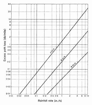
FIG. 19. Rain attenuation versus rainfall rate (Theoretical, after Ryde and Ryde, 1945).
