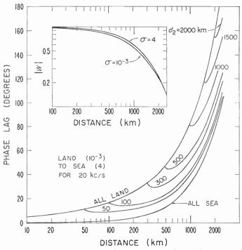
FIG. 14. Amplitude and phase of the relative field as a function of distance for propagation from land to sea.
