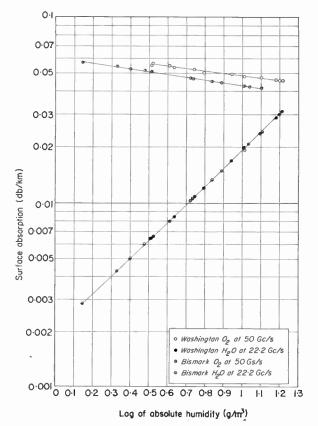
FIG. 13. Surface value of 22.2 and 50 Gc/s absorption versus absolute humidity at Washington, D.C., and Bismarck, North Dakota.
