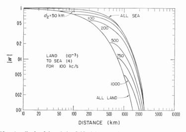
FIG. 13a. Amplitude of the relative field of the ground wave as a function of distance for propagation from land towards the sea. The coast line is a distance  $d_2$  from the transmitter (which is on the land).
