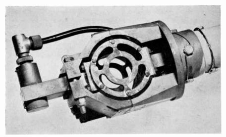
FIG. 7. A view of the ventilation employed with a measuring cavity in a microwave refractometer developed by Lane *et al.* (1961) following the Birnbaum principle. Somewhere around 75 per cent of the end plate material is removed to permit free access of air.
