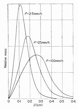
FIG. 18. Relative total mass of liquid water in the air contributed by drops of diameter D for various precipitation rates. (Derived from Laws and Parsons' distributions for a horizontal surface by dividing by the appropriate terminal velocities.)
