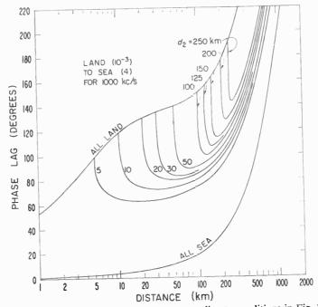
FIG. 10b. Phase of the relative field corresponding to conditions in Fig. 10a.
