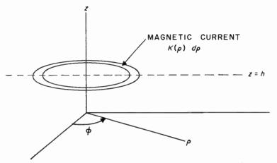
FIG. 4. Excitation of surface waves by a magnetic ring source. The magnetic current  $K(\rho)$  flows in the  $\phi$  direction.
