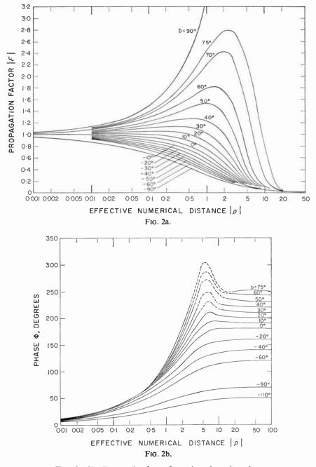
FIGS. 2a, 2b. Propagation factor for an impedance boundary. (The precise numerical values for large |p| and positive b are somewhat uncertain.)
