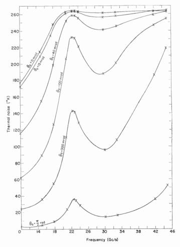
FIG. 27. Thermal noise versus frequency for mean profile conditions, and various antenna elevation angles,  $\theta_0$ , at Bismarck, North Dakota.
