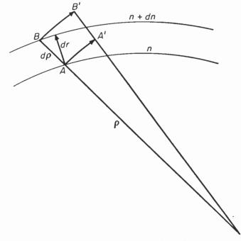
FIG. 2. Differential geometry used in the derivation of the effective-earth's-radius-model atmosphere.
