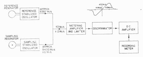
FIG. 3. Block diagram of the basic circuit for all models of the Crain refractometer.
