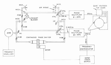
FIG. 12. Block diagram of the Tolbert phase shift refractometer.
