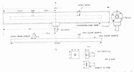
FIG. 11. Schematic view of the ceramic, open-end half-wavelength coaxial cavity employed with the 400 Mc/s Deam refractometer.
