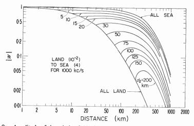
FIG. 9a. Amplitude of the relative field of the ground wave as a function of distance for propagation from land towards the sea. The coast line is a distance  $d_2$  from the transmitter (which is on the land).
