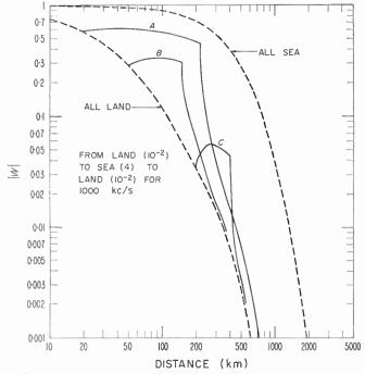
FIG. 15. Amplitude of the relative field for propagation over a three-section path consisting of two land portions separated by a sea portion.
