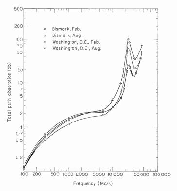
FIG. 12. Total path absorption over a 1 000 km propagation path with the climate of Bismarck, North Dakota, and Washington, D.C.
