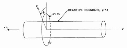
FIG. 5. Excitation of surface waves on a cylindrical rod (of infinite length) by a magnetic ring source.
