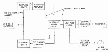
FIG. 5. Block diagram of the basic circuit for the various models of the Birnbaum refractometer.
