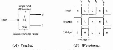
Fig. 3-46. Monostable multivibrator.
