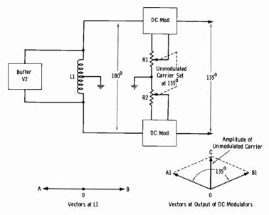
Fig. 9-31. Principle of carrier phase set.
