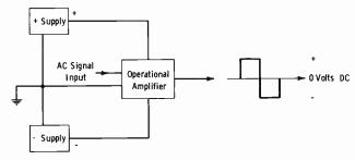
(B) Method of obtaining dc ground at output.
