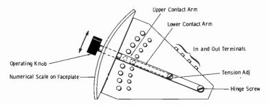
Fig. 6-16. Side view of typical vertical attenuator.
