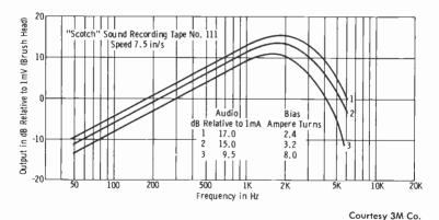
Fig. 4-29. Effect of bias on frequency response.
