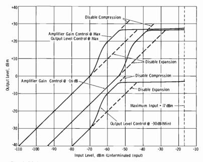
Fig. 6-44. Input-output characteristics of BA-43 and BA-45 combination.
