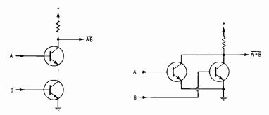
Fig. 3-37. Direct-coupled-transistorlogic NAND circuit.
