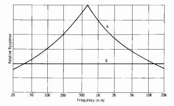
Fig. 4-6. Dynamic-microphone response curves.
