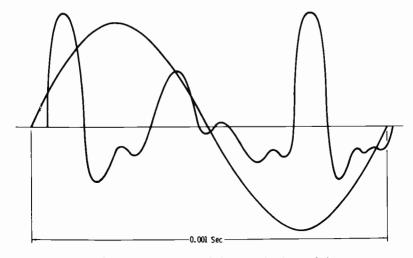
Fig. 14-2. Curves indicating peak factors of voice and sine waves.
