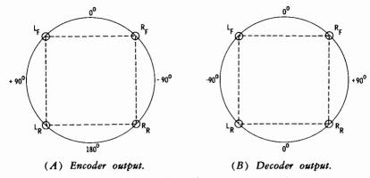
Fig. 7-13. Phase relationship between channels.
