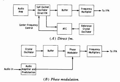
Fig. 10-12. Block diagrams of pm and fm transmitters.
