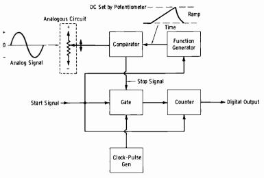
Fig. 3-59. Comparison method of analog-to-digital conversion.
