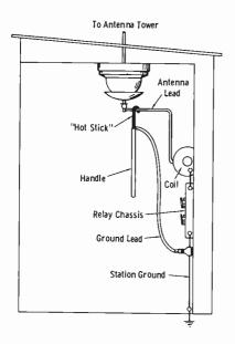
Fig. 14-37. Safety device for grounding high-voltage points.
