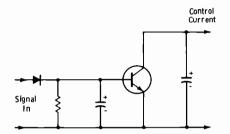
Fig. 6-38. Power rectifier circuit diagram.
