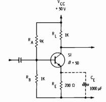
Fig. 3-2. Class-A common-emitter amplifier circuit.
