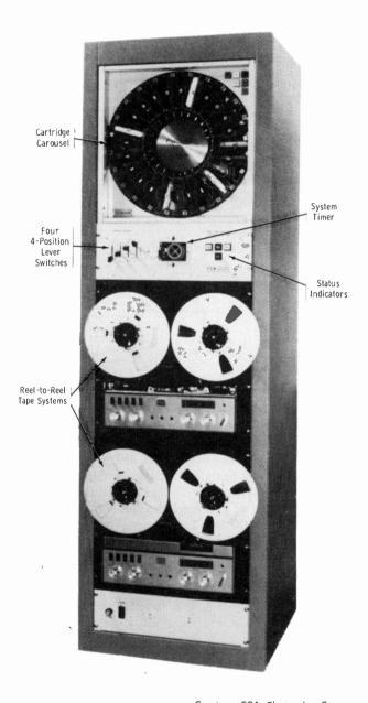
Courtesy CCA Electronics Corp. Fig. 7-28. CCA Mini-Automation system.
