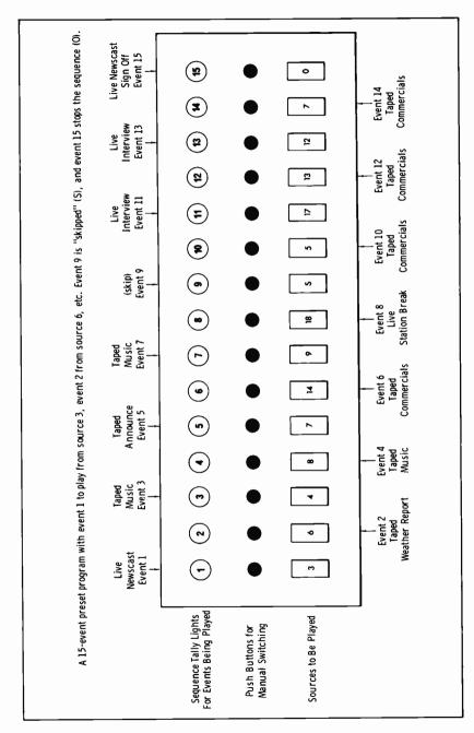
Fig. 7-30. RCA BCA-15B programmer.
