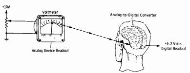
Fig. 3-21. Familiar example of analog-to-digital conversion.
