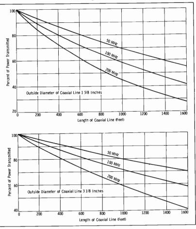
transmitted by coaxial cables.
