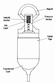
Fig. 4-16. Unidirectional microphone.
