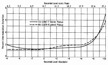
Fig. 13-7. Percent intermodulation distortion for one type of stereo cartridge.
