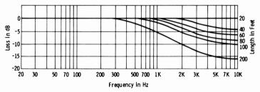
Fig. 4-2. Signal loss versus cable length (high-impedance input).
