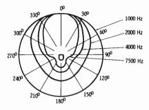
Fig. 4-13. Frequency dependence of directivity.
