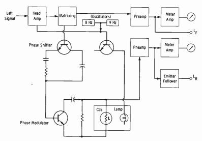
Fig. 7-18. Phase modulator circuit.
