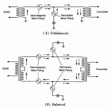
Fig. 12-2. Remote telephone lines.
