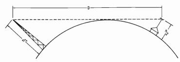
Fig. 10-2. Calculation of line-of-sight distance.
