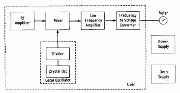
Fig. 9-40. Metron Model 510 analog a-m frequency monitor.
