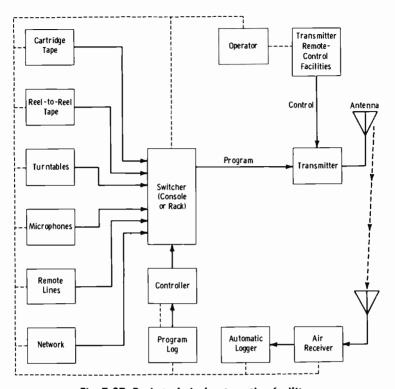
Fig. 7-27. Basic technical automation facility.
