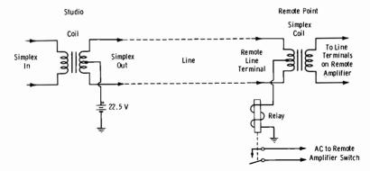
Fig. 8-14. Simplex circuit for control of remote amplifier.
