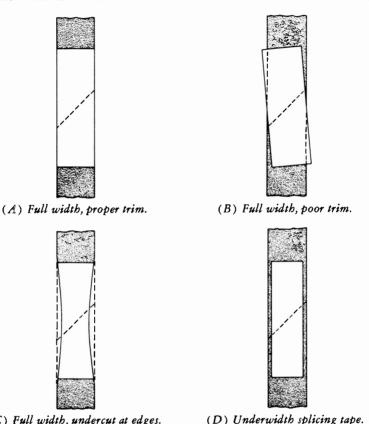
Fig. 13-26. Splicing widths.
