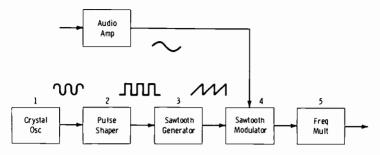
Fig. 10-15. Block diagram of pm exciter.
