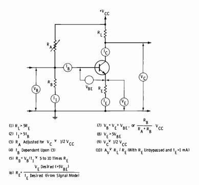
Fig. 3-1. Design parameters for common-emitter amplifier.
