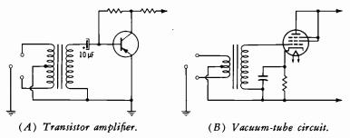
Fig. 4-3. Microphone input circuits.
