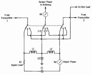
Fig. 9-38. Simplified diagram of combiner network.
