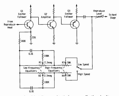
Fig. 5-4. Simplified diagram of typical post-equalization circuitry.
