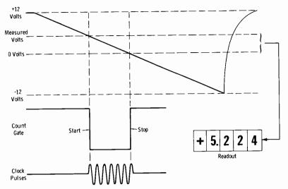
Fig. 3-22. Time-to-voltage conversion for digital voltmeter readout.
