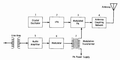
Fig. 9-23. Block diagram of typical 1-kW a-m transmitter.
