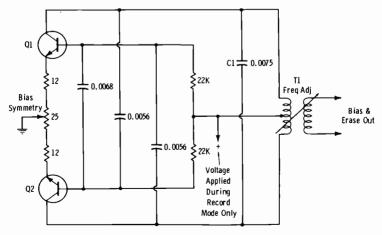
Fig. 5-7. Typical erase and bias oscillator.
