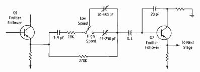
Fig. 5-3. Typical pre-equalization in two-speed tape system.
