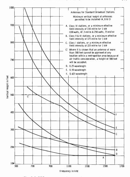
Fig. 9-8. FCC antenna requirements for a-m stations.
