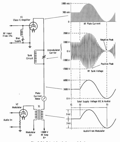
Fig. 9-26. Principle of plate modulation.
