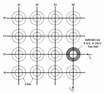
Fig. 3-66. Basic function of magnetic-core array.
