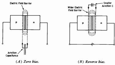
Fig. 10-18. Voltage-variable-capacitance diode.
