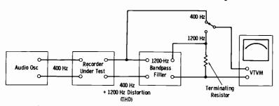
Fig. 13-17. Method of measuring third-harmonic distortion.
