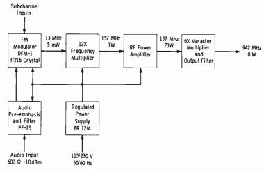
Fig. 8-25. Block diagram of stl transmitter.
