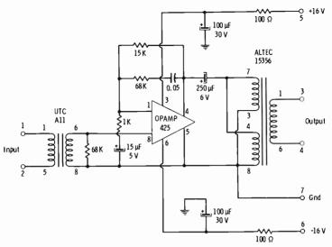
Fig. 7-4. Circuit of line amplifier.
