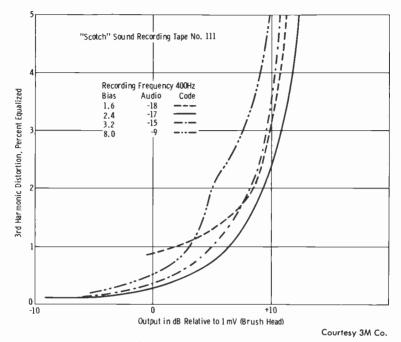
Fig. 4-28. Effect of bias on distortion.
