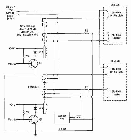
Fig. 6-23. Speaker muting and on-air light arrangement.
