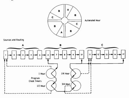
Fig. 7-32. Use of clock timers for breaks at quarter-hour intervals.
