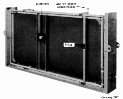
Fig. 11-30. Electromechanical reverberation unit.
