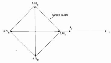
Fig. 7-9. Encoder output when  $L_F = R_F = L_R = R_R$ .
