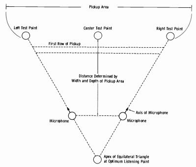
Fig. 11-29. Basic arrangement for stereo pickup.
