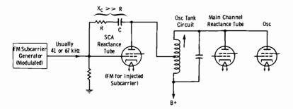
Fig. 10-28. Main-channel and SCA modulation of oscillator.
