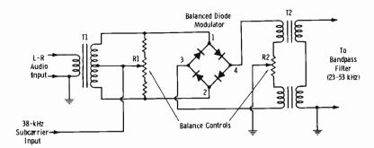
Fig. 10-33. Balanced modulator using diode bridge.
