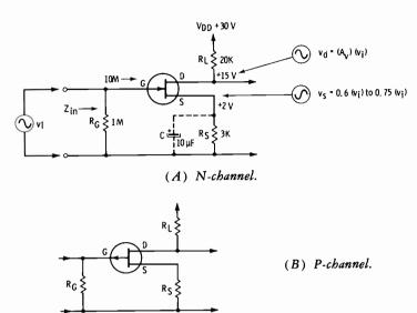
Fig. 3-15. Amplifier circuits using FETs.
