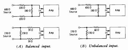
Fig. 6-29. Matching pads for amplifier driven by a preceding amplifier.
