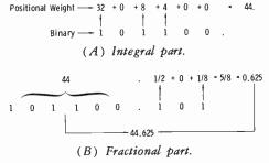
Fig. 3-25. Conversion of binary number to decimal form.
