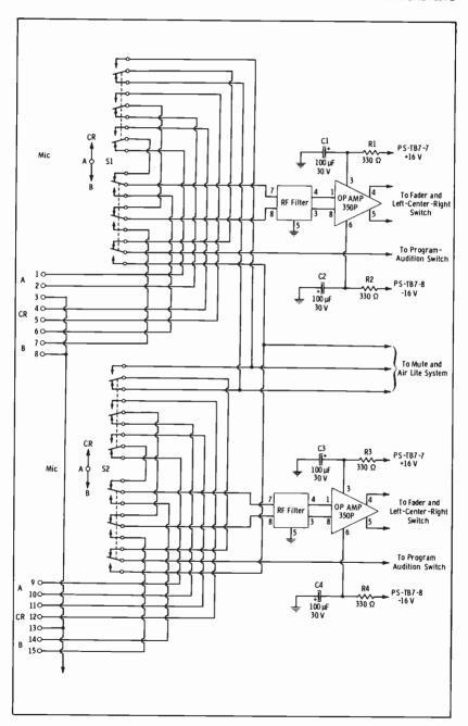
Fig. 7-5. Microphone input circuitry.
