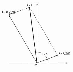
Fig. 2-9. Example of vector addition with vectors in first and second quadrants.
