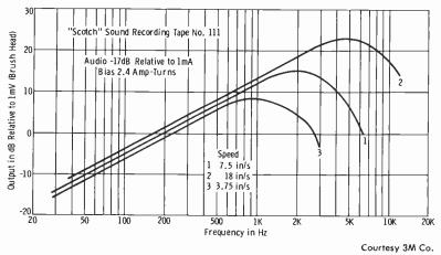
Fig. 4-30. Effect of tape speed on frequency response.
