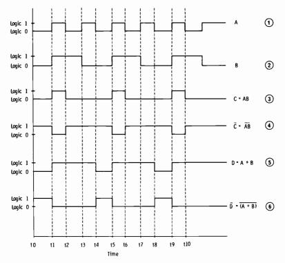
Fig. 13-11. Timing diagram.
