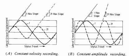
Fig. 6-30. Two basic methods of recording.
