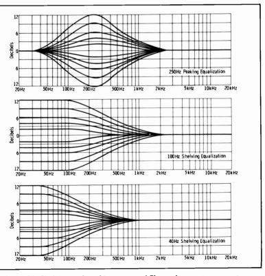
Fig. 6-20. Shelving and peaking curves of Electrodyne system-cont.
