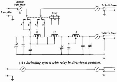
(B) Equivalent circuit for nondirectional operation.
