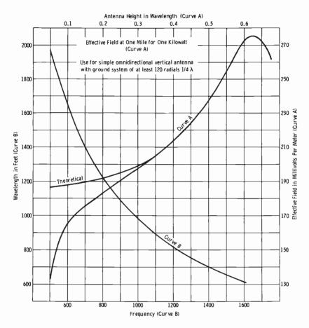
Fig. 9-10. Chart of wavelengths and effective field intensity.
