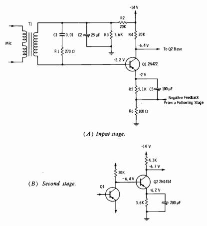
Fig. 6-27. Microphone preamplifier circuits.
