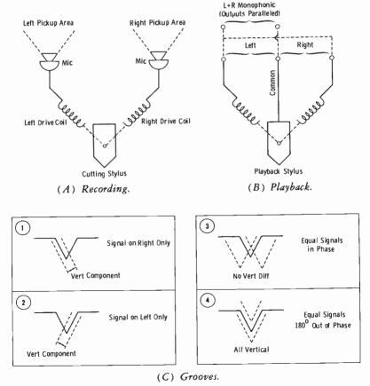
Fig. 4-22. Principles of stereo disc recording.
