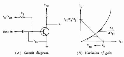
Fig. 6-39. Base-bias control of gain.
