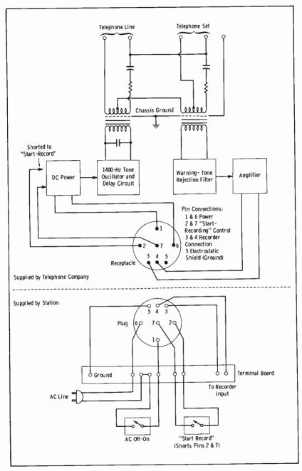
Fig. 8-16. Typical recorder-connector arrangement.
