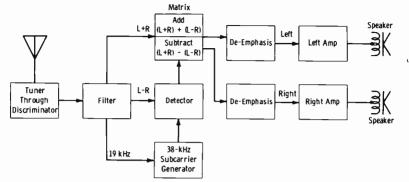
Fig. 10-32. Block diagram of stereo receiver.
