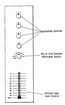
Fig. 6-18. Typical control module for individual channel.
