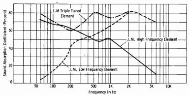
Fig. 6-4. Sound absorbing characteristics of three acoustical materials.
