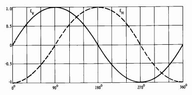
Fig. 10-6. Horizontal component of radiation delayed from vertical component by 90 electrical degrees.
