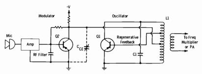
Fig. 8-12. Basic frequency-modulated oscillator.
