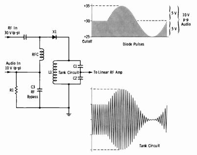
Fig. 9-29. Basic diode modulator.
