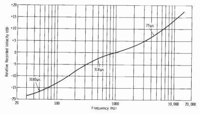
Fig. 6-31. EIA standard lateral disc-recording characteristic.
