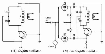
Fig. 10-21. Use of voltage-variable-capacitance diodes for direct fm.
