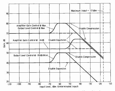
Fig. 6-45. Gain characteristics of BA-43 and BA-45 combination.
