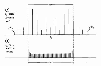
Fig. 10-14. Spectrum analysis of fm signals.
