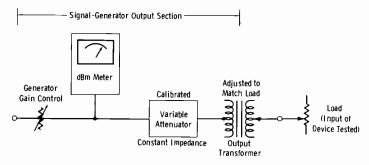
Fig. 2-14. Connection of signal generator to system being tested.
