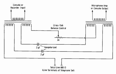
Fig. 8-18. Hybrid circuit for two-way communication.
