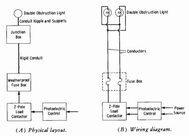
Fig. 9-15. Typical lighting system for a 150-foot tower.
