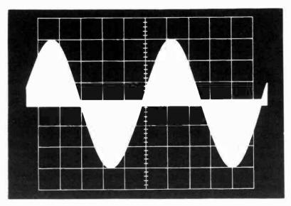
(B) Proper detected main-channel output.
