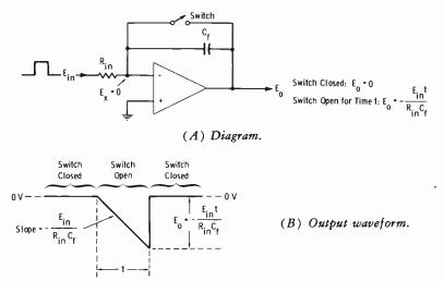
Fig. 3-57. Integrator or ramp generator.
