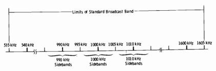
Fig. 1-1. Channels in standard broadcast band.
