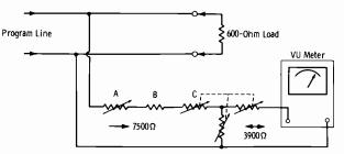
Fig. 2-13. External circuit of standard VU meter.
