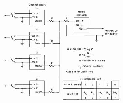
Fig. 6-14. Low-level mixing circuit, 1:1 impedance ratio.
