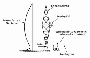
(A) Coil mounted on tower.
