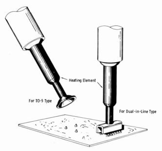
Fig. 13-13. Desoldering tools for integrated circuits.
