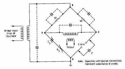
Fig. 14-5. Equivalent circuit of shielded rf bridge.
