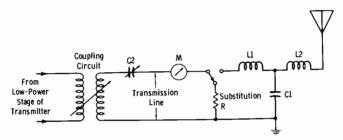
Fig. 14-7. Substitution method for adjusting antenna system.
