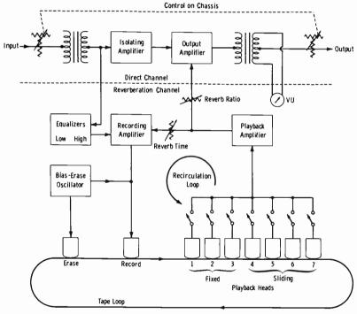
Fig. 11-13. Block diagram of tape reverberation unit.
