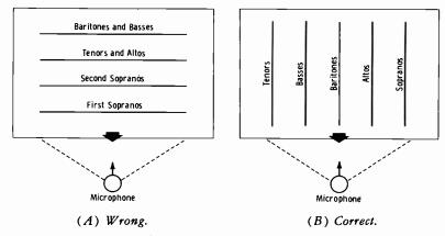
Fig. 11-21. Arrangement for choral pickups.
