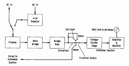
Fig. 14-12. Block diagram of noise-distortion meter.
