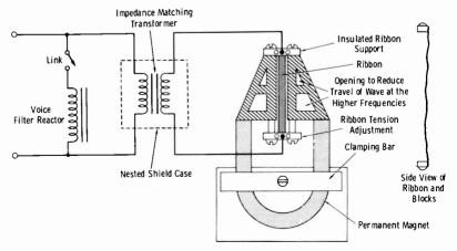
Fig. 4-8. Fundamental construction of ribbon microphone.
