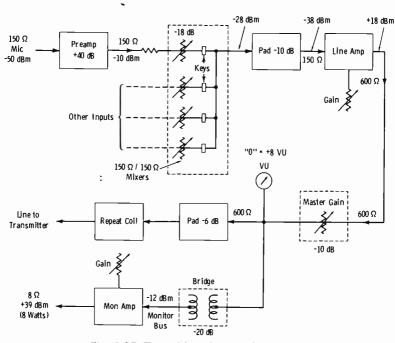
Fig. 6-35. Typical broadcast audio circuit.
