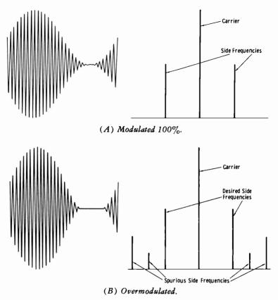
Fig. 9-35. Sidebands of amplitude-modulated carrier.
