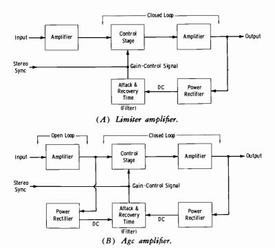
Fig. 6-37. Audio level-control devices.
