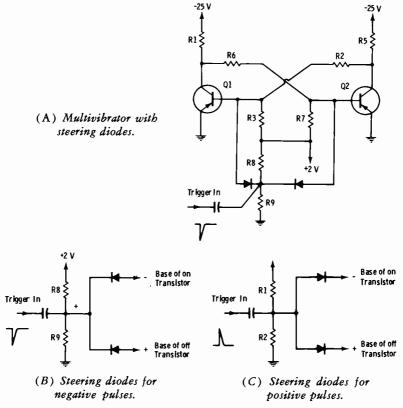
Fig. 3-61. Fundamentals of pulse steering.
