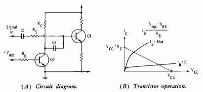
Fig. 6-41. Variable impedance with transistor.
