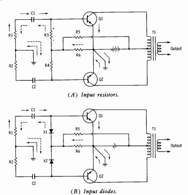
Fig. 3-19. Class-B amplifier with RC input coupling.
