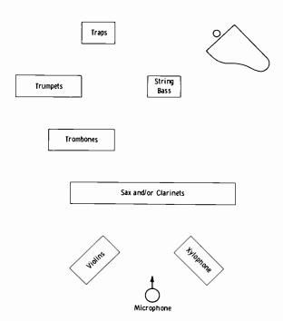
Fig. 11-17. Arrangement for small-orchestra pickup.
