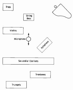
Fig. 11-18. Small-orchestra pickup with bidirectional microphone.
