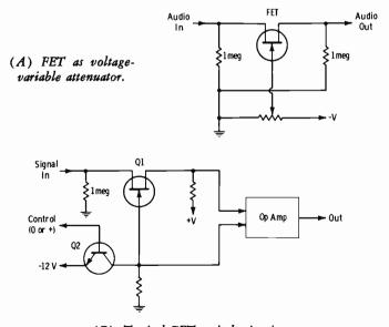
(B) Typical FET switch circuit.
