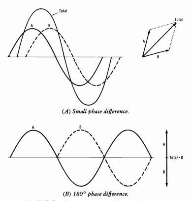
Fig. 11-7. Two harmonic motions of the same frequency.
