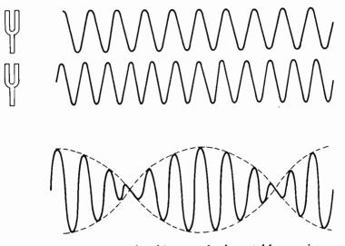
Fig. 11-3. Beat note produced from two fundamental frequencies.
