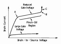
to provide a control element analogous to the grid of a vacuum tube. The FET also has a *source* (analogous to the cathode) and a *drain* (analogous to the plate). Note that the gate receives a voltage which is the reverse bias neccessary to control majority-carrier current in the *channel*.
