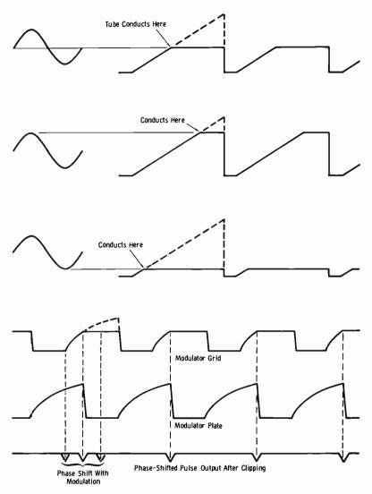
Fig. 10-16. Modulated sawtooth waveforms.
