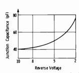
(B) Variable-capacitance diode.
