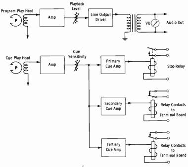
Fig. 5-12. Typical playback electronics in tape cartridge system.
