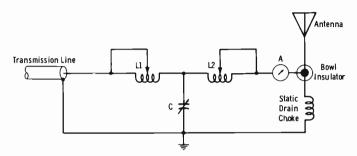
Fig. 9-13. Single-antenna tuning unit.
