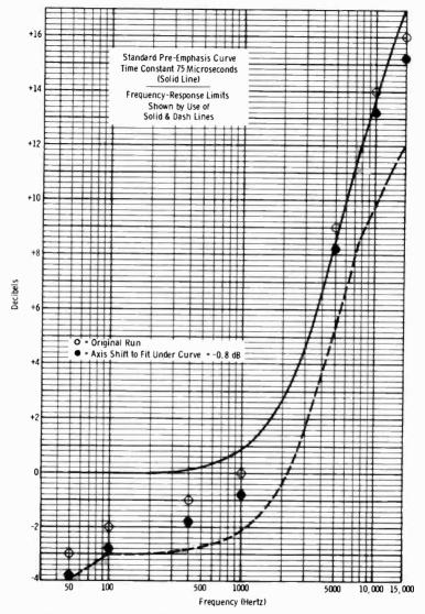
Fig. 14-20. Sample plot of frequency-response data for fm transmitter.
