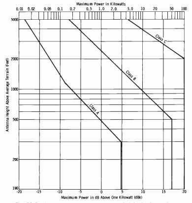
Fig. 10-1. Maximum power versus antenna height for fm stations.
