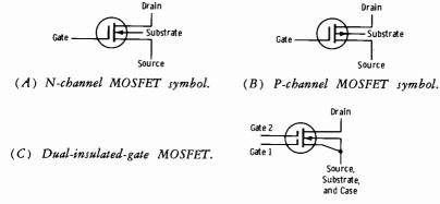
Fig. 3-16. Schematic symbols for MOSFETs.
