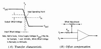
Fig. 3-55. Open-loop operational-amplifier operation.
