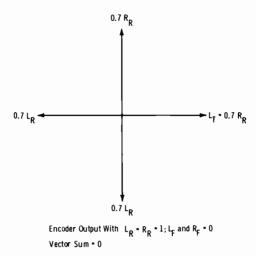
Fig. 7-8. Lack of "rear center" channel.
