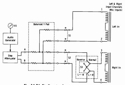
Fig. 14-26. Studio setup for stereo measurements.
