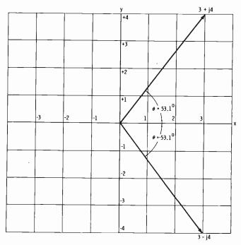
Fig. 2-10. Two vectors in rectangular form.
