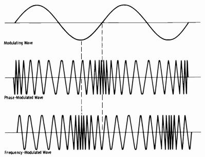
Fig. 10-13. Comparison of phase and frequency modulation.
