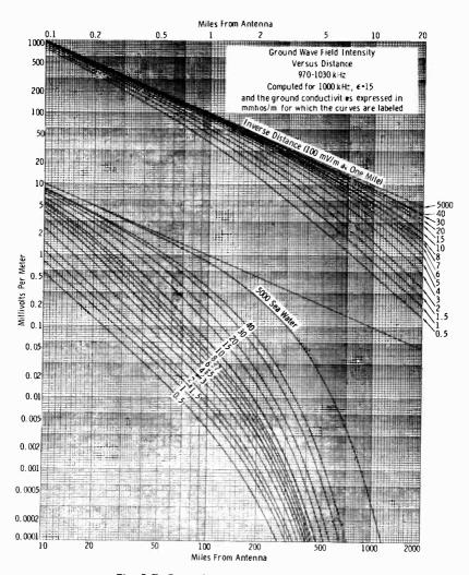
Fig. 9-7. Ground-wave field-intensity chart.
