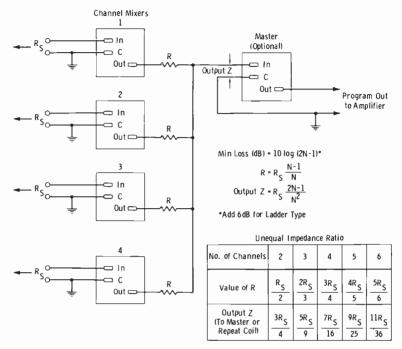
Fig. 6-15. Low-level mixing circuit, unequal impedances.
