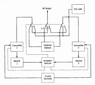
Fig. 9-37. Block diagram of CCA Dual Reliable transmitter.
