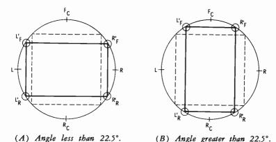
Fig. 7-17. Reproduced sound field simulation when gngle  $\theta$  is not 22.5°.
