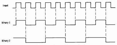
Fig. 3-63. Waveforms of binary circuits.
