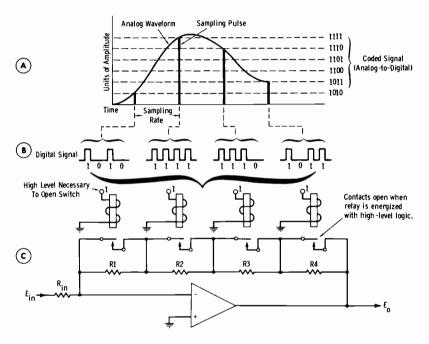
Fig. 3-58. Digital-to-analog conversion using operational amplifier with variable feedback controlled by relays.
