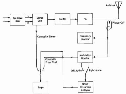
Fig. 14-27. Transmitter setup for stereo measurements.
