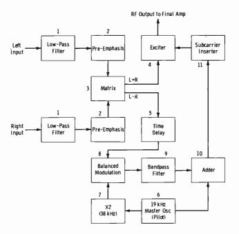
Fig. 10-30. Block diagram of basic stereo transmitter.
