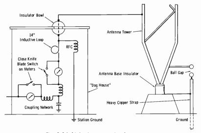
Fig. 9-14. Lightning protection for a-m tower.
