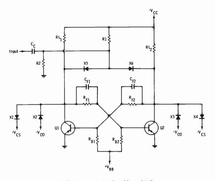
Fig. 3-62. Nonsaturating bistable multivibrator.
