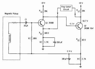
Fig. 6-32. Preamplifier for pickup.
