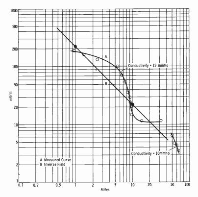
Fig. 14-10. Example of field-strength plot.
