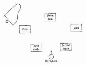
Fig. 11-15. Microphone placement for chamber orchestra.
