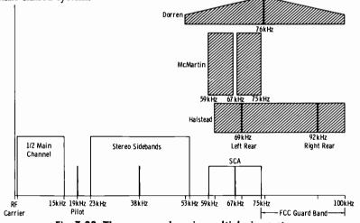
Fig. 7-22. Three proposed carrier multiplexing systems.
