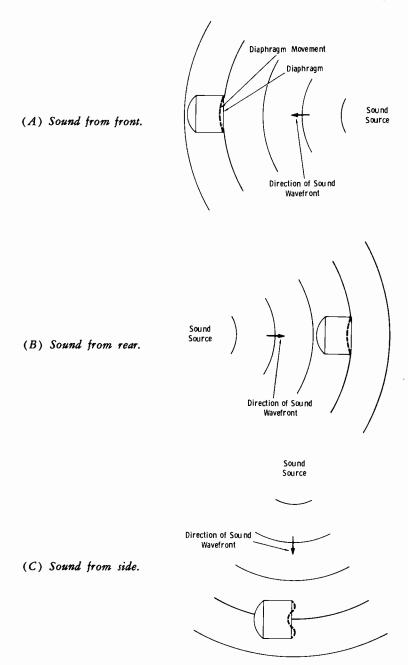
Fig. 4-11. Action of pressure microphone.
