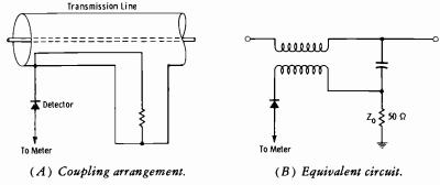
Fig. 10-27. Principle of directional coupler.
