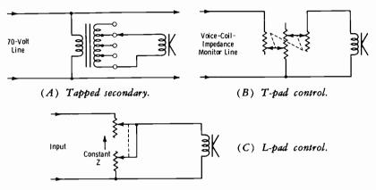
Fig. 6-49. Control of volume of individual speakers.
