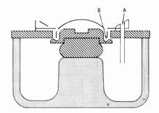
so that it vibrates freely in a magnetic field. This ribbon constitutes its own diaphragm; since it is not housed in any closed type of case and is exposed to the air on its two active sides, there are no adverse effects of cavity resonance, diaphragm resonance, or pressure doubling.
