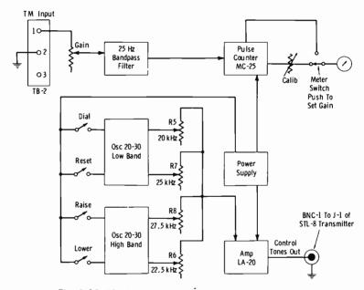
Fig. 8-29. Block diagram of remote-control studio unit.
