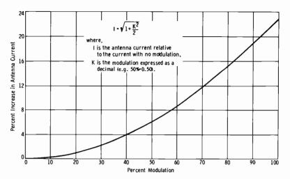
Fig. 9-27. Relation between antenna current and percentage modulation.
