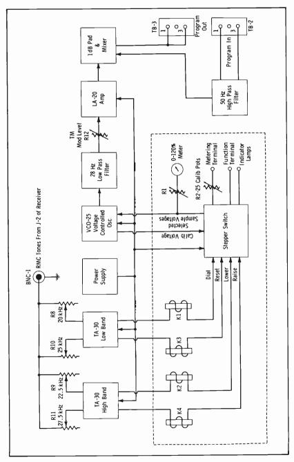
Fig. 8-30. Block diagram of remote-control transmitter unit.
