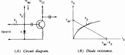
Fig. 6-40. Variable-impedance gain control.
