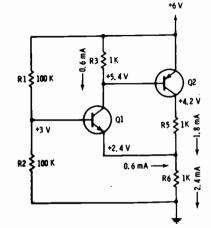
Fig. B-1. Dc equivalent of Fig. 3-69.
