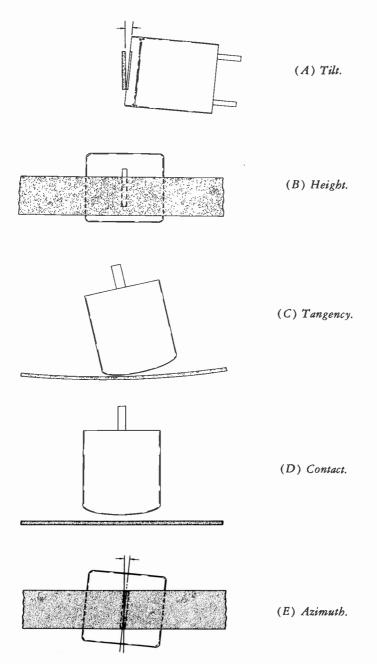
Fig. 13-20. Details of head adjustment planes.
