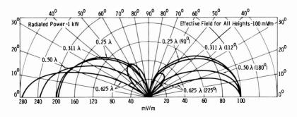
Vertical Radiation Patterns for Different Heights of Vertical Wire Antennas
