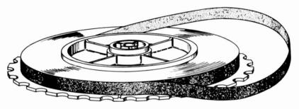
(B) Tape spliced in continuous loop.
