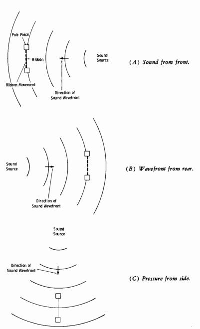
Fig. 4-12. Action of ribbon microphone.
