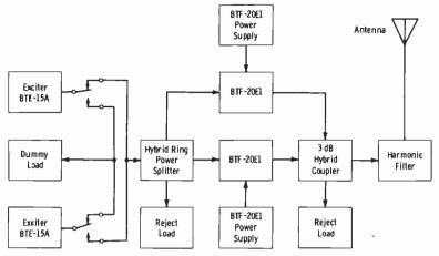
Fig. 10-25. Block diagram of RCA BTF-40E1 fm transmitter.
