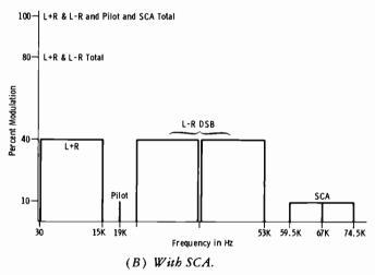
Fig. 10-29. Frequency distribution of fm stereo signal.
