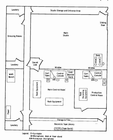
Fig. 1-2. Example of studio and control-room layout.
