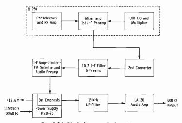
Fig. 8-26. Block diagram of stl receiver.
