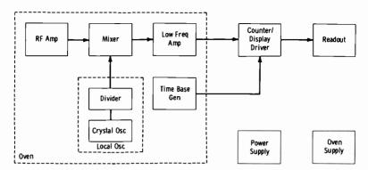
Fig. 9-41. Metron Model 520 digital a-m frequency monitor.
