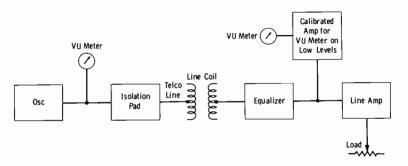
Fig. 8-15. Block diagram of line equalization.
