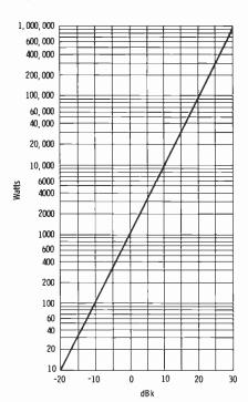
Fig. 2-18. Graph relating dBk to power in watts.
