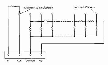
Fig. 6-11. Unbalanced ladder attenuator with cueing position.
