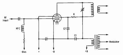
Fig. 9-28. Plate-screen modulation of rf pentode.
