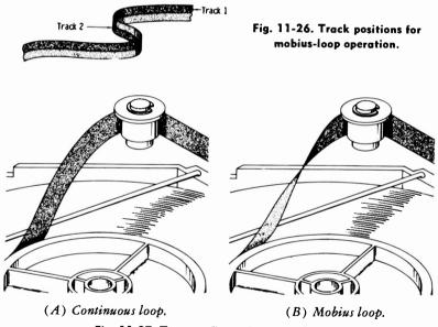
Fig. 11-27. Tape configuration around guide.
