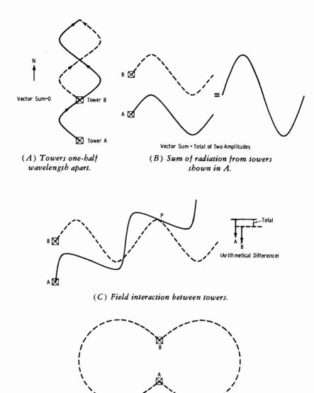
(D) Pattern in horizontal plane. Fig. 9-11. Simple directional array.
