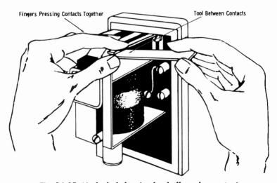
Fig. 14-35. Method of cleaning hard-alloy relay contacts.
