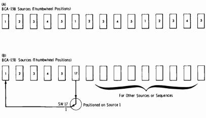
Both A and B continue to repeat a 5-source sequence, but 20-position recycling switch in B uses only six thumbwheel positions.
