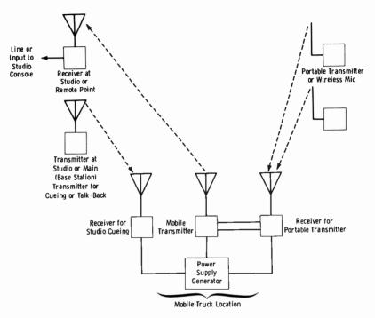
Fig. 8-10. Block diagram of remote-relay system.
