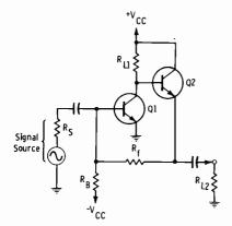
Fig. 3-4. Diagram of a feedback pair.
