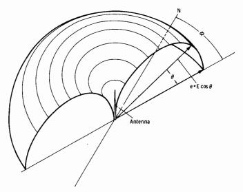
Fig. 9-4. Cross-section of radiation from a vertical antenna.
