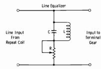
Fig. 6-17. Simplified representation of line equalizer.
