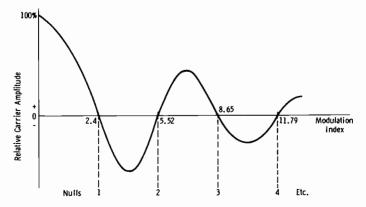
Fig. 14-30. Variation of carrier amplitude with modulation index.
