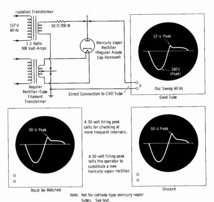
Fig. 14-33. Method of checking condition of mercury-vapor rectifier tube.
