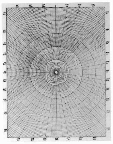
Fig. 2-21. Example of polar-coordinate paper.
