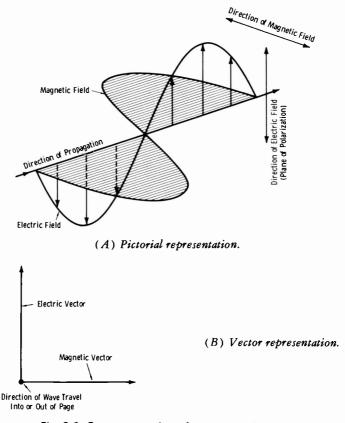
Fig. 9-3. Components of an electromagnetic wave.
