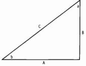
Fig. 2-6. Terminology applicable to trigonometric functions.
