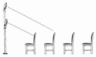
Fig. 11-16. Height and tilt adjustments.
