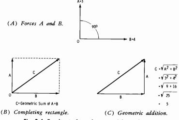
Fig. 2-4. Resultant of two forces at right angles.
