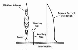
(B) Coil mounted on auxiliary mast.
