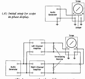
(B) Arrangement for phase-shift measurement.
