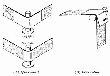
Fig. 13-24. Splice length and bend radius.
