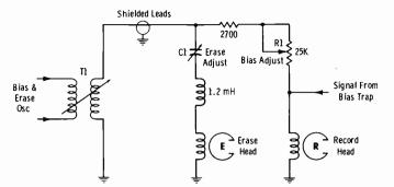
Fig. 5-8. Feeds to erase head and record head.
