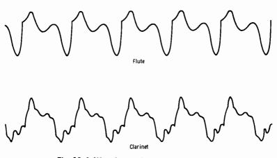
Fig. 11-4. Waveforms of two wind instruments.
