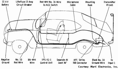
Fig. 8-9. Automotive installation of Marti remote-pickup transmitters.
