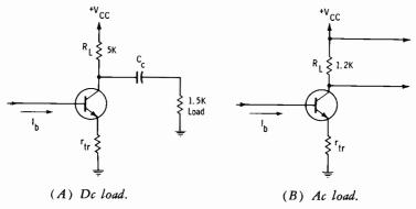
Fig. 3-6. Circuit equivalents for ac and dc gain.
