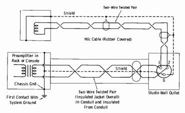
Fig. 6-50. Proper grounding of a microphone circuit.
