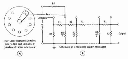
Fig. 6-10. Principles of unbalanced ladder attenuator.
