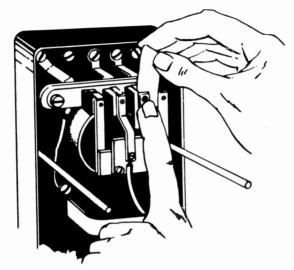
Fig. 14-34. Use of crocus-cloth strip for polishing relay contacts.
