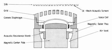
Fig. 4-5. Basic diagram of moving-coil microphone.
