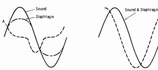
(A) Action under excessive pressure. (B) Action with normal loading.
