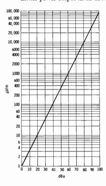
Fig. 2-17. Graph relating dBu to microvolts per meter.
