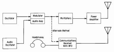
Fig. 14-31. Test setup for measurement of frequency deviation by
