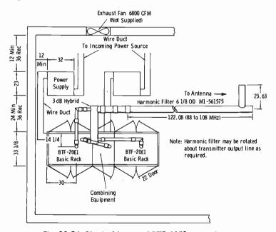
Fig. 10-26. Physical layout of BTF-40E1 transmitter.
