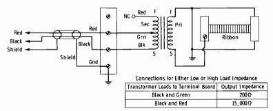
Fig. 13-2. Schematic diagram of a typical microphone.
