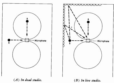
Fig. 11-10. Response patterns for a bidirectional microphone.
