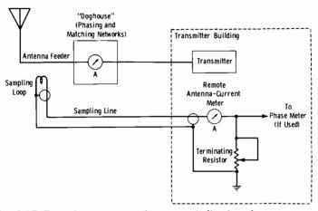
Fig. 9-17. Typical arrangement for remote indication of antenna current.
