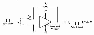
(A) Inverting input referenced to ground.
