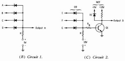
Fig. 3-52. Logic circuits for transmitter high voltage.
