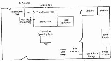
Fig. 1-4. Example of transmitter equipment layout.
