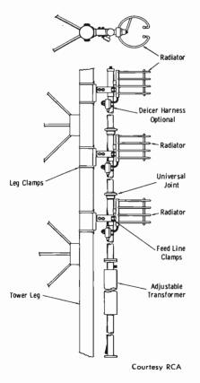
Fig. 10-4. Three-bay fm antenna side-mounted on tower.
