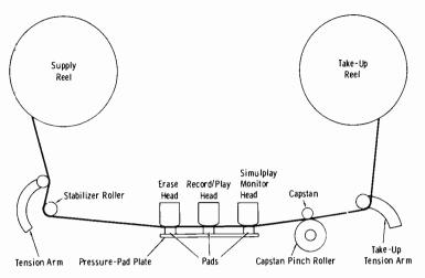
Note: Pressure pads are not used in many late model recorders.
