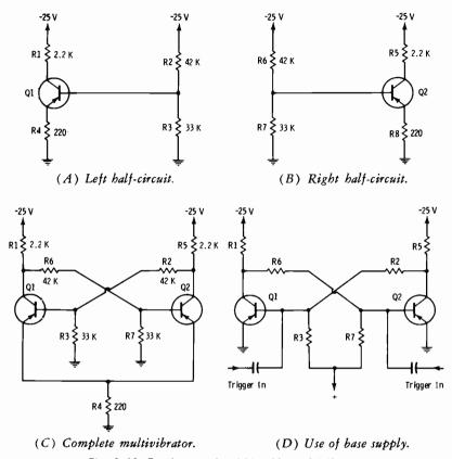
Fig. 3-60. Fundamentals of bistable multivibrator.
