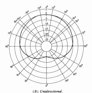
Fig. 11-9. Amplitude response of microphones.
