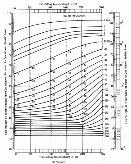
Estimated field strength exceeded at 50 percent of the potential receiver locations for at least 50 percent of the time at a receiving antenna height of 30 feet
