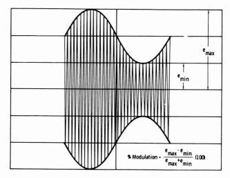
Fig. 9-34. Measurement of percent modulation.
