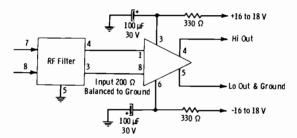
Fig. 7-3. Preamplifier for microphones.
