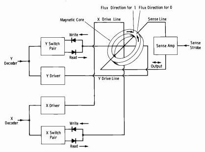
Fig. 3-65. Basic magnetic-core schematic.
