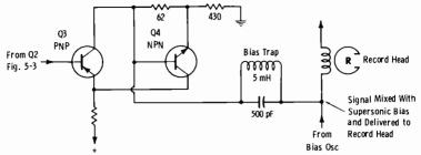
Fig. 5-6. Constant-current record-head amplifier.
