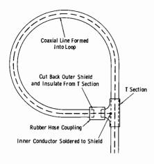
Fig. 9-18. A nonresonant pickup loop.
