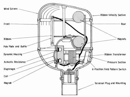
Fig. 4-14. Construction of cardioid microphone.
