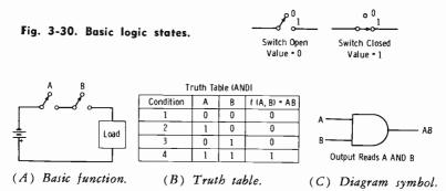
Fig. 3-31. Fundamentals of an AND circuit.
