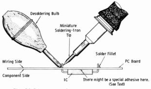
Fig. 13-14. Method for desoldering components.
