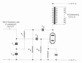
Fig. 137—Blumlein field output circuit
