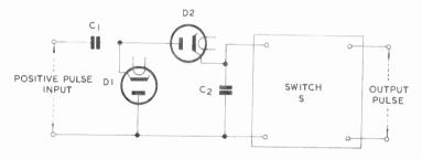
Fig. 1—Essential features of one type of step counter
