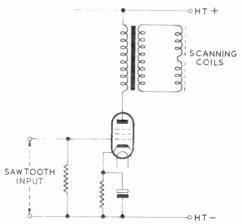
Fig. 138—Basic circuit for line output stage
