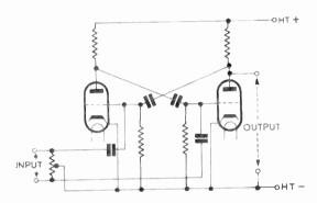
Fig. 33—Astable multivibrator with sync signals applied to the two grids in push-pull
