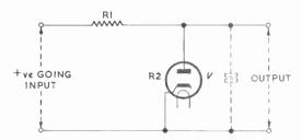
Fig. 64—Basic circuit for a gamma corrector using a diode
