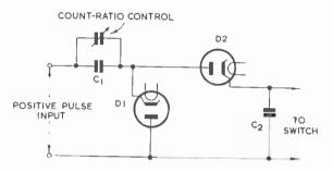
Fig. 3—One method of varying the count ratio in a step counter
