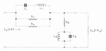
Fig. 108—Circuit of resonant constant-resistance equaliser
