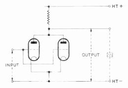
Fig. 156—Modulator consisting of two valves connected in parallel
