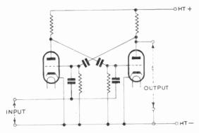
Fig. 31—Astable multivibrator frequency divider suitable for even division ratios
