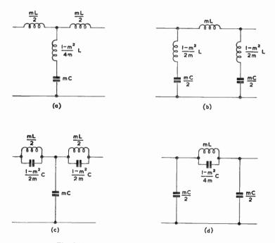
Fig. 84—Four basic types of m-derived section
