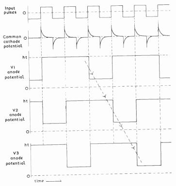
Fig. 9-Waveforms for ring counter of Figs. 7 and 8
