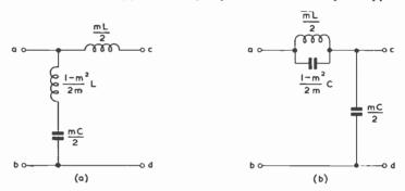
Fig. 86—Two basic forms of m-derived half-section
