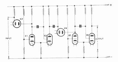
Fig. 24—A two-stage divider using cathode-coupled monostable multivibrators
