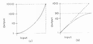
Fig. 61—Form of output signal obtained (a) when the overall gamma is too high and (b) when it is too low
