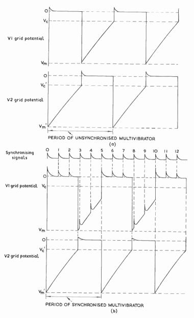
Fig. 30—Grid-potential waveforms for a symmetrical multivibrator (a) freerunning and (b) with synchronising signals applied to one control grid 50
