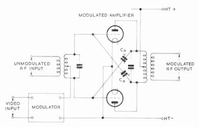
Fig. 149—Simplified circuit diagram of a class-C push-pull modulated amplifier
