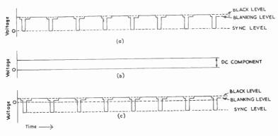
Fig. 38—A video signal for a dark scene is shown at (a); its d.c. and a.c. components are shown at (b) and (c)
