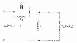
Fig. 100—Simple constant-resistance equaliser circuit
