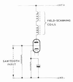
Fig. 125—Simple output stage with scanning coils connected directly in the anode circuit
