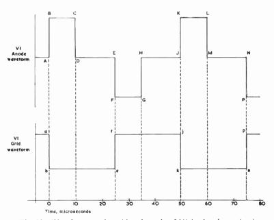
Fig. 93—Waveforms at the grid and anode of V1 in the above circuit
