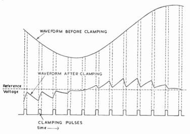
Fig. 54—Illustrating the action of a d.c. clamp
