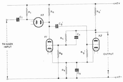
Fig. 22-A monostable multivibrator used as frequency divider
