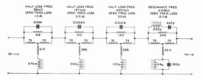
Fig. 110—Typical complete video constant-resistance equaliser
