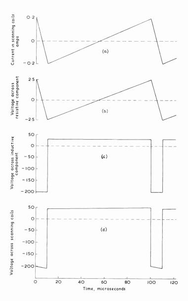
Fig. 124—Voltage waveforms in a pair of line-scanning coils fed with an ideal sawtooth current
