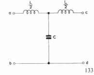
Fig. A.1 — Prototype low-pass T-section
