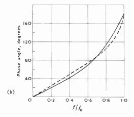
Fig. 82—The frequency response (a) and phase response (b) of a single low-pass section when terminated at both ends in an impedance  $Z_0$  (dotted) and when terminated in a resistance equal to  $\sqrt{(\mathbb{L}/\mathbb{C})}$  (solid)
