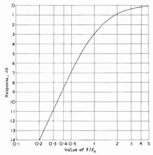
Fig. 101—Generalised frequency response for simple constant-resistance equaliser
