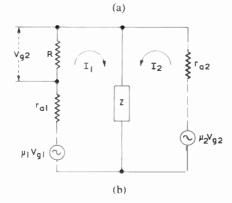
Fig. K.1—The simplified circuit diagram of one type of shunt-regulated amplifier is shown at (a) and its equivalent circuit at (b)
