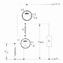
Fig. 155-Shunt-regulated amplifier with h.t. supply included
