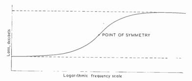
Fig. 105—General form of the curve for a "step" response
