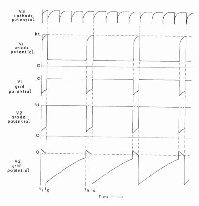
Fig. 23—Waveforms for the frequency divider of Fig. 22
