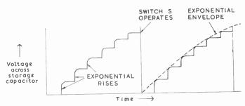
Fig. 2—Waveform across storage capacitor in step
