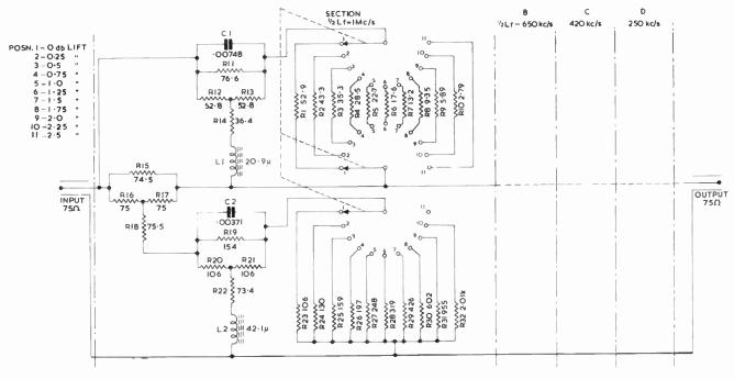
Fig. 121—Illustrating the component values in one section of a constant-resistance Bode-type variable equaliser
