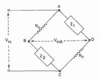
Fig. 95—Bridged circuit from which a number of constant-resistance networks can be derived
