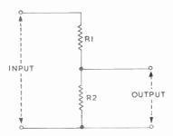
Fig. 63—A simple potential divider
