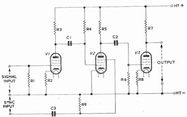
Fig. 72—Basic form of a negative-film gamma corrector employing a variable-ma valve as the non-linear device
