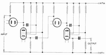
Fig. 27—A divider consisting of two cathode-coupled phantastrons in cascade
