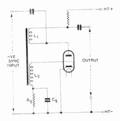
Fig. 36—Single-stage blocking-oscillator frequency divider
