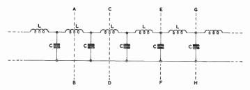
Fig. 79—A low-pass filter can be regarded as a succession of T-sections divided by lines such as AB and CD, or as a succession of  $\pi$ -sections when divided by lines such as EF and GH
