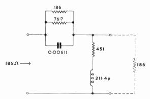
Fig. 107—Equaliser section giving 3-dB correction at a half-loss frequency of 420 kc/s, the iterative impedance being 186 ohms.
