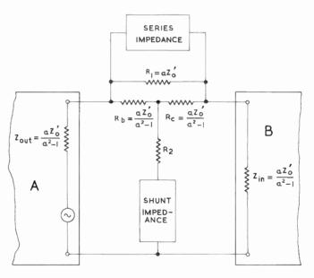
Fig. 118—Second step in modifying the network of Fig. 116 to constant-resistance form
