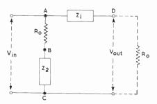
Fig. 97-The bridge circuit of Fig. 96 is usually drawn in this form
