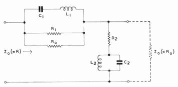
Fig. F.I—Resonant constant-resistance equaliser
