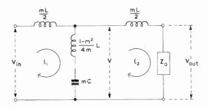
Fig. B.1—A series-derived T-section
