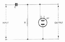
Fig. 44—Circuit of simplest type of d.c. restorer
