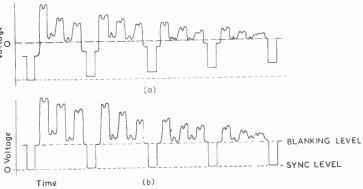
Fig. 42—A video signal with varying sync level is shown at (a) and the waveform after d.e. restoration at (b)
