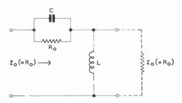
Fig. C.1—Simple constant-resistance equaliser
