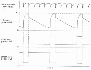
Fig. 26—Waveforms for the circuit of Fig. 25
