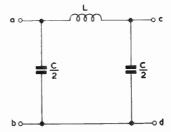
Fig. A.2—Prototype low-pass  $\pi$ -section
