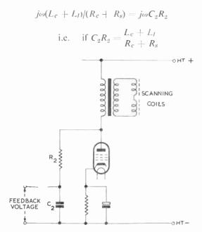
Fig. 135—Simple method of obtaining a feedback voltage from the primary winding of a scanning-coil output transformer
