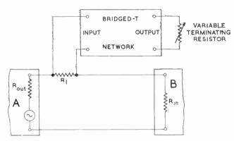
Fig. 115—A bridged-T network with variable terminating resistance can be used as the series element in a variable equaliser
