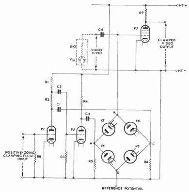
Fig. 53—One circuit for a d.c. clamp
