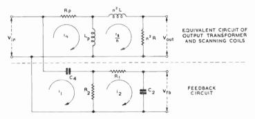
Fig. J.2—Simplified circuit equivalent to that of previous diagram
