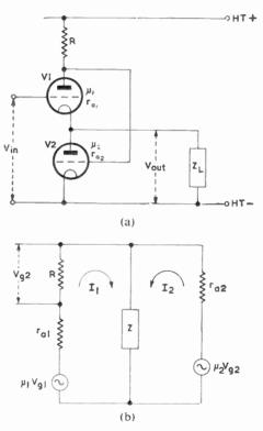
Fig. M.1—The basic circuit for a shunt-regulated cathode follower is shown at (a) and an equivalent circuit at (b)
