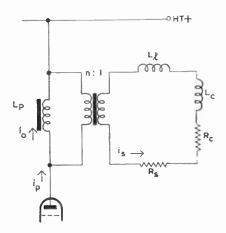
Fig. 127—Equivalent circuit of field output stage
