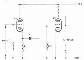
Fig. 51-Simplified circuit for d.c. restoration
