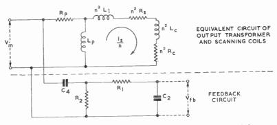
Fig. J.1—Blumlein circuit with output transformer replaced by equivalent network
