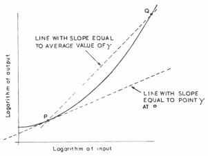
Fig. 59—Illustrating the meaning of point gamma
