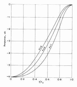
Fig. 109—Some frequency response curves for a resonant equaliser
