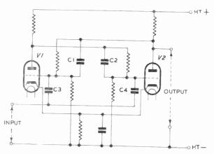
Fig. 10—Basic circuit for a binary counter
