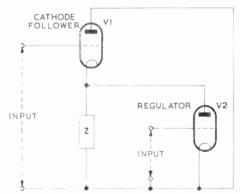
Fig. 159—Development of the circuit of a shunt-regulated eathode follower: stage 1
