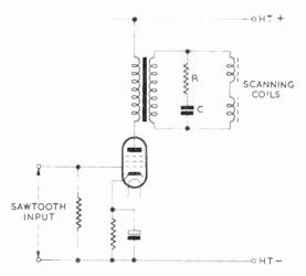
Fig. 143—Improved circuit of simple line output stage
