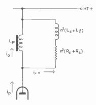
Fig. 128—Equivalent circuit of field output stage with all secondary loads referred to the primary side
