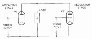
Fig. 152—Basic circuit of shunt-regulated amplifier
