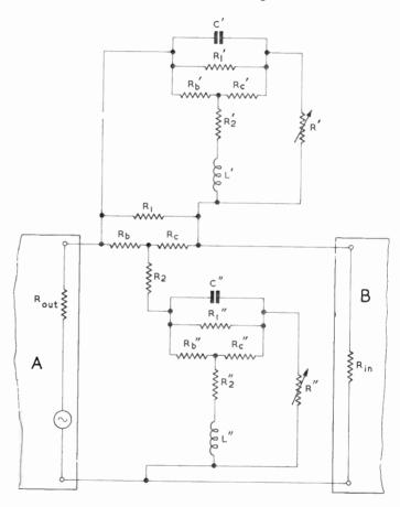
Fig. 120—Complete circuit of constant-resistance Bode-type variable equaliser 178
