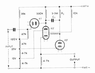
Fig. 25—Cathode-coupled phantastron frequency divider
