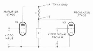
Fig. 153—Basic circuit of shunt-regulated amplifier illustrating one method of obtaining the input signal for the regulator stage
