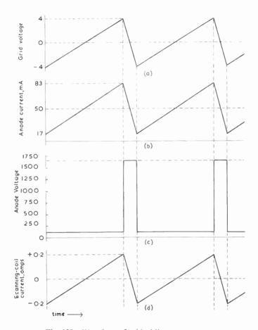
Fig. 139—Waveforms for ideal line output stage
