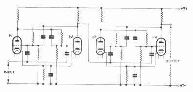
Fig. 12—Binary counter for dividing by four
