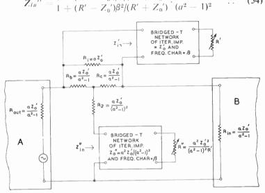
Fig. 119—Final form of constant-resistance Bode-type variable equaliser
