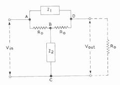
Fig. 99—Bridged-T network obtained by connecting a resistor R<sub>0</sub> between terminals B and D in Fig. 96
