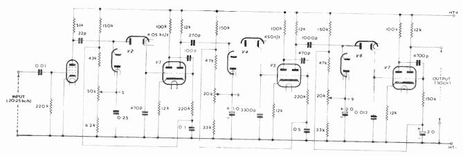
Fig. 5—Cascade step divider using multivibrator switches and dividing by 405
