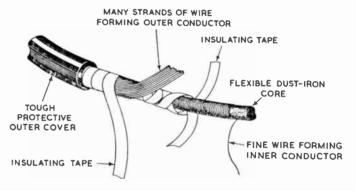
Fig. 75—Construction of a delay cable
