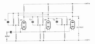
Fig. 7-Ring circuit for dividing by three
