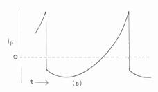
Fig. 132—Primary current waveforms needed to give a sawtooth secondary current for (a) a large primary inductance and (b) a small primary inductance
