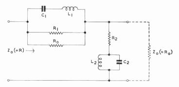
Fig. E.1—Resonant constant-resistance equaliser
