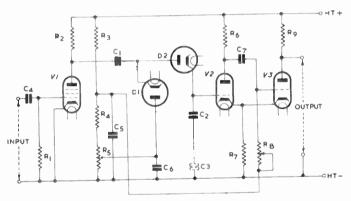
Fig. 4—Step divider using a multivibrator switch
