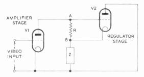
Fig. 154—Fundamental circuit of shunt-regulated amplifier with all d.c. feeds omitted
