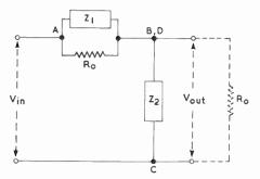
Fig. 98—Alternative form of constant-resistance L-network obtained from the bridge circuit of Fig. 96 by short-circuiting terminals B and D
