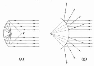
Fig. 5. Reflection of Sound Waves from Curved Surfaces
