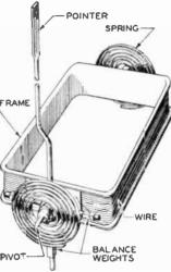
Fig. 4. Enlarged Detail of the Moving Coil of a D'Arsonval Instrument
