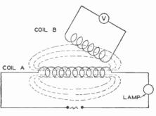
Fig. 6. Method of Exploring a Magnetic Field around a Coil
