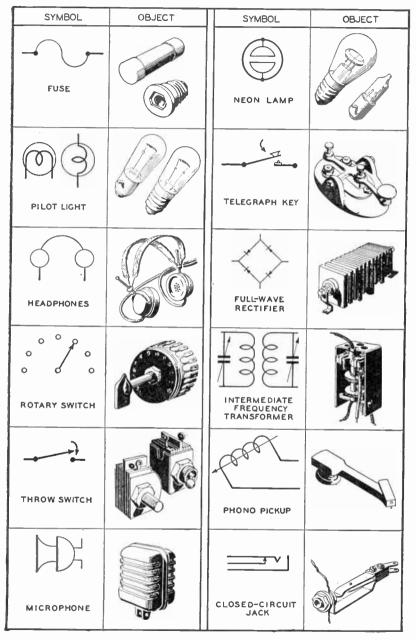
Fig. 3. Radio Symbols for Fuse, Lamps, Switches, Microphone, Rectifier, and Jack
