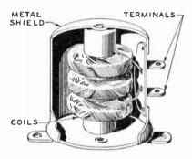
Fig. 4. Radio-Frequency Choke Coil
