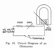
higher. battery voltage as well as the dropping voltage encountered during use. It must be remembered that the total 4500ohm resistance which includes the 50-ohm coil resistance must be placed in series with the 4.5volt source as shown in Fig. 10. Closing the series circuit (joining the terminals together) will permit 1 milliampere of current to flow and the pointer of the
