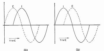
Fig. 3. Diagram Showing Effect of Inductance and Capacitance in an Aiternating-Current Circuit
