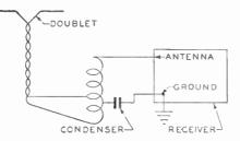
Fig. 8. Antenna System Providing Noise Reduction on Only Short-Wave Bands
