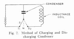
caused or produced by continuous direct current supplied by a battery, as shown in Fig. 2. Two separate circuits are included in Fig. 2. If the switch arm S is thrown to position  $S_1$ , current will flow from the battery to the condenser until the potential difference
