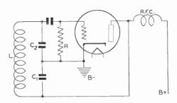
Fig. 7. Colpitts Oscillator Using Capacitive Feedback
