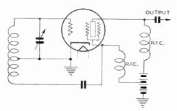
Fig. 12. Electron-Coupled Oscillator
