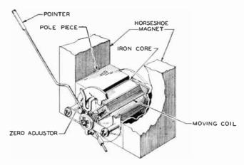
Fig. 3. Enlarged Detail of D'Arsonval-Meter Movement
