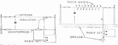
Fig. 2. Counterpoise Antenna System Fig. 3. Action of Radio Waves on Antenna
