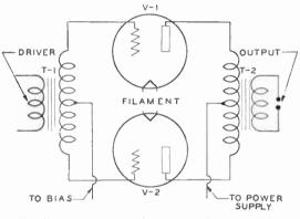
Fig. 9. Diagram Showing a Push-Pull Amplifier Stage
