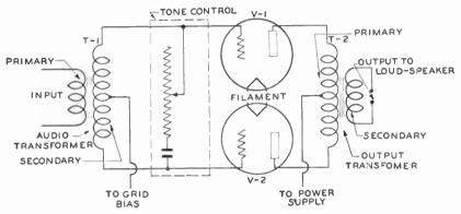
Fig. 14. Tone Control Connected Across the Secondary of Audio or Input Transformer in a Push-Pull Amplifier Stage
