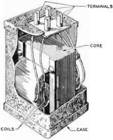
Fig. 7. Iron-Core Transformer
