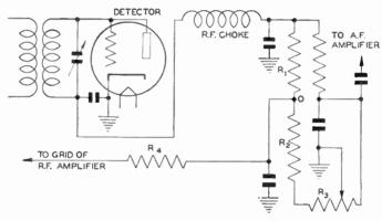
Fig. 12. Automatic Volume-Control Circuit
