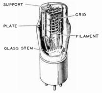
Fig. 4. Illustration Showing Triode Tube and Arrangement of Filament, Grid, and Plate
