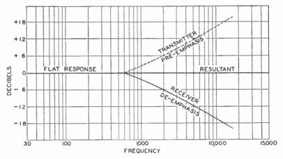
Fig. 8. Curve Showing Resultant in Response to Pre-emphasis at Transmitter and De-emphasis at Receiver
