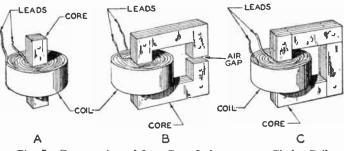
Fig. 7. Construction of Iron-Core Inductance or Choke Coil
