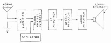
Fig. 1. Route of Radio Signal Through Superheterodyne Receiver
