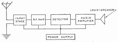
Fig. 1. Block Diagram of Units of Radio Receiver
