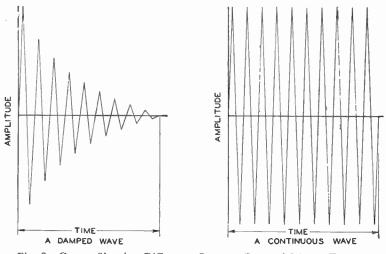
Fig. 2. Curves Showing Difference Between Damped Wave (Type B) and Continuous Wave (Type A)
