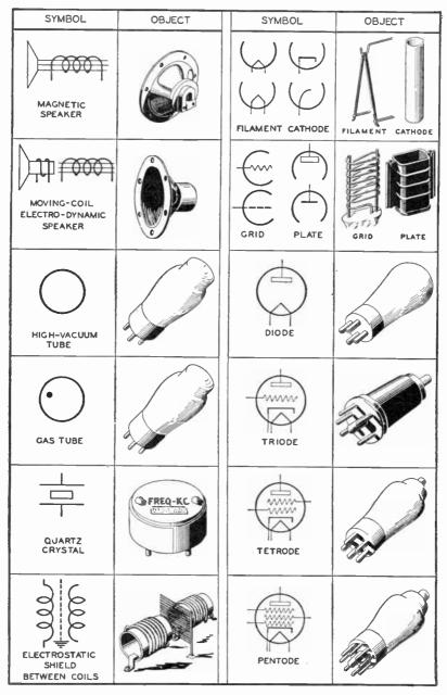
Fig. 4. Radio Symbols for Speaker, Shield, and Tubes
