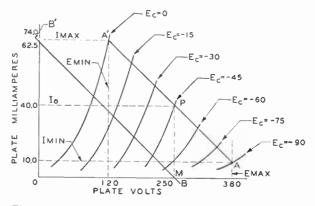
Fig. 10. A Group of Plate-Voltage Plate-Current Curves Obtained with Different Grid-Bias Voltages
