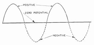
Fig. 3. Sine-Wave Alternating Current
