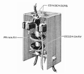
Fig. 7. Intermediate-Frequency Transformer
