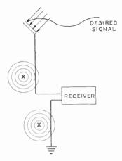
Fig. 6. Electrical Disturbances at Points Marked X Enter Receiver with Desired Signal and Issue from Speaker as Annoying Interference
