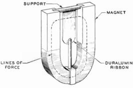
Fig. 8. Diagram Illustrating Principle of a Velocity Microphone
