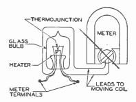
Fig. 9. This Diagram Shows Connections of a Thermocouple-Type Meter
