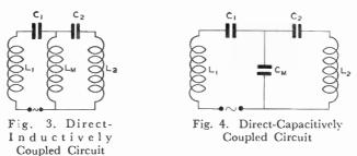
**Direct-Capacitive Coupling.** Similar to direct-inductive coupling is the transfer of energy by capacitive coupling—that form of coupling that employs capacitances. Fig. 4 shows a circuit in which the capacitance  $C_{M}$  is common to the primary and the secondary circuits, thus forming a *direct-capacitively coupled* circuit. The transfer of energy in such a circuit is obtained by electrostatic means, and utilizes the effect of alternately charging and discharging the condenser  $C_{M}$ .
