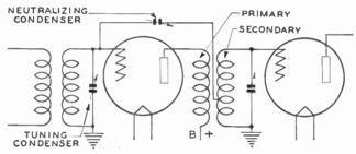
Fig. 4. Neutrodyne Method of Controlling Feedback
