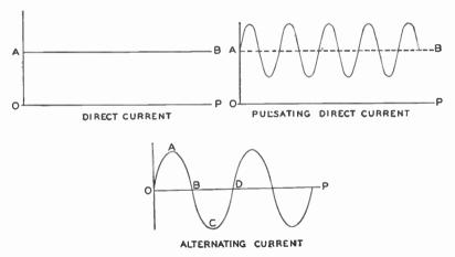
Fig. 1. Diagrammatic Views of Direct Current, Pulsating Direct Current, and Alternating Current
