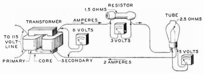
Fig. 15. Diagram Shows Circuit Consisting of Radio-Power Transformer, Resistor, and Tube
