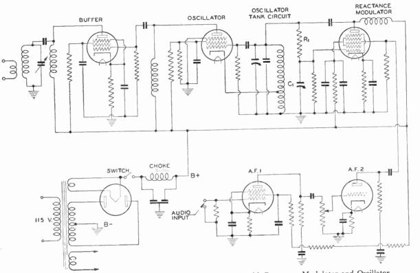
Fig. 2. Circuit Diagram of Frequency-Modulation Transmitter, with Reactance Modulator and Oscillator
