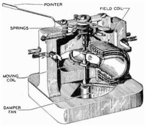
Fig. 7. Interior View of a Dynamometer Type Instrument
