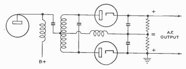
Fig. 6. Discriminator Stage of Frequency-Modulation Receiver
