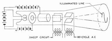
Fig. 14. Sweep Circuit Used to Produce Pattern on Fluorescent Screen
