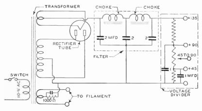
Fig. 6. Wiring Diagram of Power-Supply Unit of Radio Set
