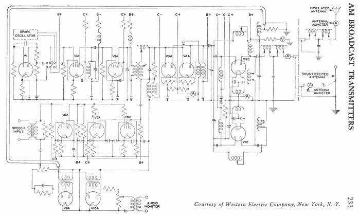
Fig. 3. Schematic Circuit Diagram of 405B-2, 5-Kilowatt Radio Transmitting Equipment
