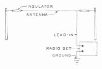
Fig. 1, Simple Antenna System
