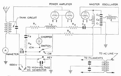
Fig. 4. Master-Oscillator, Power-Amplifier Radiotelegraph Transmitter
