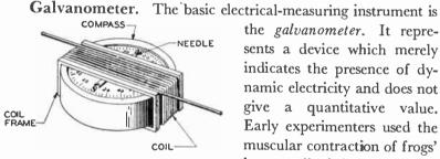
Fig. 1. A Tangent Galvanometer
