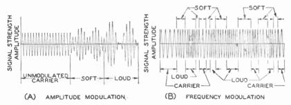
Fig. 1. Comparison of Amplitude Modulation and Frequency Modulation. (A) Shows, at Left, the Unmodulated Carrier; Next, Low-Percentage Modulation of Carrier Produced by Soft Tone; at Right, High-Percentage Modulation Produced by Loud Tone. Note That Frequency Is Unchanged. (B) Frequency Deviation of Carrier Caused by Application of Modulation. Note That Amplitude Remains Constant.
