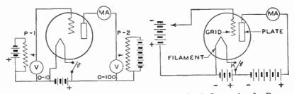
Fig. 5. Radio-Tube Test Circuit for Determining the Amplification Factor of the Tube
