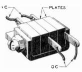
Fig. 8. Enlarged View of a Copper Oxide Rectifier Used with a D'Arsonval Instrument
