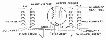
Fig. 1. Radio-Frequency Amplifier Circuit
