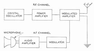
Fig. 2. Block Diagram of Radiotelephone Transmitter
