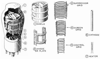
Fig. 12. A Cutaway View of a Pentode Tube and Enlarged Detail of the Separate Parts
