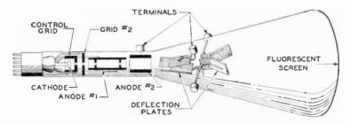
Fig. 13. Cathode-Ray Tube of an Oscilloscope
