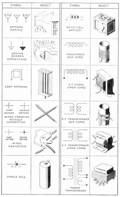
Fig. 1. Symbols of Antenna, Ground, Wires, Cells, Batteries, Transformers
