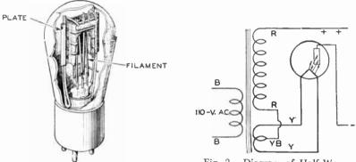
Fig. 1. Half-Wave Diode Rectifier Tube
