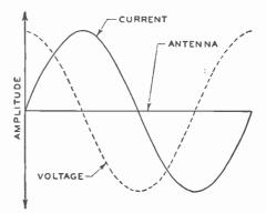
Fig. 2. Voltage and Current Distribution in Hertz Antenna Operating as a Half-Wave Antenna System
