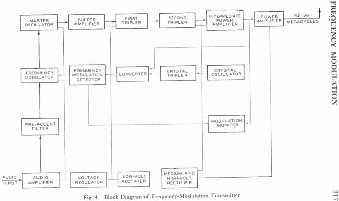
Fig. 4. Block Diagram of Frequency-Modulation Transmitter
