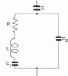
Fig. 9. Quartz-Crystal Oscillator
