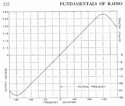
Fig. 7. Curve Showing Output Voltage Produced Due to Variation in Frequency of Signal
