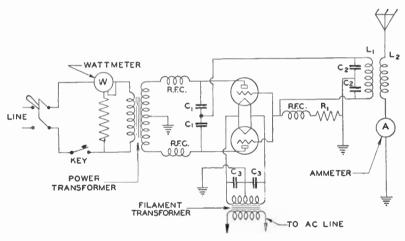
Fig. 3. Self-Rectifying Radiotelegraph Transmitter
