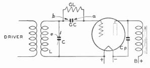
Fig. 6. Diagram of Grid-Leak, Condenser Detector Circuit
