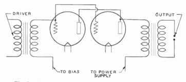
Fig. 8. Diagram Showing a Plate Circuit Using Two Power Tubes in Parallel
