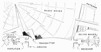
Fig. 1. How Radio Programs Are Transmitted to the Listener
