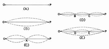
Fig. 6. Diagram Showing How Harmonics and Overtones Are Produced
