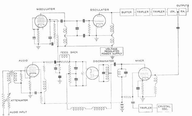
Fig. 3. Schematic Diagram of Frequency-Modulated Transmitter
