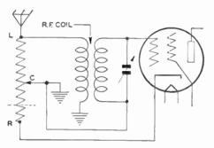
Fig. 8. Combination of Antenna and Grid-Bias Control
