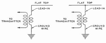
(A) INVERTED-L TYPE (B) T TYPE Fig. 1. Two Types of Marconi Transmitting Antennas
