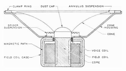
Fig. 4. Cross Section of Electrodynamic Speaker
