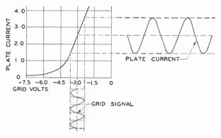
Fig. 5. Showing Type of Signal Produced When a Tube Is Operated on Straight Portion of Characteristic Curve
