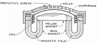
Fig. 7. Cross-Section of a Dynamic Type Microphone
