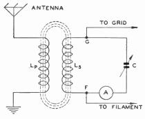
Fig. 2. Antenna Tuning Circuit
