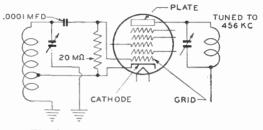
Fig. 4. Oscillator and Output Circuit of 12SA7 Tube
