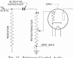
Fig. 10. Resistance-Coupled, Audio, Volume-Control Circuit
