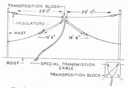
Fig. 5. Double-Doublet Type of Antenna
