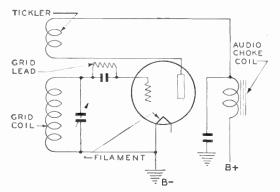
Fig. 5. Armstrong Regenerative Circuit The plate circuit coil is called the "tickler coil" and provides feedback.
