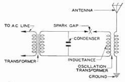
Fig. 1. An Early Spark-Gap Transmitter
