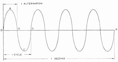
Fig. 2. Diagram Showing Four Cycles of Alternating Current
