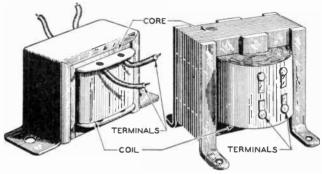
Fig. 3. Audio Transformers (Iron Core)
