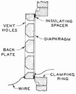
Fig. 4. Cross-Section of a Condenser Type Microphone
