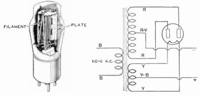
Fig. 4. Full-Wave Diode Rectifier Tube
