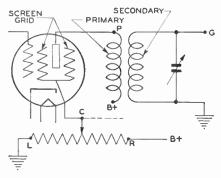
Fig. 9. Screen-Grid and Plate-Circuit Control
