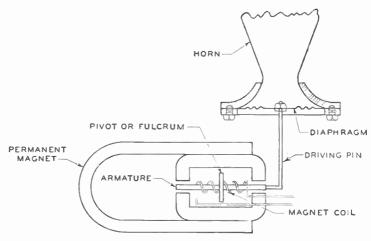
Fig. 3. Balanced-Armature Type of Speaker Unit
