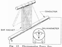
Fig. 12. Electromotive Force Produced by a Moving Magnetic Field
