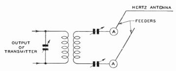
Fig. 4. Series-Tuned Zeppelin Type of Feed System for Antenna
