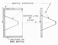
Fig. 5. Box- and Flat-Type Baffles
