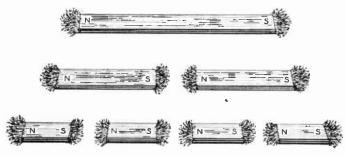
Fig. 2. Results of Breaking a Bar Magnet. Showing Iron Filings Clinging to Ends of Broken Bars
