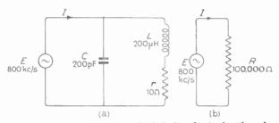
Fig. 8.12—The circuit composed of C, L and r having the values marked (a) can at  $800 \ ke/s$  be replaced by a high resistance (b), so far as the phase and magnitude of the current taken by the generator is concerned
