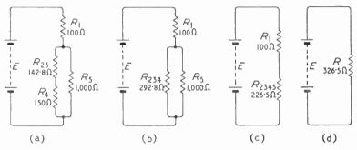
Fig. 2.10—Successive stages in simplifying the circuit of Fig. 2.9.  $R_{11}$  stands for the single resistances equivalent to  $R_1$  and  $R_2$ ; and so on. R represents the whole system
