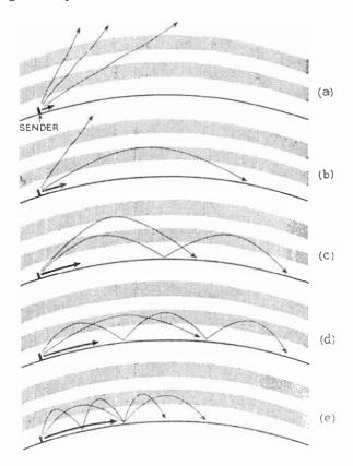
Fig. 15.11—Showing (not to scale) the relative ranges of ground wave and reflected wave from very high frequencies (a) to very low (e)
