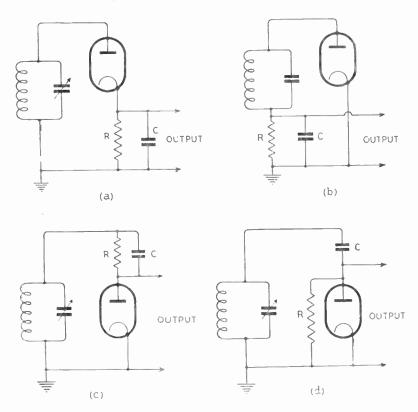
Fig. 16.8-The principal varieties of diode detector circuit
