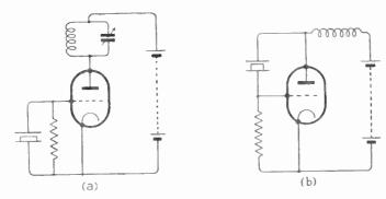
Fig. 13.4-Two types of crystal-controlled oscillator circuit
