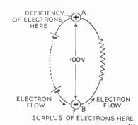
Fig. 3.1—Before a p.d. can be established between any two parts of a circuit (such as A and B) they must be charged, and when the p.d. is rapidly varied the charging current may be important
