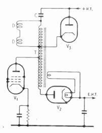
Fig. 23.9—Typical e.h.t. generator in television receiver, making use of line fly-back
