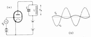
Fig. 12.4—Diagram b shows the relative amplitude and phase of grid and anode voltages when their frequency is the same as the natural frequency of the circuit LC
