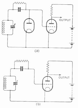
Fig. 16.9—If a diode detector (Fig. 16.8c variety) is connected straight to a triode amplifier (a), the grid-cathode path of the triode renders a separate diode unnecessary; this is what happens in the grid type of detector (b) 216
