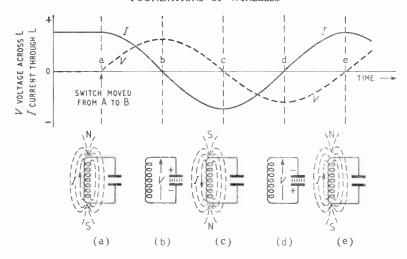
Fig. 12.2—Sequence of events in Fig. 12.1 after the switch has been moved to B. Stages a to e cover one complete cycle of oscillation
