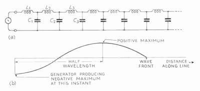
Fig. 14.5—(a) Electrical representation of the generator end of a transmission line, and (b) instantaneous voltage (and current) diagram  $\frac{3}{4}$  of a cycle from the start of generating a sine wave
