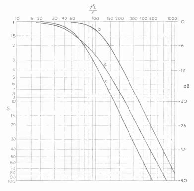
Fig. 19.12—Comparison between the overall resonance curve for a pair of similar tuned circuits, (a) uncoupled, and (b) "critically" coupled. Curve c is the same as b but shifted to the left to represent a halving of resistance
