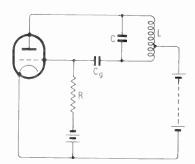
Fig. 12.6—The series-fed Hartley circuit, showing parallel-fed grid bias using a grid leak R and capacitor Cg
