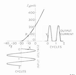
Fig. 13.1 — Illustrating "Class B" operation with the aid of a valve anodecurrent/grid-voltage characteristic curve
