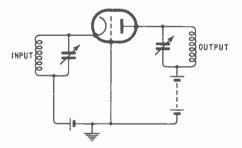
Fig. 19.9—Common-grid amplifier circuit
