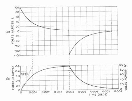
Fig. 4.9—Curves showing the current and voltage in the circuit of Fig. 4.8 when the switch is moved first to A and then to B
