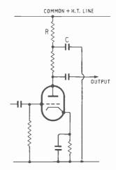
Fig. 23.10—Decoupling a valve from the b.t. line is performed by inserting R to block signal currents, and providing C to give them a path back to earth
