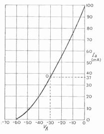
Fig. 20.2—Typical characteristic curve of a triode, showing nonlinearity. If the working point is O (as a result of applying a grid bias of —30 V), a 30 V positive half-cycle of signal on the grid would increase the anode current by 62 mA, but an equal negative half-cycle would decrease it by only 37 mA; see Fig. 20.3
