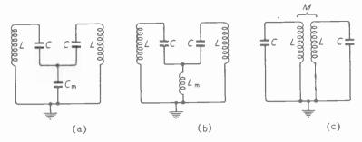
Fig. 19.11—Three methods of coupling two tuned circuits: (a) by capacitance common to both,  $C_M$ ; (b) by common inductance,  $L_M$ ; and (c) by mutual inductance, M
