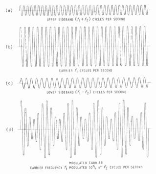
Fig. 18.2—Showing that a modulated carrier wave (d) is identical with three unmodulated waves (a, b and c) added together
