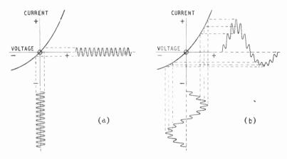
Fig. 19.4—Showing the effect of adding a strong signal to a weak signal through a nonlinear device such as a valve. The amplitude of the weak signal is varied (or modulated) by the strong
