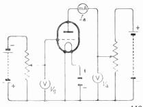
Fig. 9.4— Circuit for taking characteristic curves of a triode
