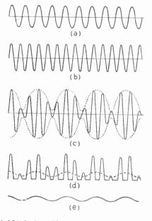
Fig. 19.1—Showing the action of a frequency-changer
