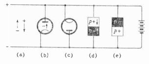
Fig. 10.7—Showing how in diodes the presence or absence of current depends on the presence or absence of the right kind of current-carriers
