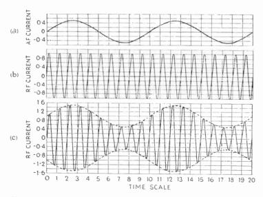
Fig. 13.5—Curve a represents two cycles of audio-frequency current, such as might be flowing in a microphone circuit; b represents the much larger number of radio-frequency cycles generated by the sender. When these have been amplitude-modulated by a, the result is as shown at c
