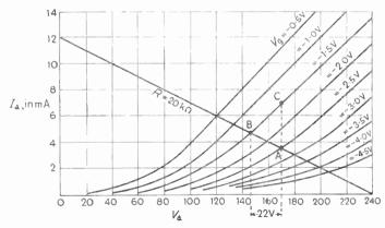
Fig. 11.2—The problem of finding the amplification of the valve in Fig. 11.1 is here worked out on an  $J_a/V_a$  curve sheet
