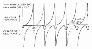
Fig. 14.8—Showing how the reactances of short-circuited and opencircuited lines vary with their length
