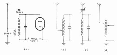
Fig. 13.10—Some of many varieties of method in coupling aerial to sender. a is the inductive coupling or r.f. transformer method, worked out in the text for a particular example; b is the aerial tapping or auto-transformer; c is the series capacitor method; and at d the valve is tapped down to reduce the effective load resistance
