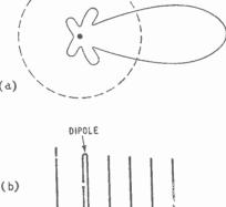
array shown in Fig. 15.10b, which is called a Yagi aerial. Its polar diagram (a) shows a very considerable advantage over that of the single dipole.
