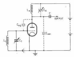
Fig. 17.4—The effect of  $C_{\rm ao}$  in Fig. 17.2 can be overcome by substituting a tuned coupling for the resistance, but there is still trouble due to  $C_{\rm ag}$
