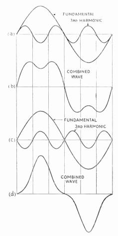
In most sets the voltage needed to drive the output valve fully is not more than about 10 V, so the a.f. amplifier does not have to work very hard, and there is seldom any difficulty in keeping non-linearity within tolerable limits. This kind of distortion will therefore be considered in connection with the output stage where it is the main problem. We shall concentrate now on frequency distortion.
