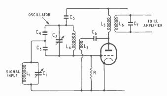
Fig. 19.5—Typical additive frequency-changer, in which a single valve serves as both modulator and generator of the local oscillations
