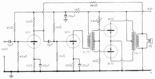
Fig. 22.11—Circuit diagram of a three-stage transistor a.f. amplifier, similar in configuration to a valve amplifier but requiring only a small fraction of the power supply. Junction transistors with common cmitter are used for all stages. (Courtesy of Messrs. Mullard Ltd.)
