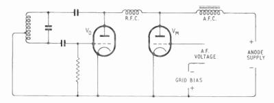
Fig. 13.7—Anode modulation, sometimes called "choke control" modulation. RFC is a r.f. choke for keeping r.f. current out of the modulator circuit
