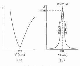
Fig. 8.13 — Plotting the current and impedance of the Fig. 8.12a circuit as a whole at various frequencies gives the shapes shown here:
