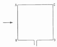
Fig. 15.16—The effectiveness of a receiving aerial consisting of a loop or coil of wire depends on the direction from which the waves are arriving
