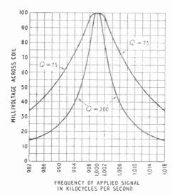
Fig. 8.7—In this diagram the curve "Q=200" is the same as in Fig. 8.6, but, to enable the selectivity of the Q=75 circuit to be more easily compared, the voltage injected into it has been raised from 0.5 mV to 1.33 mV, so as to make the output voltage at resonance equal to that across the Q=200 circuit
