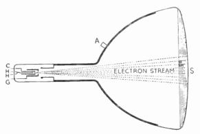
Fig. 21.1—Section of typical cathode-ray tube, H=heater; C=cathode; G=grid; A=anode; S=fluorescent screen
