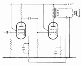
Fig. 20.17—In this negative feedback circuit the whole of the voltage across the loudspeaker is fed back to the last stage but one
