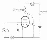
Fig. 11.1—Simple voltage-amplifier circuit
