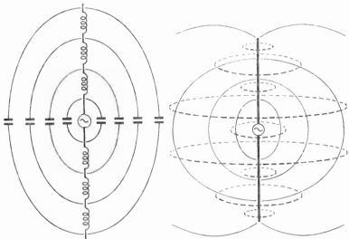
Fig. 15.3—Approximate representation of the distributed inductance and capacitance in the half-wavelength system of Fig. 15.2
