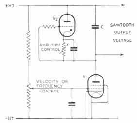
Fig. 21.7—Outline circuit of sawtooth generator
