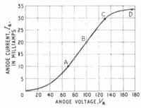
Fig. 9.3—Characteristic curve of a diode
