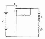
Fig. 4.8—Circuit used for studying the rise and fall of current in an inductive circuit
