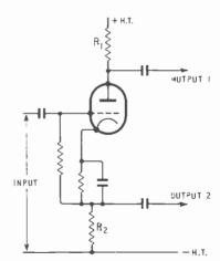
Fig. 20.21—The "concertina" phase-splitter circuit as an alternative to the transformer T<sub>1</sub> in F g. 20.20
