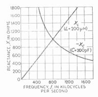
Fig. 8.5—Reactances of the coil and eapacitor in Fig. 8.4 plotted against frequency
