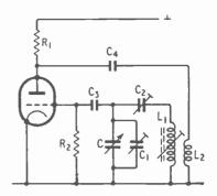
parallel-fed via  $C_4$ .  $R_2$  and  $C_3$  are the usual grid leak and capacitor for making the oscillation generate its own negative bias (p. 217).
