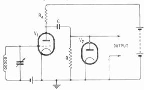
Fig. 17.1—This resistance-coupled amplifier is of little or no value for r.f. amplification
