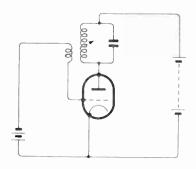
Fig. 12.5—The reaction-coil valve oscillator circuit
