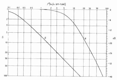
Fig. 18.7—Comparison on an equal-gain basis of a stage of amplification with two tuned circuits (curve a) with a single tuned circuit given a high magnification by positive feedback (b)
