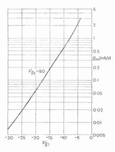
Fig. 19.20—Mutual conductance plotted against  $V_{g_1}$  for the valve represented by b in Fig. 19.19
