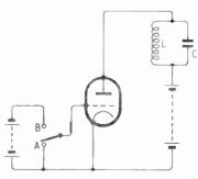
Fig. 12.1—Valve-operated device for setting up oscillations in the circuit LC
