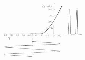
Fig. 13.2—" Class C" operation. Comparing this with Fig. 13.1, we see that the working grid bias (-35 V in this example) is considerably more than enough to cut off anode current, which flows during only part of the positive half-cycles of signal
