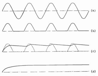
Fig. 23.3—(a) Original a.c.; (b) after rectification; (c) the effect of a reservoir capacitor; (d) after passing through a smoothing filter
