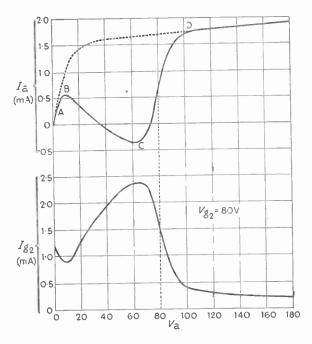
Fig. 17.8—The dotted line indicates the shape the anode-current curve would take but for secondary emission, which in tetrodes causes the curious departure BC. The corresponding variation in screen-grid current is graphed below
