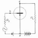
take no account of any loss in  $R_S$ . If this stage were followed by another identical one,  $R_L$  would be shunted by the  $r_{iu}$  of the next stage, which would bring it down to 1,350. raising  $A_I$  to 43.5 but reducing  $A_V$  to 30 and  $A_P$  to 1,300 (31 dB).
