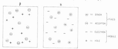
Fig. 10.5—Simplified representation of pieces of impure germanium, showing only the electric charges of broken impurity atoms. In p-type material the mobile charges are predominantly positive (holes), and in n-type material negative (electrons)
