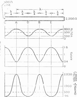
Fig. 14.6 — Diagrams of voltage, current, and (as a result) impedance at the load end of an unmatched transmission line, showing standing waves
