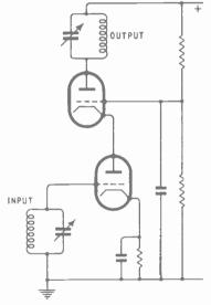
Fig. 19.10-Cascode amplifier circuit
