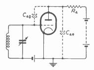
Fig. 17.2—The reasons for the lack of success with Fig. 17.1 are the capacitances from anode to grid and earth, shown here dotted
