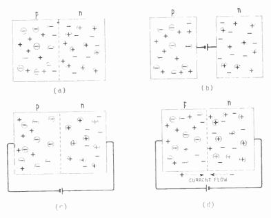
Fig. 10.6—Some mobile charges stray across an undefended frontier (a) causing an excess of negative on the p side and positive on the n side; this can be represented symbolically as at b. An external e.m.f. connected + to n (c) increases this p.d. against itself, sealing the circuit against current flow; but with + to p (d) it reduces or even removes the p.d. and current tlows freely
