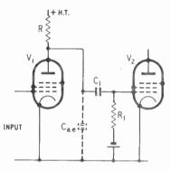
Fig. 20.6—Simple form of resistance-coupled amplifier. Cae denotes unavoidable stray capacitance
