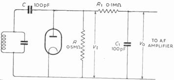
Fig. 16.10—To prevent the r.f. voltages left over after rectification being passed on to the a.f. amplifier, a simple filter, R<sub>1</sub> and C<sub>1</sub>, is commonly used. The component values shown are typical
