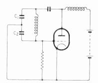
Fig. 12.8—Parallel-fed Colpitts circuit
