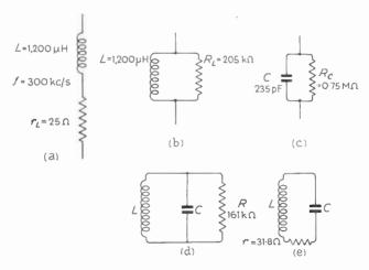
Fig. 8.15—Example to illustrate series and parallel equivalents. b is equivalent to a; and d and e are alternative ways of expressing the result of combining c with b
