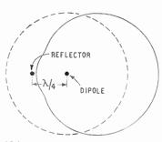
Fig. 15.9—Showing how the equalall-round radiation of Fig. 15.8 (a) (repeated here dotted) is modified by an unconnected dipole placed quarter of a wavelength away from the first, and of such a length as to have a 45° phase angle
