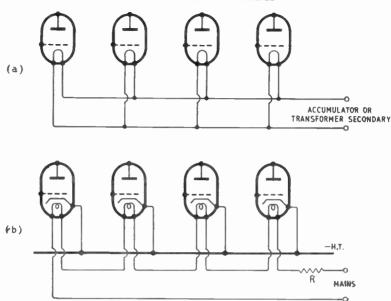
Fig. 23.2—Diagram a shows the usual method of connecting the filaments of battery valves or heaters of a.c. valves, namely, in parallel. To run heaters direct from either d.c. or a.c. mains, they are connected in series, as at b. Note that in spite of the different potentials of the heaters all cathodes can be joined to — b.t.
