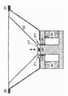
Fig. 20.22—Cross-section of a moving-coil loudspeaker
