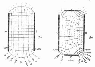
Fig. 21.2—Diagrams to illustrate electrostatic focusing
