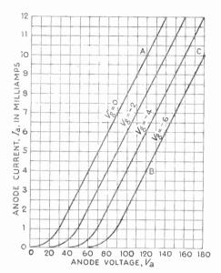
Fig. 9.5—Characteristic curves of triode valve, at different grid voltages. (These curves are somewhat idealized, being straighter and more parallel than in actual practice)
