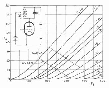
Fig. 12.10—The oscillatory circuit LC is equivalent at resonance to a high resistance R and the voltage across it can be derived from a load line on the valve characteristic curves. From this follows the proportion to be fed back to the grid to sustain oscillation
