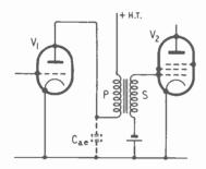
Fig. 20.8 — Simple transformercoupled amplifier circuit
