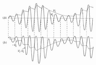
Fig. 16.7—In diagram a,  $V_1$  represents a modulated r.f. input voltage and  $V_c$  the resulting output voltage. In diagram b, the full line shows  $V_1 - V_c$ ; i.e., the voltage across the diode
