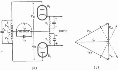
Fig. 16.17—(a) Circuit of phase discriminator for f.m. detection, arranged to bring out the principle: L<sub>p</sub> and L<sub>b</sub> are the primary and secondary windings of the input r.f. transformer; (b) vectors of voltages marked, for carrier wave frequency. Dotted lines indicate the effect of f.m. deviation
