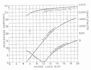
Fig. 20.15—Output and harmonic distortion related to load resistance for a pentode
