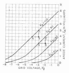
Fig. 9.6—Four samples of anodecurrent/grid-voltage characteristic curve, each taken at a different anode voltage
