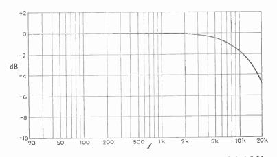
Fig. 20.7—Frequency curve of the amplifier of Fig. 20.6 when  $r_a$  of  $V_1$  is 1.5 M $\Omega$ , R and  $R_1$  in parallel is 0.5 M $\Omega$ , and  $C_{ae}$  is 30 pF, showing falling-off (in decibels) at the top audio frequencies due to  $C_{ae}$
