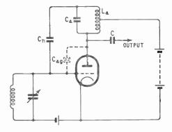
As transistors are still in the triode stage of development, neutralization is used in r.f. transistor amplifiers (p. 352). It is still used to some extent in the r.f. amplifying stages of fixed-frequency senders. But in receivers for tuning over a wide range of frequencies it is difficult to obtain a single setting of  $C_n$  for them all, and a more satisfactory solution was found which will now be considered.
