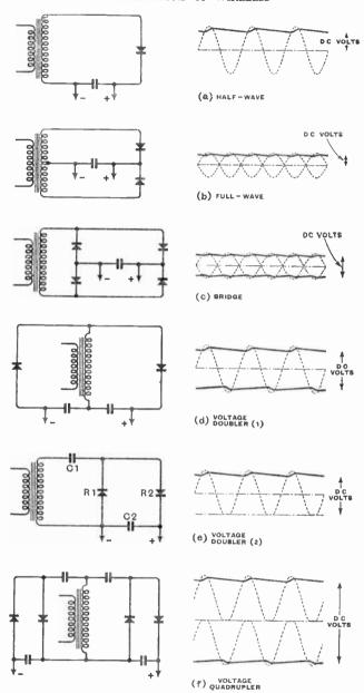
Fig. 23.5—Comparison of various rectifier circuits, the voltage supplied from the transformer being the same in all. Note the comparative output voltages
