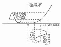
Fig. 16.15—Graph of one-way or z.f. voltage derived from a rectifier is plotted against r.f. input voltage. It enables the distortion of the modulation to be ascertained for any r.f. amplitude and depth of modulation. The input curve here represents 50% modulation
