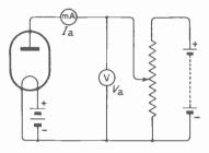
Fig. 9.2—Circuit for finding the relationship between the anode voltage  $(V_a)$  and the anode current  $(I_a)$  in a diode
