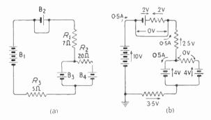
Fig. 2.12—(a) is an imaginary circuit for illustrating the meanings of e.m.f. and p.d. The voltages and currents in different parts of it are marked in (b). Arrows alongside voltages show the direction of rise of potential
