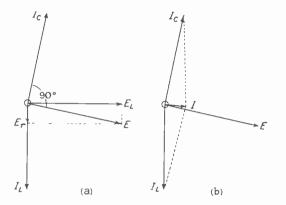
Fig. 8.11—(a) Modification of Fig. 8.9 to allow for the presence of resistance as in Fig. 8.10
