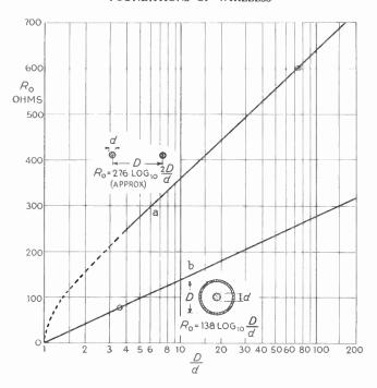
Fig. 14.4—Graphs showing characteristic resistance (R<sub>0</sub>) of (a) parallelwire and (b) coaxial transmission lines in terms of dimensions
