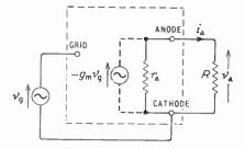
equivalent circuit must give the same answers as the voltage-generator circuit. We have already calculated the output voltage  $(v_a)$  with the help of the voltage-generator circuit (p, 144); it is
