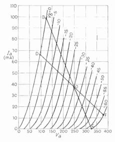
Fig. 20.12—Two trial load lines drawn on a curve sheet relating to a triode output valve. With load line BOC the distortion is excessive (see Fig. 20.3, which was derived from this). The higher resistance represented by DOF is better
