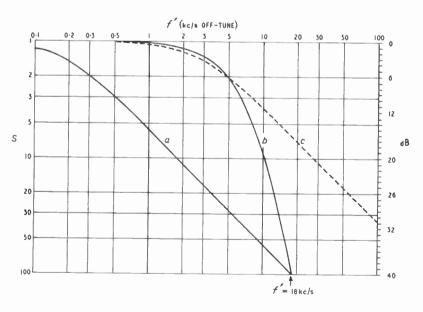
Fig. 18.8—Response curves of one (a) and six (b) tuned circuits on a basis of equal selectivity at 18 kc/s, showing how the six preserve sideband frequencies much better. Curve c refers to a single tuned circuit with its resonance flattened to give equal response at 5 kc/s off-tune
