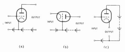
Fig. 22.3—The three basic amplifier configurations of a valve
