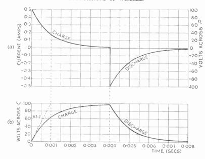
Fig. 3.6—These curves show the current and voltage in the circuit of Fig. 3.5 during charge and discharge
