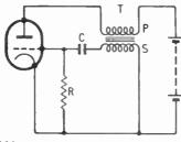
Fig. 21.8—Blocking oscillator circuit
