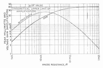
Fig. 11.4—The full line shows how the voltage amplification depends on the value of load resistance R. It is calculated for a valve with  $\mu=39$  and  $r_{\rm A}=14.5~{\rm k}\,\Omega$ . The dotted line shows the peak milliwatts delivered to R for a grid input of 1 V peak.
