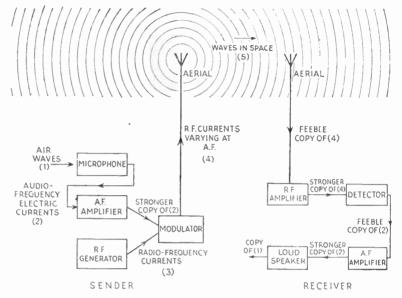
Fig. 1.9—The wireless telegraph of Fig. 1.8 converted into a wireless telephone by controlling the output of the sender by sound waves instead of just turning it on and off.
