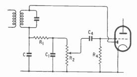
Fig. 16.13—Alternative arrangement in which the negative grid bias for the a.f. amplifier is developed across a grid leak ( $R_4$ ) of exceptionally high resistance
