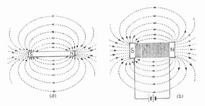
Fig. 4.1—The dotted lines indicate the direction and distribution of magnetic field around (a) a permanent bar magnet, and (b) a cwil of wire carrying current
