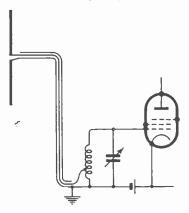
Fig. 17.10—Although it does not provide for balancing to earth, this simple method of connecting a dipole aerial to the receiver by means of a coaxial feeder is often used
