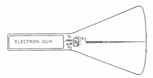
Fig. 21.3—Arrangement of deflector plates in a cathode-ray tube
