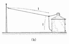
moderately by adding a horizontal portion, as in the familiar T or inverted L aerials, Fig. 15.15. The effect of the horizontal extension is to localize the bulk of the capacitance in itself so that the current in the vertical part, instead of tailing off to zero, remains at nearly the maximum and therefore radiates more. The top portion radiates too, but with a different polarization, so the addition due to it may not be very noticeable in a vertical receiving aerial.
