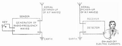
Fig. 1.8—Elementary wireless telegraph. Currents flow in the receiving headphones and cause sound whenever the sender is radiating waves
