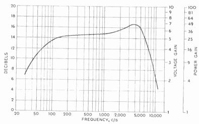
Fig. 20.1—A typical a.f. gain/frequency curve, with logarithmic scales in both directions
