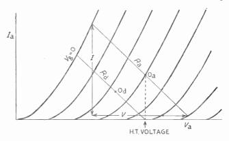
Fig. 20.10—Rd is a typical load line for a direct resistance load. Ra represents a load having negligible resistance to d.c. and the same resistance to a.c. as Rd
