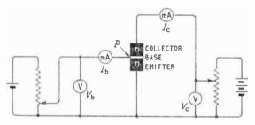
Fig. 10.13—Arrangement, similar to Fig. 9.4, for obtaining characteristic curves of a transistor
