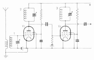
Fig. 17.13-Two-stage r.f. amplifier, using tuned-anode couplings
