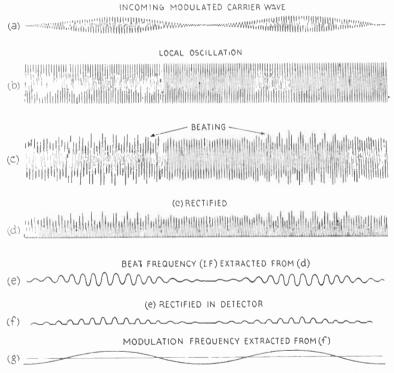
Fig. 19.2—In this diagram the sequence of Fig. 19.1 is elaborated to show what happens when the incoming carrier wave is modulated. The additional lines, (f) and (g), show the extraction of the modulation frequency
