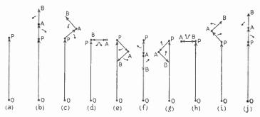
Fig. 18.3—Progressive series of vector diagrams, showing how adding a pair of oppositely-rotating vectors (PA and AB) alternately lengthens and shortens the original vector (OP) without affecting its phase
