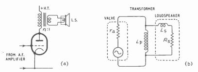
Fig. 20.9—(a) Circuit of output stage in its simplest form. Electrically this can be approximately represented by the generator circuit (b)
