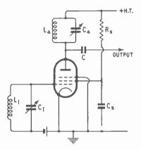
Fig. 17.9—Mødification of Fig. 17.4 to convert it into a workable amplifier circuit by using a screened valve
