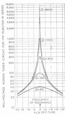
Fig. 18.1—Showing how r.f. voltage across a tuned circuit varies with frequency at different Q values, obtained by adjusting positive feedback
