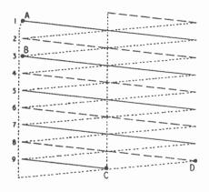
Fig. 21.9—Nine-line interlaced "raster". The dotted lines are fly-backs, which normally are invisible
