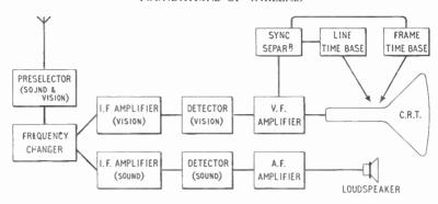
Fig. 21.10-Block diagram of a television receiver
