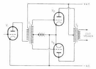
Flg. 20.20—Two output valves, V, and V, in push-pull
