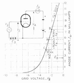
Fig. 9.7-The result of applying an alternating e.m.f. (vg) to the grid of a triode can be worked out from the  $I_a/V_g$  curve, as here. The fixed starting voltage,  $E_6$ , in this case is -2.5 V
