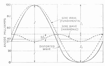
Fig. 20.11—Fig. 20.3 c again, with symbols added for convenience in deriving a formula for percentage second-harmonic distortion.  $I_1$  is the peak value of the fundamental current, and  $I_2$ , of the harmonic;  $I_3$  is the peak current of the larger half-cycle of the distorted current, and  $I_3$  the smaller
