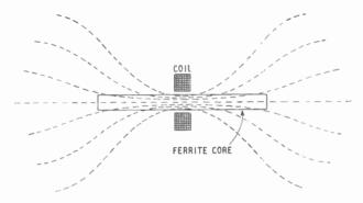
Fig. 15.17—The concentrating effect of a suitable magnetic core on the magnetic field of the waves greatly increases the effectiveness of a small coil as an aerial
