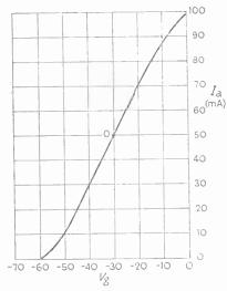
Fig. 20.4—Non-linearity of this kind does not cause second-harmonic distortion, for the half-cycles of anode current resulting from equal half-cycles of grid voltage are also equal; but it does introduce third-harmonic distortion
