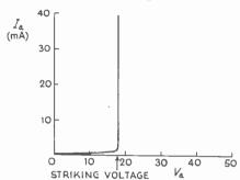
gas. Beyond that point the slope resistance is nil, and if the current were not limited by the external circuit resistance it would very soon destroy the valve. This striking voltage is therefore the voltage drop across the valve, almost regardless of the current flowing.
