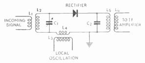
Fig. 19.3—Simple type of frequency-changer, in which the incoming signal and the local oscillation are added together by connecting their sources in series, and then rectified
