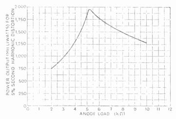
Fig. 20.13—The results of calculating the output power at 5% second-harmonic distortion in Fig. 20.12 for various values of load resistance
