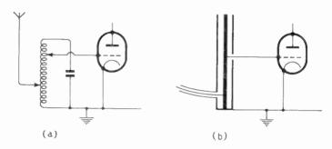
Fig. 14.9—(a) Conventional aerial input circuit using "lumped" components, and (b) distributed equivalent using a quarter-wave coaxial line
