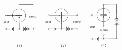
Fig. 22.4—The three basic amplifier configurations of a transistor, corresponding to Fig. 22.3
