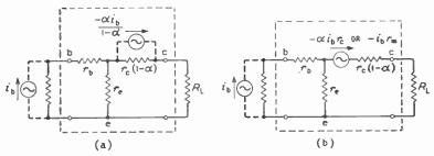
Fig. 22.6—Common-emitter T circuits corresponding to the common-base circuits of Fig. 22.5, using the same symbols
