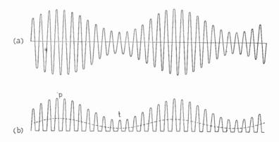
Fig. 16.1—(a) Sample of an amplitude-modulated carrier wave, similar to Fig. 13.5 c. The average value of each cycle is zero; but if one half of each is eliminated (b) the average value of the other halves, shown dotted, fluctuates in the same manner as the modulating waveform (e.g., Fig. 13.5 a)
