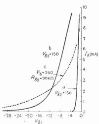
Fig. 19.19— $I_0/V_{g_1}$  curves of (a) an ordinary screened pentode, (b) a variable-mu type, and (c) a variable-mu valve with  $g_2$  fed through a resistor so that  $V_{g_2}$  rises as —  $V_{g_1}$  is increased
