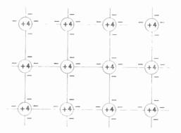
Fig. 10.1—Diagrammatic representation of the four-fold linkage of germanium atoms to form a perfect crystal. The "valency" electrons responsible are shown as four minus signs
