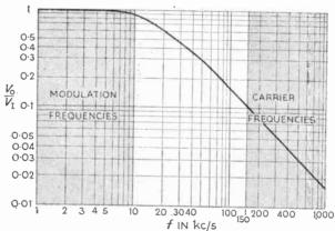
Fig. 16.11—The filtering action of R, C, in Fig. 16.10 is here shown as a graph of  $V_o/V_t$  against frequency
