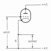
must be less than 1, no matter what the characteristics of the valve and the value of R. The value of B in the formula given on p. 312 is 1, so the "gain" is A/(1+A) as just found. If A is made large by using a high- $\mu$  valve and high R, the output is very nearly as much as the input, but never quite as much. A stage that gives out less voltage than is put in may not appear worthy of further attention; but it is too soon to jump to such a conclusion.
