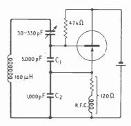
especially with changes in temperature. And whereas the input impedance of a valve is so high at all negative grid voltages that driving it beyond cut-off makes little difference, driving a transistor beyond cut-off reduces its input resistance from perhaps less than  $1 \ k\Omega$  to more than  $100 \ k\Omega$ . If this impedance were closely coupled to the tuned circuit, one half of each cycle would be much more heavily damped than the other and the waveform would be distorted.
