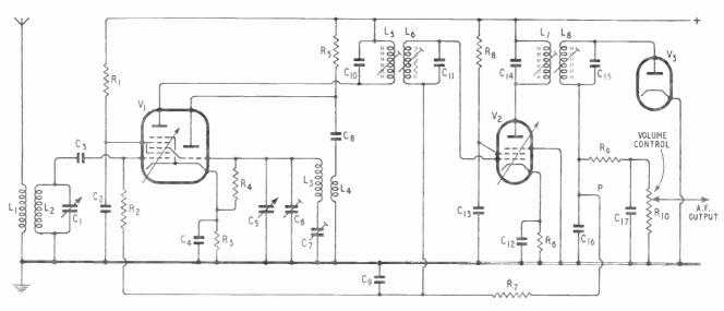
Fig. 19.21—Circuit diagram of a typical superheterodyne receiver from aerial to volume control, including frequency-changer, i.f. amplifier and detector stages, with automatic gain control
