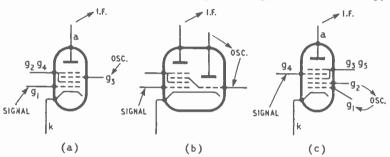
Fig. 19.6—Some frequency-changer valves: (a) hexode; (b) triode-hexode; (c) heptode
