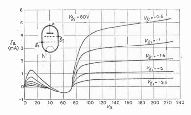
Fig. 17.7—Characteristic curves of a screened tetrode of the original type, which has now gone out of use
