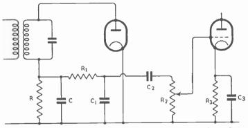
Fig. 16.12—Typical detector circuit, in which R is the load resistor, C the reservoir, R<sub>1</sub>C<sub>1</sub> the r.f. filter, R<sub>1</sub>C<sub>2</sub> the z.f. filter, R<sub>1</sub> the volume control, R<sub>1</sub> the biasing resistance, and C<sub>2</sub> its by-pass
