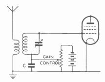
Fig. 19.16—Method of controlling the amplification (or gain) of a valve by adjusting its grid bias
