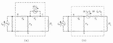
Fig. 22.5—Equivalent T circuits of a common-base-connected transistor: (a) current generator; (b) voltage generator
