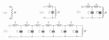
Fig. 14.3—Synthesis of transmission line from basic circuit elements
