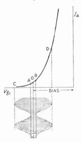
Fig. 19.17—Showing how the average slope of the valve curve varies during each modulation cycle of a strong signal
