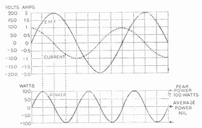
Fig. 6.8—The current and voltage graphs for a capacitance load (Fig. 6.4) are here repeated, with a power graph derived from it plotted helow
