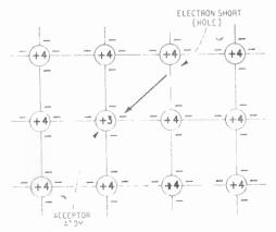
Fig. 10.4—Showing how the perfect crystal is modified when an impurity atom with three valency electrons occupies a place
