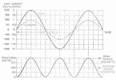
Fig. 5.2—Time graphs of e.m.f., current and power in the circuit Fig. 5.1
