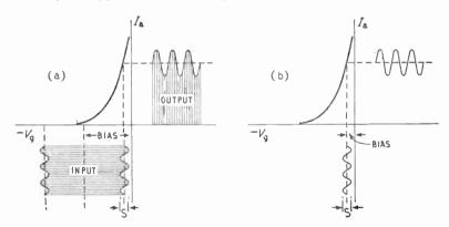
Fig. 19.7—Diagram showing how conversion conductance compares with mutual conductance
