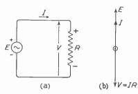
Fig. 5.8—(a) A.c. circuit at the instant when the e.in.f. is at its positive maximum, and (b) the corresponding vector diagram
