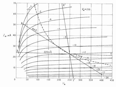
Fig. 20.14—Typical I<sub>a</sub> V<sub>a</sub> curves for a small output pentode. The line AOC represents a usual load
