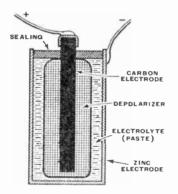
Fig. 23.1—Cross-section of a dry cell, showing the essential parts
