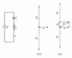
Fig. 18.5—Vector diagrams of a tuned circuit, (a) exactly at resonance, and (b) off resonance, showing how the total impedance increases from r to z
