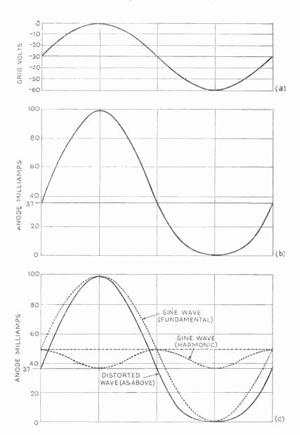
Fig. 20.3—Showing that the distorted output (b) resulting from applying the input (a) to the valve whose characteristics are given in Fig. 20.2 is equivalent to (c) the combination of an undistorted wave with its second harmonic
