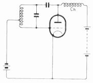
Fig. 12.7— Parallel-fed Hartley circuit with the anode current supplied through a choke Ch.
