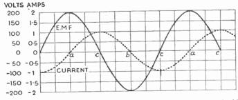
Fig. 7.2—E.m.f. and current graphs for Fig. 7.1, drawn to correspond with Figs. 5.2 and 6.4
