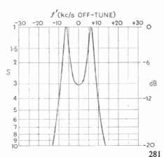
Fig. 19.14—The result of trying to maintain sidebands when using excessively selective coils in a bandpass filter—the "rabbit's ears" produced by over-coupling
