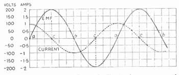
Fig. 6.4—E.m.f. and current diagram for Fig. 6.1, drawn to correspond with Fig. 5.2
