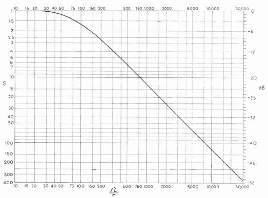
Fig. 18.6—Generalized resonance curve for any single tuned circuit. To make it refer to any particular circuit, divide the numbers on the horizontal scale by L/r (or by  $Q/2\pi f_r$ ) to convert them to a scale of f'. The units are: L in  $\mu H$ ; r in  $\Omega$ ; f' in kc/s;  $f_r$  in Mc/s
