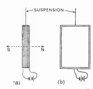
Fig. 4.4—A coil carrying current, and free to rotate, sets itself with its axis pointing N and S. a is a side view and b an end view
