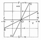
Fig. 16.2—Characteristic curves of various linear resistances. The line COD is seen to represent 500  $\Omega$ . If the resistance to negative voltages is different from that to positive, as shown for example by the line COB. the result is a partial rectifier
