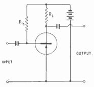
Fig. 22.9—This method of applying base current bias to a transistor, via R<sub>b</sub>, is unsatisfactory in practice
