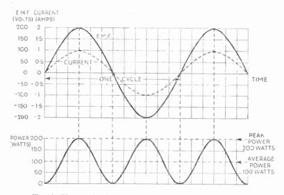
Fig. 44-Time graphs uf e.m.f., current and power in the circuit Fig. 43
