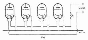
Fig. 213—Diagram a shows the usual method of connecting the filaments of battery valves or heaters of a.c. valves, namely, in parallel. To run heaters from d.c. mains, they are connected in series, as at b. Note that in spite of the different potentials of the heaters all cathodes can be joined to -h.t.
