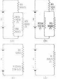
Fig. 24—The current through and voltage across each resistor in this complicated network can be calculated by applying the two simple rules derived from Figs. 22 and 23
