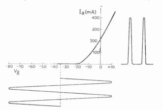
Fig. 110—" Class C " operation. Comparing this with Fig. 109, we see that the working grid bias (-35 V in this example) is considerably more than enough to cut off anode current, which flows during only part of the positive half-cycles of signal
