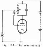
valve oscillator circuit
