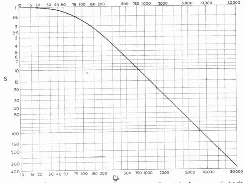
Fig. 172—Generalized resonance curve for any single tuned circuit. To make it refer to any particular circuit, multiply the numbers on the horizontal scale by r/L (or by  $2\pi f_r/Q$ ) to convert them into a scale of f'
