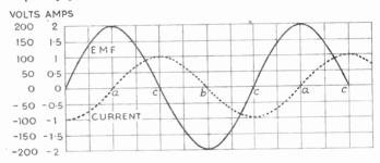
Fig. 66-E.m.f. and current graphs for Fig. 65, drawn to correspond with Figs. 44 and 55
