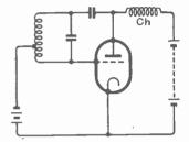
Fig. 105 — Parallel-fed Hartley circuit with the anode current supplied through a choke Ch. The grid bias is series-fed
