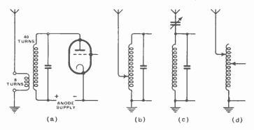
Fig. 119—Some of many varieties of method in coupling aerial to sender. a is the inductive coupling or r.f. transformer method, worked out in the text for a particular example; b is the aerial tapping or auto-transformer; c is the series capacitor method; and at d the valve is tapped down to reduce the effective load resistance
