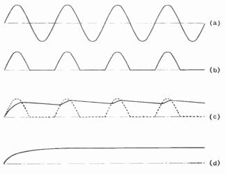
Fig. 214—(a) Original a.c.; (b) after rectification; (c) the effect of a reservoir capacitor; (d) after passing through a smoothing filter
