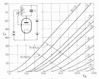
Fig. 108—The oscillatory circuit LC is equivalent at resonance to a high resistance R and the voltage across it can be derived from a load line on the valve characteristic curves. From this follows the proportion to be fed back to the grid to sustain oscillation
