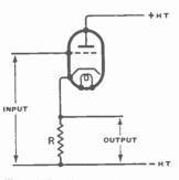
Fig. 207 - Simplest form of cathode-follower circuit Fig. 207.
