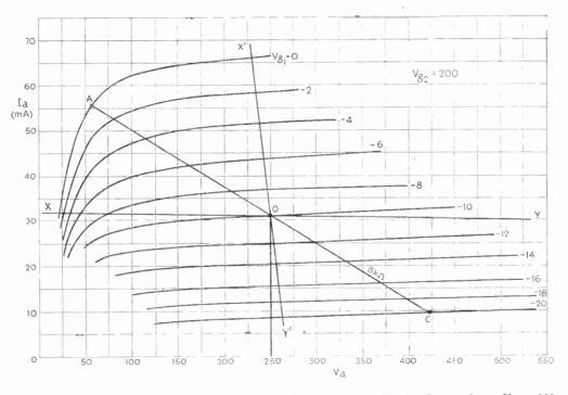
Fig. 204—Typical output-pentode curves. The line AOC represents a usual load. Curves taken at  $V_{g_1} = 200$
