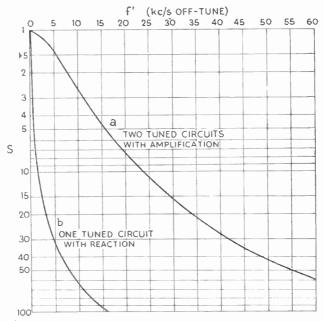
Fig. 173—Comparison of (a) two ordinary tuned circuits plus valve amplification (A = 50) with (b) a single tuned circuit made to give equal signal output at resonance by means of reaction, showing the poor selectivity of a and the sideband-cutting of b
