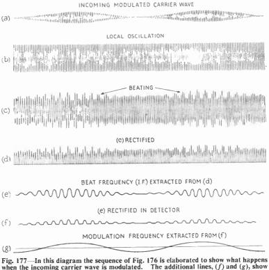
when the incoming carrier wave is modulated. The additional lines, (f) and (g), show the extraction of the modulation frequency
