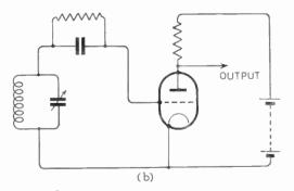
Fig. 139—If a diode detector (Fig. 138c variety) is connected straight to a triode amplifier (a), the gridcathode path of the triode renders a separate diode unnecessary; this is what happens in the grid type of detector (b)
