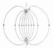
Fig. 30—The dotted lines indicate the direction and distribution of electric field between two oppositely-charged terminals, A and B
