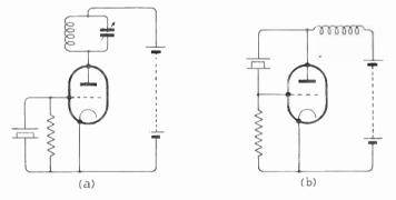
Fig. 112-Two types of crystal-controlled oscillator circuit
