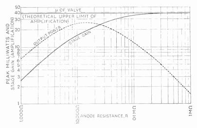
Fig. 98—The full line shows how the voltage amplification depends on the value of load resistance R. It is calculated for a valve with  $\mu = 39$  and  $r_a = 14.5 \text{ k}\Omega$ . The dotted line shows the peak milliwatts delivered to R for a grid input of 1 V peak. The maximum power is obtained when  $R - r_a$ .
