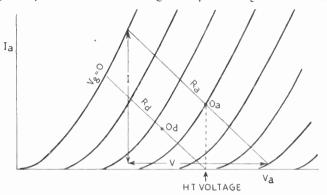
Fig. 200— $R_{\rm d}$  is a typical load line for a resistance load as in Fig. 96.  $R_{\rm a}$  represents a load having negligible resistance to d.c. and the same resistance to a.e. as  $R_{\rm d}$
