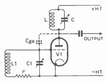
Fig. 157 –The grid-to-anode capacitance of V1 ( $C_{ga}$ ) causes difficulty in working the tuned-anode amplifier
