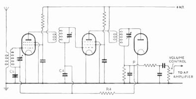
Fig. 169—Circuit diagram of the r.f. amplifier and detector portion of a receiver, showing automatic gain control
