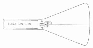
Fig. 222-Arrangement of deflector plates in a cathode-ray tube
