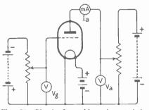
Fig. 91—Circuit for taking characteristic curves of a triode
