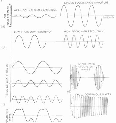
Fig. 8—Graphical representation of the four basic ways in which sound (or any other) waves can differ. (a) amplitude; (b) pitch or frequency; (c) waveform; and (d) envelope
