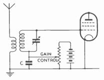
Fig. 163—One possible method but not a good one---of controlling signal strength
