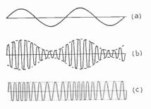
Fig. 116—Curve (a) represents 2 cycles of audio [frequency used to modulate a r.f. carrier wave. If amplitude modulation is used, the result is represented by (b); if frequency modulation, by (c)
