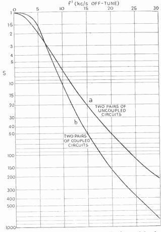
Fig. 185—In this comparison between coupled and uncoupled tuning circuits, two pairs are used, and the r.f. resistance of the coupled circuits (for which L/r=20) is half that of the uncoupled circuits (L/r=10)
