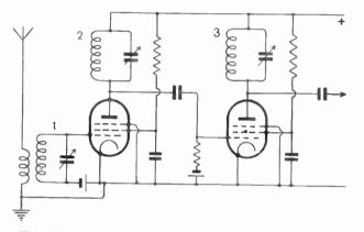
Fig. 162-Two-stage r.f. amplifier, using tuned-anode couplings
