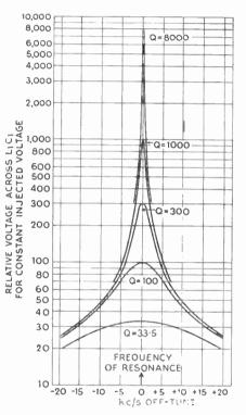
Fig. 152—Showing how r.f. voltage across a tuned circuit varies with frequency at different Q values, obtained by adjusting the reaction control
