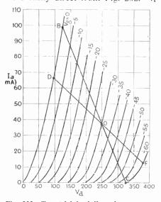
Fig. 202—Two trial load lines drawn on a curve sheet relating to a triode output valve. With load line BOC the distortion is excessive (see Fig. 192, which was derived from this). The higher resistance represented by DOF is better
