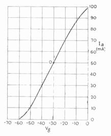
Fig. 193—Non-linearity of this kind does not cause second-harmonic distortion, for the half-cycles of anode current resulting from equal half-cycles of grid voltage are also equal; but it does introduce thirdharmonic distortion
