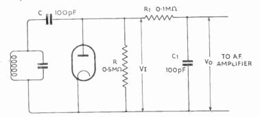
Fig. 140—10 prevent the r.f. voltages left over after rectification being passed on to the a.f. amplifier, a simple filter,  $R_1$  and  $C_1$ , is commonly used. The component values shown are typical
