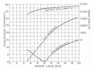
Fig. 205—Output and harmonic distortion related to load resistance for the pentode of Fig. 204. Working point O; input signal 10 V peak
