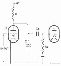
Fig. 195-Simple form of resistancecoupled amplifier. C denotes the unavoidable stray eapacitance
