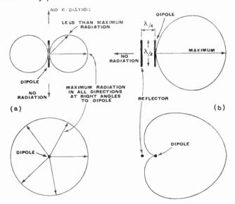
Fig. 129—Polar diagrams of radiation from a simple dipole aerial (a), and dipole with reflector (b). The upper diagrams are side views and the lower diagrams end views
