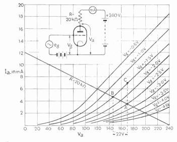
Fig. 96—An example of the problem set by Fig. 95 is here worked out on an  $I_a - V_a$  curve sheet
