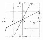
Fig. 132—Characteristic curves of various linear resistances. The line COD, by Ohn's Law, is seen to represent 500 (2). If the resistance to negative voltages is different from that to positive, as shown for example by the line COB, the result is a partial rectifier
