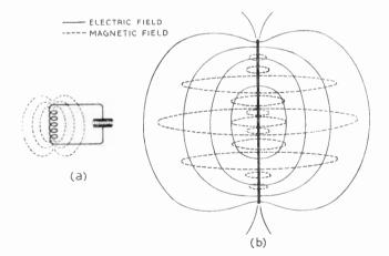
Fig. 122—In a concentrated tuned circuit (a) the electric and magnetic fiedsl are confined and radiation is slight. Opening out the circuit (b) extends the fields and also the radiation
