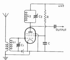
Fig. 161—Modification of Fig. 156 to convert it into a workable amplifier circuit by using a screened valve. Note the method of supplying the screen grid at a lower voltage than the anode, and at the same time avoiding signalfrequency variations in potential
