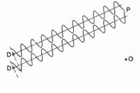
Fig. 130—Showing how the waves from two dipoles radiating in phase arrive at certain angles in completely opposite phase
