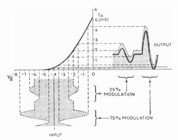
Fig. 146--Illustrating the action of the anode-bend detector with varying depth of modulation
