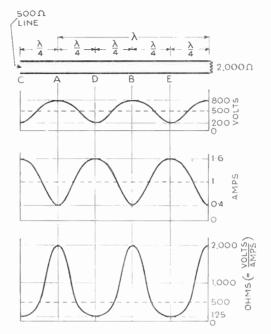
Fig. 232—Diagrams of voltage, current, and (as a result) impedance at the load end of an unmatched transmission line, showing standing waves
