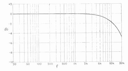
Fig. 196—Frequency curve of the amplifier of Fig. 195 when  $r_a$  of VI is 1.5 M  $\Omega_c$ , R and R, in parallel is 0.5 M  $\Omega_c$ , and C is 30 pF, showing falling-off (in decibels) at the top audio frequencies due to C. It has been necessary to assume an abnormally high value for R in order to show appreciable loss in this frequency band
