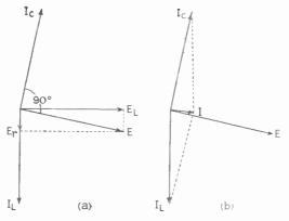
Fig. 83—(a) Modification of Fig. 81 to allow for the presence of resistance as in Fig. 82. As the two branch currents  $I_c$  and  $I_L$  are not exactly opposite in phase, the result of combining them is a small current I (b) nearly in phase with E
