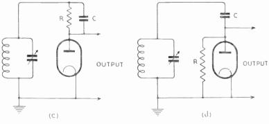
Fig. 138- The principal varieties of diode detector circuit
