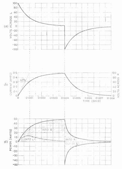
Fig. 41—Curves showing the current, voltage and power in the circuit of Fig. 40 when the switch is moved first to X and then to B
