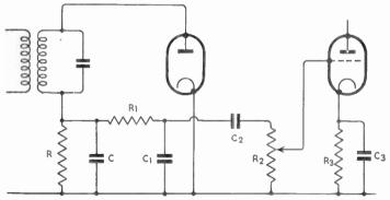
Fig. 142—Typical detector circuit, in which R is the load resistance, C the reservoir,  $R_1 C_1$  the r.f. filter,  $R_2 C_2$  the z.f. filter,  $R_1$  the volume control,  $R_2$  the biasing resistance, and  $C_2$  its by-pass
