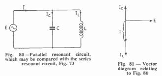
too, that  $I_L$  will lag E by 90°, and  $I_C$  will lead E by 90°; so the currents must be in exactly opposite phase, as were the voltages in Fig. 74. The net current taken from the generator will, therefore, be the simple difference between the two individual currents.
