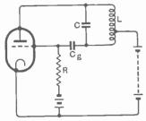
Fig. 104—The series-fed Hartley circuit, showing parallel-fed grid bias using a grid leak R and capacitor  $C_{\kappa}$
