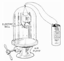
Fig. 7-Experiment to demonstrate that sound waves cannot cross empty space, As the air is removed from the glass vessel, the sound of the bell fades away
