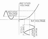
the negative half-cycle almost completely neutralizing the positive half. Small-signal detection is therefore very inefficient.
