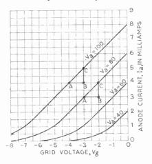
Fig. 93—Four samples of anode-current/gridvoltage characteristic curve, each taken at a different anode voltage
