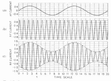
Fig. 113—Curve *a* represents two cycles of andio-frequency current, such as might be flowing in a microphone circuit; *b* represents the nuch larger number of radio-frequency cycles generated by the sender. When these have been modulated by *a*, the result is as shown at *c*
