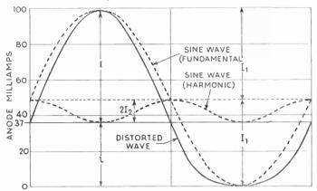
Fig. 201—Fig. 192 c again, with symbols added for convenience in deriving a formula for percentage second-harmonic distortion.  $I_1$  is the peak value of the fundamental current, and  $I_2$  of the harmonic; I is the peak current of the larger half-cycle of the distorted current, and i the smaller
