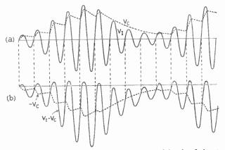
Fig. 137—Ln diagram a,  $V_1$  represents a modulated r.f. input voltage and  $V_0$  the resulting output voltage. The carrier frequency would normally be much higher relative to the modulation frequency, and this would permit a shorter time-constant (= CR) so that  $V_0$ could follow the peaks of  $V_1$  more closely. In diagram b, the full line shows  $V_1 - V_0$ ; i.e., the voltage across the diode
