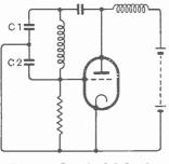
Fig. 106-Parallel-fed Colpitts circuit
