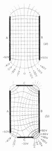
Fig. 221 –Diagrams to illustrate electrostatic focusing, by showing how the nearly parallel lines of force between two plates maintained at opposite potential (a) are bent and made to converge by means of a third electrode C, held at a suitable intermediate potential (b). The dotted lines are equipotential lines
