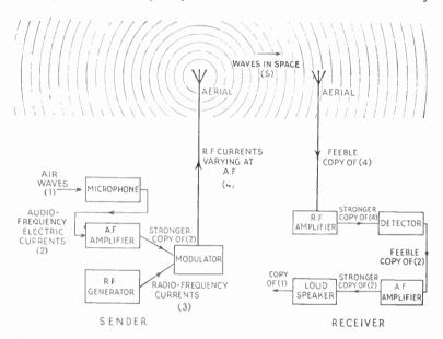
Fig. 15—The wireless telegraph of Fig. 14 converted into a wireless telephone by controlling the output of the sender by sound waves instead of just turning it on and off. In practice it is also generally necessary to use amplifiers where shown
