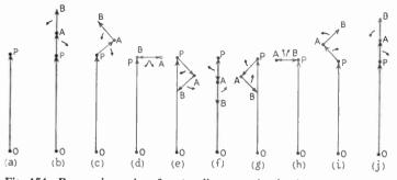
Fig. 154—Progressive series of vector diagrams, showing how adding a pair of oppositely-rotating vectors (PA and AB) alternately lengthens and shortens the original vector (OP) without affecting its phase
