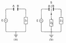
Fig. 158--Illustrating the theory of screening
