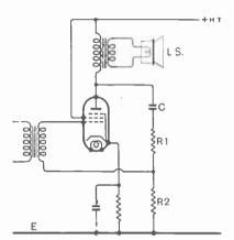
Fig. 206—One circuit arrangement for negative feedback in an output stage.  $R_1$  and  $R_2$  form a potential divider across the output, the voltage developed across  $R_2$  being fed back into the grid circuit in series with the transformer secondary
