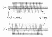
Fig. 166—Comparison between the grid of an ordinary valve (a) and a variable-mu valve (b)
