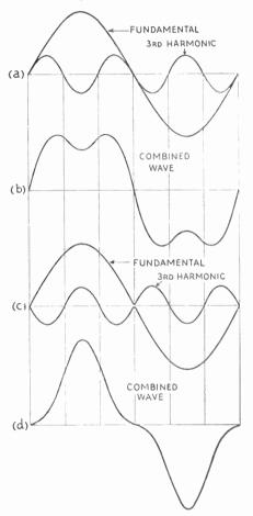
Fig. 194—The waveform resulting from adding together the fundamental and third harmonic seen at a is shown at b. The fundamental and harmonic at c have the same amplitudes and frequencies as at a, and differ only in relative phase, but the waveform of the combination (d) is quite different from b
