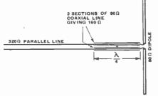
Fig. 233—Example of a quarter-wave length of line being used as a matching transformer
