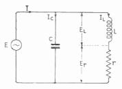
Fig. 82—Parallel resonant circuit with resistance in the inductive branch, which may be compared with Fig. 76
