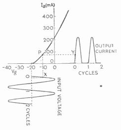
Fig. 109—Illustrating "Class B " operation with the aid of a valve anode-current grid-voltage characteristic curve. The working grid bias nearly cuts off anode current, and only the positive half-cycles of grid signal are effective in reproducing themselves in the form of anode current
