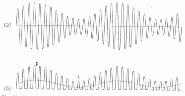
Fig. 131—(a) Sample of a modulated carrier wave, similar to Fig. 113 c. The'' average value of each cycle is zero; but if one half of each is eliminated (b) the average value of the other halves, shown dotted, fluctuates in the same manner as the modulating waveform (e.g., Fig. 113 a)
