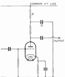
Fig. 219—Decoupling a valve from the h.t. line is performed by inserting R to block signal currents, and providing C to give them a path back to earth
