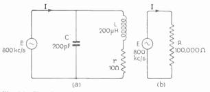
Fig. 84—The circuit composed of C, L and r having the values marked (a) can at 800 kc/s be replaced by a high resistance (b), so far as the phase and magnitude of the current taken by the generator is concerned
