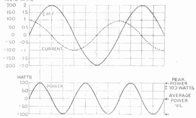
Fig. 59—The current and voltage graphs for a capacitance load (Fig. 55) are here repeated, with a power graph derived from it plotted below. Note that over any complete cycle the total power is zero, because the exact amount put into the capacitor during one half is returned during the other half
