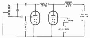
Fig. 115—Anode modulation, sometimes called "choke control" modulation because the audio voltage is developed across an a.f. choke, AFC, which forms the anode load of the modulator valve  $V_w$  and causes the anode voltage delivered to the oscillator valve  $V_o$  to vary in accordance with the audio voltage.  $V_a$  acts simply as a high-power a.f. amplifier. RFC is a r.f. choke for keeping r.f. current out of the modulator circuit
