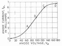
Fig. 90 – Typical characteristic curve of a diode
