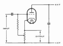
Fig. 208—A more practical form of cathodefollower, in which provision is made for reduced grid bias, and for keeping the anode at a steady voltage
