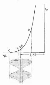
Fig. 165—Showing how the average slope of the valve curve varies during each modulation cycle of a strong signal fore receive quite a large voltage along with that of the weaker station to which the set is tuned.
