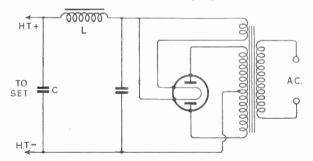
Fig. 218—Full-wave rectifier circuit (b in Fig. 217) fitted with smoothing filter, LC
