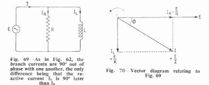
vector diagram, Fig. 70, is therefore with this exception the same as Fig. 63. So we have for the total current  $I = \sqrt{(I_R^2 + I_L^2)}$ ; and as the impedances are inversely proportional to the currents,  $1/Z = \sqrt{(I/R^2 + 1/X^2)}$ , giving as before
