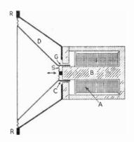
Fig. 211-Cross-section of a movingcoil loudspeaker
