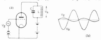
Fig. 102—Diagram b shows the relative amplitude and phase of grid and anode voltages when their frequency is the same as the natural frequency of the circuit LC
