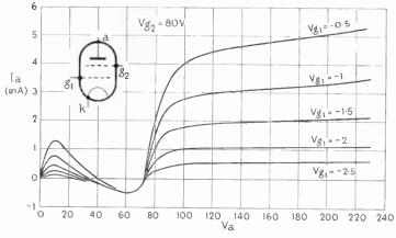
Fig. 159—Characteristic curves of a screened tetrode of the original type, which has now gone out of use
