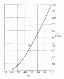
Fig. 191—Typical characteristic curve of a triode, showing non-linearity. If the working point is O (as a result of applying a grid bias of -30 V), a 30 V positive half-cycle of signal on the grid would increase the anode current by 62 mA, but an equal negative half-cycle would decrease it by only 37 mA; see Fig. 192
