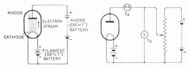
Fig. 88—Electron flow from cathode to anode in a directly-heated diode valve
