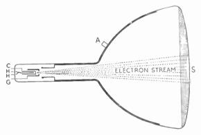
Fig. 220—Section of typical cathode-ray tube of a type in which focusing and deflection are by means of coils round the outside of the neck. H = heater; C = cathode; G = grid; A = anode; S = fluorescent screen
