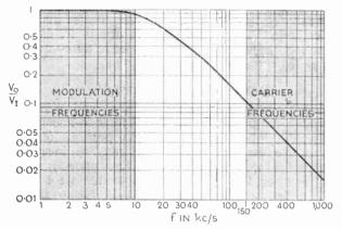
Fig. 141—The filtering action of  $R_{\perp} C_{\perp}$  in Fig. 140 is here shown as a graph of  $V_{\omega}/V_{t}$  against frequency
