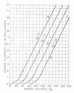
Fig. 92—Characteristic curves of triode valve, each showing change of anode current with change of anode voltage. (These curves are somewhat idealized, being straighter and more parallel than in actual practice)
