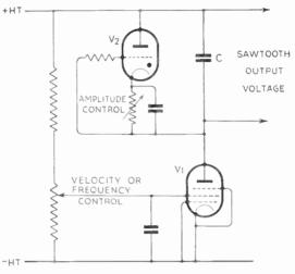
Fig. 225-Outline circuit uf sawtooth generator
