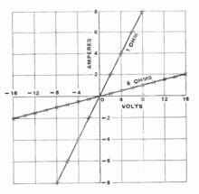
Fig. 18—Graph showing the results of an experiment on the relationship between current in amps and e.m.f. in volts, for two different circuits
