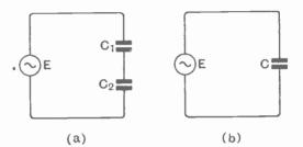
Fig. 58—If the one capacitor C in b is to take the same current as the two in series at a, its capacitance must be equal to  $1 (I_1 C_1 + I C_2)$
