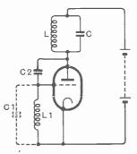
Fig. 107—Tuned-anode tunedgrid (T.A.T.G.) oscillator circuit. The phase-reversing part of the circuit is C. (normally the valve itself) and L
