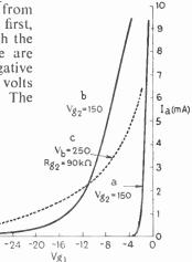
Fig. 167—  $I_a - V_{g_1}$  curves of (a) an ordinary screened pentode, (b) a variablemu type, and (c) a variable-mu valve with  $g_2$  fed through a resistor so that  $V_{g_4}$  rises as  $-V_{g_4}$  is increased
