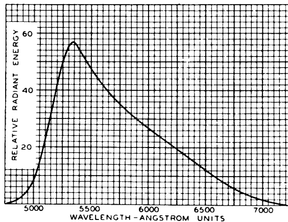
Fig. 5 - Spectral energy characteristic of phosphor No.3.
