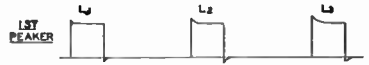
Fig. 6—Effect produced on a square wave with the peaker potentiometer open for various values of inductance (first peaker).
