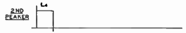
Fig. 7—Effect on a Square Wave with the peaker potentiometer open (second peaker).
