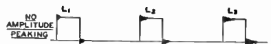
Fig. 9—Effects produced on a square wave by the introduction of various values of inductance in series with a small fixed capacity in the phase shifting sections.
