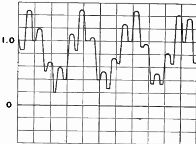
Fig. 9(c) — Combined light intensity of two successive scans of the same line on a black-and-white receiver.
