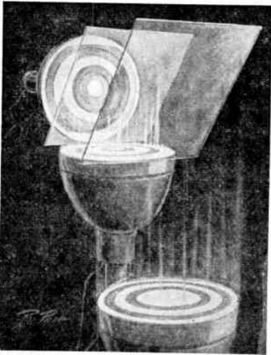
Fig. 8—Direct-view picture-reproducing system using three kinescopes and a pair of dichroic mirrors.
